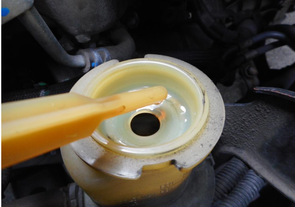
Photo 15 shows the power steering fluid reservoir of the Motor Lorry at the time of my inspection. The power steering fluid was observed to be of sufficient level (arrowed) and without any visible contamination.
