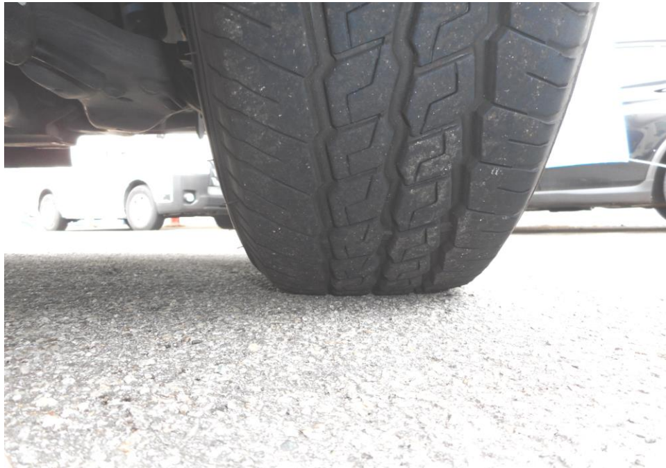
Photo 7 shows the condition of the front right tyre of the Motor Lorry, which was observed to be in serviceable condition with remaining tread depth of approximately 6.6mm. The tyre, which was wrapped around standard steel wheel rim, was also observed to be sufficiently inflated for vehicular operation. There was no tear, cut or burst mark(s) on the outer and the inner sidewalls as well as across the tread of the 4 tyres that were fitted on the Motor Lorry.
