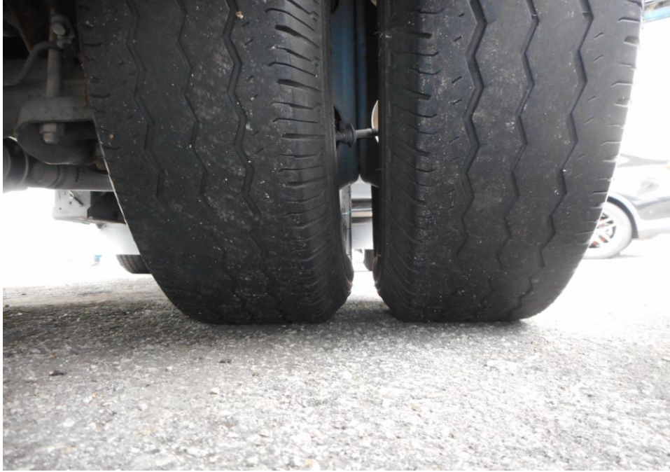
Photo 8 shows the condition of the rear right tyre of the Motor Lorry, which was observed to be in serviceable condition with remaining tread depth of approximately 3 mm. The tyre, which was wrapped around standard steel wheel rim, it was observed to be sufficiently inflated for vehicular operation.
