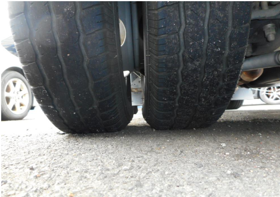
Photo 9 shows the condition of the rear left tyres of the Motor Lorry, which was observed to be in serviceable condition with remaining tread depth of approximately 2.5mm. The tyres, which were wrapped around standard steel wheel rim, were also observed to be sufficiently inflated for vehicular operation. There was also no damage found on all 4 steel wheel rims of the Motor Lorry.
