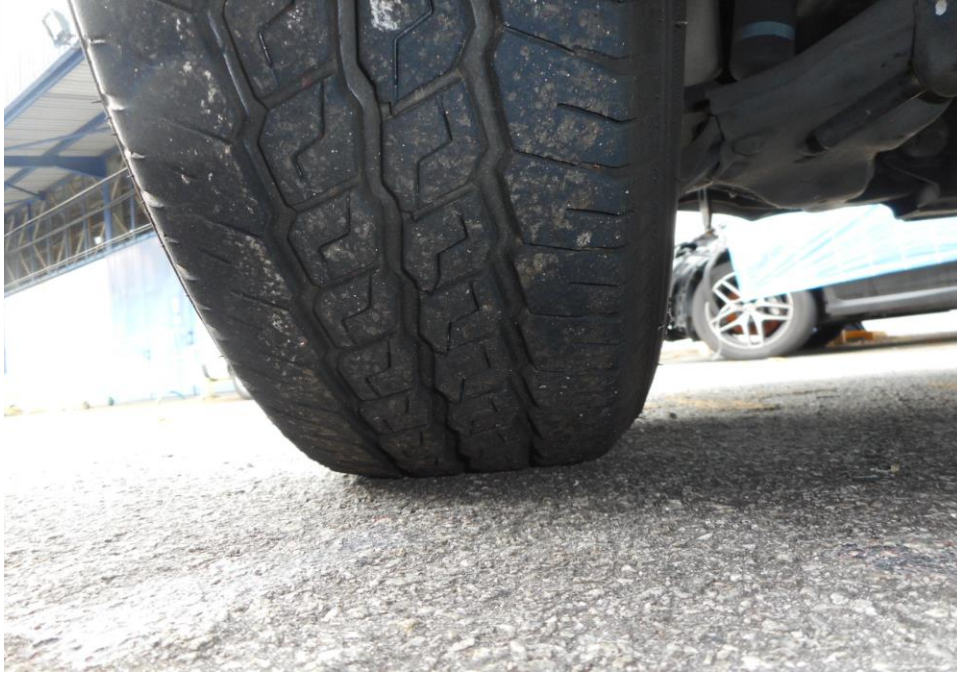
Photo 10 shows the condition of the rear right tyres of the Motor Lorry, which were observed to be in serviceable condition with remaining, tread depth of approximately 6.5mm. There was also no tear, cut or burst mark(s) on the outer and the inner sidewalls as well as across the tread of the 4 tyres that were fitted on the Motor Lorry.
