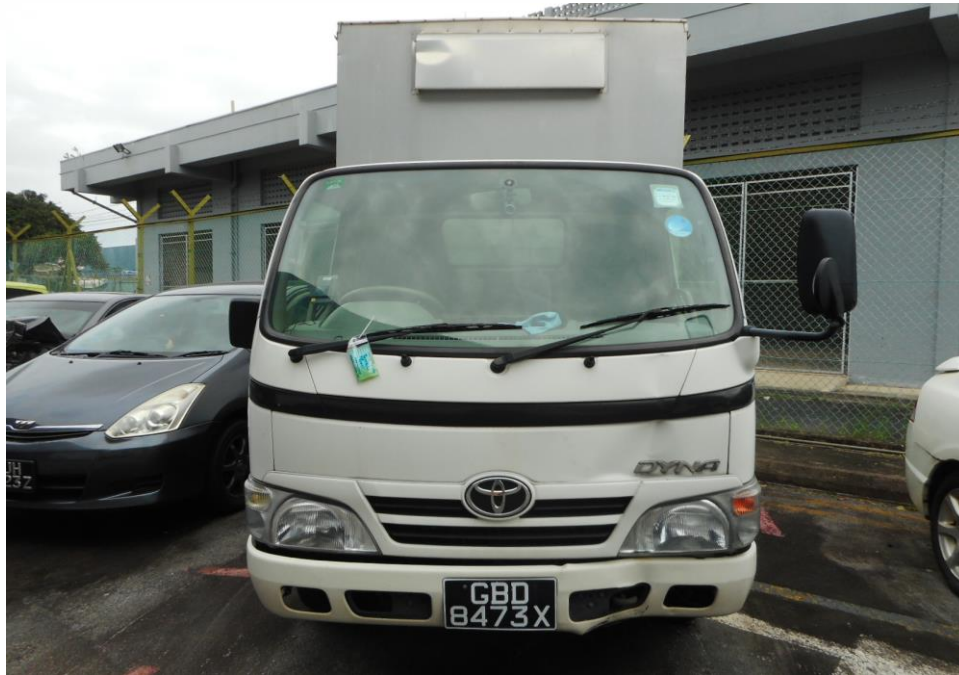
Photo 2 shows a general view of the Motor Lorry's frontal portion at the time of my inspection. It appeared to have sustained damage at its frontal portion. Its front body panel and front bumper were damage at the time of my inspection.
