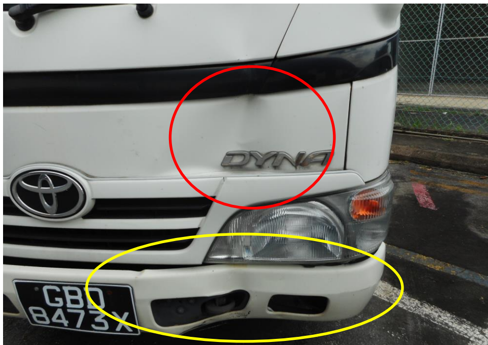
Photo 3 shows a close up view of the Motor Lorry's frontal portion at the time of my inspection. It appeared to have sustained damage at its frontal portion. Its front body panel (red circle) and front bumper (yellow circle) was damage at the time of my inspection as a result of the accident.
