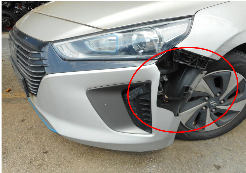
Photo 4 shows the close up view of the Motor Taxi's front body at the time of my inspection. The Motor Taxi was observed to have sustained damage at its front bumper (circled) as a result of the accident.
