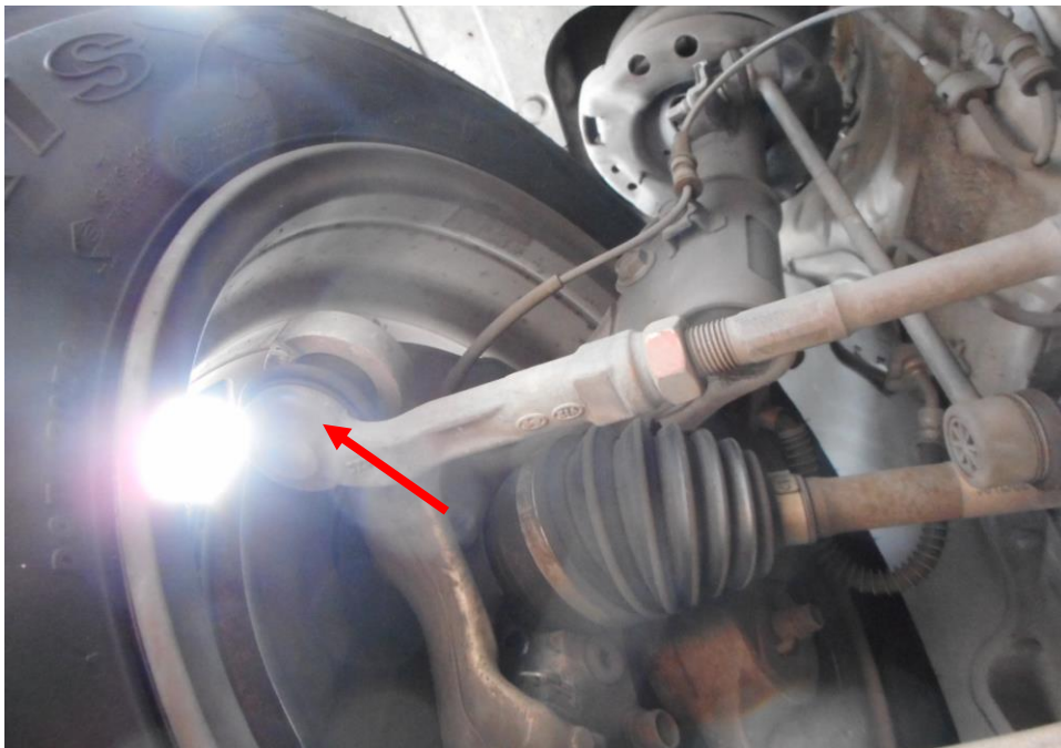
Photo 23 shows the various undercarriage components at the front left wheel of the Motor Taxi, which had included the steering tie rod (red arrow). The various undercarriage components of the Motor Taxi were all found to be intact without any visible damage.
