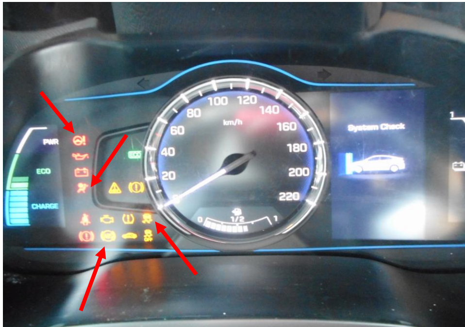
Photo 24 shows the warning light for Anti-Lock Brake System (ABS) and Power Steering System (EPS), Supplemental Restraint System (SRS) and Traction Control (TC) (arrowed) appearing on the instrument panel of the Motor Taxi during the self-test of its various electronic operating systems when its engine was cranked.
