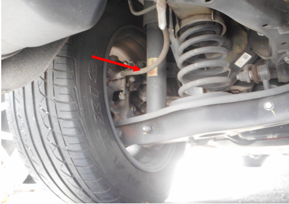
Photo 18 shows the brake hose/pipe (arrowed) at the rear left wheel of the Motor Taxi. I did not observe any leakage of brake fluid at the time of my inspection of the Motor Taxi. Static tests of the Motor Taxi's braking system had indicated that there was no internal leakage of pressure/vacuum. The undercarriage components of the Motor Taxi were also all found to be intact and without any visible damage.
