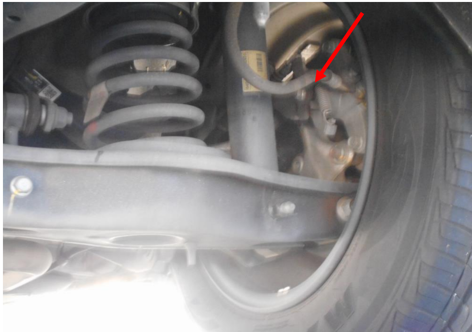
Photo 17 shows the brake hose/pipe (arrowed) at the rear right wheel of the Motor Taxi. No leakage of brake fluid was observed. Visual examination of the various components of the braking system like the drum brake, brake booster, brake pedal etc. had revealed all to be intact and without visible damage.
