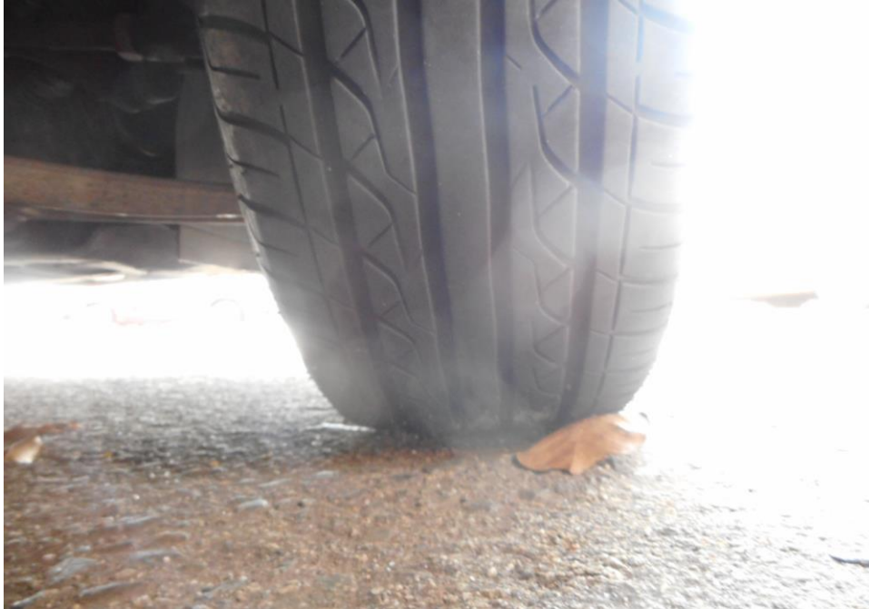
Photo 8 shows the condition of the front right tyre of the Motor Taxi, which was observed to be in serviceable condition with remaining tread depth of approximately 5.1mm. The tyre was sufficiently inflated for vehicular operation with no tear, cut or burst mark(s) on the outer and the inner sidewalls as well as across the tread. The 4 tyres of the Motor Taxi were wrapped around standard steel wheel rims without any damage.
