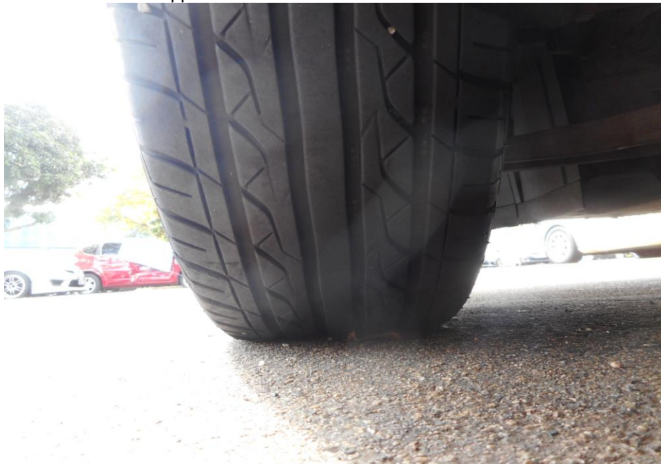
Photo 11 shows the condition of the front left tyre of the Motor Taxi, which was observed to be in serviceable condition with remaining tread depth of approximately 4.6mm. There was also no tear, cut or burst mark(s) on the outer and the inner sidewalls as well as across the tread of the Motor Taxi's 4 tyres.
