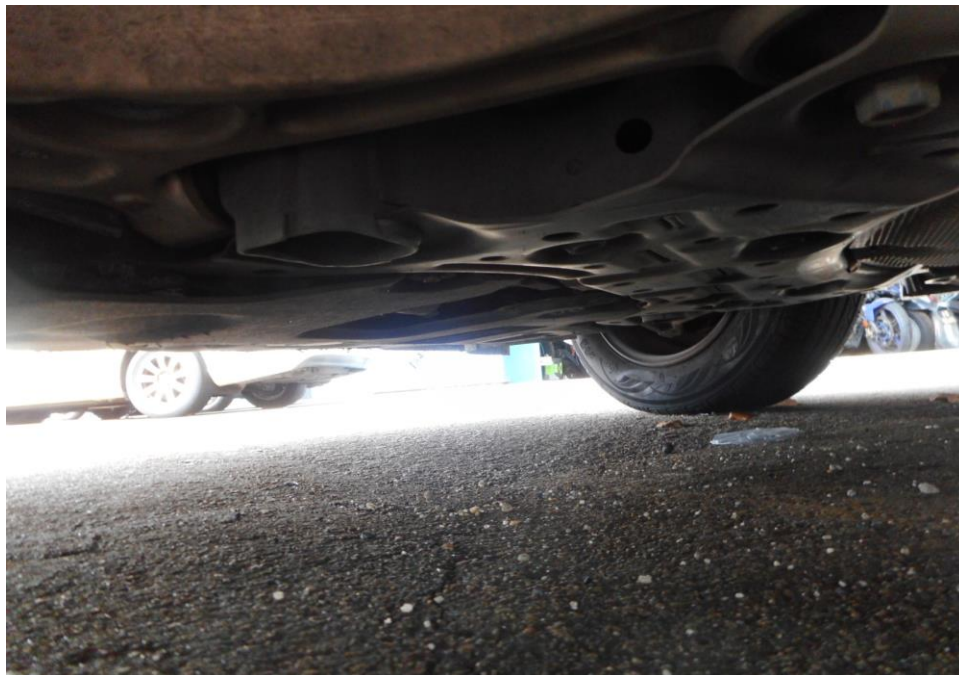
Photo 16 shows the undercarriage of the Motor Taxi, at the area where the engine housing and transmission housing are located. I did not find any sign(s) or indication(s) of fluid leak and/or fluid stain(s) on the underside of the Motor Taxi.
