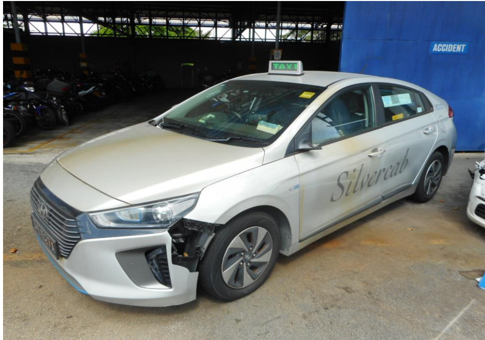
Photo 6 shows a general view of the Motor Taxi's left body at the time of my inspection. The left portion of the Motor Taxi was observed to have been unaffected by the accident.
