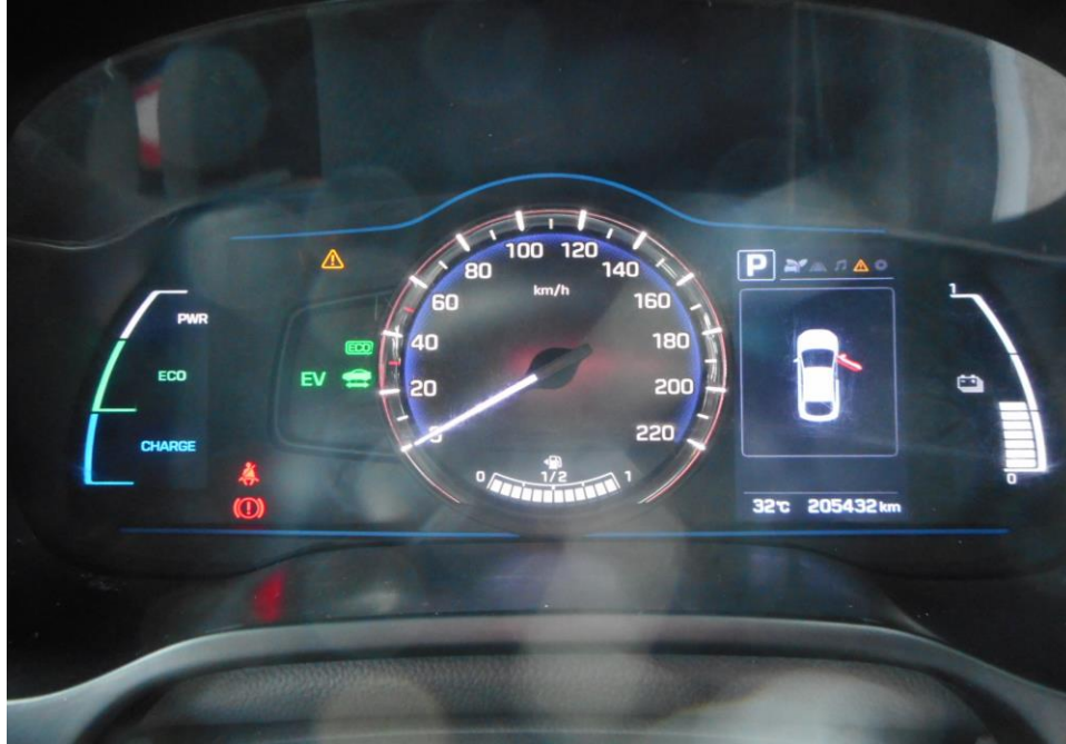
Photo 25 shows no warning lights illuminated on the instrument panel of the Motor Taxi after the engine was cranked. This would suggest that there was no abnormality to the electronic operating system of the Motor Taxi, like the ABS, EPS, SRS, and TC etc.
