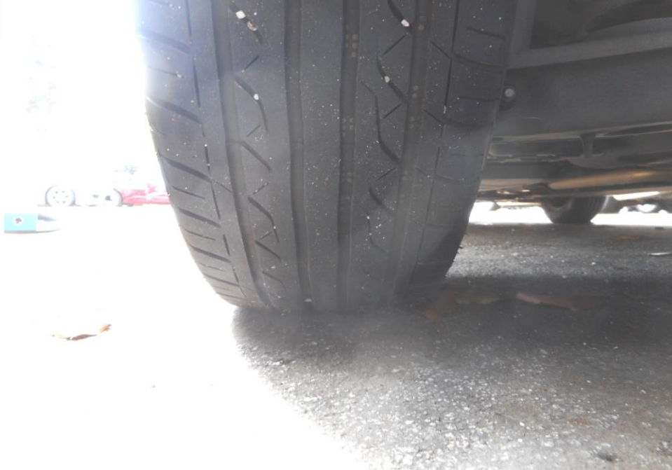
Photo 10 shows the condition of the rear left tyre of the Motor Taxi, which was observed to be in serviceable condition with remaining tread depth of approximately 3.9mm. The tyre, which was wrapped around steel wheel rim, was also observed to be sufficiently inflated for vehicular operation. The 4 tyres of the Motor Taxi were wrapped around standard steel wheel rims.
