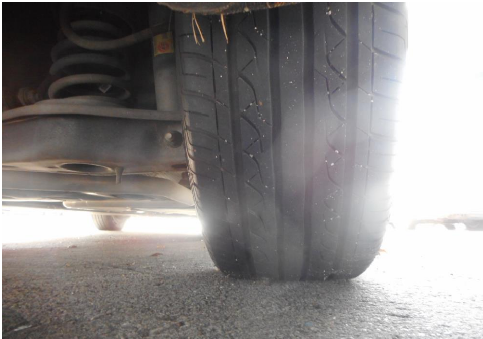
Photo 9 shows the condition of the rear right tyre of the Motor Taxi, which was observed to be in serviceable condition with remaining tread depth of approximately 4.4mm. The tyre was also observed to be sufficiently inflated for vehicular operation with no tear, cut or burst mark(s).
