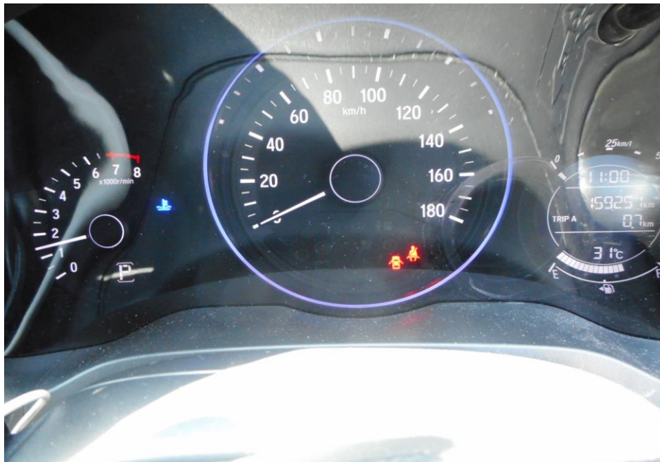
Photo 24 shows no warning lights illuminated on the instrument panel of the Motor Car after the engine was cranked. This would suggest that there was no abnormality to the electronic operating system of the Motor Car, like the ABS, EPS, SRS, and TC etc.
