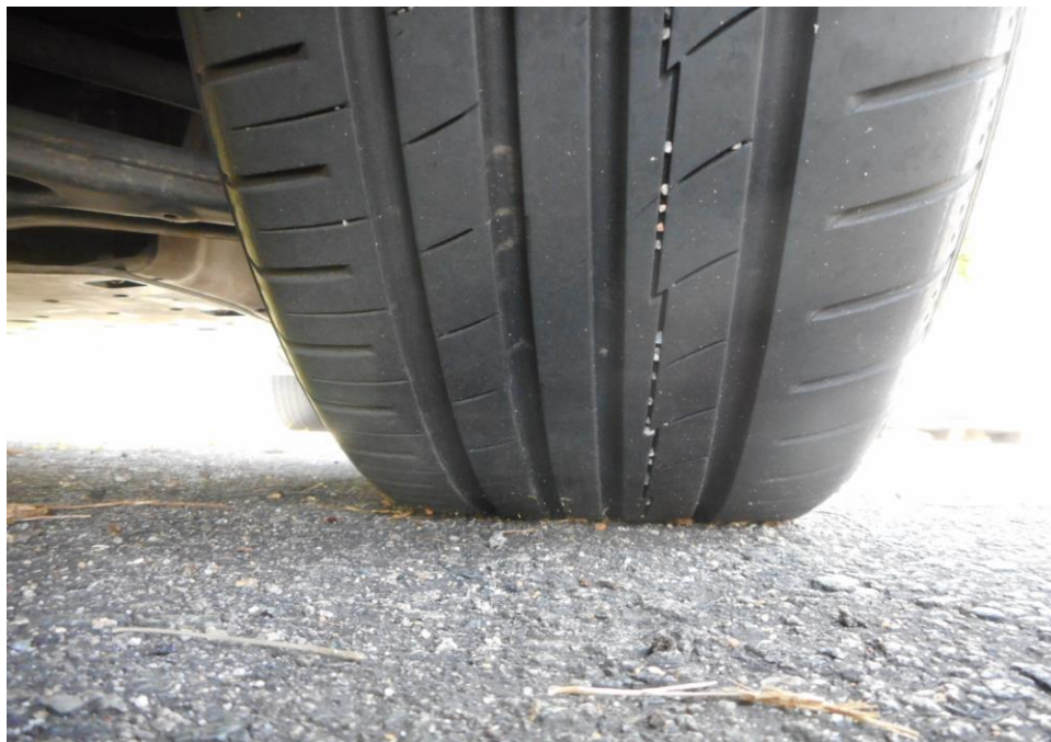
Photo 7 shows the condition of the front right tyre of the Motor Car, which was observed to be in serviceable condition with remaining tread depth of approximately 5mm. The tyre was sufficiently inflated for vehicular operation with no tear, cut or burst mark(s) on the outer and the inner sidewalls as well as across the tread. The 4 tyres of the Motor Car were wrapped around standard steel wheel rims without any damage.
