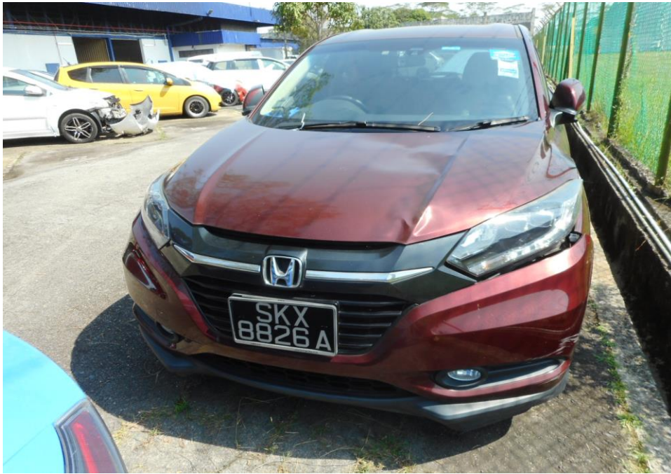
Photo 2 shows a general view of the Motor Car's front body at the time of my inspection. The front portion of the Motor Car was observed to have sustained damage. Its front bonnet and front bumper was the body parts that were damaged as a result of the accident.
