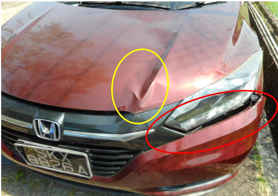
Photo 3 shows the close up view of the Motor Car's front body at the time of my inspection. The Motor Car was observed to have sustained damage at its front bumper (red circle) and front bonnet (yellow circle), as a result of the accident.
