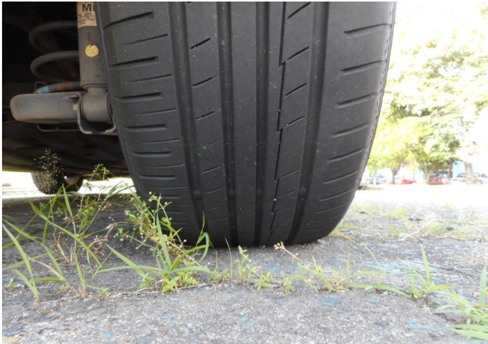
Photo 8 shows the condition of the rear right tyre of the Motor Car, which was observed to be in serviceable condition with remaining tread depth of approximately 4.5mm. The tyre was also observed to be sufficiently inflated for vehicular operation with no tear, cut or burst mark(s).
