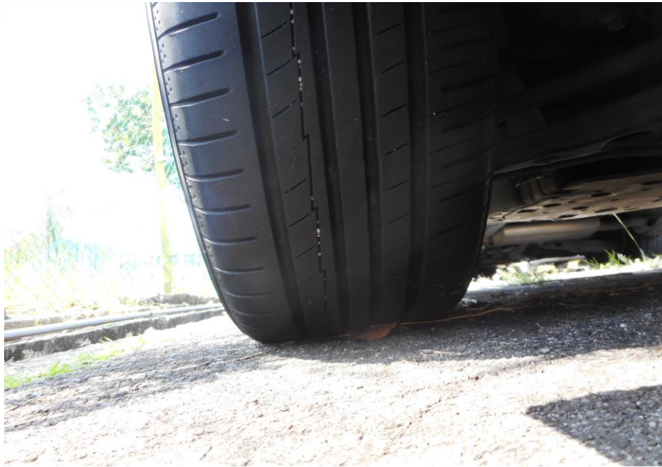
Photo 10 shows the condition of the front left tyre of the Motor Car, which was observed to be in serviceable condition with remaining tread depth of approximately 4.8mm. There was also no tear, cut or burst mark(s) on the outer and the inner sidewalls as well as across the tread of the Motor Car's 4 tyres.
