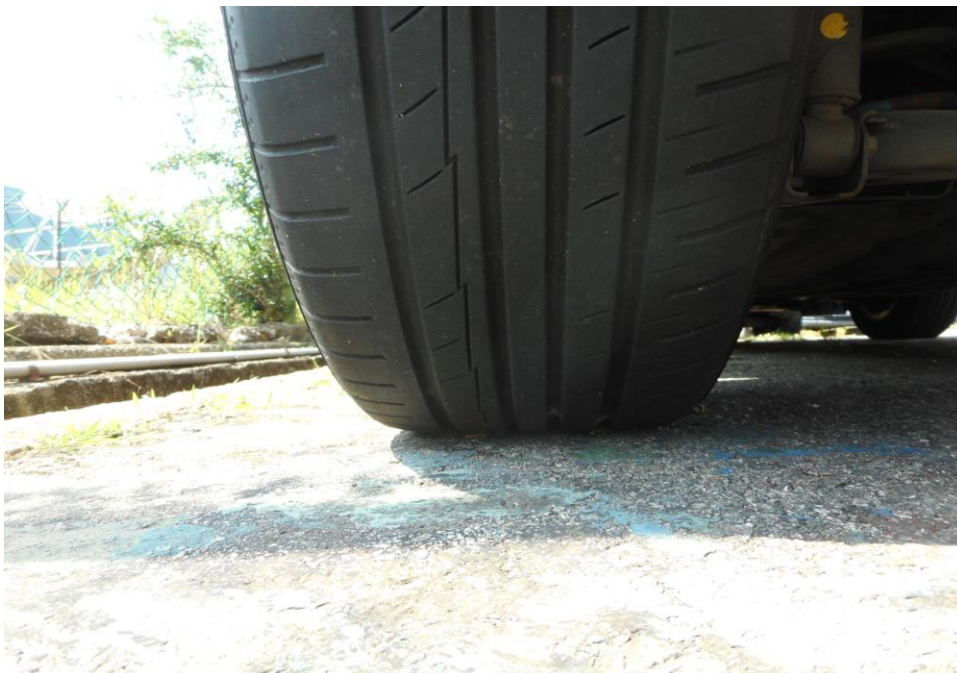
Photo 9 shows the condition of the rear left tyre of the Motor Car, which was observed to be in serviceable condition with remaining tread depth of approximately 4mm. The tyre, which was wrapped around steel wheel rim, was also observed to be sufficiently inflated for vehicular operation. The 4 tyres of the Motor Car were wrapped around standard steel wheel rims.
