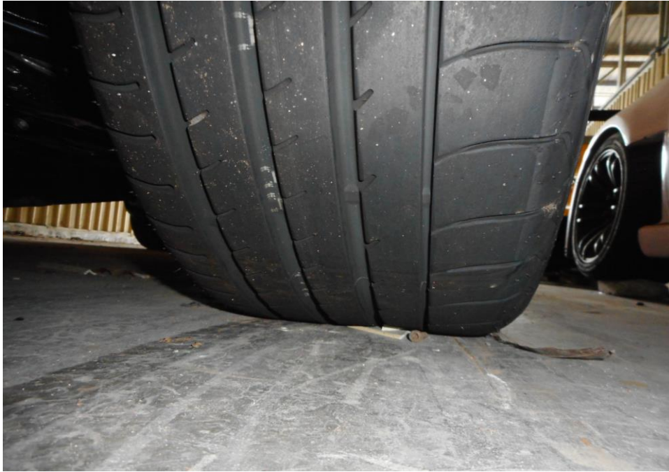
Photo 9 shows the condition of the front right tyre of the Motor Car, which was observed to be in serviceable condition with remaining tread depth of approximately 6.7mm. The tyre, which was wrapped around alloy wheel rim, was also observed to be sufficiently inflated for vehicular operation.
