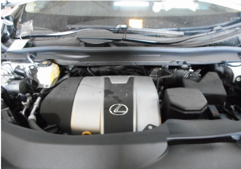
Photo 14 shows a general view of the Motor Car's engine compartment, which was accessed by lifting the front cabin of the Motor Car. The various parts and components inside the engine compartment are shown. There was no sign(s) or indication(s) of fresh fluid leakage and/or fluid stain within the engine compartment
