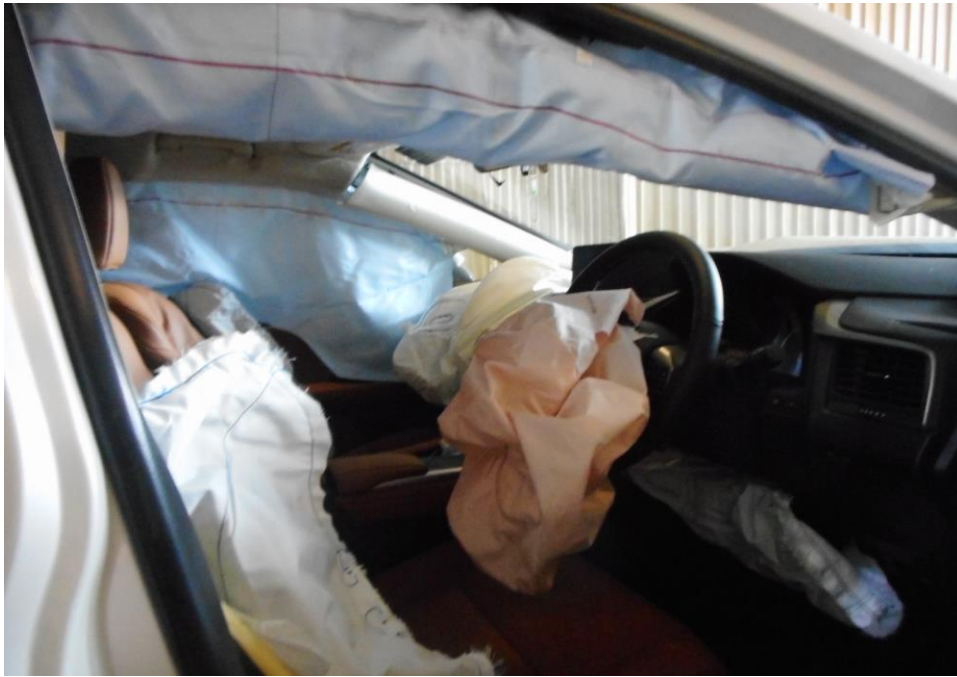
Photo 13 shows the deployment of the Supplemental Restraint System (SRS) airbag in the Motor Car as a result of the accident.
