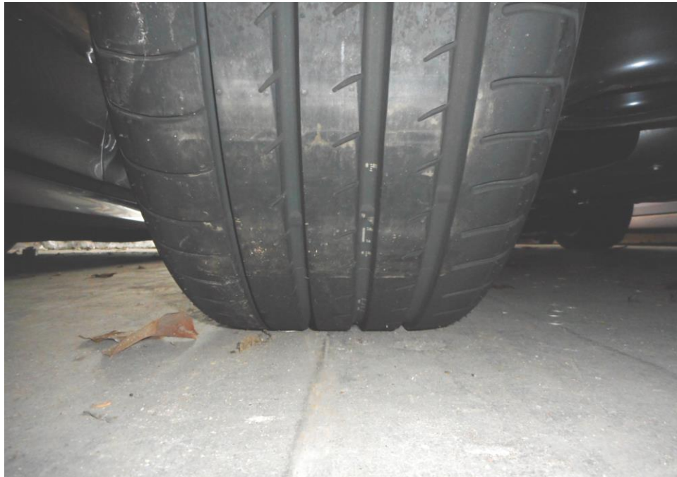
Photo 11 shows the condition of the rear left tyre of the Motor Car, which was observed to be in serviceable condition with remaining tread depth of approximately 7.5mm. The tyre was also observed to be sufficiently inflated for vehicular operation with no tear, cut or burst mark(s).
