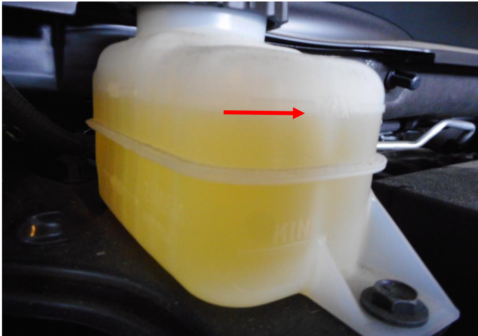
Photo 15 shows the brake fluid reservoir of the Motor Car at the time of my inspection. The brake fluid was observed to be of sufficient level (arrowed) and without any visible contamination.
