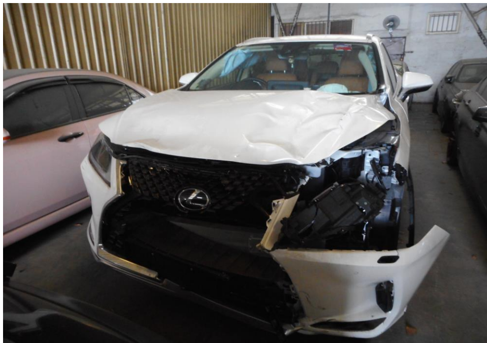
Photo 2 shows a general view of the Motor Car's front body at the time of my inspection. The Motor car was observed to have sustained damage at its front portion. Its front bonnet, front bumper, front left headlamp was amongst the body parts and various components in the engine compartments were also damaged as a result of the accident. The Supplemental Restraint System (SRS) was activated as a result of the accident.
