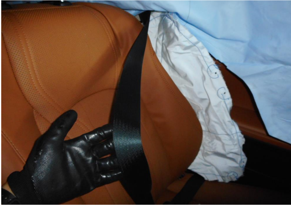
Photo 26 shows that the seat belt on the left seat was worn at the material time of accident as the safety pre-tensioners was activated at the moment of impact and caused the seat belt to be locked into the last position.
