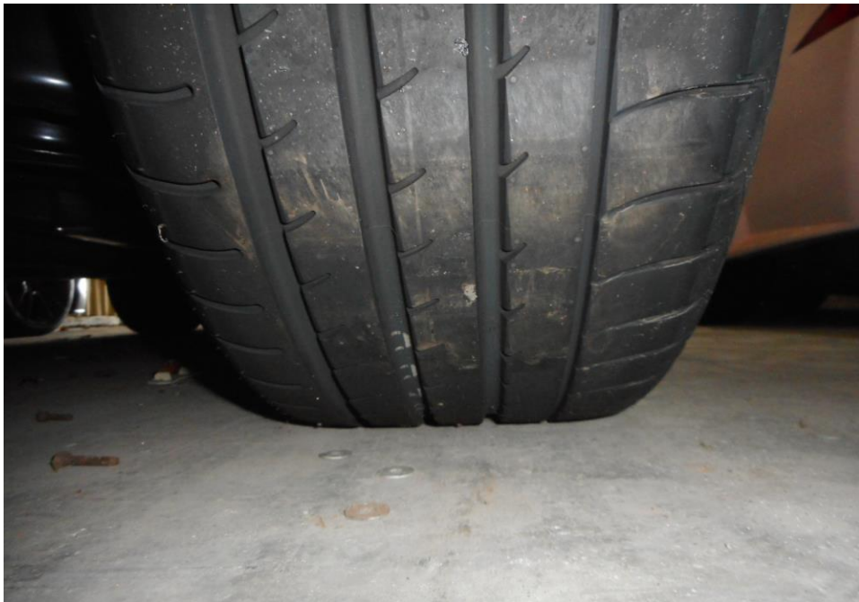
Photo 10 shows the condition of the rear right tyre of the Motor Car, which was observed to be in serviceable condition with remaining tread depth of approximately 7.1mm. The tyre was also observed to be sufficiently inflated for vehicular operation with no tear, cut or burst mark(s).
