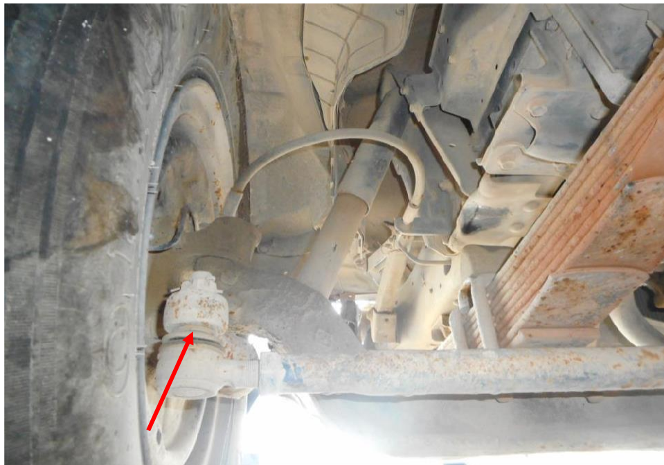
Photo 28 shows the various undercarriage components at the front left wheel of the Motor Lorry, in particular the steering tie rod end (arrowed). The various undercarriage components of the Motor Lorry were all found to be intact without any visible damage. There was also no sign of fluid stain(s) observed on the various undercarriage components.
