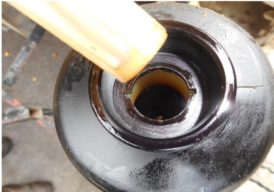
Photo 18 shows the power steering fluid reservoir of the Motor Lorry at the time of my inspection. The power steering fluid was observed to be of sufficient level (arrowed) and without any visible contamination.
