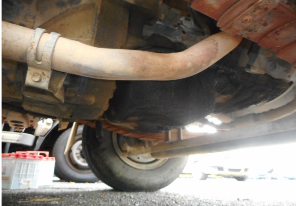
Photo 19 shows the undercarriage of the Motor Lorry, at the area where the engine housing and transmission housing are located. I did not find any sign(s) or indication(s) of fluid leak and/or fluid stain(s) on the underside of the Motor Lorry.
