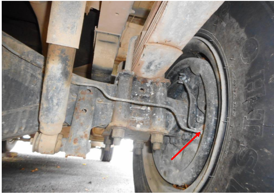
Photo 20 shows the brake pipe (arrowed) at the rear right wheel of the Motor Lorry. I did not observe any leakage of brake fluid at the time of my inspection of the Motor Lorry.
