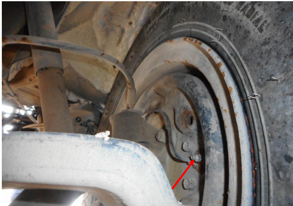
Photo 22 shows the brake hose/pipe (arrowed) at the front right wheel of the Motor Lorry. No leakage of brake fluid was observed. Visual examination of the various components of the braking system like the brake drum (circled), brake pedal etc had revealed all to be intact and without visible damage at the time of accident. There was also no sign of fluid stain(s) observed on the various undercarriage components.
