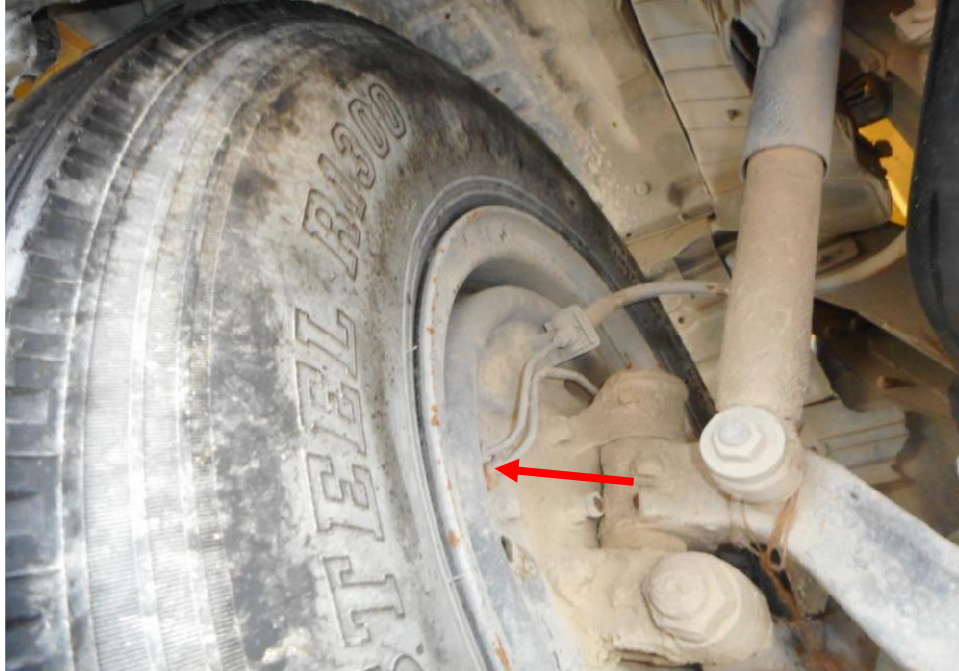
Photo 23 shows the brake hose/pipe (arrowed) at the front left wheel of the Motor Lorry. No leakage of brake fluid was observed. Visual examination of the various components of the braking system like the brake drum (circled), brake pedal etc had revealed all to be intact and without visible damage at the time of accident. There was also no sign of fluid stain(s) observed on the various undercarriage components.
