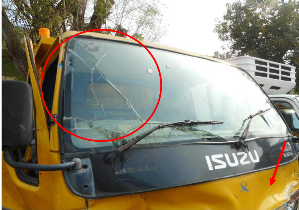
Photo 4 shows a close up view of the Motor Lorry's frontal portion at the time of my inspection. It appeared to have sustained damage at its frontal portion. Its front windscreen (circled) and front body panel (arrowed) was damage at the time of my inspection as a result of the accident.
