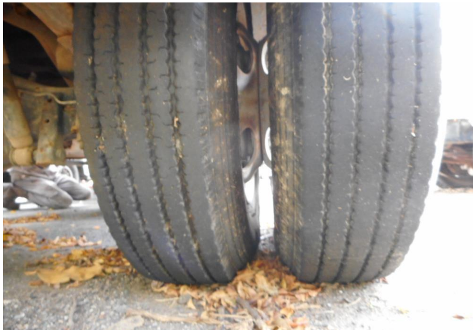
Photo 11 shows the condition of the rear right tyre of the Motor Lorry, which was observed to be in serviceable condition with remaining tread depth of approximately 3.4mm. The tyre, which was wrapped around standard steel wheel rim, it was observed to be sufficiently inflated for vehicular operation.
