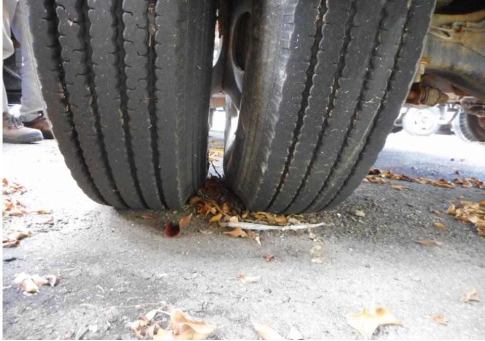
Photo 12 shows the condition of the rear left tyres of the Motor Lorry, which was observed to be in serviceable condition with remaining tread depth of approximately 6.8mm. The tyres, which were wrapped around standard steel wheel rim, were also observed to be sufficiently inflated for vehicular operation. There was also no damage found on all 6 steel wheel rims of the Motor Lorry.
