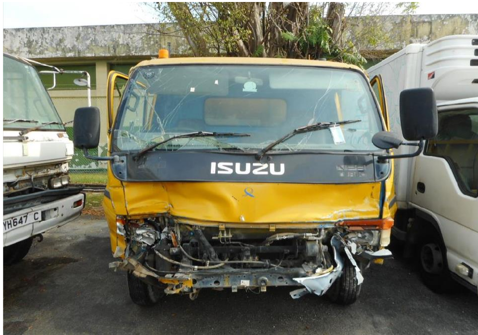
Photo 3 shows a general view of the Motor Lorry's frontal portion at the time of my inspection. It appeared to have sustained damage at its frontal portion. Its front windscreen, front body panel, front bumper, both front headlamps, left and right doors were damage at the time of my inspection.
