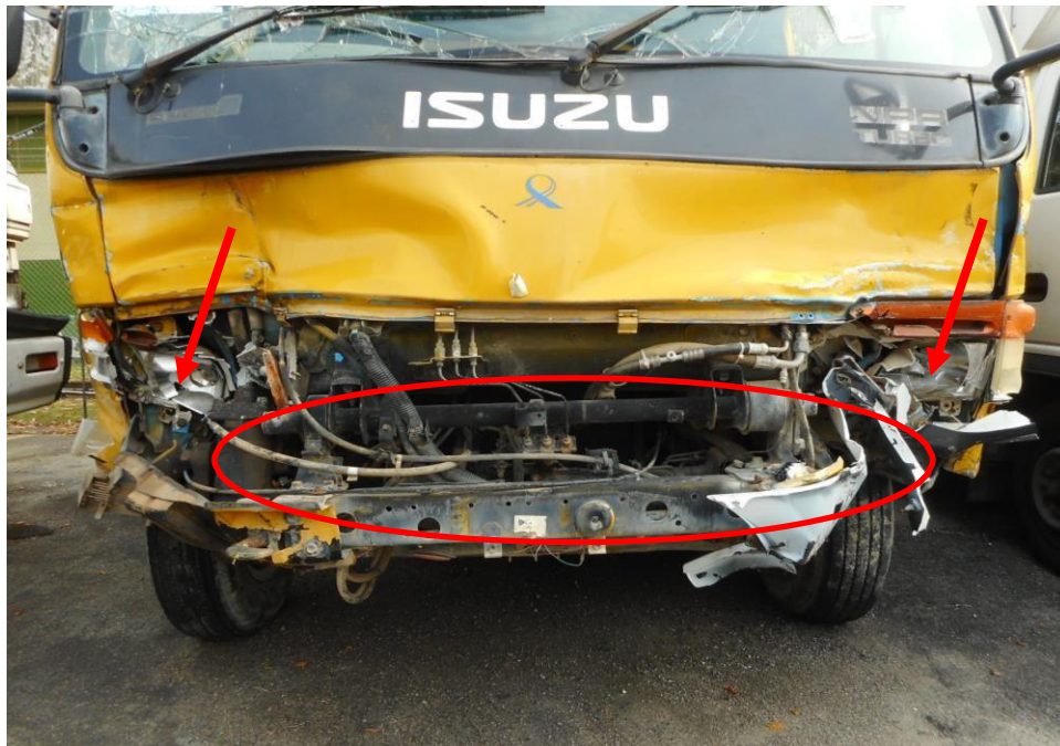
Photo 5 shows a close up view of the Motor Lorry's frontal portion at the time of my inspection. It appeared to have sustained damage at its frontal portion. Its front bumper (circled) and both front headlamps (arrowed) was damage at the time of my inspection as a result of the accident.
