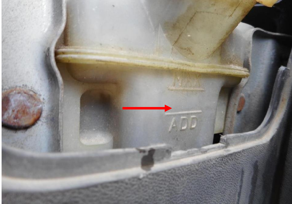
Photo 15 shows the brake fluid reservoir of the Motor Lorry at the time of my inspection. The brake fluid was observed to be of sufficient level (arrowed) and without any visible contamination.
