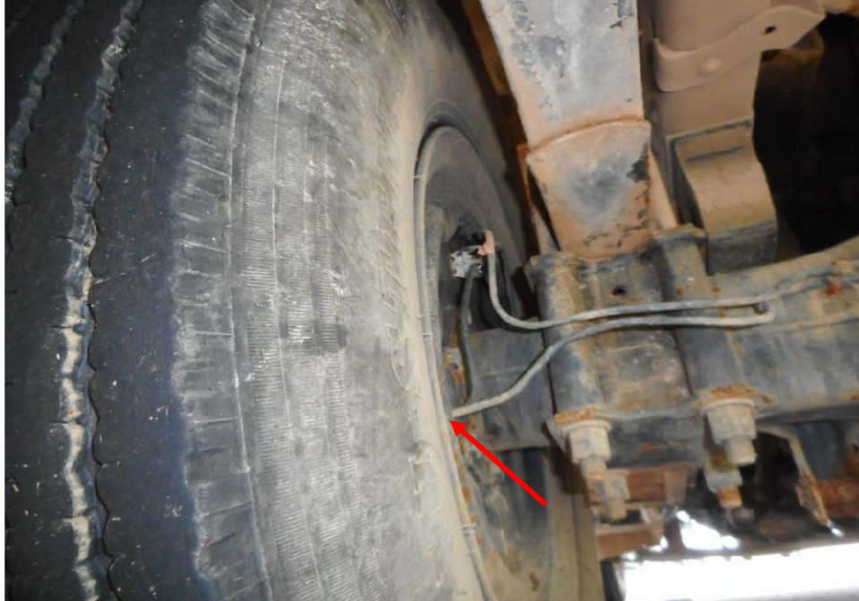
Photo 21 shows the brake pipe (arrowed) at the rear left wheel of the Motor Lorry. I did not observe any leakage of brake fluid at the time of my inspection of the Motor Lorry.
