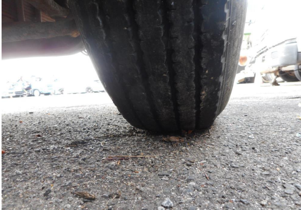
Photo 10 shows the condition of the front right tyre of the Motor Lorry, which was observed to be in serviceable condition with remaining tread depth of approximately 4.4mm. The tyre, which was wrapped around standard steel wheel rim, was also observed to be sufficiently inflated for vehicular operation. There was no tear, cut or burst mark(s) on the outer and the inner sidewalls as well as across the tread of the 6 tyres that were fitted on the Motor Lorry.
