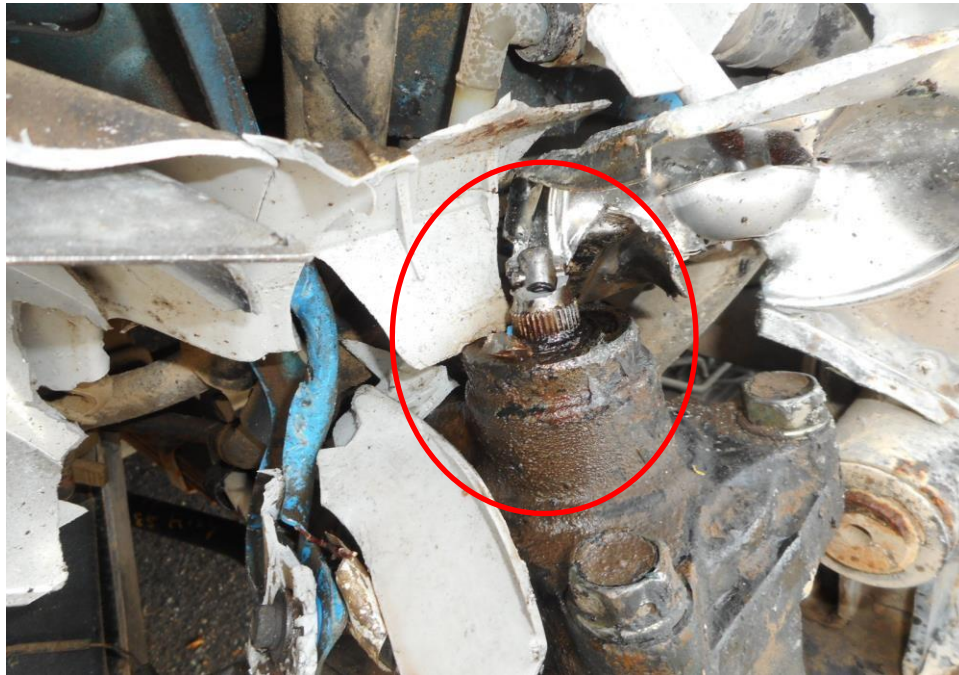
Photo 26 shows a close up view of the steering box (circled) of the Motor Lorry at the time of my inspection. The steering box was observed to be damaged as result of the accident.
