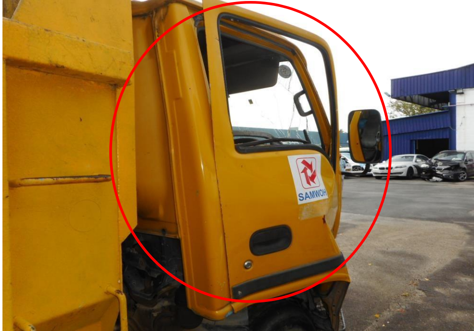
Photo 6 shows a close up view of the Motor Lorry's frontal portion at the time of my inspection. It appeared to have sustained damage at its frontal portion. Its right door (circled) was damage at the time of my inspection as a result of the accident.
