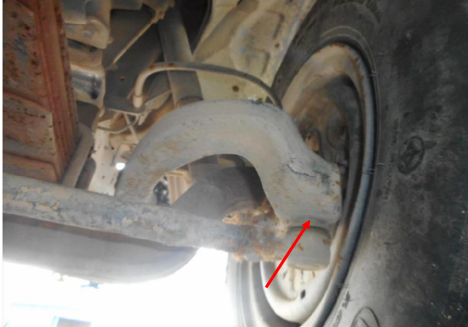
Photo 27 shows the various undercarriage components at the front right wheel of the Motor Lorry, in particular the steering tie rod end (arrowed). The various steering components were all found to be intact, suggesting that the steering system of the Motor Lorry was likely to be in serviceable condition at the material time of accident. There was also no sign of fluid stain(s) observed on the various undercarriage components.
