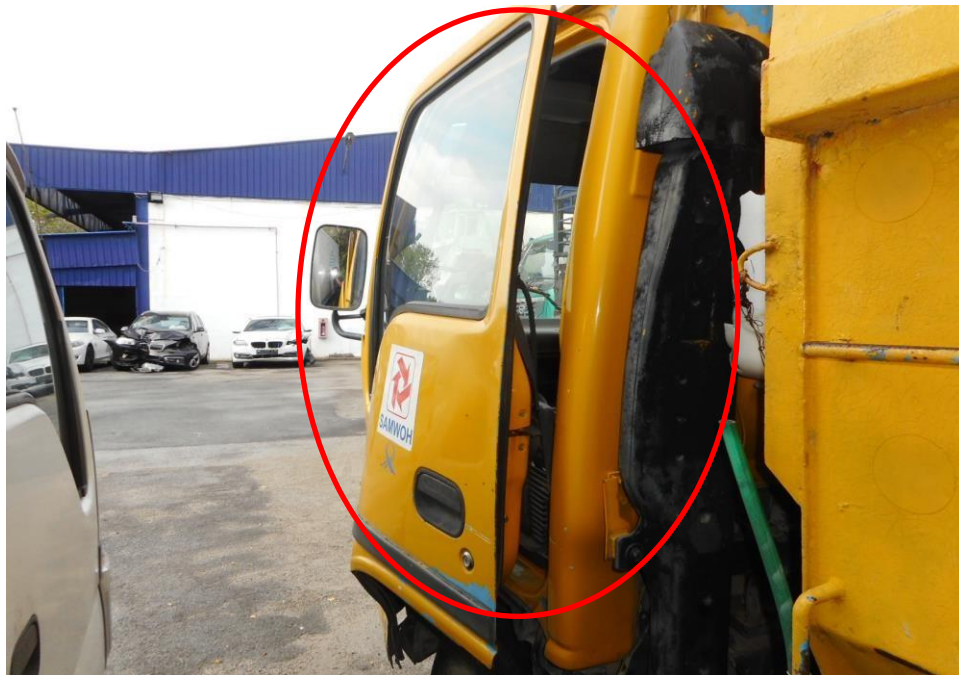
Photo 7 shows a close up view of the Motor Lorry's frontal portion at the time of my inspection. It appeared to have sustained damage at its frontal portion. Its left door (circled) was damage at the time of my inspection as a result of the accident.
