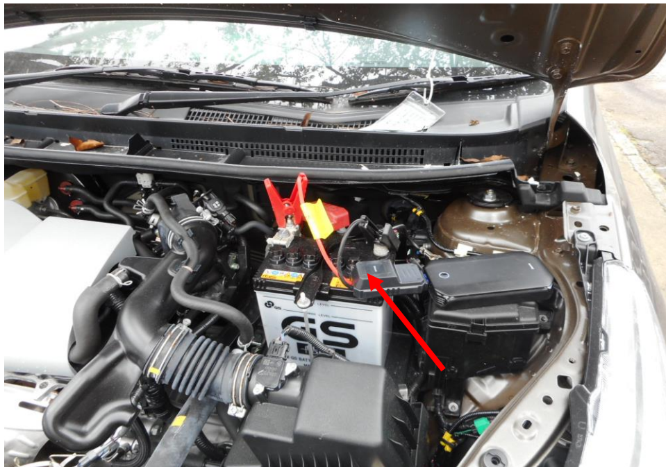
Photo 19 shows the jumpstarting process of the Motor Car's engine. The engine of the Motor Car was unable to be jumpstarted up despite multiple attempts in starting it.
