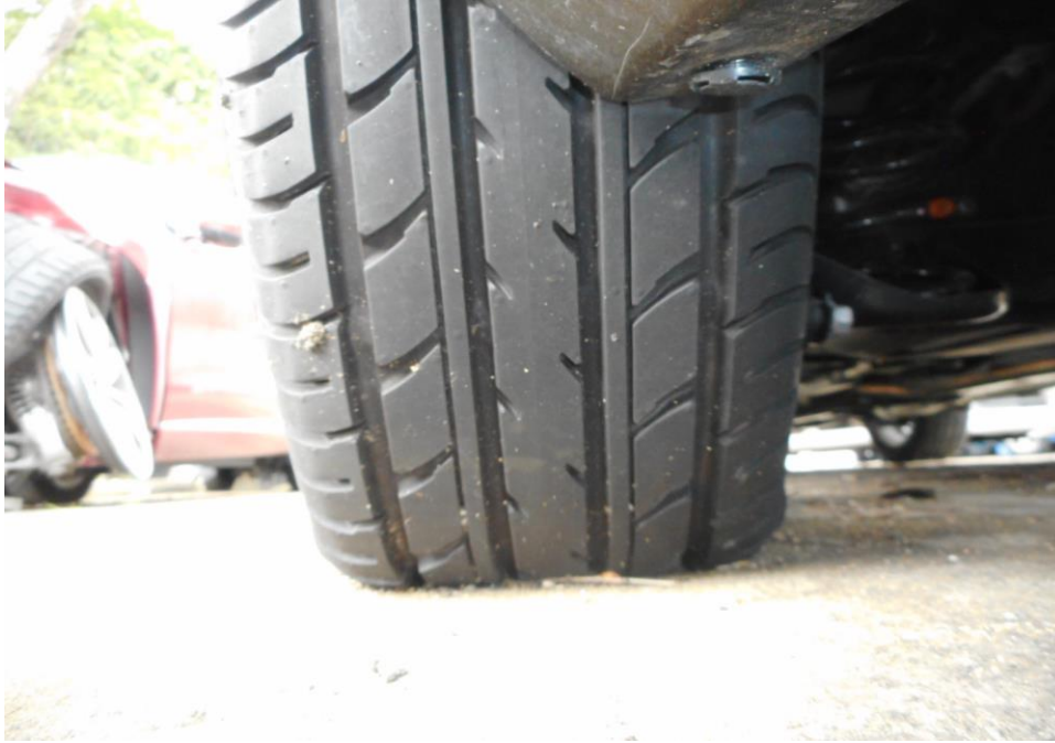
Photo 12 shows the condition of the rear left tyre of the Motor Car, which was observed to be deflated with remaining tread depth of approximately 6.2mm. There was also no tear, cut or burst mark(s) on the outer and the inner sidewalls as well as across the tread of the Motor Car's 4 tyres.
