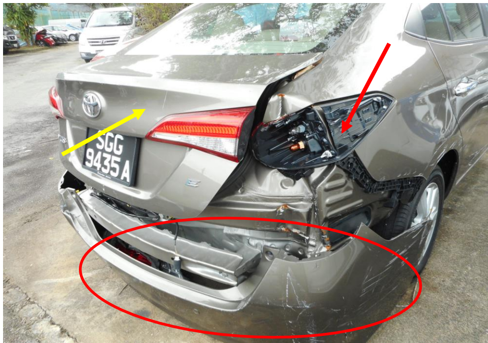
Photo 9 shows the close up view of the Motor Car's left body at the time of my inspection. The rear boot (yellow arrow) rear right brake lamp (red arrow) and the rear bumper (circled) of the Motor Car was observed to have been damaged by the accident.
