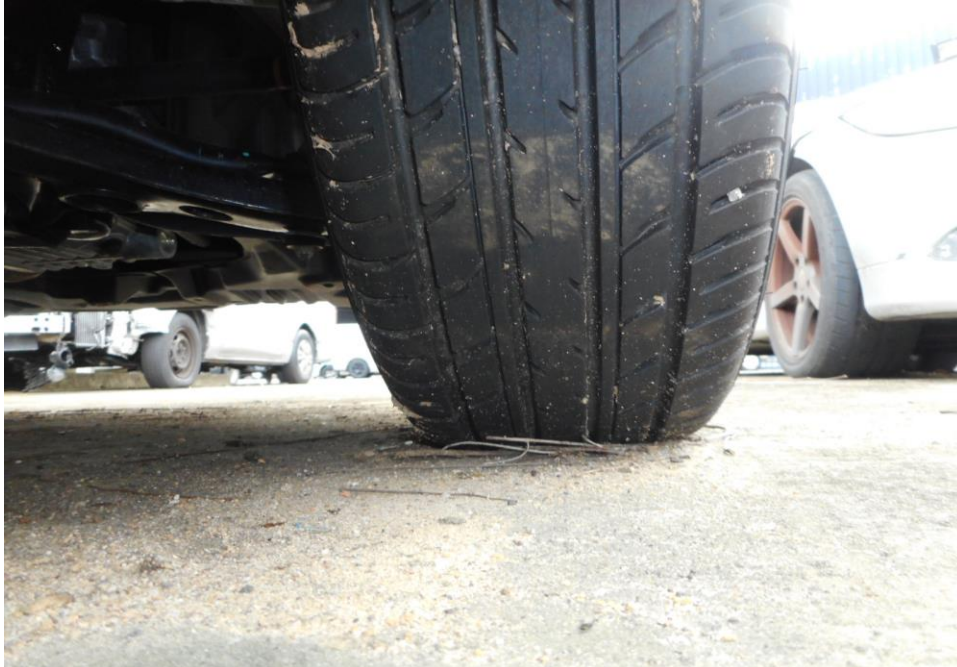
Photo 10 shows the condition of the front right tyre of the Motor Car, which was observed to be in serviceable condition with remaining tread depth of approximately 6.5mm. The tyre was sufficiently inflated for vehicular operation with no tear, cut or burst mark(s) on the outer and the inner sidewalls as well as across the tread. The 4 tyres of the Motor Car were wrapped around standard steel wheel rims without any damage.
