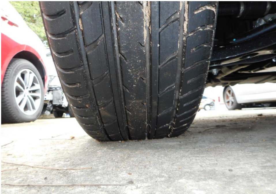
Photo 13 shows the condition of the front left tyre of the Motor Car, which was observed to be in serviceable condition with remaining tread depth of approximately 6.3mm. There was also no tear, cut or burst mark(s) on the outer and the inner sidewalls as well as across the tread of the Motor Car's 4 tyres.
