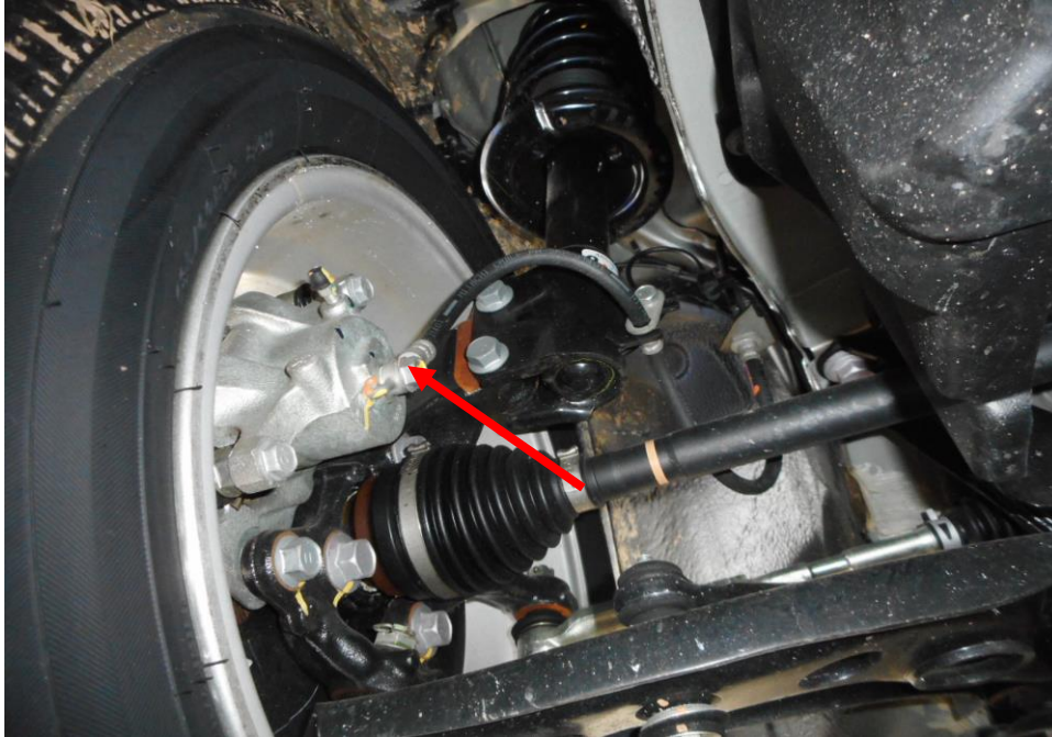
Photo 22 shows the brake hose/pipe (arrowed) at the front right wheel of the Motor Car. I did not observe any leakage of brake fluid at the time of my inspection of the Motor Car. Static tests of the Motor Car's braking system had indicated that there was no internal leakage of pressure/vacuum. The undercarriage components of the Motor Car were also all found to be intact and without any visible damage.
