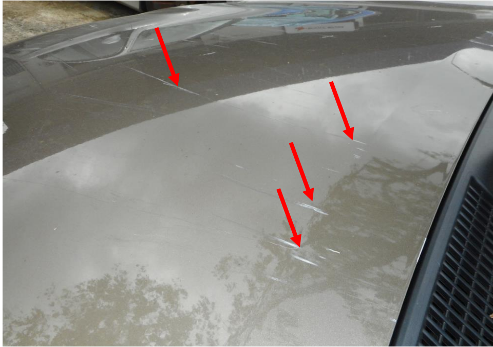
Photo 2 shows the close-up view of the Motor Car's front body at the time of my inspection. The Motor Car was observed to have sustained damage at its front bonnet (arrowed) as a result of the accident.
