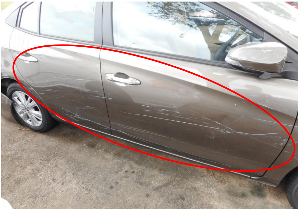
Photo 5 shows the close up view of the Motor Car's right body at the time of my inspection. The right body panels (circled) of the Motor Car was observed to have been damaged by the accident.
