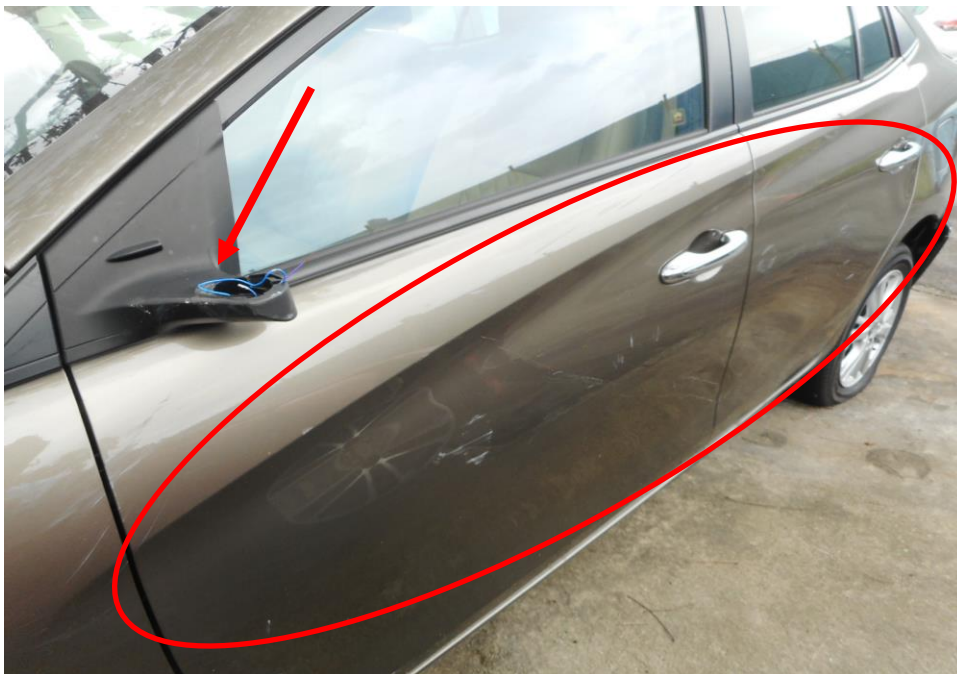
Photo 7 shows the close up view of the Motor Car's left body at the time of my inspection. The left body panels (circled) and left rear view mirror (arrowed) of the Motor Car was observed to have been damaged by the accident.
