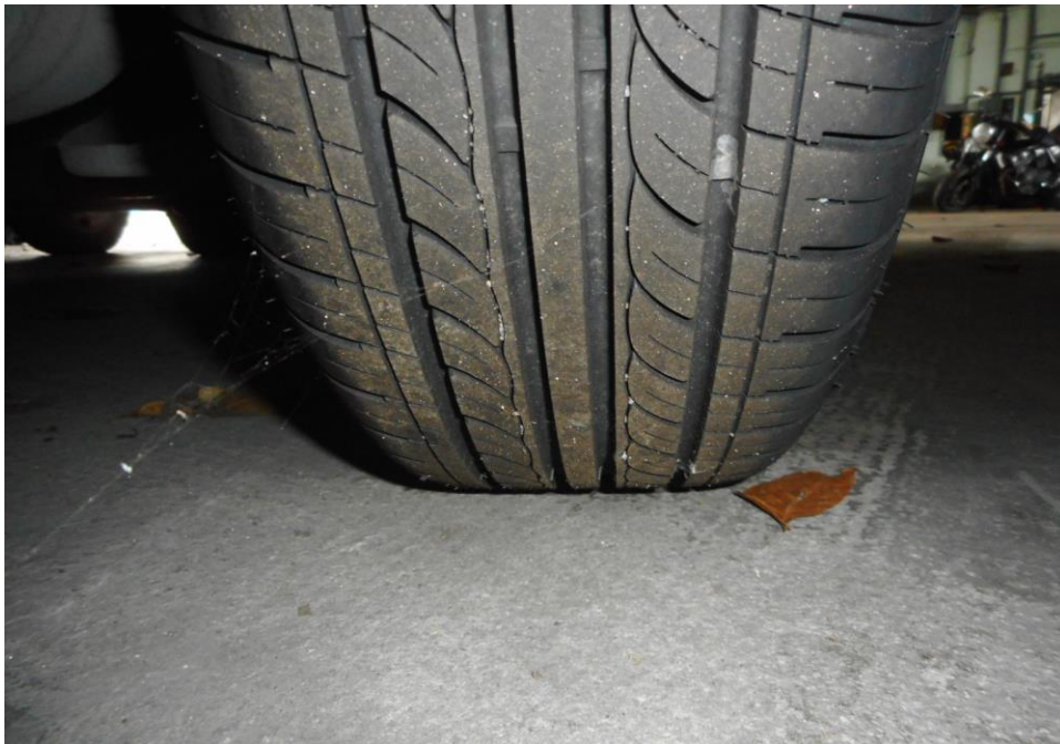
Photo 9 shows the condition of the rear right tyre of the Motor Car, which was observed to be in serviceable condition with remaining tread depth of approximately 6.1mm. The tyre was also observed to be sufficiently inflated for vehicular operation with no tear, cut or burst mark(s).
