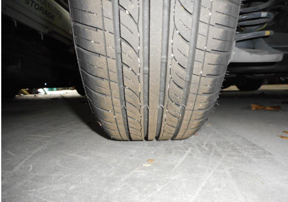
Photo 10 shows the condition of the rear left tyre of the Motor Car, which was observed to be in serviceable condition with remaining tread depth of approximately 6.3mm. The tyre, which was wrapped around steel wheel rim, was also observed to be sufficiently inflated for vehicular operation. The 4 tyres of the Motor Car were wrapped around standard steel wheel rims.
