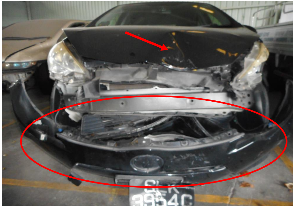
Photo 4 shows the close up view of the Motor Car's front body at the time of my inspection. Its front bumper (circled) and front bonnet (arrowed) are the body parts that were damaged as a result of the accident.
