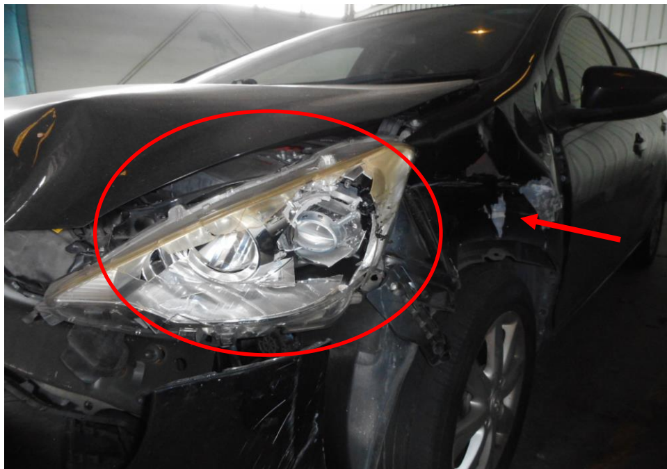
Photo 5 shows the close up view of the Motor Car's front body at the time of my inspection. Its front left headlamp (circled) and front left fender (arrowed) are the body parts that were damaged as a result of the accident.
