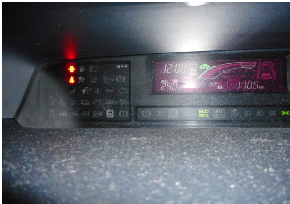
Photo 22 shows no warning lights illuminated on the instrument panel of the Motor Car after the engine was cranked. This would suggest that there was no abnormality to the various electronic operating systems of the Motor Car, like the ABS, TCS, SRS and EPS.
