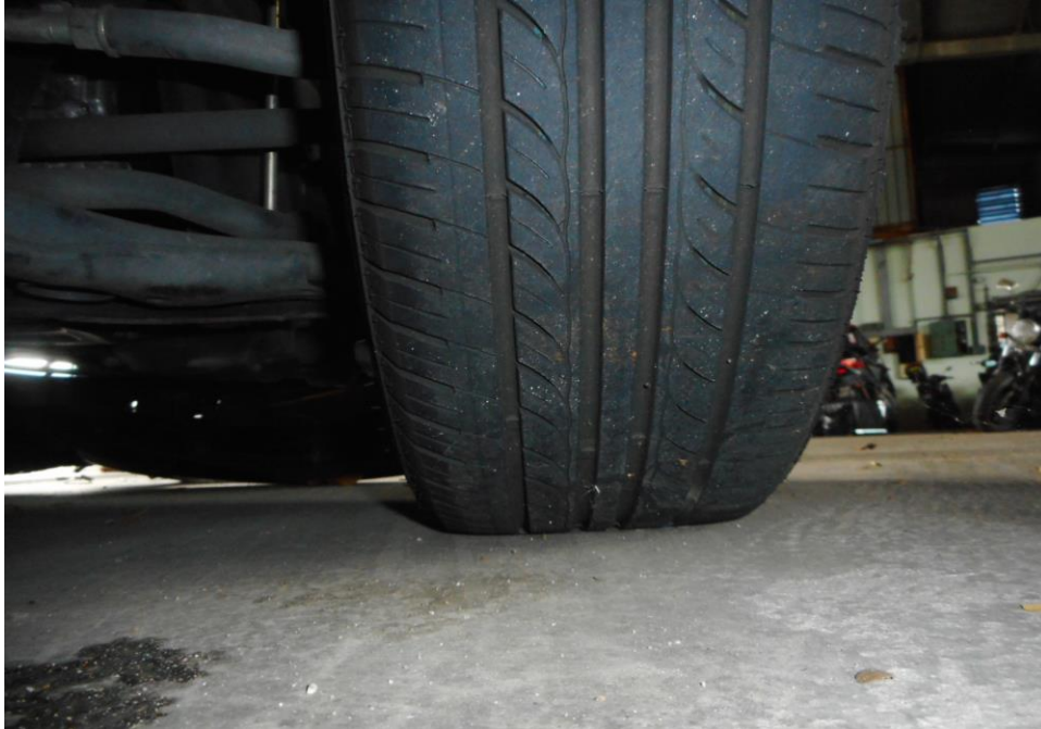
Photo 8 shows the condition of the front right tyre of the Motor Car, which was observed to be in serviceable condition with remaining tread depth of approximately 4.1mm. The tyre was sufficiently inflated for vehicular operation with no tear, cut or burst mark(s) on the outer and the inner sidewalls as well as across the tread. The 4 tyres of the Motor Car were wrapped around standard steel wheel rims without any damage.
