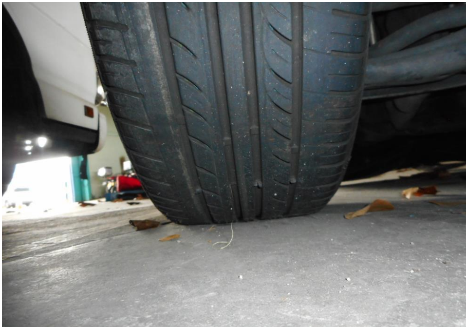
Photo 11 shows the condition of the front left tyre of the Motor Car, which was observed to be in serviceable condition with remaining tread depth of approximately 3.8mm. The tyre, which was wrapped around steel wheel rim, was also observed to be sufficiently inflated for vehicular operation. The 4 tyres of the Motor Car were wrapped around standard steel wheel rims.
