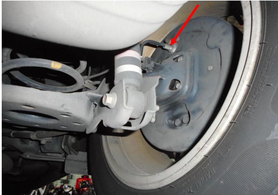
Photo 14 shows the brake hose/pipe (arrowed) at the rear right wheel of the Motor Car. No leakage of brake fluid was observed. Visual examination of the various components of the braking system like the brake caplier, brake booster, brake pedal etc. had revealed all to be intact and without visible damage.
