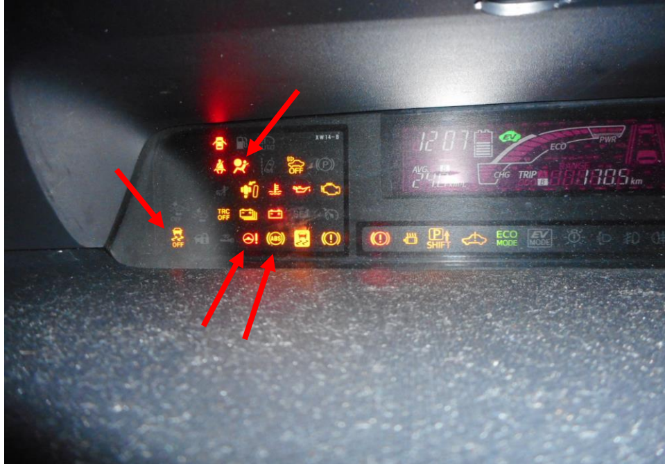
Photo 21 shows the warning light for Anti-Lock Brake System (ABS), Traction Control System (TCS), Power Steering System (EPS) and Supplemental Restraint System (SRS) (arrowed) appearing on the instrument panel of the Motor Car during the self-test of its various electronic operating systems when its engine was cranked.
