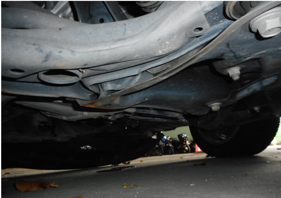
Photo 13 shows the undercarriage of the Motor Car, at the area where the engine housing and transmission housing are located. I did not find any sign(s) or indication(s) of fluid leak and/or fluid stain(s) on the underside of the Motor Car.
