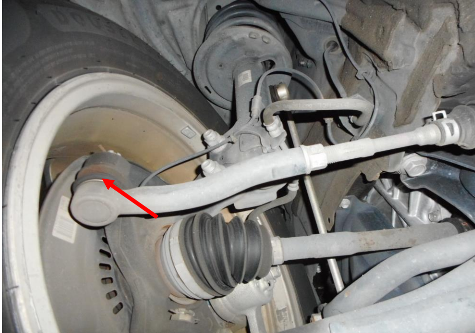
Photo 20 shows the various undercarriage components at the front left wheel of the Motor Car, which had included the steering tie rod (red arrow). The various undercarriage components of the Motor Car were all found to be intact without any visible damage.
