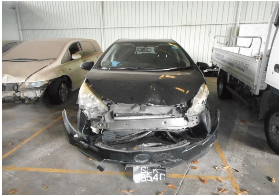
Photo 3 shows a general view of the Motor Car's front body at the time of my inspection. Its front bonnet, front bumper, front left fender and front left headlamp are the body parts that were damaged as a result of the accident.
