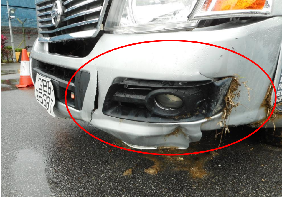
Photo 4 shows the close up view of the Motor Van's front body at the time of my inspection. Its front bumper (circled) are the body parts that were damaged as a result of the accident.
