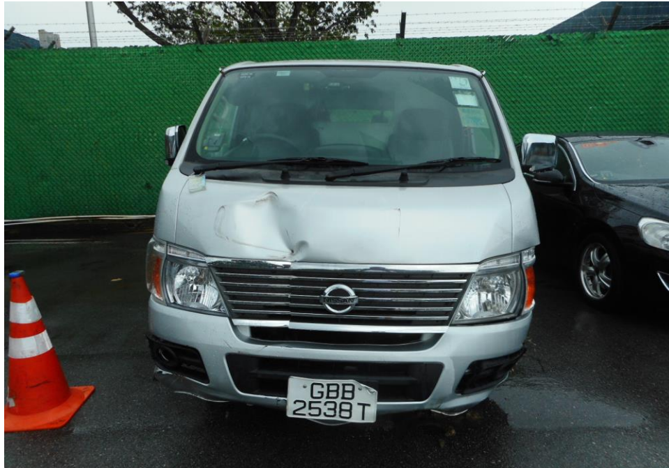
Photo 2 shows a general view of the Motor Van's front body at the time of my inspection. Its front body panel, front grille and front bumper are the body parts that were damaged as a result of the accident.
