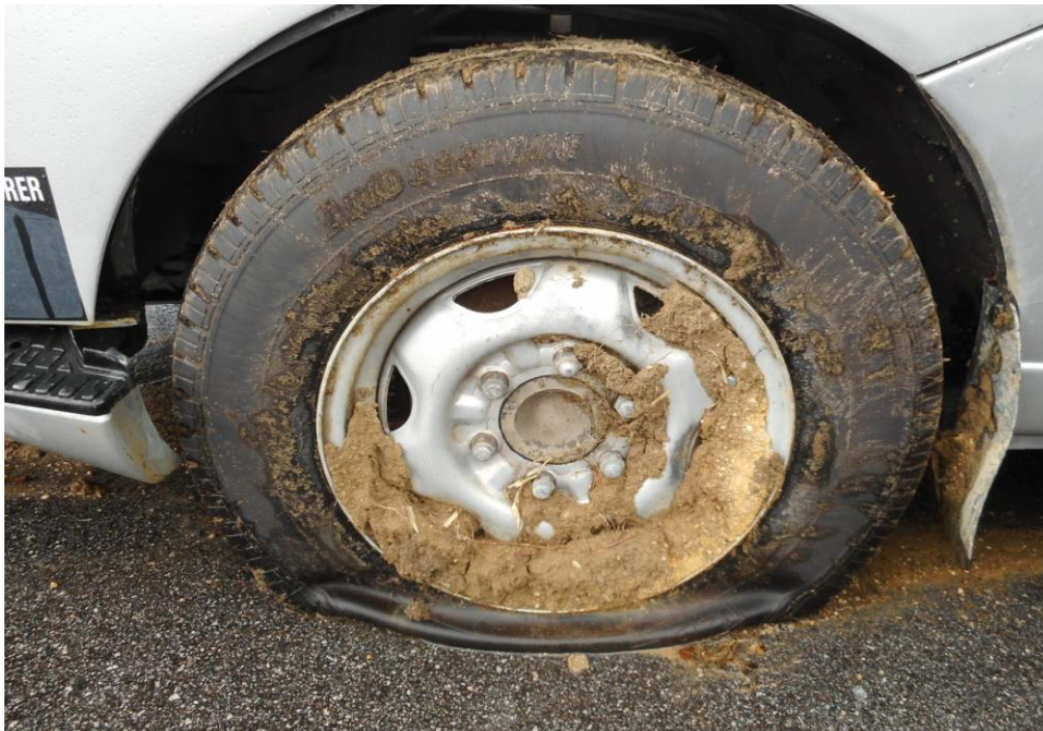
Photo 11 shows the condition of the front left tyre of the Motor Van, which was observed to be deflated likely due to the result of the accident. The with remaining tread depth of approximately 8.1mm
