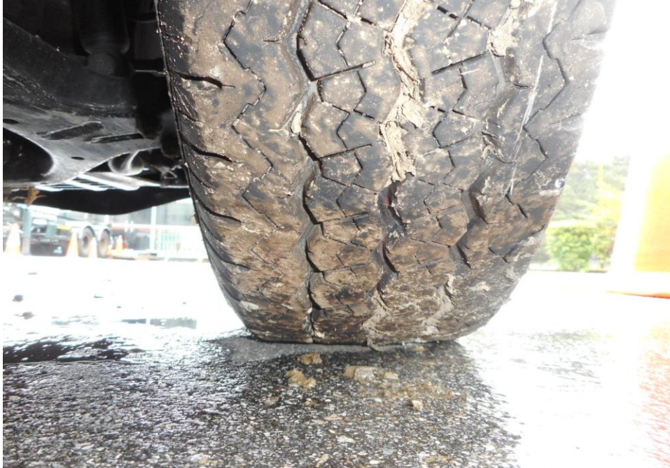
Photo 8 shows the condition of the front right tyre of the Motor Van, which was observed to be in serviceable condition with remaining tread depth of approximately 8.2mm. The tyre was sufficiently inflated for vehicular operation with no tear, cut or burst mark(s) on the outer and the inner sidewalls as well as across the tread. The 4 tyres of the Motor Van were wrapped around standard steel wheel rims without any damage.
