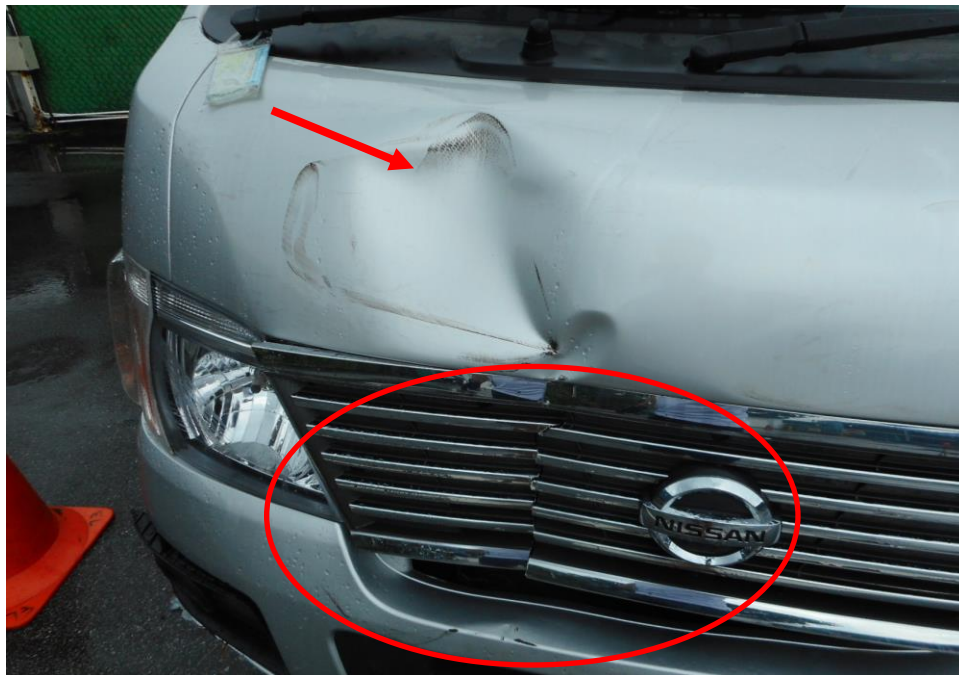
Photo 3 shows the close up view of the Motor Van's front body at the time of my inspection. Its front body panel (arrowed) and front grille (circled) are the body parts that were damaged as a result of the accident.
