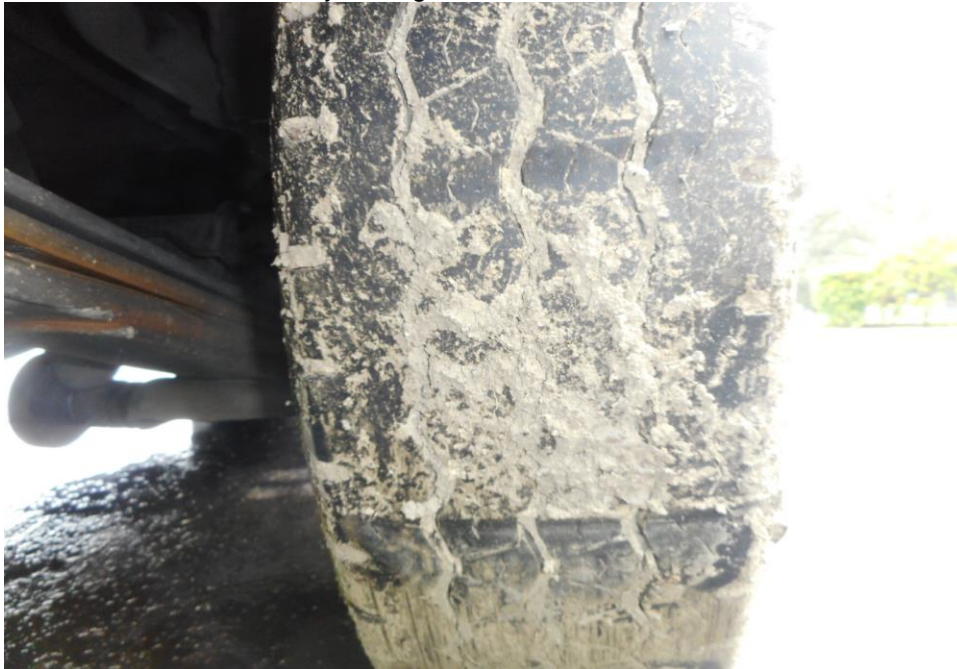
Photo 9 shows the condition of the rear right tyre of the Motor Van, which was observed to be in serviceable condition with remaining tread depth of approximately 4.8mm. The tyre was also observed to be sufficiently inflated for vehicular operation with no tear, cut or burst mark(s).
