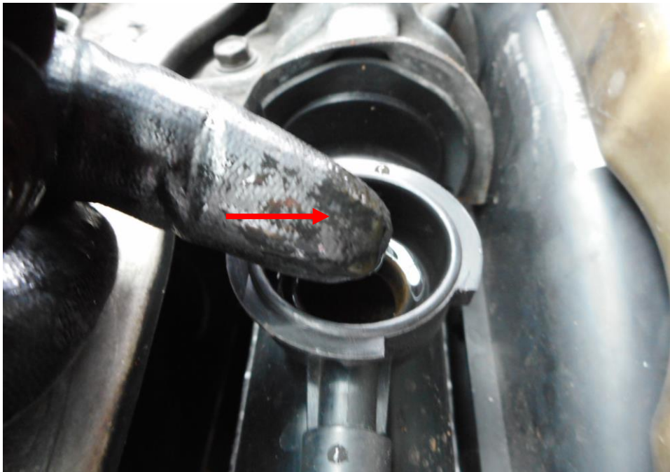
Photo 14 shows checks being carried out to the engine coolant of the Motor Van at the time of my inspection. The engine coolant was observed to be of sufficient level (arrowed) and without any visible contamination.
