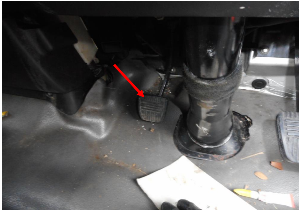
Photo 24 shows the clutch pedal of the Motor Van, after depressing (red arrow). The actual workings of the clutch pedal is that it will return to pre-depressing position when it is not depressed, however for this case the clutch pedal remained in depressed position even when there was no pressing motion on it. These suggest a mechanical fault to the clutch system of the Motor Van.
