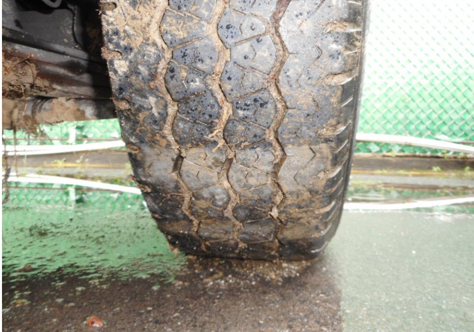
Photo 10 shows the condition of the rear left tyre of the Motor Van, which was observed to be in serviceable condition with remaining tread depth of approximately 5.2mm. The tyre, which was wrapped around steel wheel rim, was also observed to be sufficiently inflated for vehicular operation. The 4 tyres of the Motor Van were wrapped around standard steel wheel rims.
