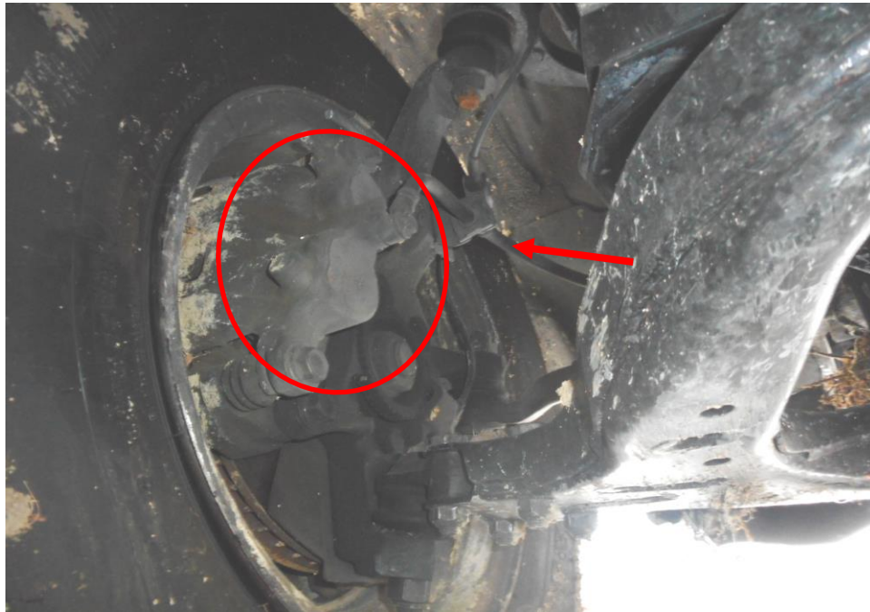
Photo 20 shows the brake hose/pipe (arrowed) at the front left wheel of the Motor Van. No leakage of brake fluid was observed. Visual examination of the various components of the braking system like the brake caliper (circled), brake booster, brake pedal etc had revealed all to be intact and without visible damage.
