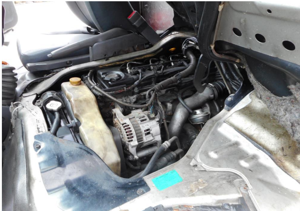
Photo 12 shows a general view of the Motor Van's engine compartment. The various parts and components inside the engine compartment were unaffected by the accident. There was also no sign(s) or indication(s) of fluid leakage and/or fluid stain within the engine compartment.
