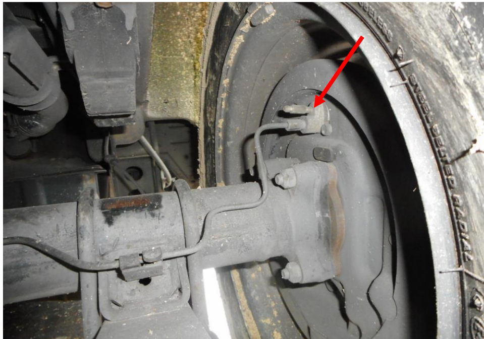
Photo 17 shows the brake hose/pipe (arrowed) at the rear right wheel of the Motor Van. No leakage of brake fluid was observed. Visual examination of the various components of the braking system like the brake caliper, brake booster, brake pedal etc. had revealed all to be intact and without visible damage.
