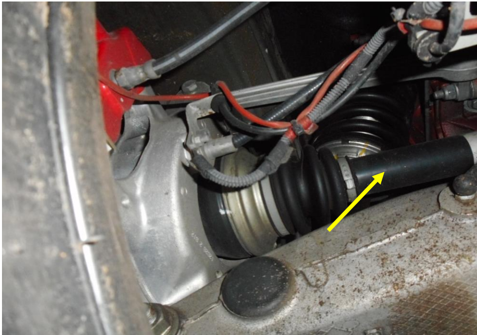
Photo 26 shows the various undercarriage components at the rear left wheel of the Motor Car, in particular the drive shaft (yellow arrow). The various undercarriage components of the Motor Car were all found to be intact without any visible damage. There was also no sign of fluid stain(s) observed on the various undercarriage components.
