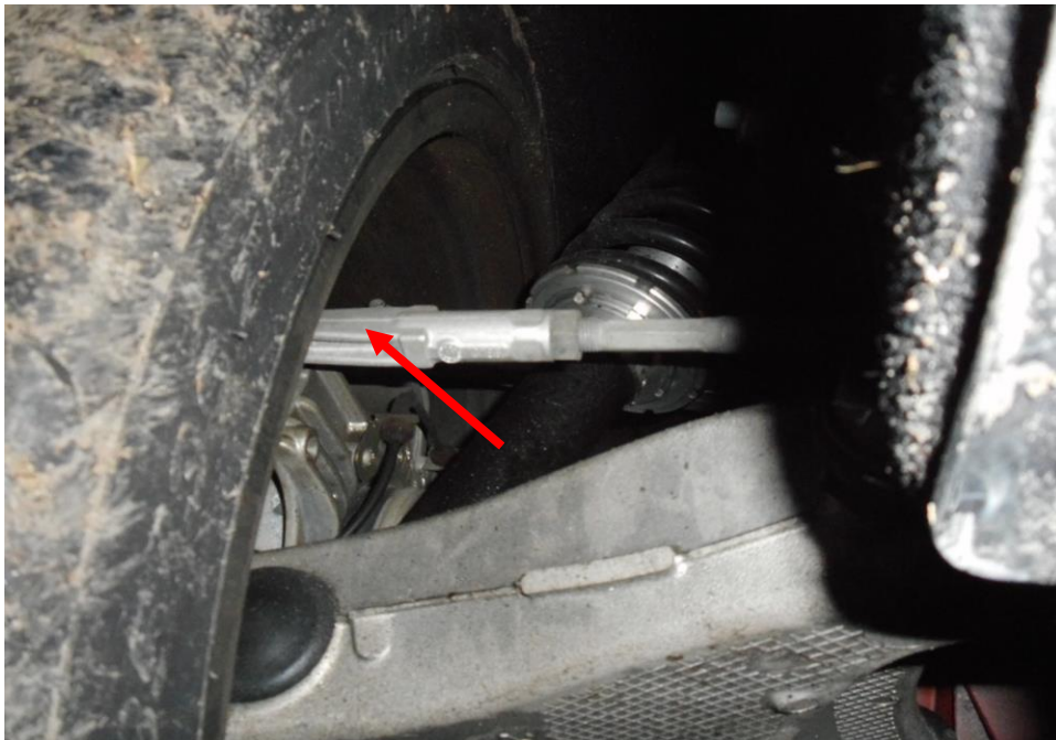
Photo 24 shows the various undercarriage components at the rear left wheel of the Motor Car, which had included the rear tie rod (arrowed) were found to be intact without any visible damage.
