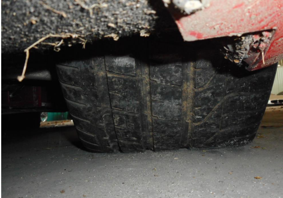
Photo 7 shows the condition of the rear right tyre of the Motor Car, which was observed to be in serviceable condition with remaining tread depth of approximately 5.7mm. The tyre was also observed to be sufficiently inflated for vehicular operation with no tear, cut or burst mark(s).
