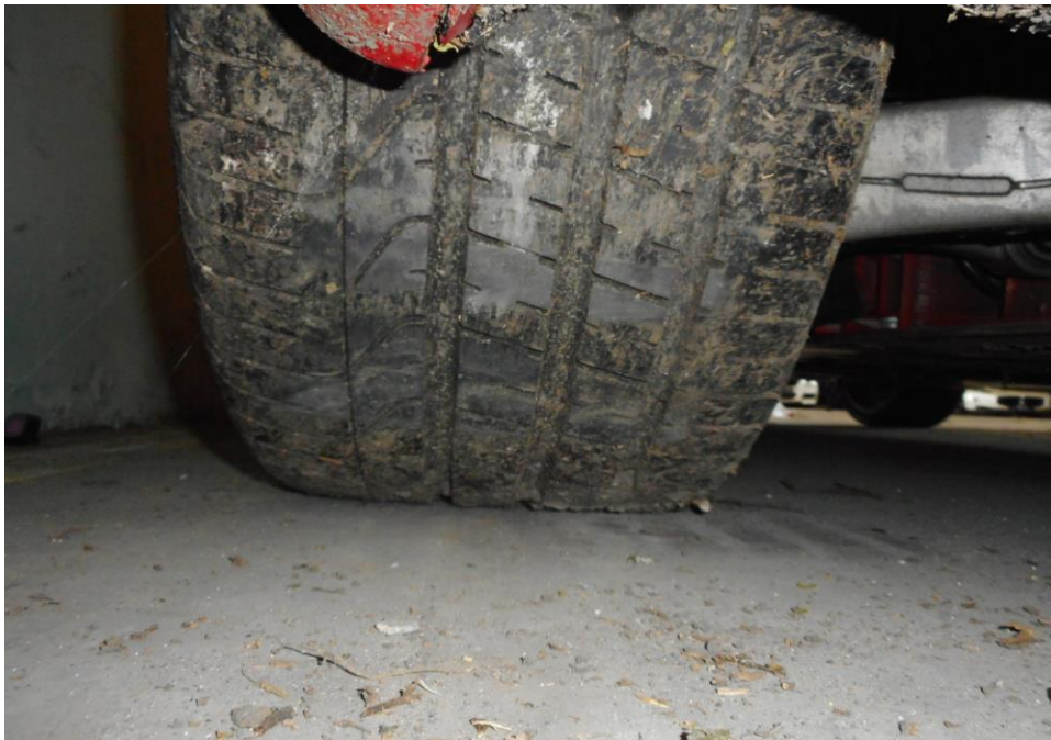
Photo 8 shows the condition of the rear left tyre of the Motor Car, which was observed to be in serviceable condition with remaining tread depth of approximately 5.5mm. The tyre was also observed to be sufficiently inflated for vehicular operation with no tear, cut or burst mark(s).
