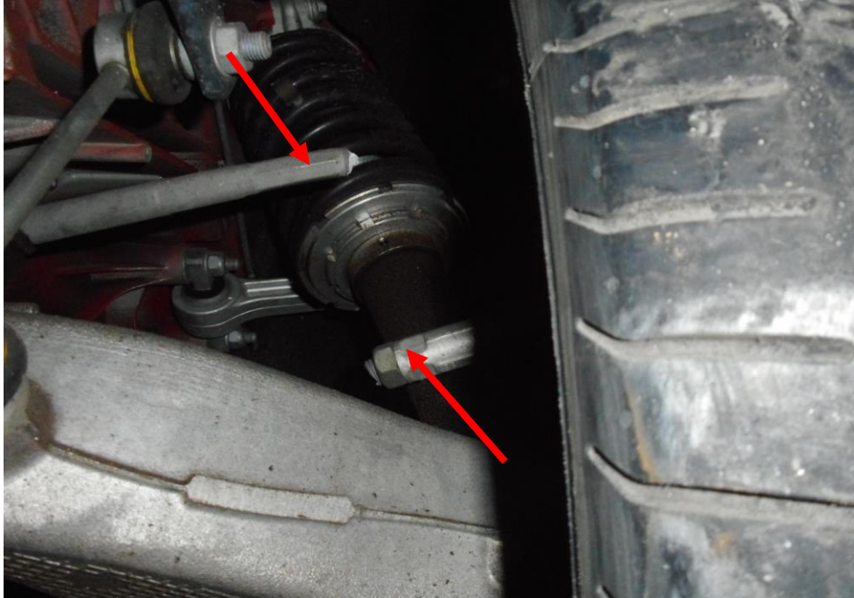
Photo 25 shows the various undercarriage components at the rear right wheel of the Motor Car, in particular the rear tie rod (arrowed) was observed to be damage as a result of the accident.
