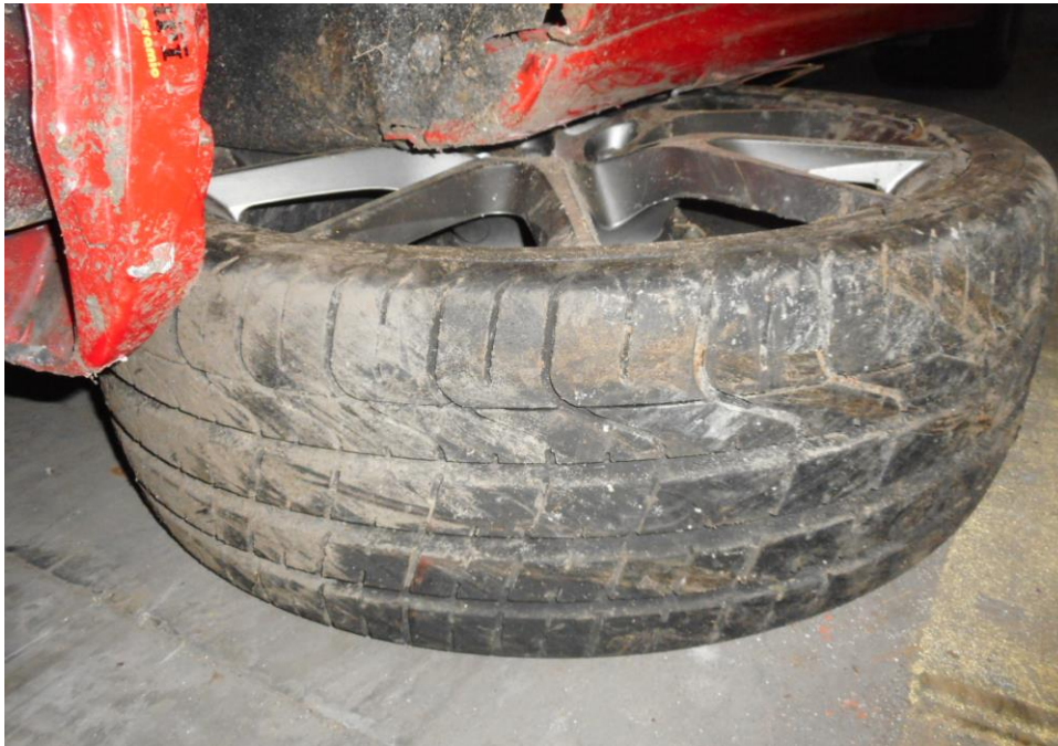
Photo 10 shows the condition of the front left tyre of the Motor Car, which was observed to be in serviceable condition with remaining tread depth of approximately 5.7mm. The tyre was also observed to be sufficiently inflated for vehicular operation with no tear, cut or burst mark(s).
