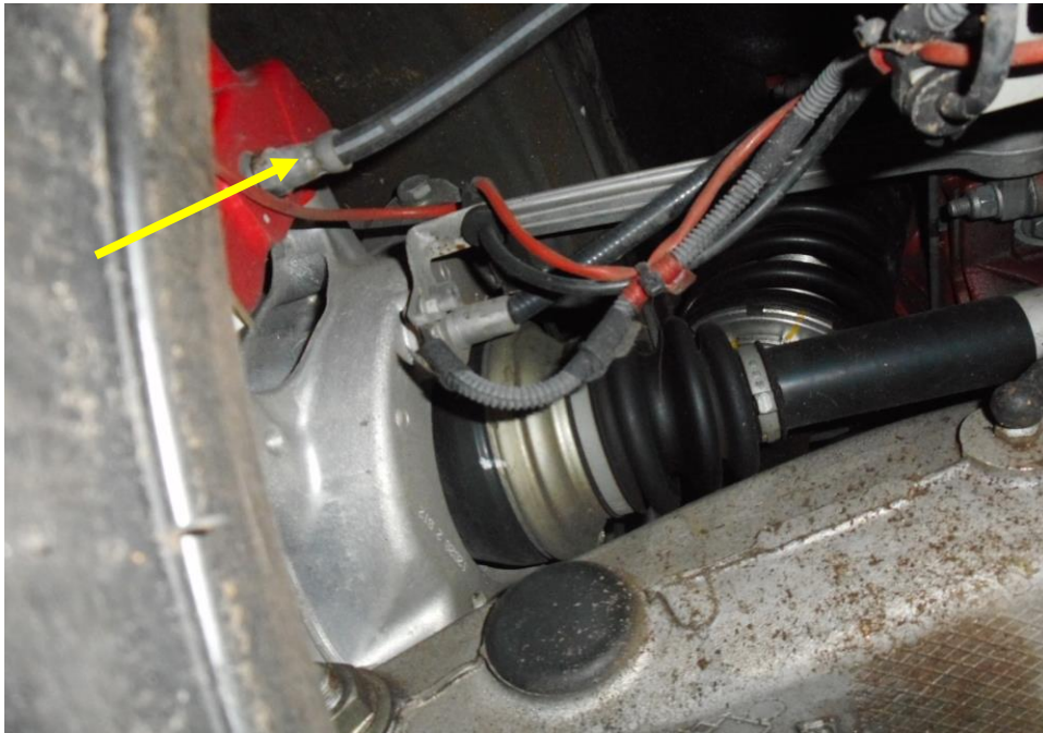
Photo 18 shows the brake hose/pipe (arrowed) at the rear right wheel of the Motor Car. No leakage of brake fluid was observed. Visual examination of the various components of the braking system like the drum brake, brake booster, brake pedal etc. had revealed all to be intact and without visible damage.
