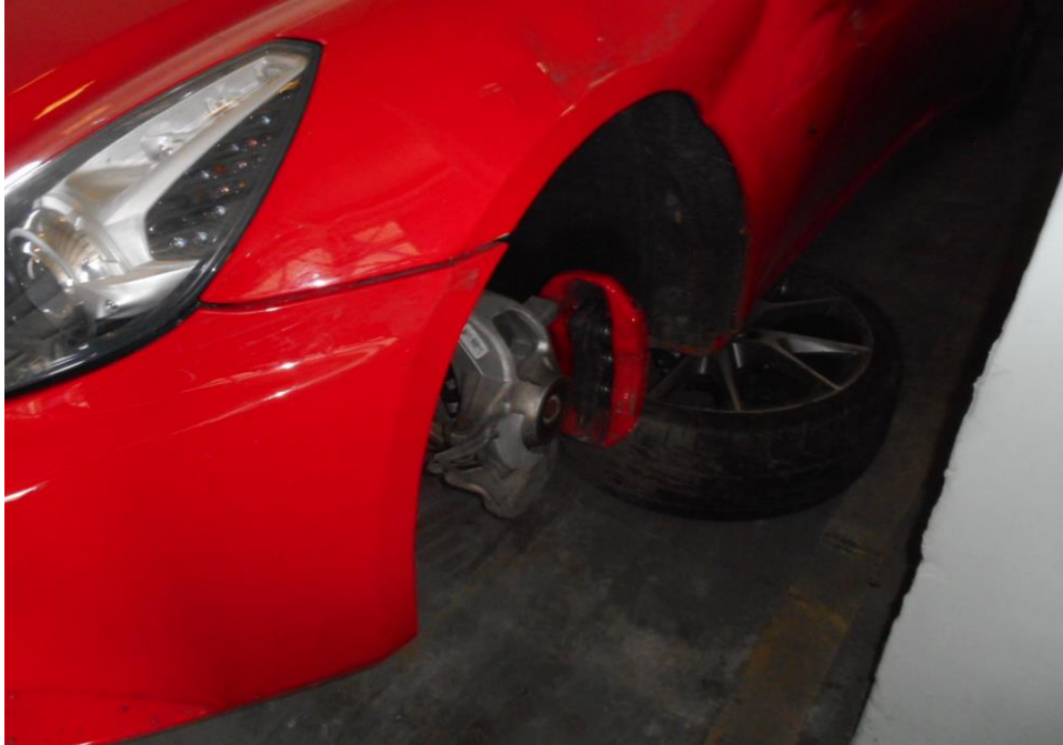
Photo 9 shows the condition of the front left tyre and rim of the Motor Car, which was observed to be broken off as a result of the accident.
