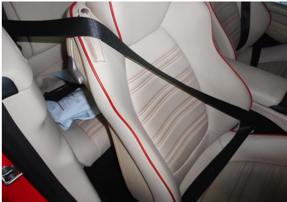
Photo 27 shows that the seat belt on the right seat were able to be fastened securely into the respective pre-tensioners that were fitted at the sides of the each seat.
