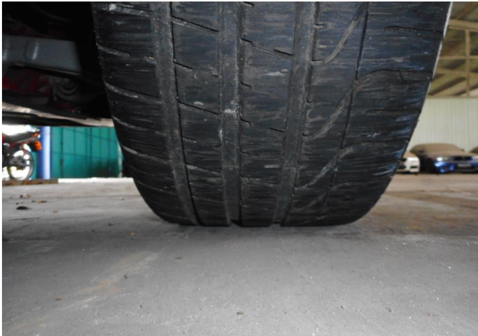
Photo 6 shows the condition of the front right tyre of the Motor Car, which was observed to be in serviceable condition with remaining tread depth of approximately 6.1mm. The tyre was also observed to be sufficiently inflated for vehicular operation with no tear, cut or burst mark(s).
