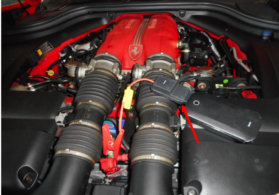
Photo 17 shows the use of a jump starter (arrowed) at the battery of the Motor Car. Despite multiple attempts in jumpstarting the Motor Car, the engine was not able to be started up.
