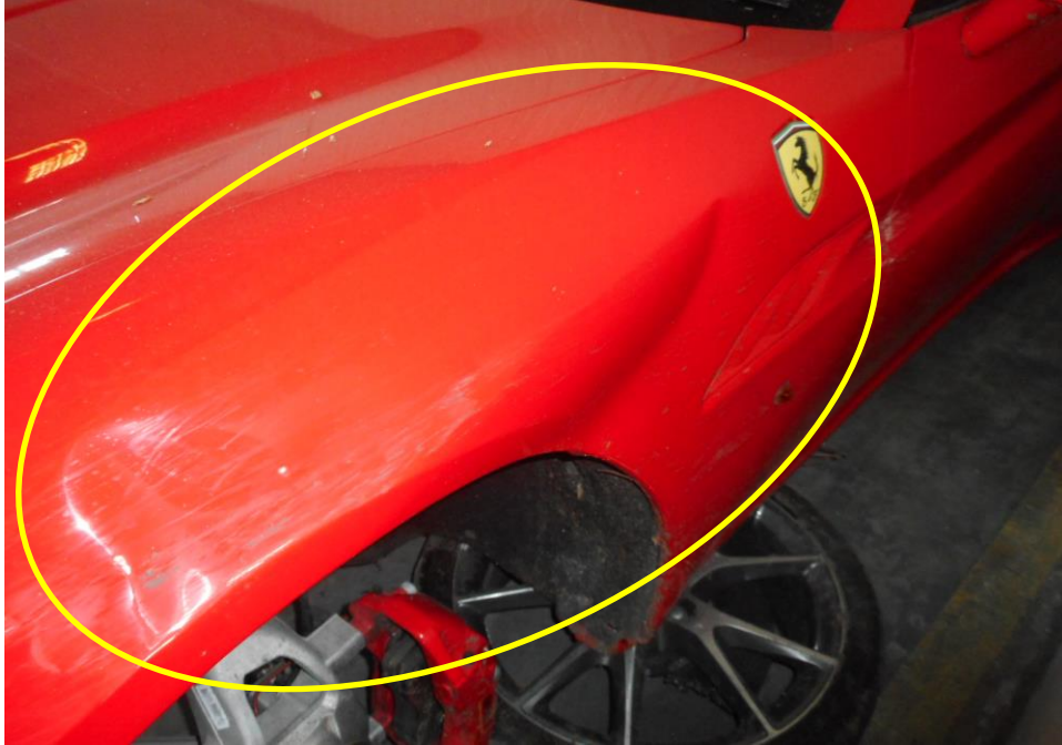
Photo 5 shows a close up view of the Motor Car's front portion at the time of my inspection. The left portion of the Motor Car was observed to have sustained damage to its front left fender (circled) were amongst the body part that were damaged as a result of the accident.
