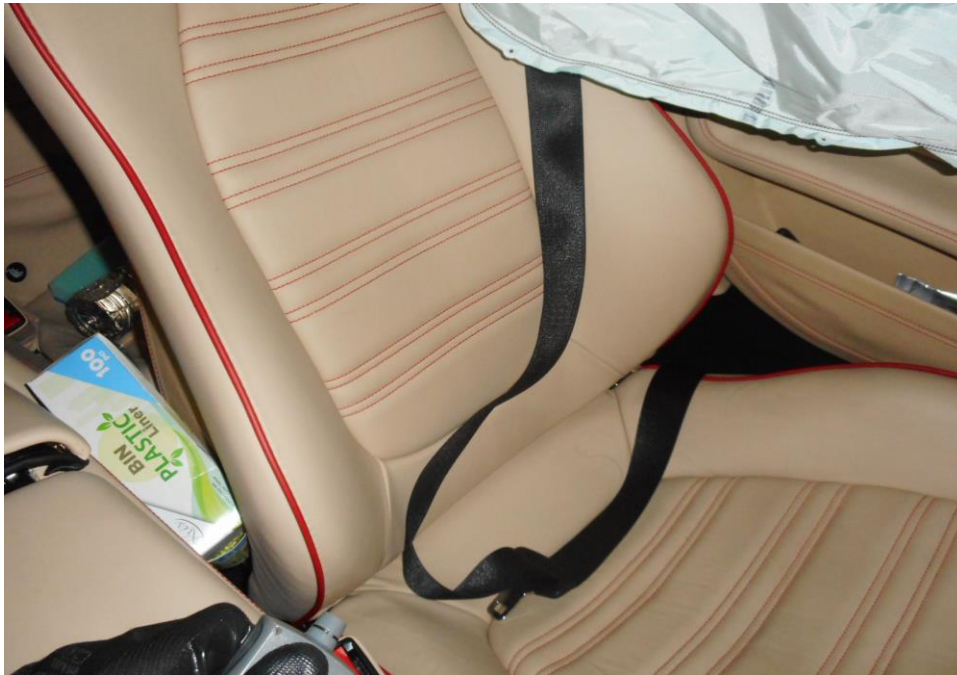
Photo 28 shows that the seat belt on the left seat was worn at the material time of accident as the safety pre-tensioners was activated at the moment of impact and caused the seat belt to be locked into the last position. The airbag was also deployed as of result of the accident.
