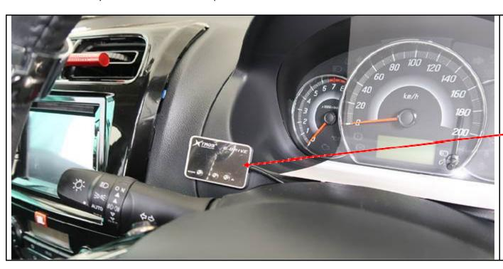
After mark Throttle controller. to improve response o venicle for pickup. Ca to difference of sensitivi
