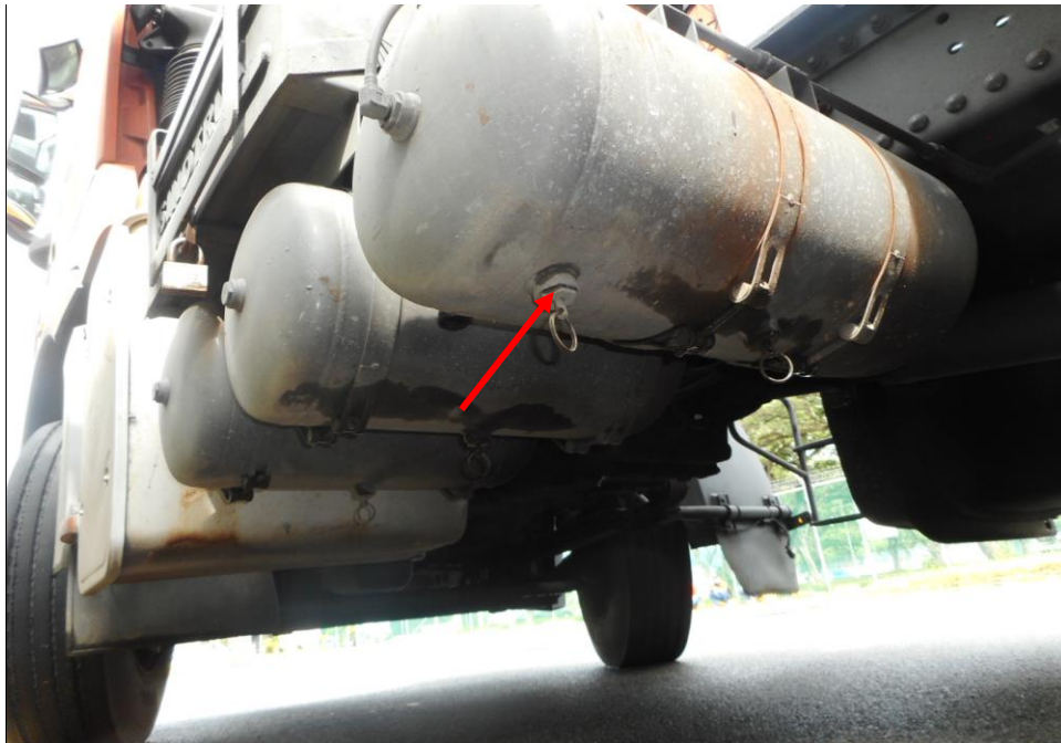
Photo 26 shows the air brake cylinders (arrowed) at the undercarriage of the Motor Trailer. I did not observe any leakage of air brake fluid at the time of my inspection of the Motor Trailer. My static tests of the Motor Trailer's braking system, along with my visual examination of the various mechanical components in the braking system had indicated that there was no internal leakage of pressure/vacuum. Hence the braking system of the Motor Trailer was likely to be in serviceable condition at the material time of accident.
