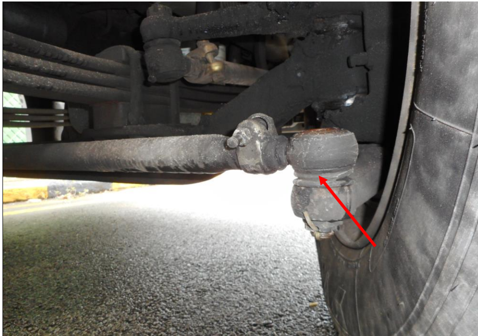
Photo 27 shows the various undercarriage components at the front right wheel of the Motor Trailer, in particular the steering tie rod end (arrowed). The various steering components were all found to be intact, suggesting that the steering system of the Motor Trailer was likely to be in serviceable condition at the material time of accident. There was also no sign of fluid stain(s) observed on the various undercarriage components.
