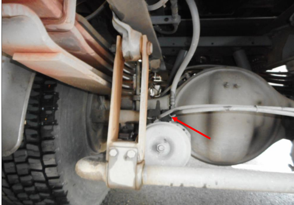
Photo 23 shows the brake pipe (arrowed) at the rear left wheel of the Motor Trailer. I did not observe any leakage of brake fluid at the time of my inspection of the Motor Trailer. My static tests of the Motor Trailer's braking system, along with my visual examination of the various mechanical components in the braking system, had indicated that there was no internal leakage of pressure/vacuum. Hence the braking system of the Motor Trailer was likely to be in serviceable condition at the material time of accident.
