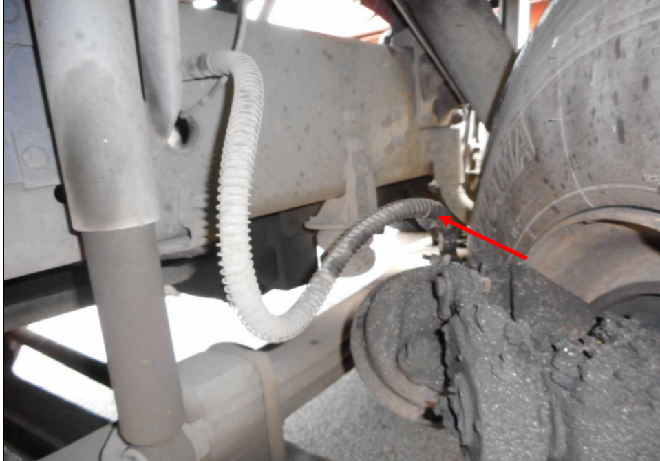
Photo 25 shows the brake pipe (arrowed) at the front left wheel of the Motor Trailer. I did not observe any leakage of brake fluid at the time of my inspection of the Motor Trailer. My static tests of the Motor Trailer's braking system, along with my visual examination of the various mechanical components in the braking system had indicated that there was no internal leakage of pressure/vacuum. Hence the braking system of the Motor Trailer was likely to be in serviceable condition at the material time of accident.
