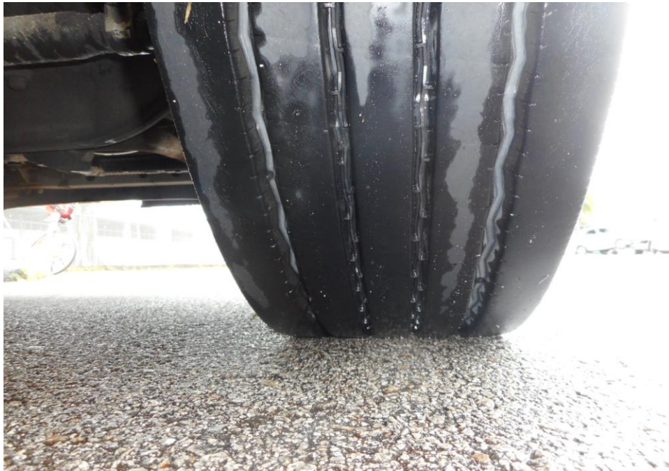
Photo 10 shows the condition of the front right tyre of the Motor Trailer, which was observed to be in serviceable condition with remaining tread depth of approximately 12.6 mm. The tyre, which was wrapped around standard steel wheel rim, was also observed to be sufficiently inflated for vehicular operation. There was no tear, cut or burst mark(s) on the outer and the inner sidewalls as well as across the tread of the 6 tyres that were fitted on the Motor Trailer.
