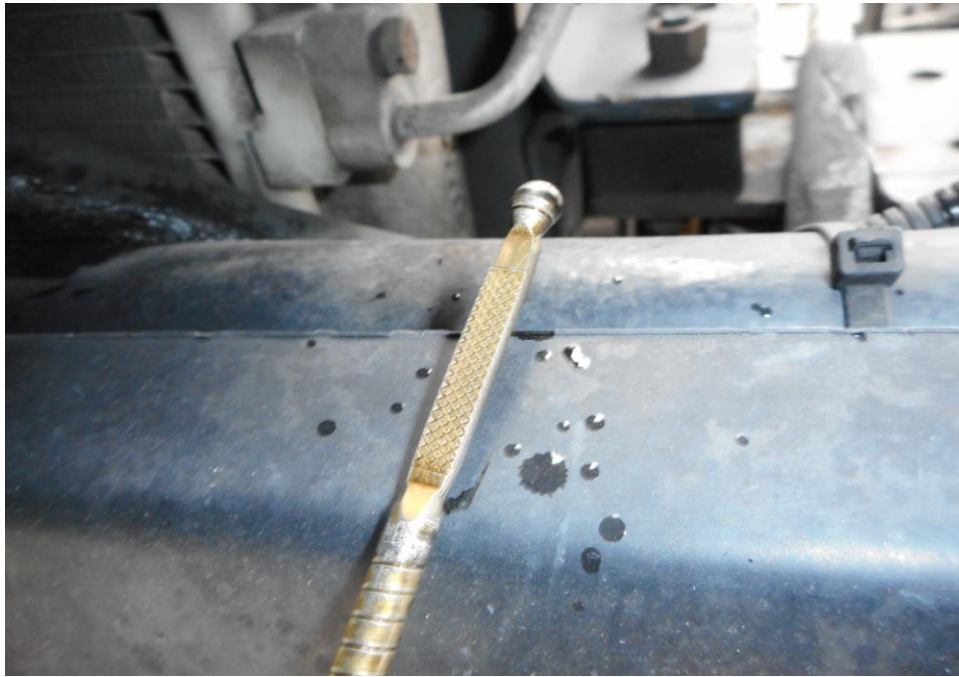
Photo 20 shows the engine oil dip stick of the Motor Trailer at the time of my inspection. The engine oil was observed to be of insufficient level at the time of our inspection.
