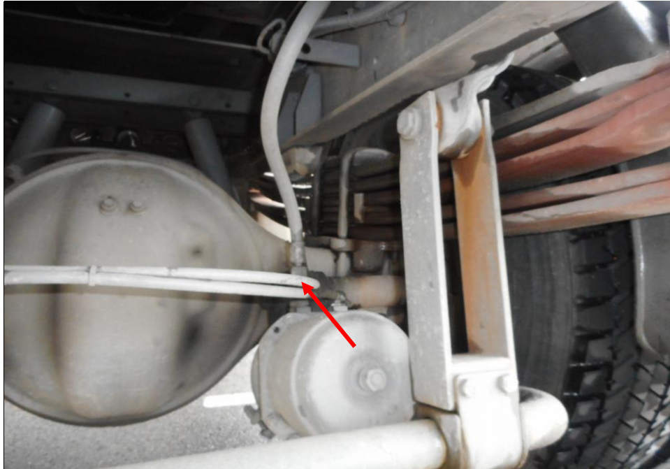
Photo 22 shows the brake pipe (arrowed) at the rear right wheel of the Motor Trailer. I did not observe any leakage of brake fluid at the time of my inspection of the Motor Trailer. My static tests of the Motor Trailer's braking system, along with my visual examination of the various mechanical components in the braking system, had indicated that there was no internal leakage of pressure/vacuum. Hence the braking system of the Motor Trailer was likely to be in serviceable condition at the material time of accident.
