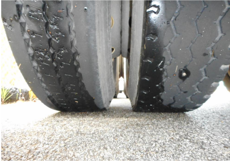
Photo 15 shows the condition of the left tyres of the trailer, which was observed to be in serviceable condition with remaining tread depth of approximately 6mm. The tyres, which were wrapped around standard steel wheel rim, were also observed to be sufficiently inflated for vehicular operation. There was also no damage found on all 6 steel wheel rims of the Motor Trailer.
