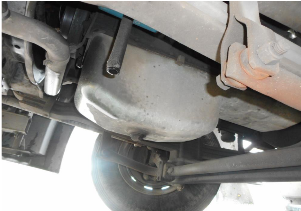
Photo 21 shows the undercarriage of the Motor Trailer, at the area where the engine housing located. I did not find any sign(s) or indication(s) of fluid leak, however old fluid stain(s) was observed on the underside of the Motor Trailer.
