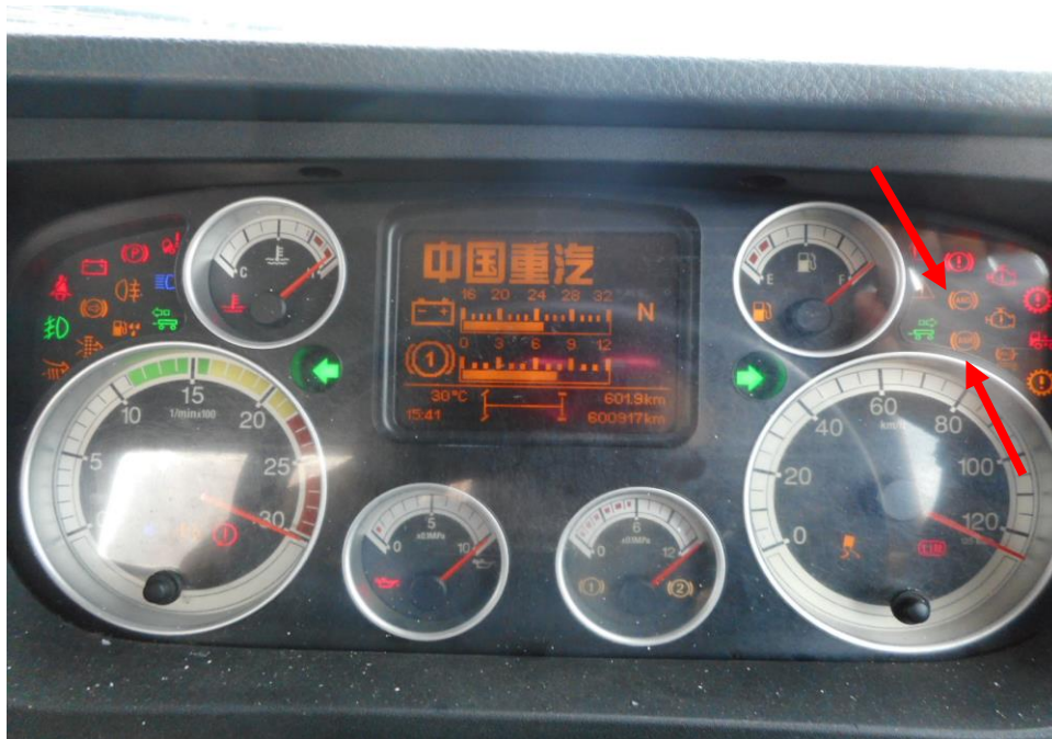
Photo 31 shows the warning light for Anti-Lock Brake System (ABS) and Traction Control System (TC) appearing on the instrument panel of the Motor Trailer during the self-test of its various electronic operating systems when its engine was cranked.
