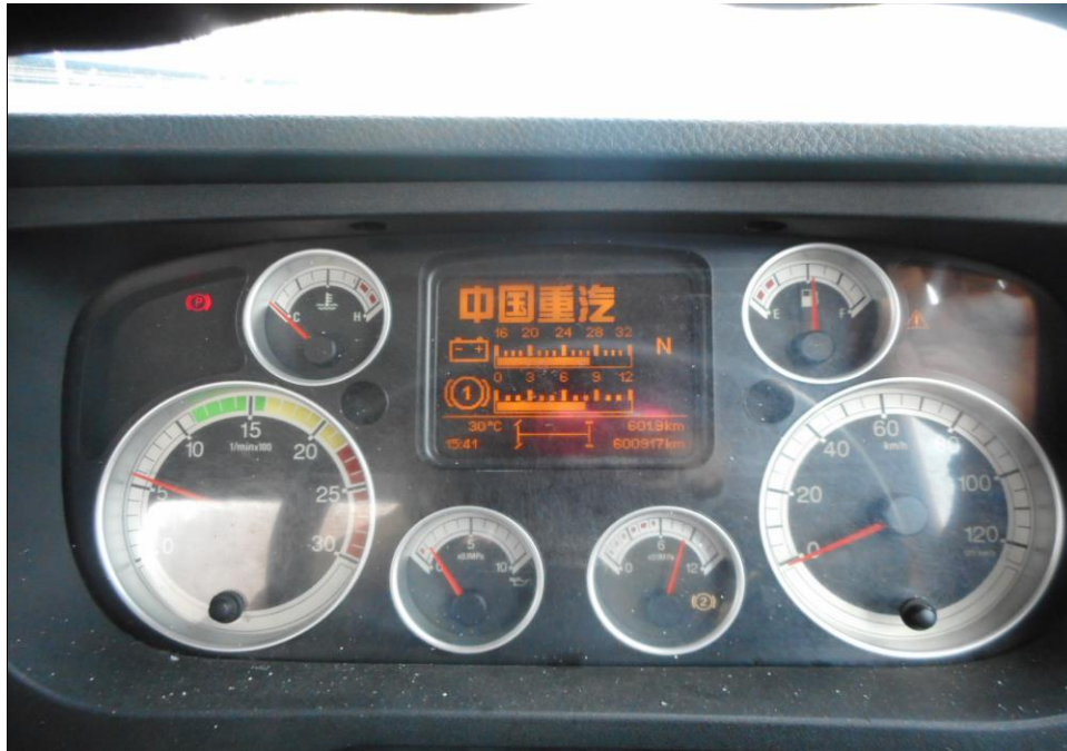
Photo 32 shows no warning lights illuminated on the instrument panel of the Motor Trailer after the engine was cranked. This would suggest that there was no abnormality to the various electronic operating systems of the Motor Trailer, like the ABS and TC.
