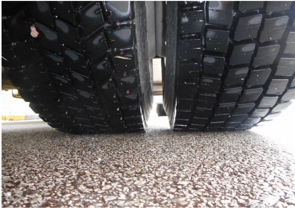
Photo 11 shows the condition of the rear right tyre of the Motor Trailer, which was observed to be in serviceable condition with remaining tread depth of approximately 14.4mm. The tyre, which was wrapped around standard steel wheel rim, was also observed to be sufficiently inflated for vehicular operation.
