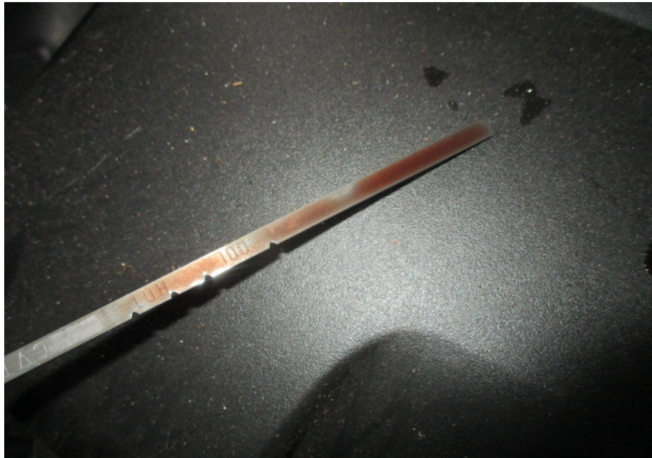
Photo 15 shows the automatic transmission fluid (ATF) dip stick of the Motor Car at the time of our inspection. The ATF was observed to be of sufficient level and without any visible contamination.
