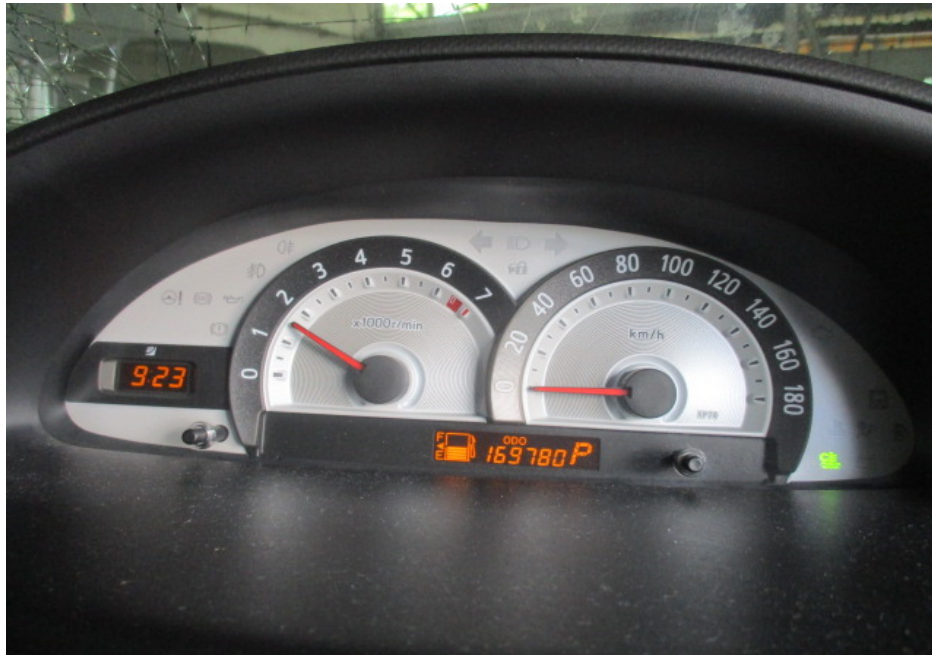
Photo 23 shows no warning lights illuminated on the instrument panel of the Motor Car after the engine was cranked. This would suggest that there was no abnormality to the various electronic operating systems of the Motor Car, like the ABS, EPS and SRS etc.
