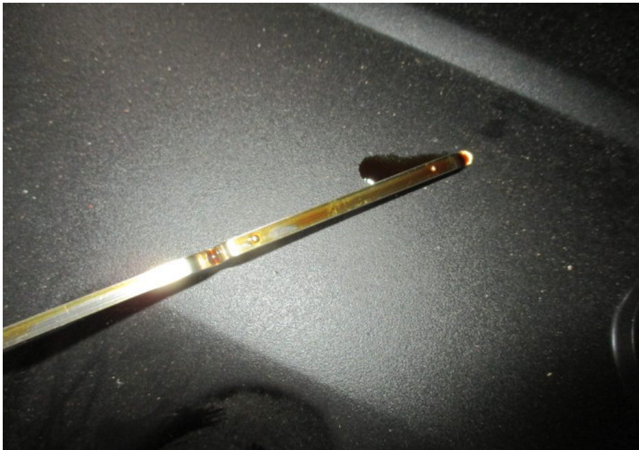
Photo 14 shows the engine oil dip stick of the Motor Car at the time of our inspection. The engine oil was observed to be of sufficient level and without any visible contamination.
