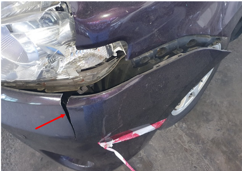
Photo 5 shows a closer view of the cracked front bumper (arrowed) of the Motor Car at the time of our inspection
