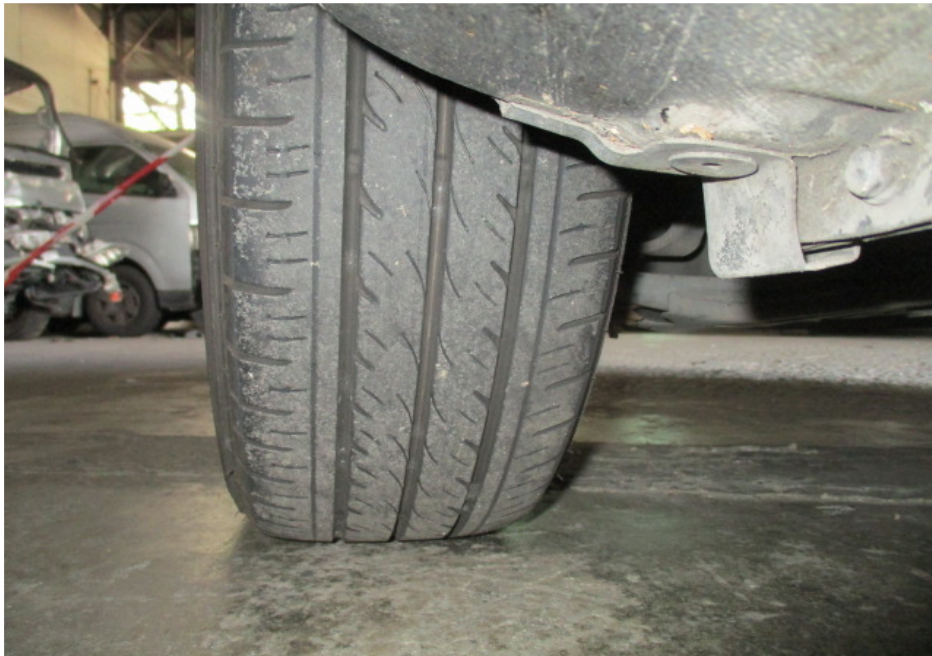
Photo 7 shows the condition of the front left tyre of the Motor Car, which was observed to be in serviceable condition with remaining tread depth of approximately 5mm. The tyre, which was wrapped around alloy wheel rim, was also observed to be sufficiently inflated for vehicular operation. There was no tear, cut or burst mark(s) on the outer and the inner sidewalls as well as across the tread of the 4 tyres.
