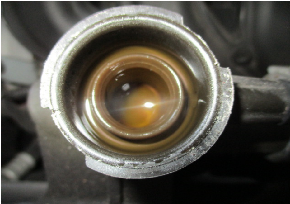
Photo 13 shows checks being carried out to the engine coolant of the Motor Car at the time of our inspection. The engine coolant was observed to be of sufficient level and without any visible contamination.
