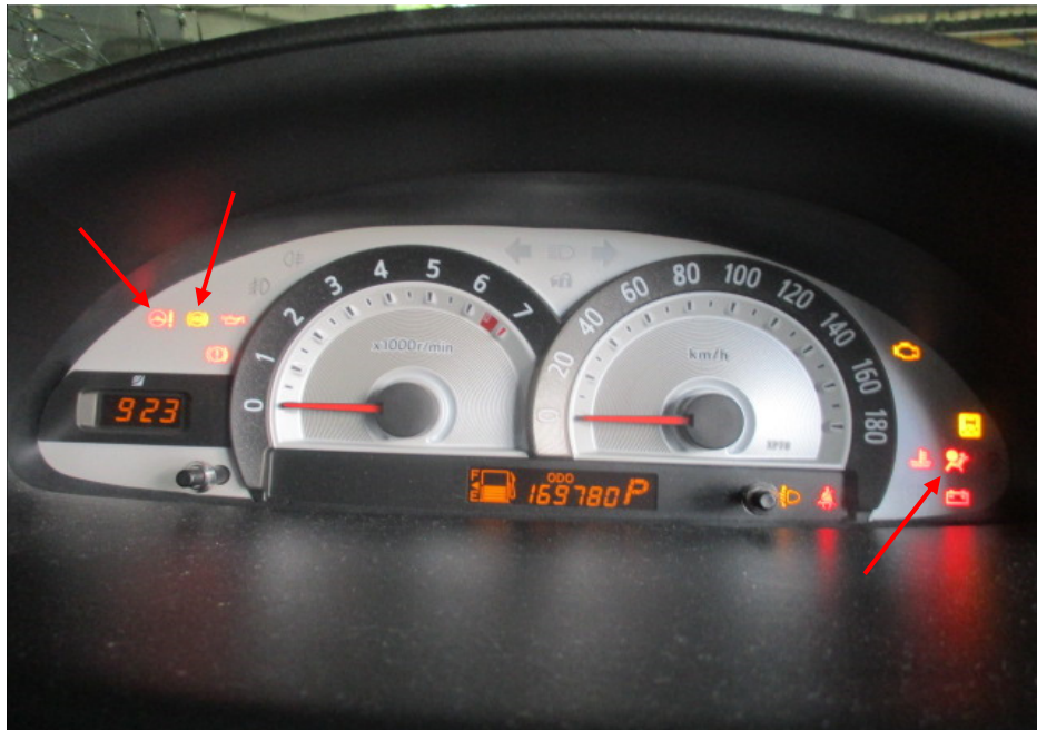
Photo 22 shows the warning lights for the various electronic operating systems of the Motor Car appearing on its instrument panel during the self-test when the engine is cranked, in particular the ABS light, EPS light and SRS light (arrowed).
