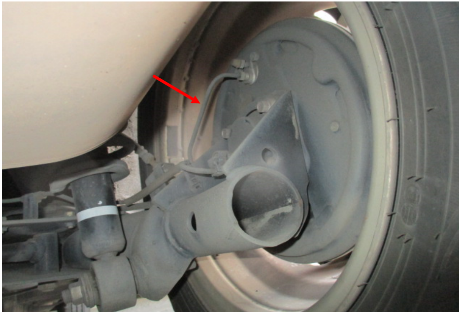
Photo 16 shows the brake hose/pipe (arrowed) at the rear right wheel of the Motor Car. We did not observe any leakage of brake fluid at the time of our inspection of the Motor Car. Static tests of the Motor Car's braking system had indicated that there was no internal leakage of pressure/vacuum. Hence the braking system was likely to be in serviceable condition at the material time of accident. The undercarriage components of the Motor Car were also all found to be intact and without any visible damage.
