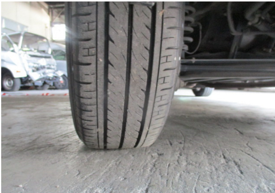
Photo 9 shows the condition of the rear left tyre of the Motor Car, which was observed to be in serviceable condition with remaining tread depth of approximately 5mm. The tyre, which was wrapped around alloy wheel rim, was also observed to be sufficiently inflated for vehicular operation. There was also no damage found on the 4 wheel rims of the Motor Car.
