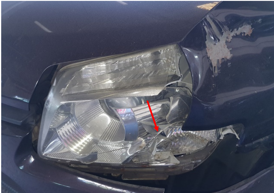
Photo 4 shows a closer view of the cracked left front headlamp (arrowed) of the Motor Car at the time of our inspection
