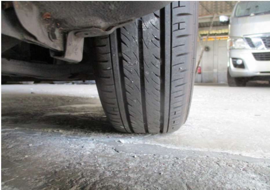
Photo 8 shows the condition of the front right tyre of the Motor Car, which was observed to be in serviceable condition with remaining tread depth of approximately 7mm. The tyre, which was wrapped around alloy wheel rim, was also observed to be sufficiently inflated for vehicular operation.
