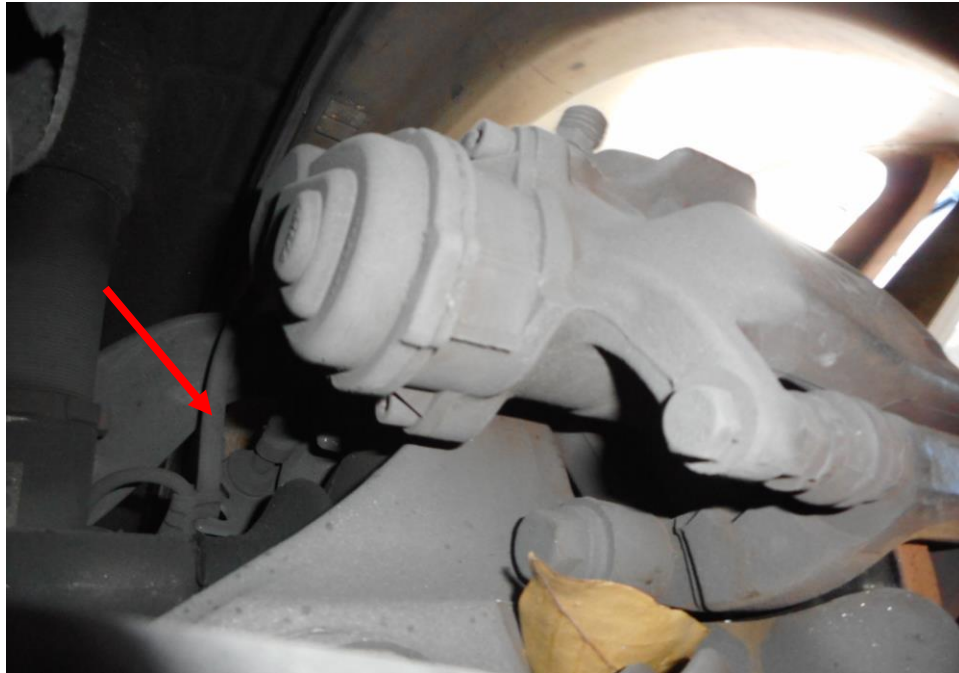
Photo 18 shows the brake hose/pipe (arrowed) at the rear right wheel of the Motor Car. No leakage of brake fluid was observed. Visual examination of the various components of the braking system like the brake caplier, brake booster, brake pedal etc. had revealed all to be intact and without visible damage.
