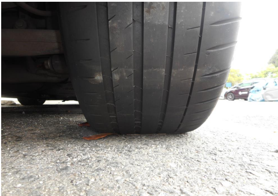
Photo 9 shows the condition of the rear right tyre of the Motor Car, which was observed to be in serviceable condition with remaining tread depth of approximately 3.7mm. The tyre was also observed to be sufficiently inflated for vehicular operation with no tear, cut or burst mark(s).
