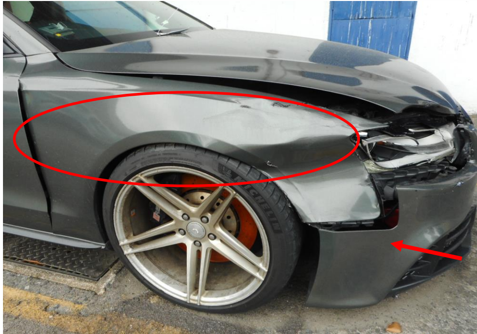
Photo 4 shows the close up view of the Motor Car's front body at the time of my inspection. Its front bumper (arrowed) and front right fender (circled) are the body parts that were damaged as a result of the accident.
