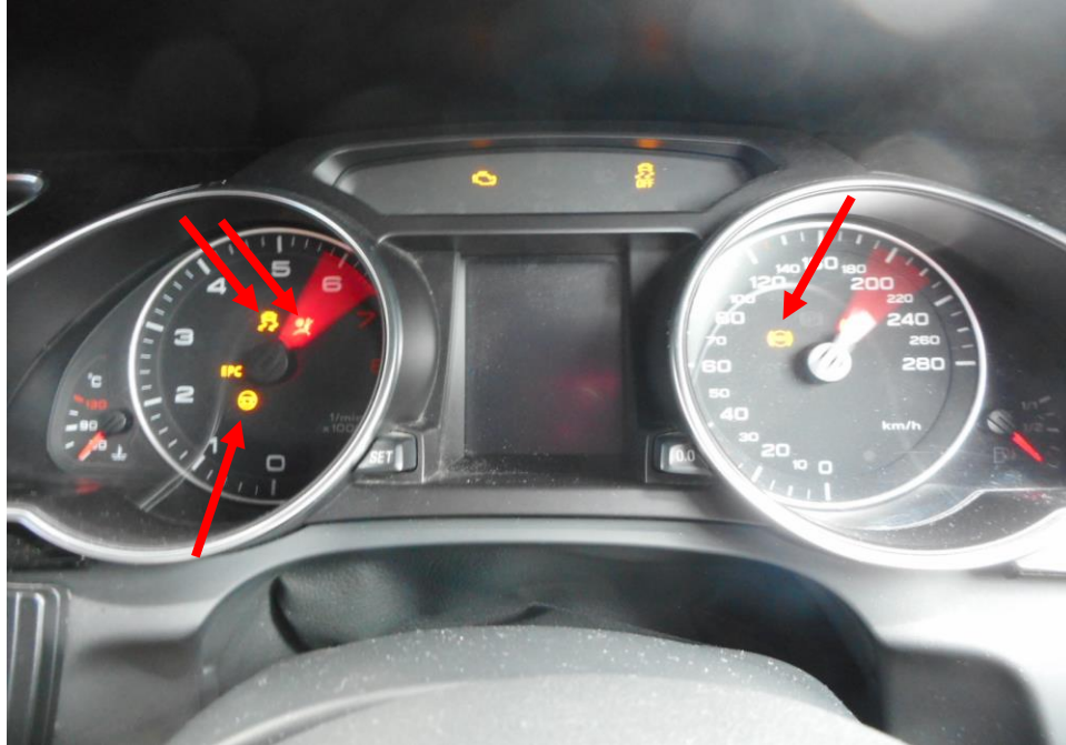
Photo 25 shows the warning light for Anti-Lock Brake System (ABS) and Power Steering System (EPS), Traction Control System (TCS) and Supplemental Restraint System (SRS) (arrowed) appearing on the instrument panel of the Motor Car during the self-test of its various electronic operating systems when its engine was cranked.
