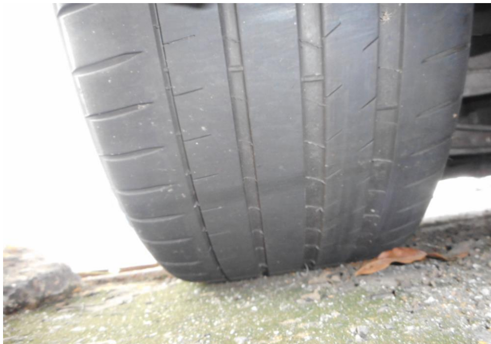
Photo 11 shows the condition of the front left tyre of the Motor Car, which was observed to be in serviceable condition with remaining tread depth of approximately 3.9mm. The tyre, which was wrapped around steel wheel rim, was also observed to be sufficiently inflated for vehicular operation. The 4 tyres of the Motor Car were wrapped around standard steel wheel rims.
