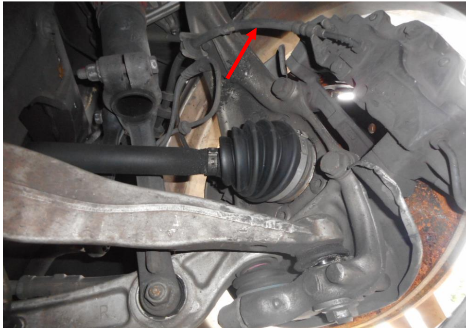
Photo 20 shows the brake hose/pipe (arrowed) at the front right wheel of the Motor Car. I did not observe any leakage of brake fluid at the time of my inspection of the Motor Car. Static tests of the Motor Car's braking system had indicated that there was no internal leakage of pressure/vacuum. The undercarriage components of the Motor Car were also all found to be intact and without any visible damage.
