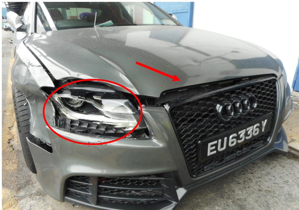
Photo 3 shows the close up view of the Motor Car's front body at the time of my inspection. Its front bonnet (arrowed) and front left headlamp (circled) are the body parts that were damaged as a result of the accident.
