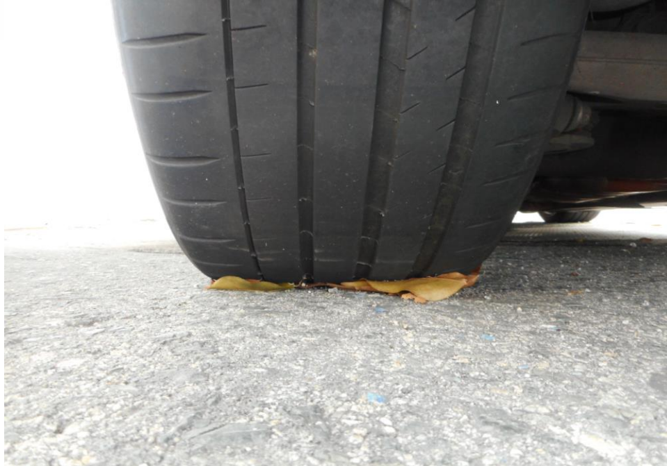
Photo 10 shows the condition of the rear left tyre of the Motor Car, which was observed to be in serviceable condition with remaining tread depth of approximately 3.8mm. The tyre, which was wrapped around steel wheel rim, was also observed to be sufficiently inflated for vehicular operation. The 4 tyres of the Motor Car were wrapped around standard steel wheel rims.
