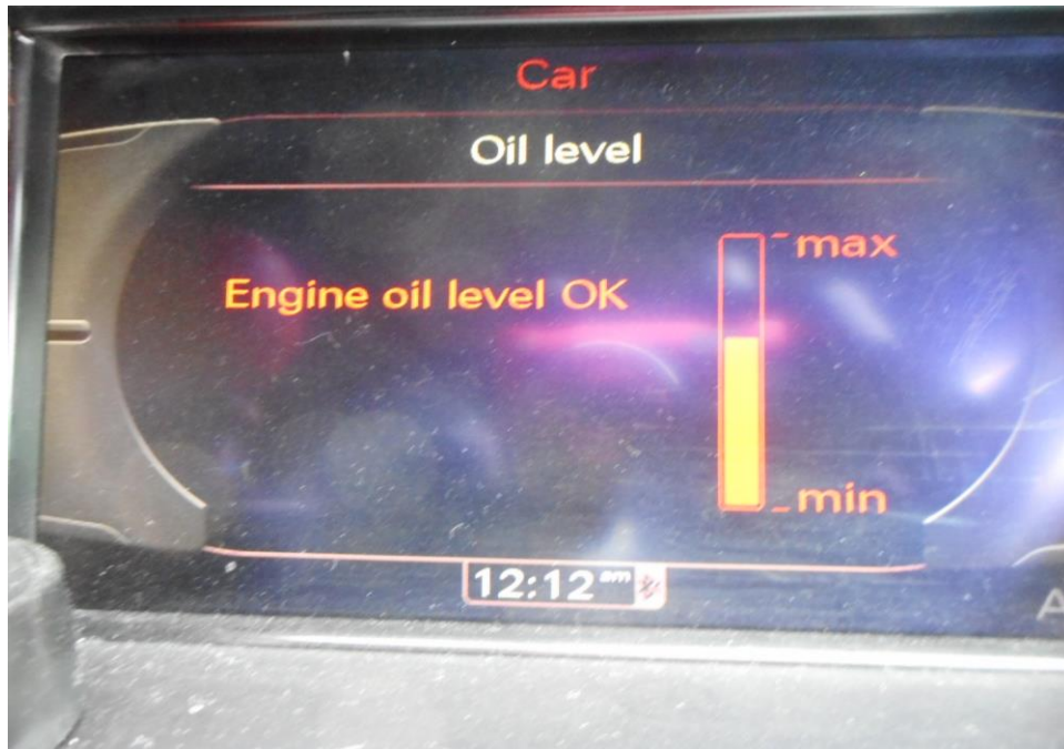
Photo 15 shows the engine oil level display of the Motor Car at the time of my inspection. The engine oil was observed to be of sufficient level and without any visible contamination.
