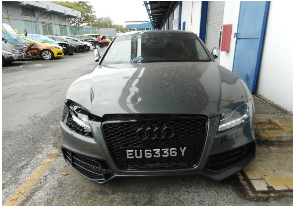
Photo 2 shows a general view of the Motor Car's front body at the time of my inspection. Its front bonnet, front bumper, front right fender and front right headlamp are the body parts that were damaged as a result of the accident.
