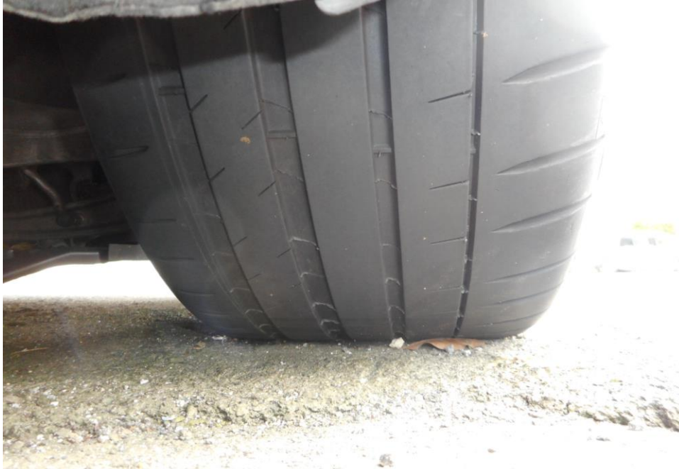
Photo 8 shows the condition of the front right tyre of the Motor Car, which was observed to be in serviceable condition with remaining tread depth of approximately 3.7mm. The tyre was sufficiently inflated for vehicular operation with no tear, cut or burst mark(s) on the outer and the inner sidewalls as well as across the tread. The 4 tyres of the Motor Car were wrapped around standard steel wheel rims without any damage.
