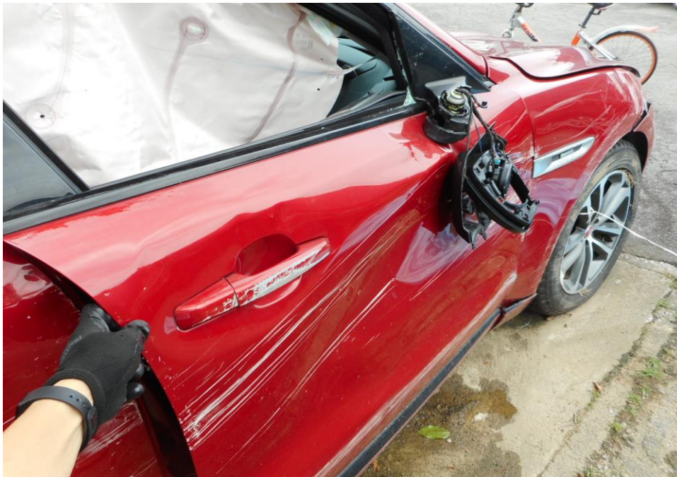
Photo 15 shows the close view of the Motor Car's right body at the time of my inspection. The Motor Car was observed to have sustained damage on its right door and the door was unable to open due to the result of the accident.
