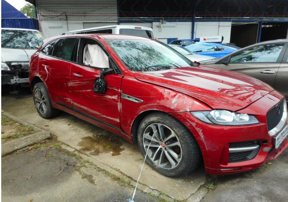
Photo 5 shows the general view of the Motor Car's right body at the time of my inspection. The Motor Car was observed to have sustained damage on its right body panels were amongst the body parts that were damaged as a result of the accident.
