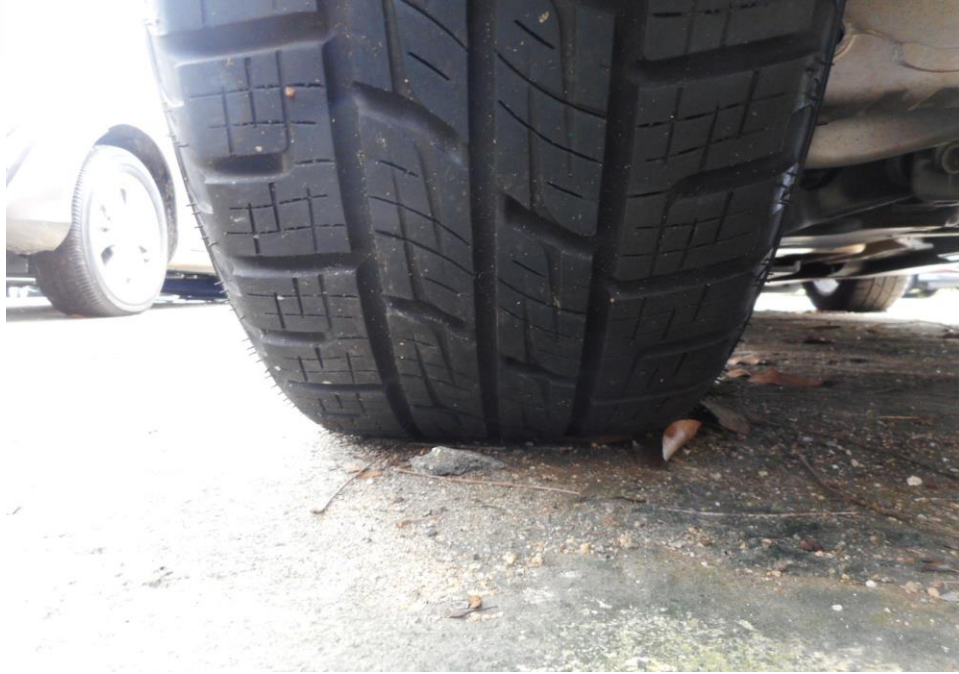
Photo 11 shows the condition of the rear left tyre of the Motor Car, which was observed to be in serviceable condition with remaining tread depth of approximately 4.8mm. There was also no tear, cut or burst mark(s) on the outer and the inner sidewalls as well as across the tread of the Motor Car's 3 left tyres.
