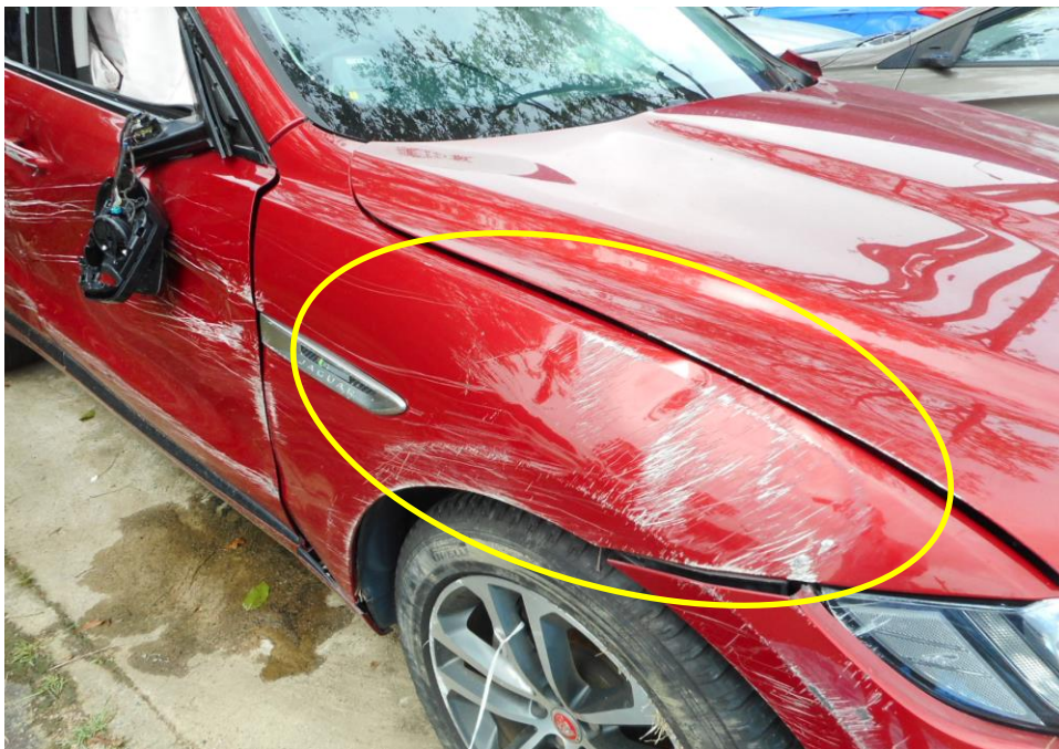
Photo 6 shows the close view of the Motor Car's right body at the time of my inspection. The Motor Car was observed to have sustained damage on its right body panels (circled) were amongst the body parts that were damaged as a result of the accident.
