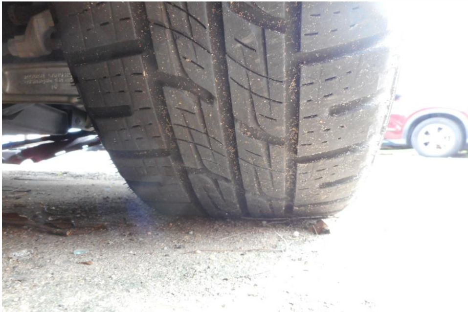
Photo 9 shows the condition of the front right tyre of the Motor Car, which was observed to be in serviceable condition with remaining tread depth of approximately 5mm. There was also no tear, cut or burst mark(s) on the outer and the inner sidewalls as well as across the tread of the Motor Car's 3 left tyres.
