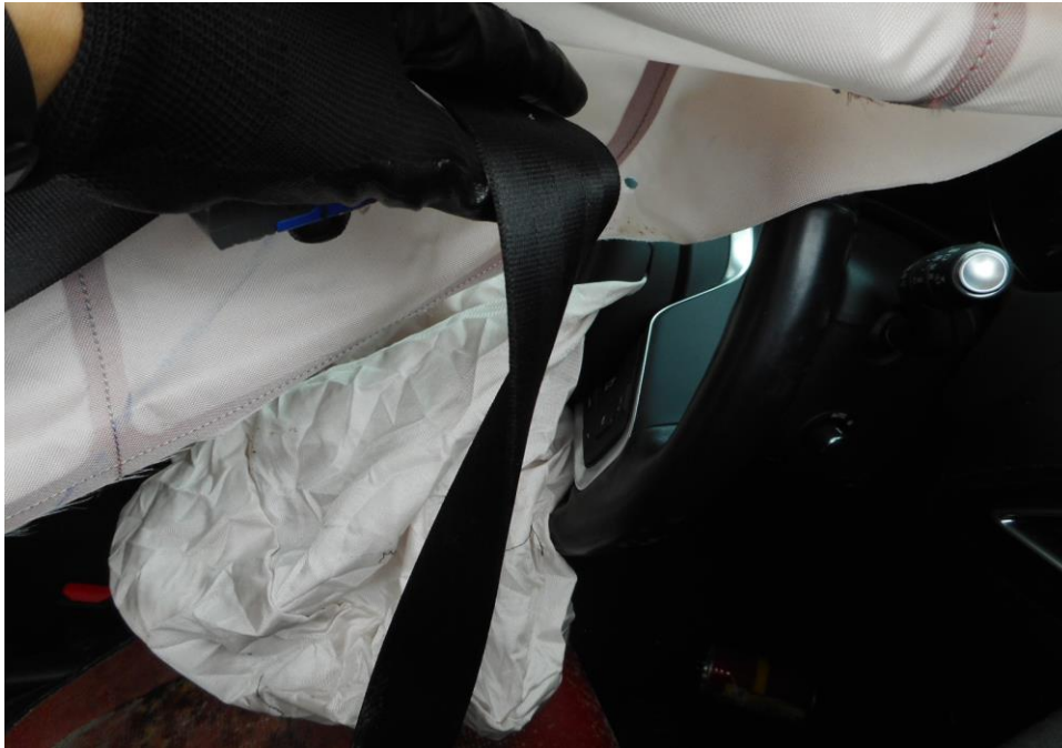
Photo 24 shows that that the seat belt on the right seat was worn at the material time of accident as the safety pre-tensioners was activated at the moment of impact and caused the seat belt to be locked into the last position.
