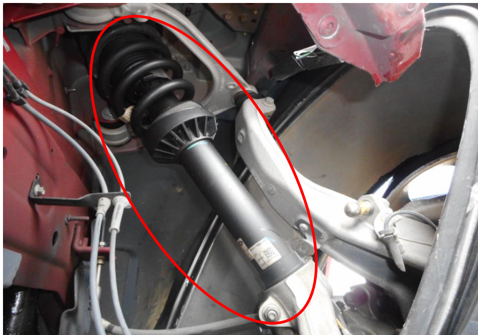
Photo 22 shows the various undercarriage components at the front left wheel of the Motor Car, the suspension system (circled) was observed to be damaged as a result of the accident.
