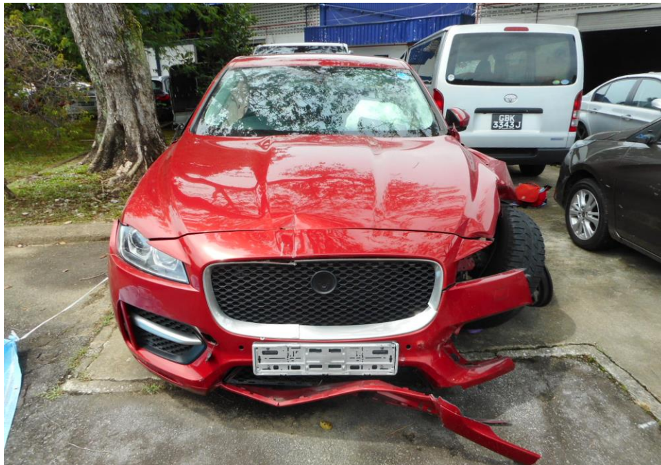
Photo 2 shows a general view of the Motor Car's front body at the time of my inspection. The Motor Car was observed to have sustained damage all around. Its front windscreen, front bonnet, front bumper, front left headlamp, its front left fender, front right side mirror and right body panels, were amongst the body parts that were damaged as a result of the accident. The Supplemental Restraint System (SRS) was activated as a result of the accident.
