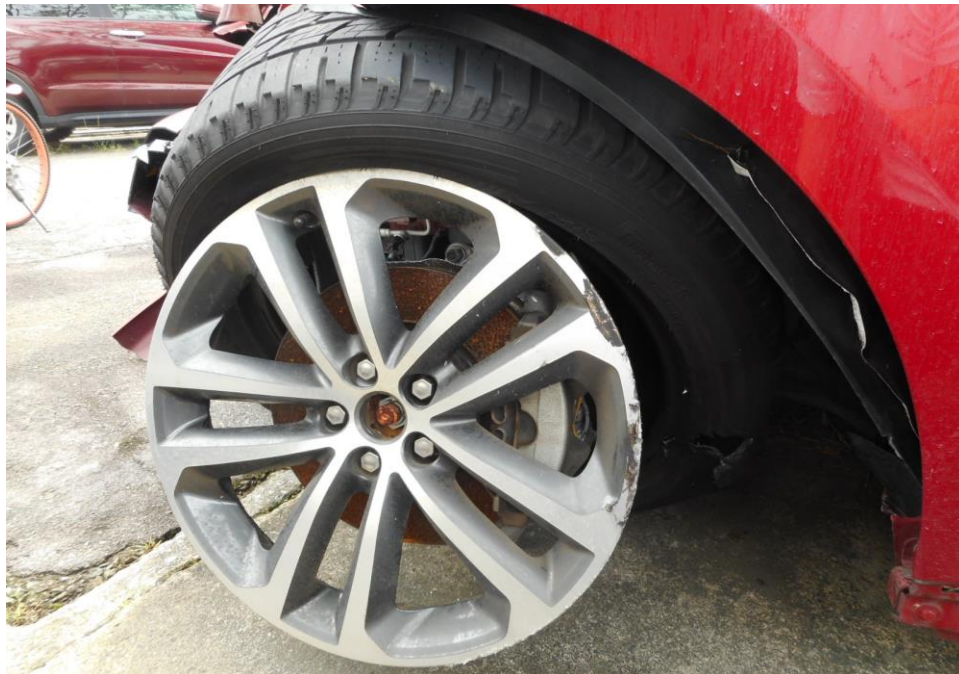
Photo 12 shows the condition of the front left tyre and wheel rim of the Motor Car, which was observed to be in unserviceable condition as it was damaged and slipped off the wheel rim as a result of the accident with remaining tread depth of approximately 4.9mm.
