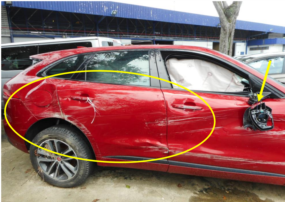
Photo 7 shows the close view of the Motor Car's right body at the time of my inspection. The Motor Car was observed to have sustained damage on its right body panels (circled) and right side mirror (arrowed) were amongst the body parts that were damaged as a result of the accident.
