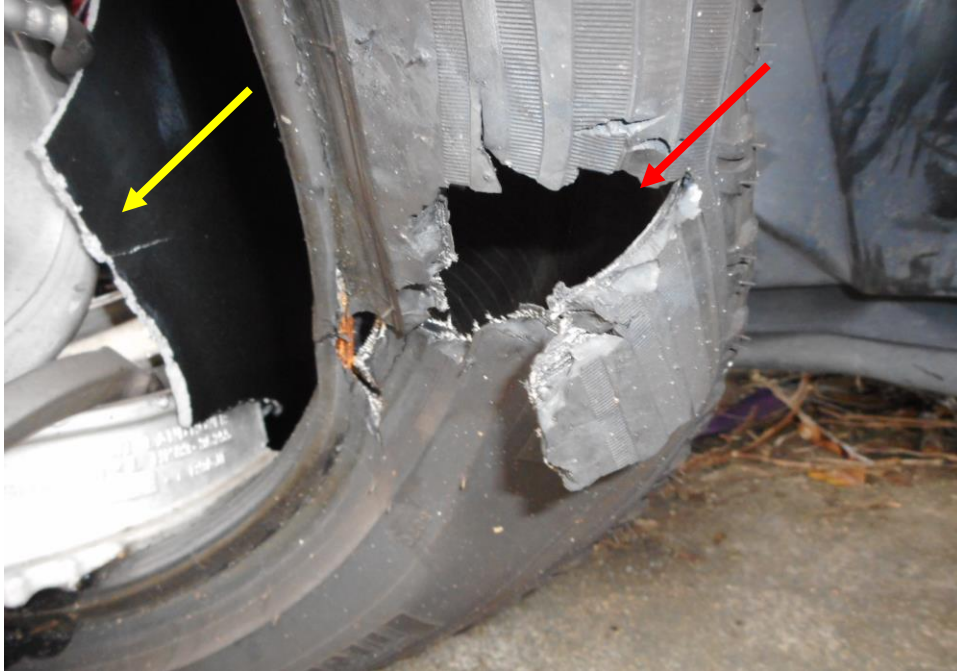
Photo 13 shows the close up condition of the front left tyre and rim of the Motor Car, which was observed that the tyre was cut (red arrow) and the wheel rim (yellow arrow) was broken, the broken wheel rim had likely caused cut on the tyre in the midst of the accident due to the impact it sustained from the collision.
