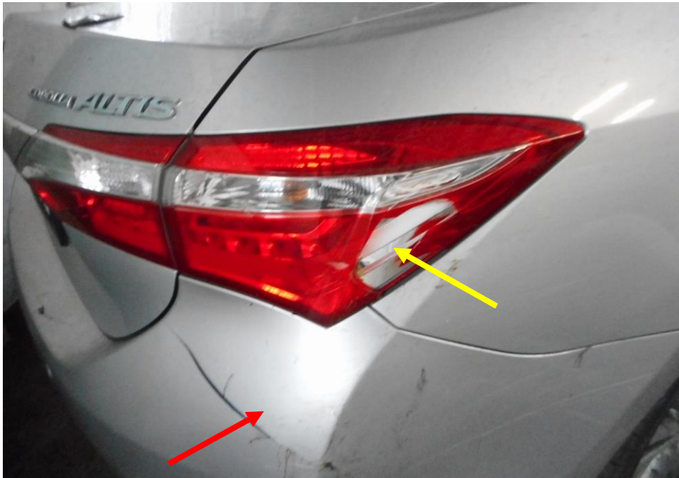
Photo 5 shows a close up view of the rear body of the Motor Car at the time of my inspection. The Motor Car was observed to be sustained damage at its rear right brake lamp (yellow arrow) and rear bumper (red arrow) as a result of the accident
