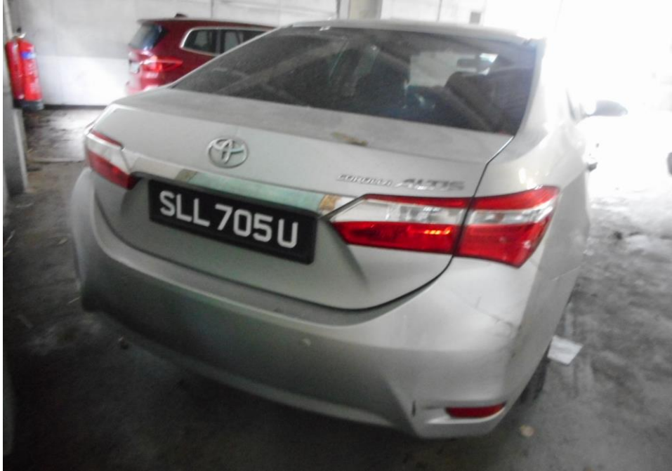
Photo 4 shows a general view of the rear body of the Motor Car at the time of my inspection. The Motor Car was observed to be sustained damage at its rear right brake lamp and rear bumper as a result of the accident
