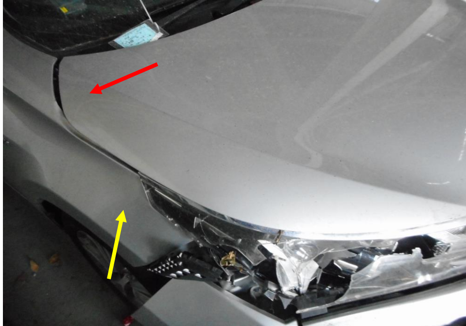
Photo 2 shows a close up view of the Motor Car at the time of my inspection. The Motor Car was observed to have sustained damage at its front portion. Its front bonnet (red arrow) and front right fender (red arrow) was amongst the body parts that were damaged as a result of the accident.
