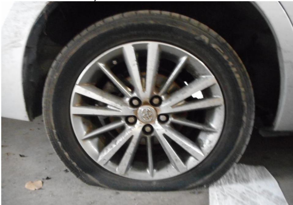
Photo 9 shows the condition of the rear right tyre of the Motor Car, which was observed to be deflated likely due to the result of the accident. The remaining tread depth was of approximately 4.4mm. There was no tear, cut or burst mark(s) on the outer and the inner sidewalls as well as across the tread of the tyre that were fitted on the Motor Car.
