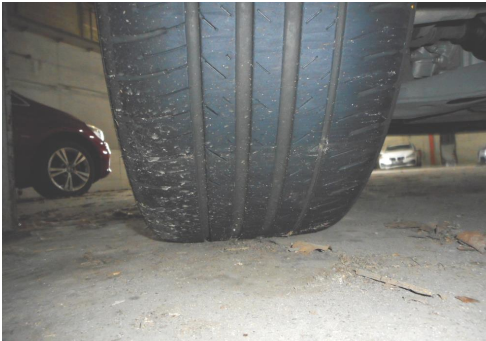
Photo 11 shows the condition of the rear right tyres of the Motor Car, which were observed to be in serviceable condition with remaining, tread depth of approximately 3.2mm. There was also no tear, cut or burst mark(s) on the outer and the inner sidewalls as well as across the tread of the 4 tyres that were fitted on the Motor Car.
