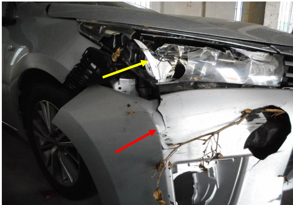
Photo 3 shows a close up view of the Motor Car at the time of my inspection. The Motor Car was observed to have sustained damage at its front portion. Its front bumper (red arrow) and front right headlamp (yellow arrow) was amongst the body parts that were damaged as a result of the accident.
