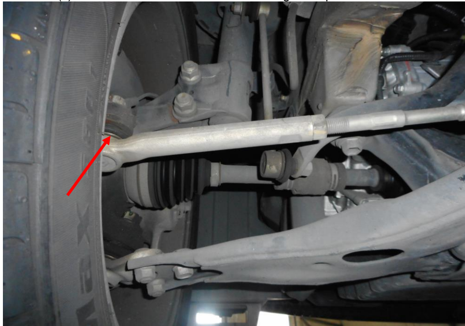
Photo 19 shows the various undercarriage components at the front left wheel of the Motor Car, in particular the steering tie rod end (arrowed). The various Undercarriage components of the Motor Car were all found to be intact without any visible damage. There was also no sign of fluid stain(s) observed on the various undercarriage components.
