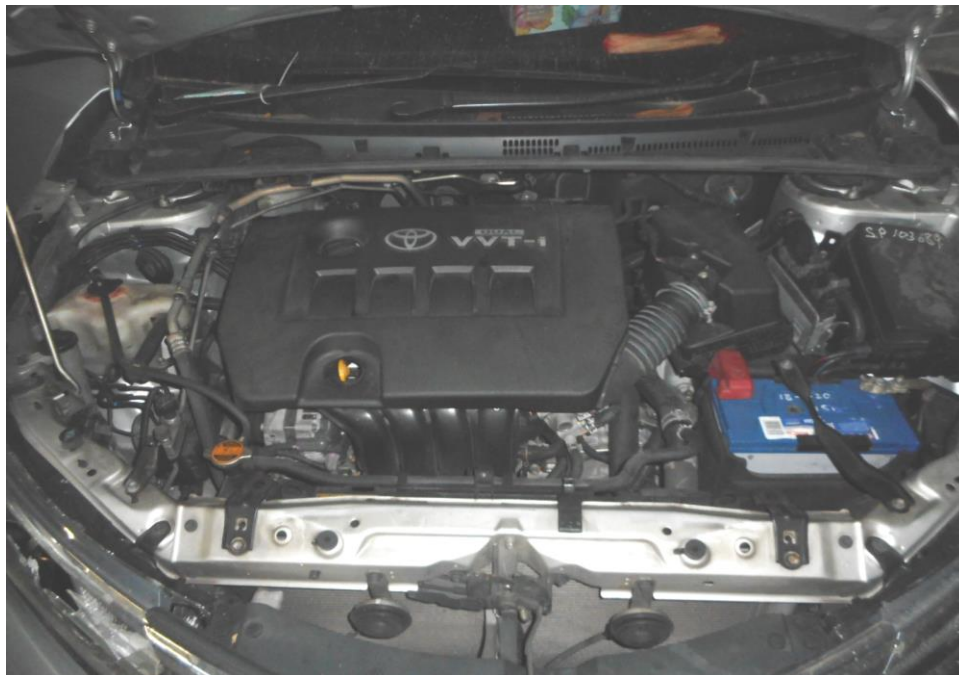
Photo 12 shows a general view of the Motor Car's engine compartment, which was accessed by lifting the front cabin of the Motor Car. The various parts and components inside the engine compartment were unaffected by the accident. There was also no sign(s) or indication(s) of fresh fluid leakage and/or fluid stain within the engine compartment
