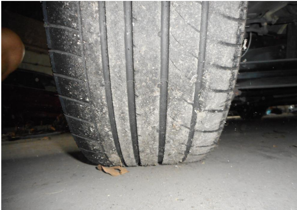
Photo 10 shows the condition of the rear left tyres of the Motor Car, which was observed to be in serviceable condition with remaining tread depth of approximately 4.4mm. The tyres, which were wrapped around standard alloy wheel rim, were also observed to be sufficiently inflated for vehicular operation. There was also no damage found on all 4 alloy wheel rims of the Motor Car.
