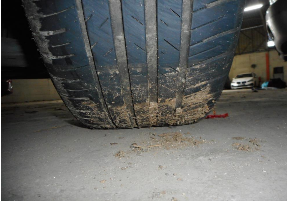
Photo 8 shows the condition of the front right tyre of the Motor Car, which was observed to be in serviceable condition with remaining tread depth of approximately 4mm. The tyre, which was wrapped around standard alloy wheel rim, was also observed to be sufficiently inflated for vehicular operation. There was no tear, cut or burst mark(s) on the outer and the inner sidewalls as well as across the tread of the 4 tyres that were fitted on the Motor Car.
