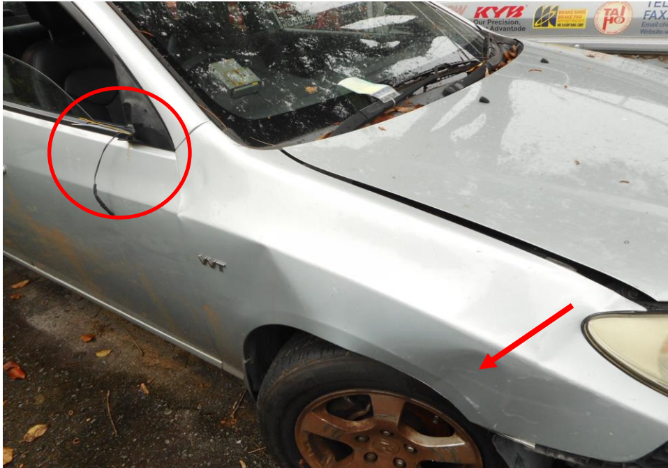
Photo 6 shows the close up view of the Motor Car's front body at the time of my inspection. Its right rear view mirror (circled) and front right fender (arrowed) are the body parts that were damaged as a result of the accident.
