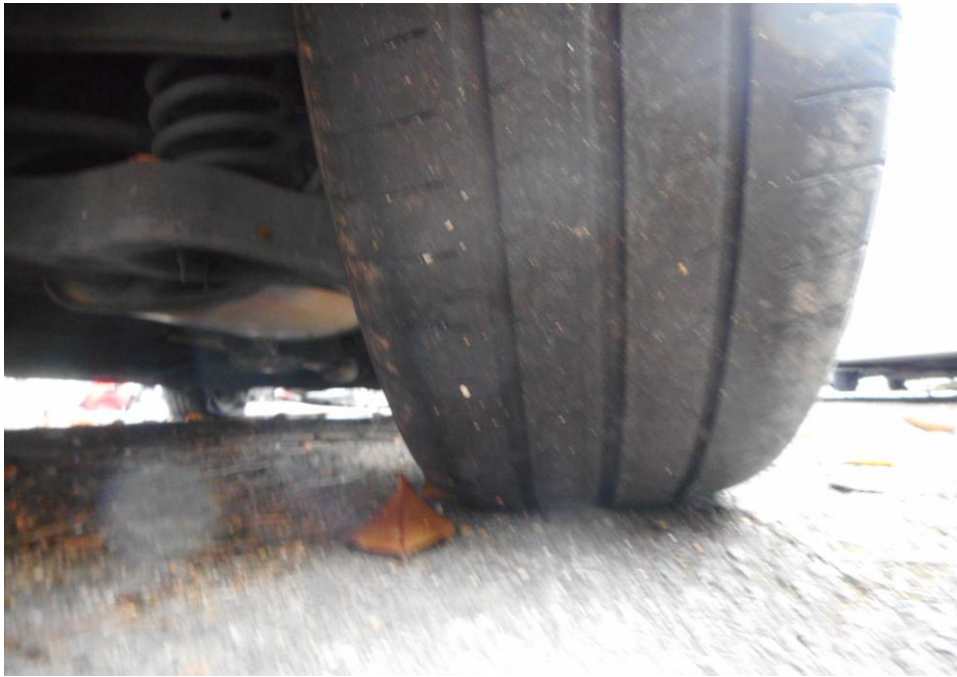
Photo 10 shows the condition of the rear right tyre of the Motor Car, which was observed to be in serviceable condition with remaining tread depth of approximately 2.8mm. The tyre was also observed to be sufficiently inflated for vehicular operation with no tear, cut or burst mark(s).
