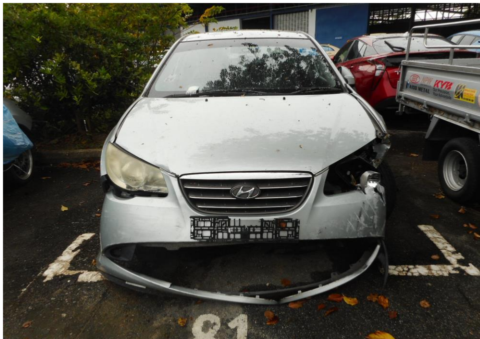
Photo 3 shows a general view of the Motor Car's front body at the time of my inspection. Its front bonnet, front bumper, front left and right fender, front left headlamp and the right rear view mirror are the body parts that were damaged as a result of the accident.
