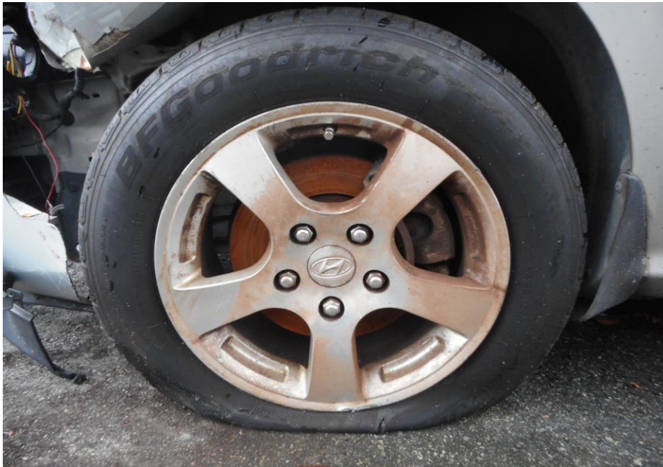
Photo 12 shows the condition of the front left tyre of the Motor Car, which was observed to be cut and deflated likely due to the result of the accident. The with remaining tread depth of approximately 5.3mm
