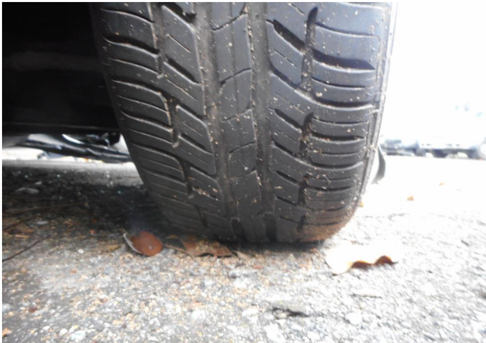
Photo 9 shows the condition of the front right tyre of the Motor Car, which was observed to be in serviceable condition with remaining tread depth of approximately 5.5mm. The tyre was sufficiently inflated for vehicular operation with no tear, cut or burst mark(s) on the outer and the inner sidewalls as well as across the tread. The 3 tyres of the Motor Car were wrapped around standard steel wheel rims without any damage.
