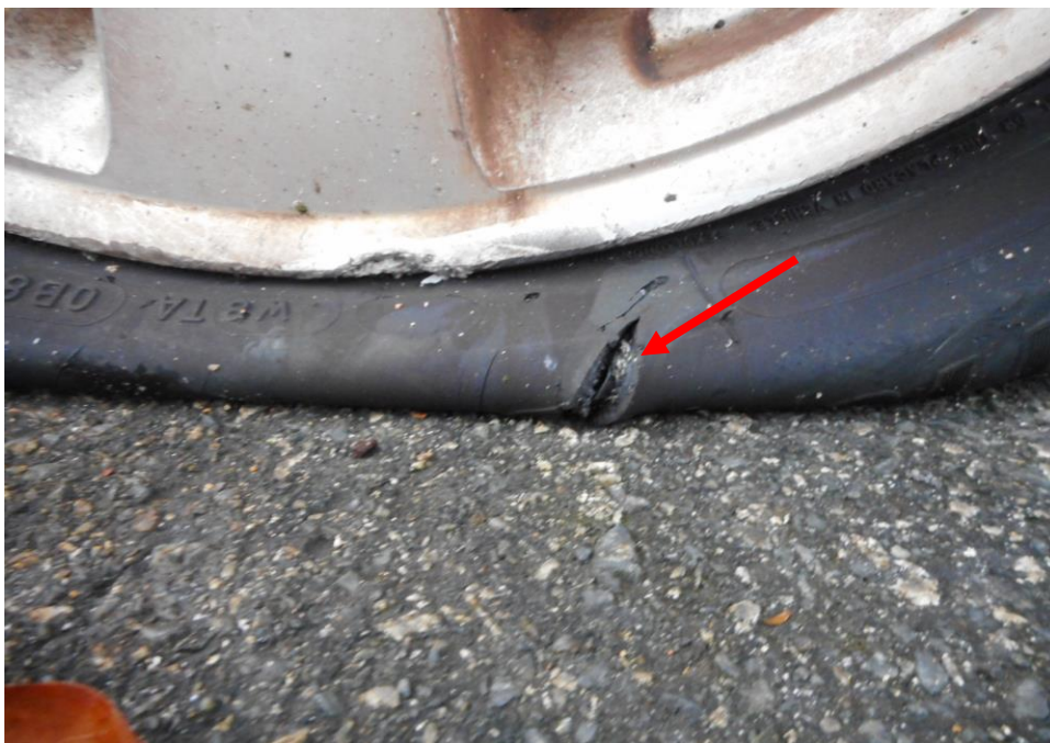
Photo 13 shows the close up condition of the front left tyre of the Motor Car, which was observed to be cut and deflated (arrowed) likely due to the result of the accident.
