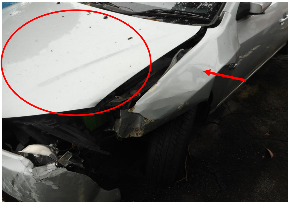
Photo 5 shows the close up view of the Motor Car's front body at the time of my inspection. Its front bonnet (circled) and front left fender (arrowed) are the body parts that were damaged as a result of the accident.
