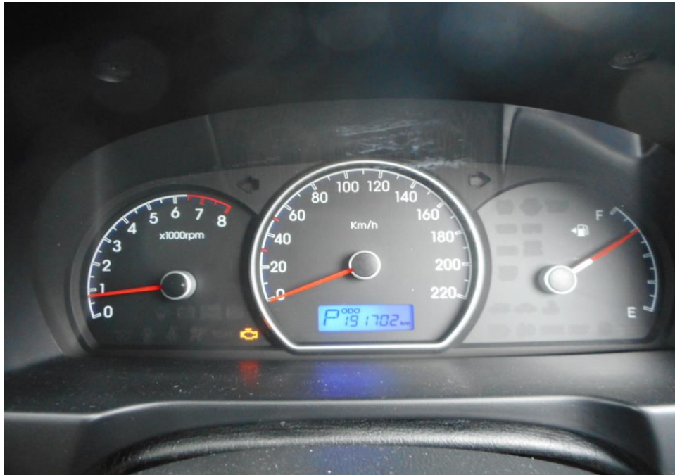
Photo 27 shows no warning lights illuminated on the instrument panel of the Motor Car after the engine was cranked. This would suggest that there was no abnormality to the various electronic operating systems of the Motor Car, like the ABS, SRS and EPS.
