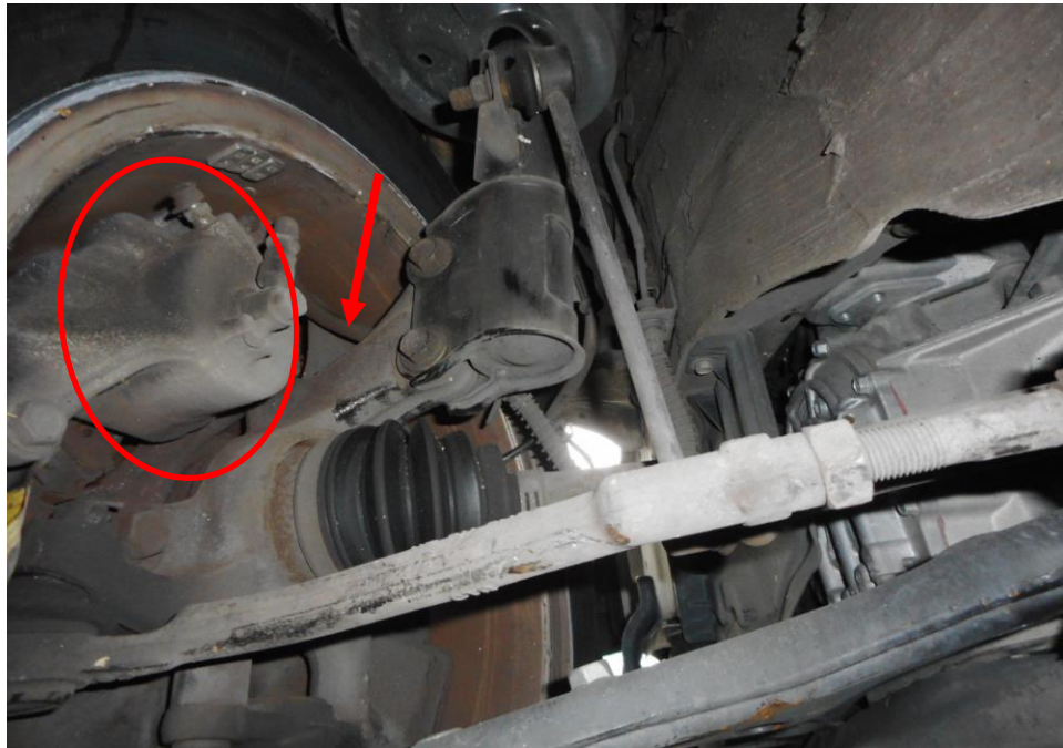
Photo 22 shows the brake hose/pipe (arrowed) at the front left wheel of the Motor Car. No leakage of brake fluid was observed. Visual examination of the various components of the braking system like the brake caliper (circled), brake booster, brake pedal etc had revealed all to be intact and without visible damage.
