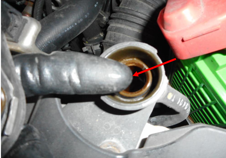
Photo 15 shows checks being carried out to the engine coolant of the Motor Car at the time of my inspection. The engine coolant was observed to be of insufficient level (arrowed).
