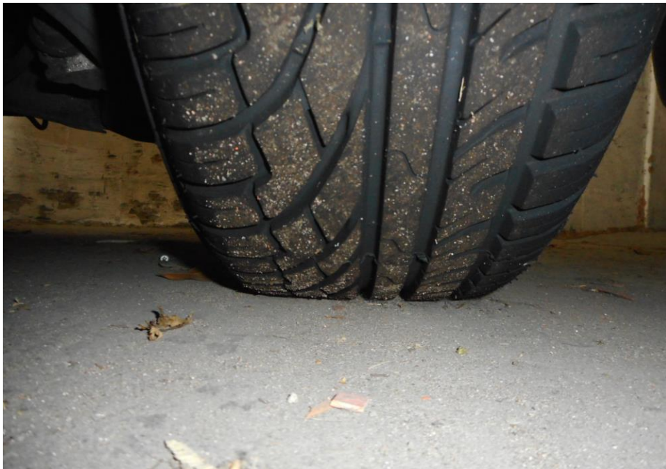
Photo 11 shows the condition of the rear left tyre of the Motor Car, which was observed to be in serviceable condition with remaining tread depth of approximately 7.2mm. The tyre, which was wrapped around steel wheel rim, was also observed to be sufficiently inflated for vehicular operation. The 4 tyres of the Motor Car were wrapped around standard steel wheel rims.
