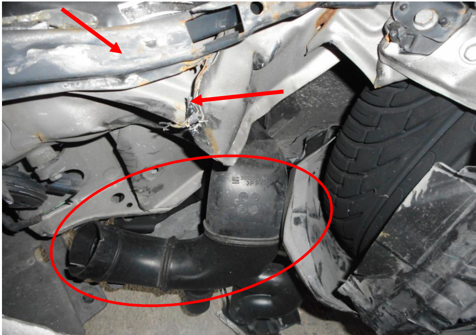
Photo 5 shows the close up view of the Motor Car's engine compartment body at the time of my inspection. The air filter box (circled) and body panels (arrowed) was observed to have sustained damage as a result of the accident.
