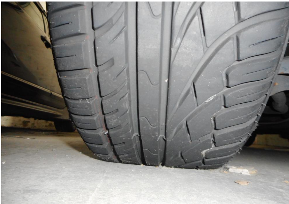
Photo 9 shows the condition of the front right tyre of the Motor Car, which was observed to be in serviceable condition with remaining tread depth of approximately 7.2mm. The tyre was sufficiently inflated for vehicular operation with no tear, cut or burst mark(s) on the outer and the inner sidewalls as well as across the tread. The 4 tyres of the Motor Car were wrapped around standard steel wheel rims without any damage.
