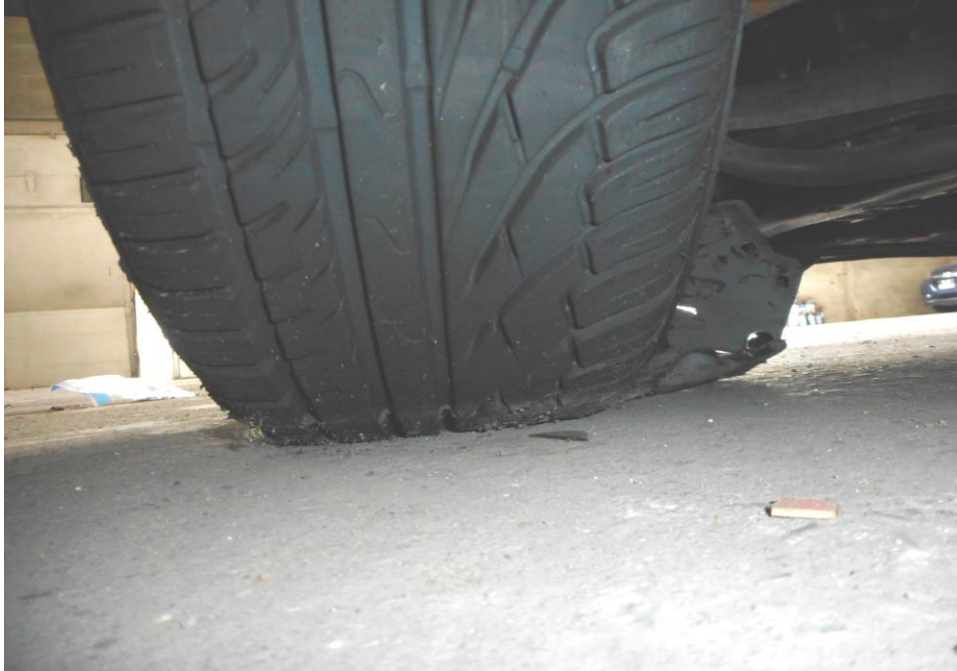
Photo 12 shows the condition of the front left tyre of the Motor Car, which was observed to be in serviceable condition with remaining tread depth of approximately 7.3mm. There was also no tear, cut or burst mark(s) on the outer and the inner sidewalls as well as across the tread of the Motor Car's 4 tyres.
