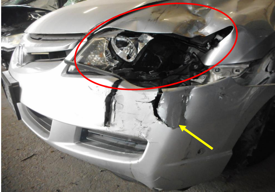
Photo 4 shows the close up view of the Motor Car's front body at the time of my inspection. The Motor Car was observed to have sustained damage at its front left headlamp (circled) and front bumper (arrowed), as a result of the accident.
