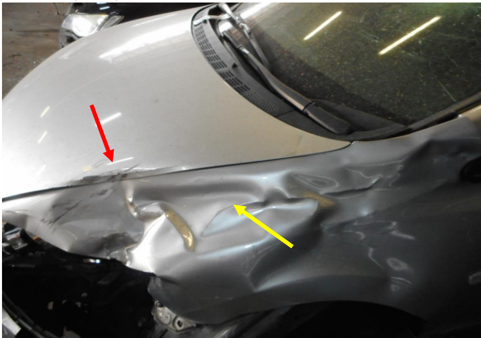
Photo 3 shows the close up view of the Motor Car's front body at the time of my inspection. The Motor Car was observed to have sustained damage at its front bonnet (red arrow) and front left fender (yellow arrow) as a result of the accident.
