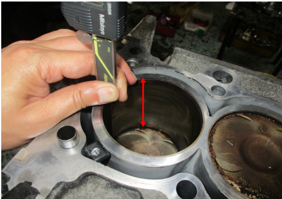
Photo 8 shows measurement being carried out to the stroke (arrowed) of cylinder 1 of the Honda engine. The bore and stroke measurements of the Honda engine were carried out using a digital Vernier Caliper that was calibrated before the start of the measurements.
