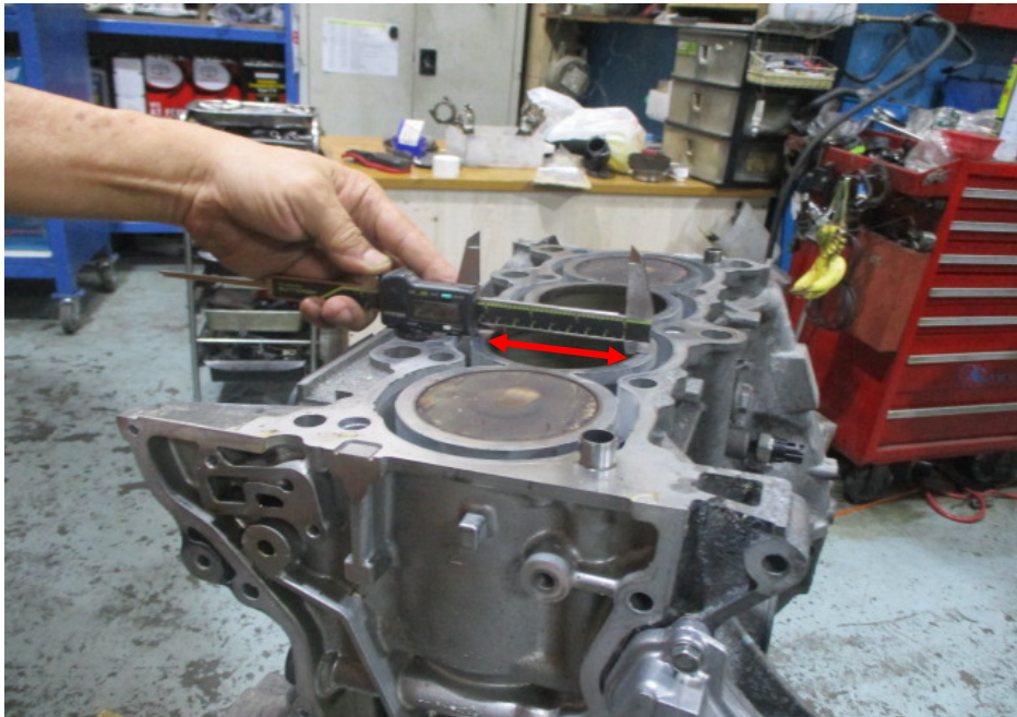
Photo 10 shows measurement being carried out to the bore (arrowed) of cylinder 2 of the Honda engine. The bore and stroke measurements of the Honda engine were carried out using a digital Vernier Caliper that was calibrated before the start of the measurements.
