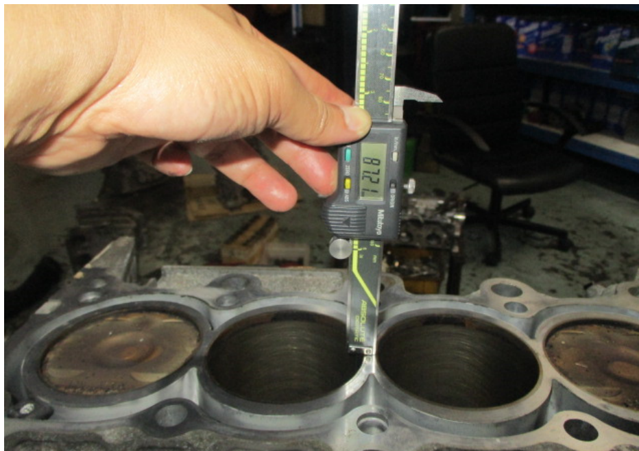
Photo 12 shows measurement of the stroke for cylinder 2 of the Honda engine that I had inspected. The bore and stroke measurements of the Honda engine were carried out using a digital Vernier Caliper that was calibrated before the start of the measurements. the stroke measurement of cylinder 2 was recorded to be 87.21mm.
