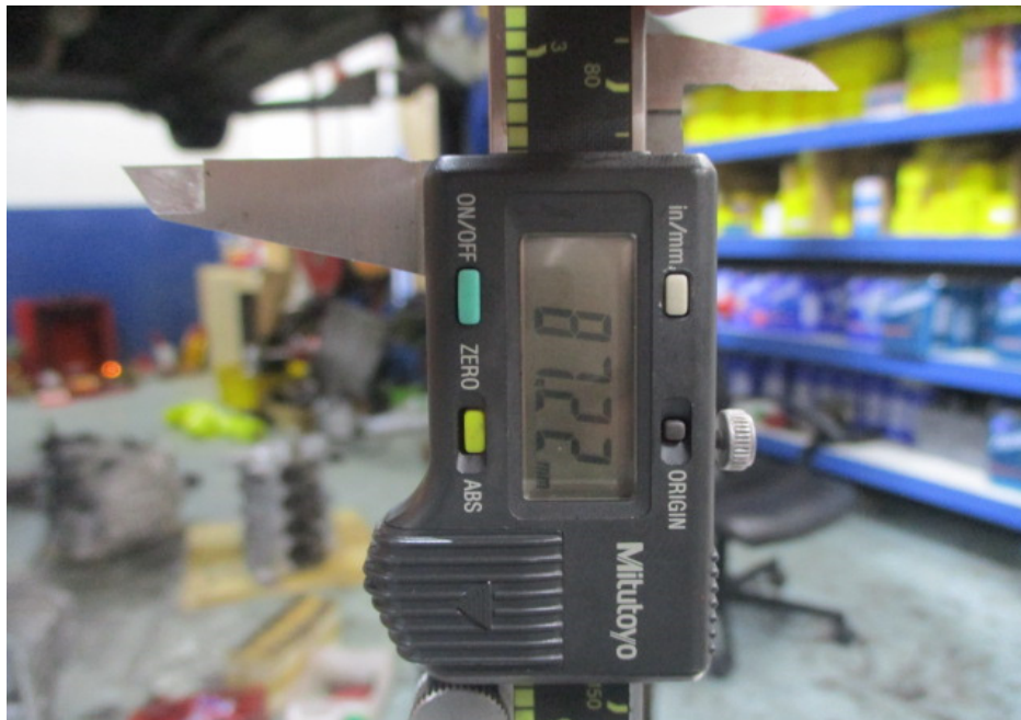
Photo 19 shows the stroke measurement of cylinder 4, which was recorded to be 87.22mm.
