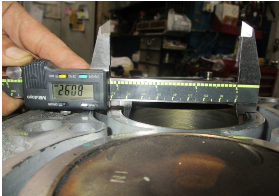
Photo 11 shows measurement being carried out to the bore of cylinder 2 of the Honda engine. The bore measurement of cylinder 2 was recorded to be 80.92mm.
