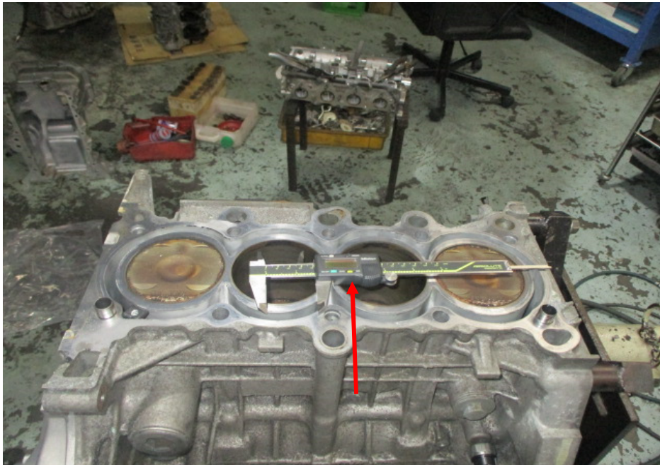
Photo 6 shows the bottom block of the Honda engine and the digital Vernier Caliper (arrowed) that was used to measure the bore and stroke measurements of each cylinder. The digital Vernier Caliper was calibrated before the start of the measurements.
