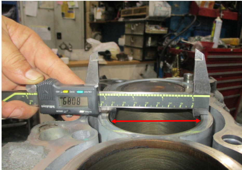
Photo 13 shows measurement being carried out to the bore (arrowed) of cylinder 3 of the Honda engine. The bore and stroke measurements of the Honda engine were carried out using a digital Vernier Caliper that was calibrated before the start of measurements. The bore measurement of cylinder 3 was recorded to be 80.89mm.
