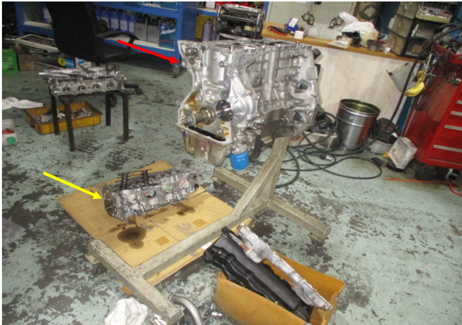
Photo 5 shows the top block (yellow arrow) of the Honda engine separated from its bottom block (red arrow). This was to enable me to carry out measurements of its cylinders, in particular the bore and stroke measurements of each cylinder, which typically can be used to determine the engine displacement or more commonly referred to as engine cc.
