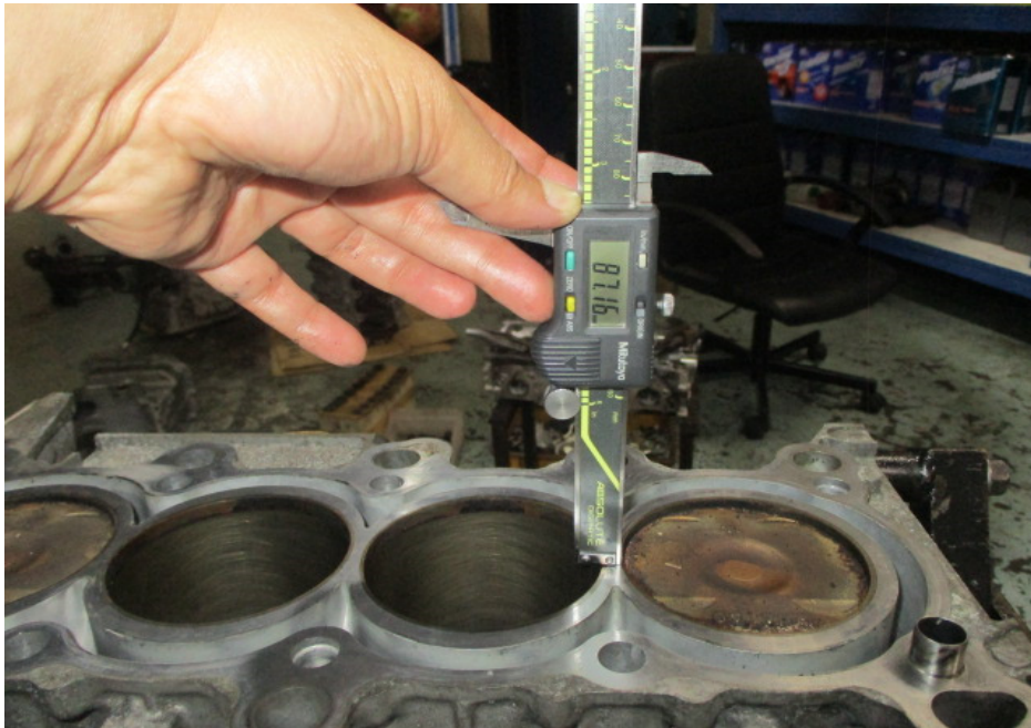
Photo 15 shows the stroke measurement of cylinder 3, which was recorded to be 87.16mm.
