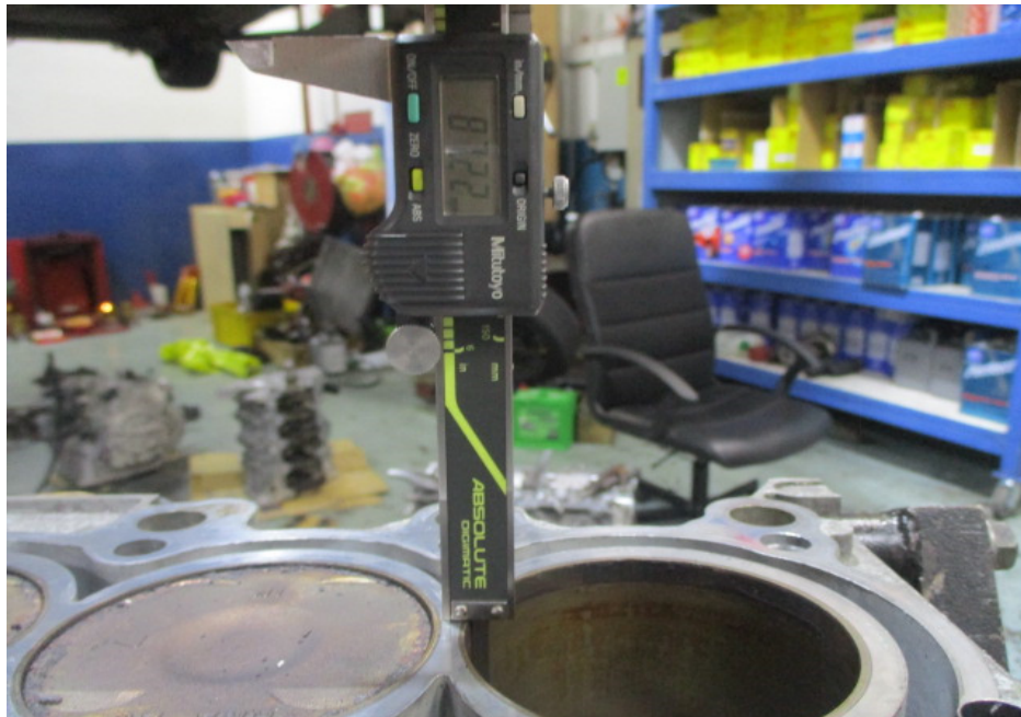
Photo 18 shows measurement being carried out to the stroke of cylinder 4 of the Honda engine. The bore and stroke measurements of the Honda engine were carried out using a digital Vernier Caliper that was calibrated prior to the start of measurements.
