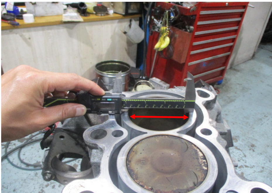
Photo 16 shows measurement being carried out to the bore (arrowed) of cylinder 4 of the Honda engine. The bore and stroke measurements of the Honda engine were carried out using a digital Vernier Caliper that was calibrated before the start of measurements.
