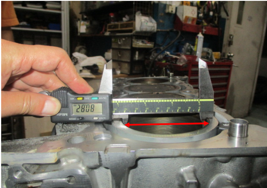
Photo 7 shows measurement being carried out to the bore (arrowed) of cylinder 1 of the Honda engine. The measurements were carried out using a digital Vernier Caliper that was calibrated before the start of the measurements. The bore measurement of cylinder 1 was recorded to be 80.82mm.
