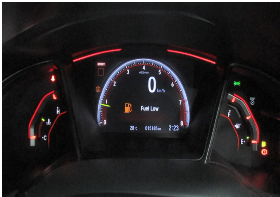
Photo 12 shows the respective warning lights no longer illuminated, indicating that there is no fault detected to the ABS, SRS, VSA, TPM and EPS systems of the Motor Car during the self-test. These electronic systems were hence in working condition at the time of my inspection.
