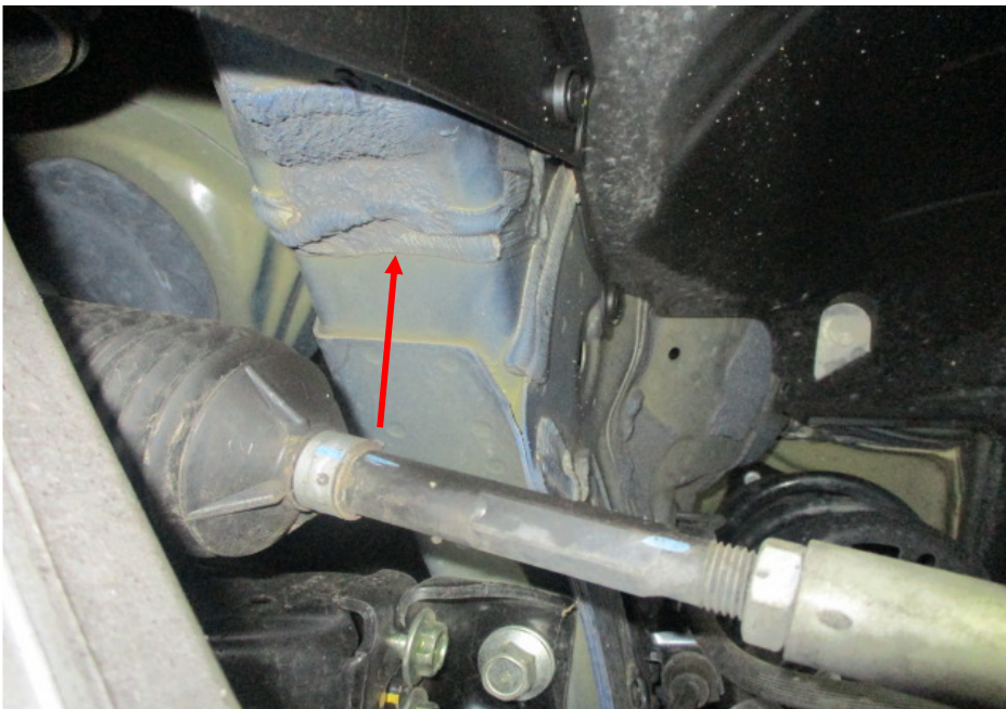
Photo 19 shows the chassis/structural body at the underside front right of the Motor Car. The original factory sealant (arrowed) at the joints along the chassis/structural body was observed to be untouched. In general, I had found no work was carried out on the chassis/structural body of the Motor Car. The chassis/structural body of the Motor Car was originally fitted.
