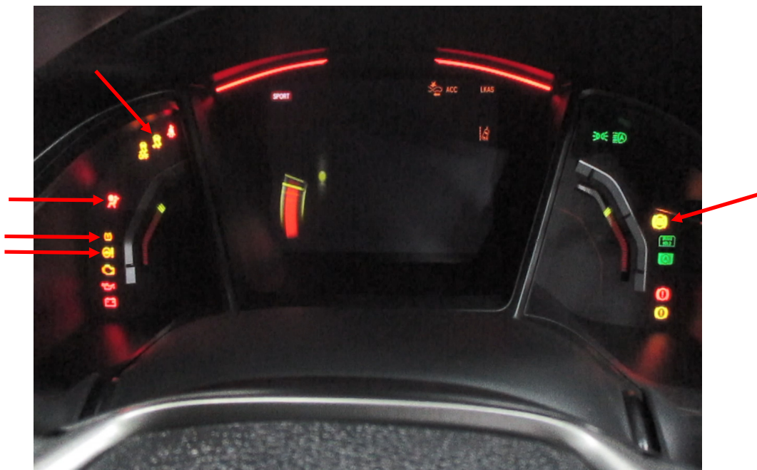
Photo 11 shows the warning lights for the various electronic safety features appearing on the instrument panel of the Motor Car during its self-test when the engine is cranked, in particular the ABS, SRS, VSA, TPM and EPS lights (arrowed).
