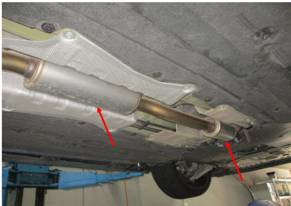
Photo 17 shows the Motor Car's centre pipe (arrowed). My examination of the Motor Car's exhaust system revealed no sign(s) or indication(s) of any cut or weld marks along its exhaust pipes and on its catalytic converter and rear mufflers.
