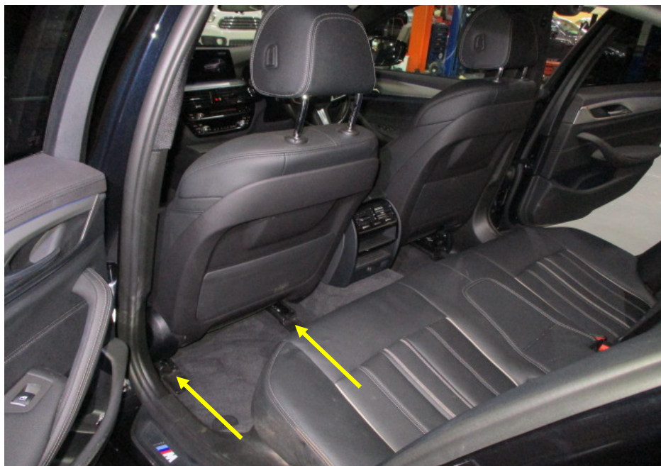
Photo 11 shows the seats of the Motor Car, which were secured via seat rails (arrowed) to the floorboard. All the seats of the Motor Car were fitted with a retractable seat belt reel and pre-tensioner. The seat belts were tested and were able to be fastened into the respective pre-tensions that were fitted on the side of each individual seat.
