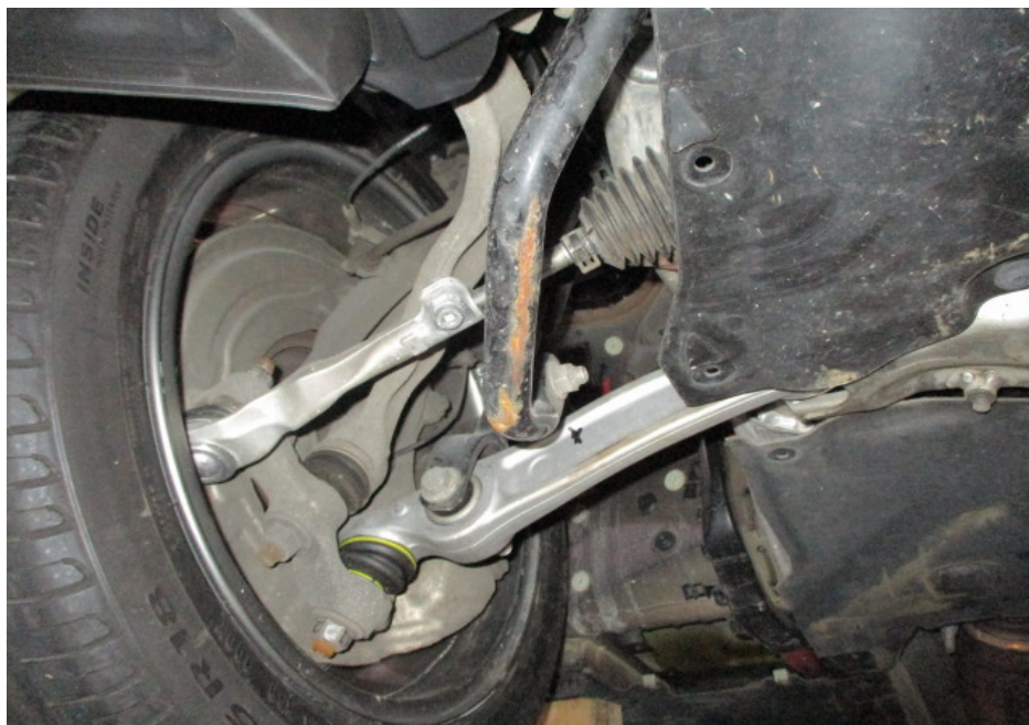
Photo 17 shows the various undercarriage components at the front right wheel of the Motor Car. The mechanical components, control arms and linkages were all found to be intact and secured in an appropriate manner. I also did not observe any fluid leak and/or fluid stain on the underside of the Motor Car.
