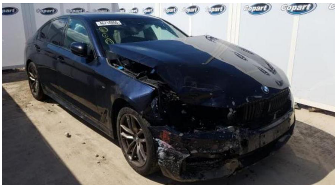
Photo 2 shows the front right body of the Motor Car (photograph provided to me). The Motor Car was observed to have sustained damage at its front right portion. The front bumper, front radiator grilles, front bonnet, front bumper right lower grille, front right headlamp and front right fender were amongst the body parts that were observed to have been damaged.
