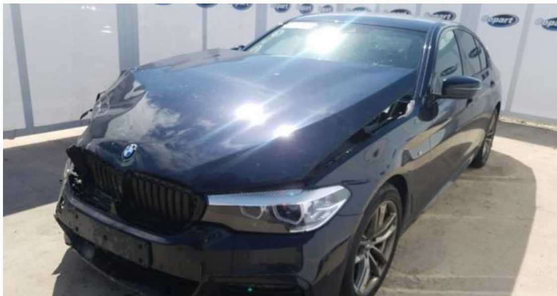
Photo 1 shows the front left body of the Motor Car (photograph provided to me). The Motor Car was observed to have sustained damage at its front right portion. The front bumper, front radiator grilles and front bonnet were amongst the body parts that were observed to have been damaged.
