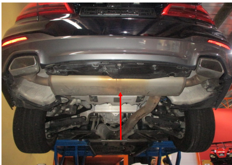
Photo 18 shows the Motor Car's rear muffler (arrowed). My examination of the Motor Car's exhaust system revealed no sign(s) or indication(s) of any cut or weld marks along its exhaust pipes and on its catalytic converter.
