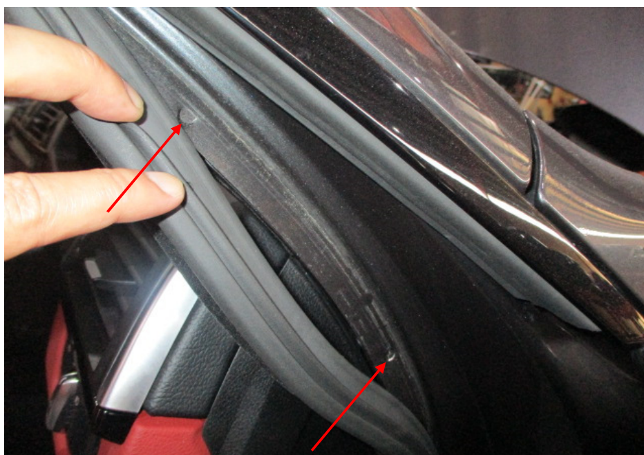
Photo 22 shows the right side "A" pillar of the Motor Car. I did not find any weld marks other than original spot weld marks (arrowed) on the right side "A" pillar of the Motor Car which, indicates that there was no re-welding works carried out. In general, I had found all the non-detachable body panels of the Motor Car to be originally fitted at the time of my inspection.
