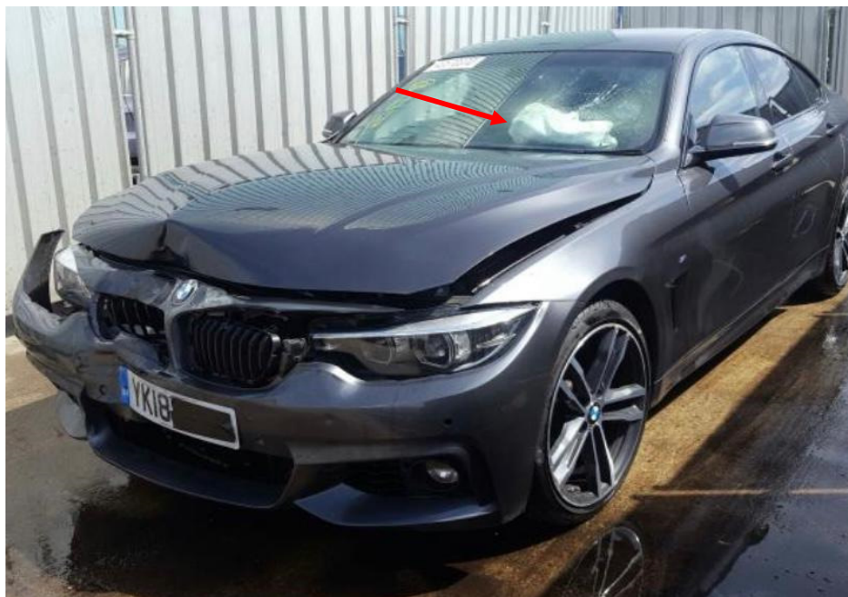
Photo 1 shows the front left body of the Motor Car (photograph provided to me). The Motor Car was observed to have sustained damage at its frontal portion. The front bumper, front grilles, front bonnet and front windscreen were amongst the body parts that were observed to have been damaged. The front left passenger airbag (arrowed) was also observed to be deployed.
