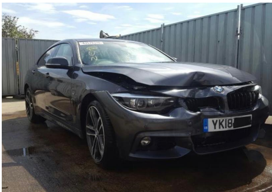
Photo 2 shows the front right body of the Motor Car (photograph provided to me). The Motor Car was observed to have sustained damage at its frontal portion. The front bumper, front grilles, front bonnet, front bumper lower grille, front right headlamp and front right fender were amongst the body parts that were observed to have been damaged.
