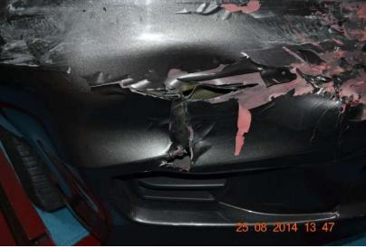
9/36: Front bumper cracked/deformed
