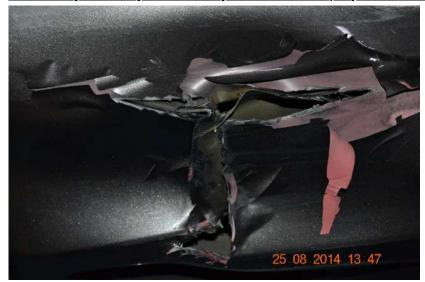
10/36: Front reinforcement bent
