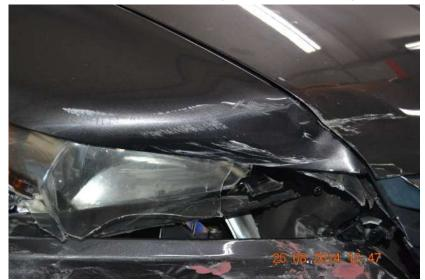
7/36: Front fender, headlamp bent/cracked
