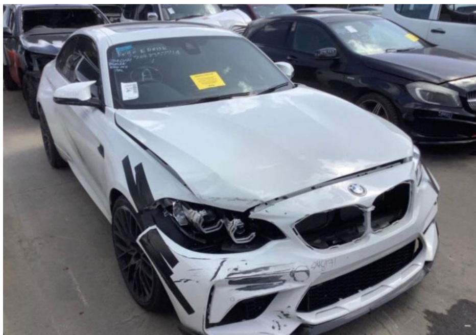
Photo 2 shows the front right body of the Motor Car prior to any repairs being carried out (photograph provided to me). The Motor Car was observed to have sustained damages at its front right portion. Amongst others, I had observed damage to the Motor Car's front bumper, front right headlamp, front bonnet, front right lower grille and front right fender.
