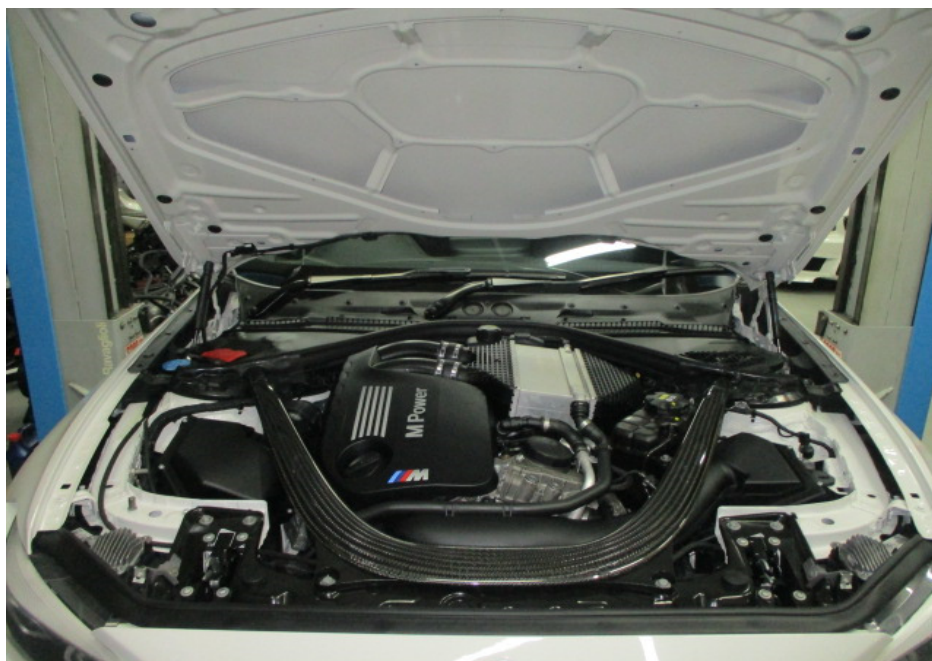
Photo 10 shows a general view of the engine compartment of the Motor Car at the time of my inspection. The various parts and components inside the engine compartment were all observed to be intact and properly fitted. There was also no sign(s) or indication(s) of fluid leak and/or fluid stain found within the engine compartment.
