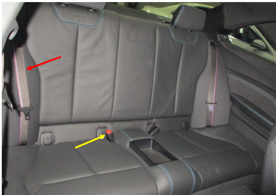
Photo 11 shows the rear seats of the Motor Car. All the seats of the Motor Car were secured via seat rails to the floorboard. They were also fitted with a retractable seat belt reel (red arrow) and a pre-tensioner (yellow arrow). The seat belts were tested and were able to be fastened securely to the respective pretension that was fitted on the side of each individual seat.
