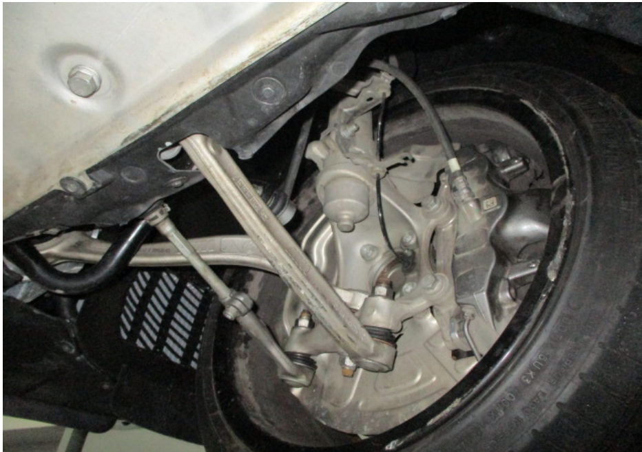
Photo 17 shows the various undercarriage components at the front right wheel of the Motor Car. The mechanical components, control arms and linkages were all found to be intact and secured in an appropriate manner. All of the Motor Car's undercarriage components were observed to be intact and secured in an appropriate manner.
