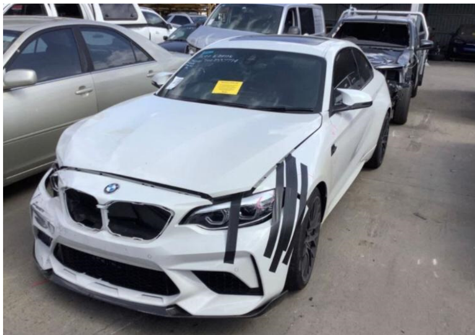
Photo 1 shows the front left body of the Motor Car prior to any repairs being carried out (photograph provided to me). The Motor Car was observed to have sustained damages at its front right portion. The body parts observed to be damaged had include the front bumper, front radiator grilles and front centre lower grille amongst others.
