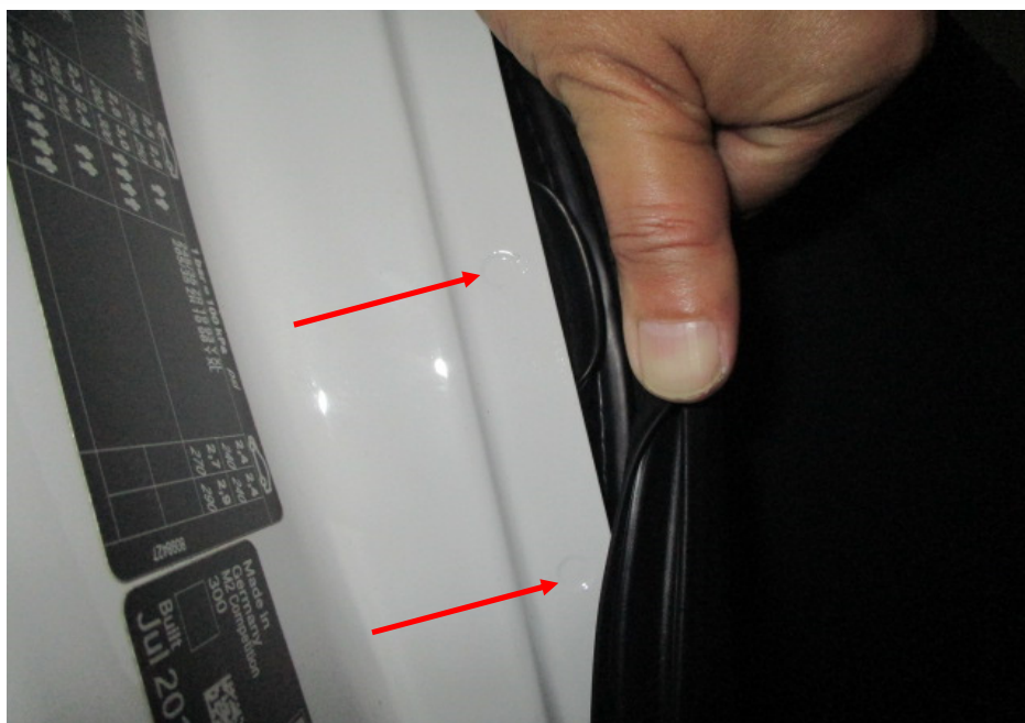
Photo 21 shows the rear right body panel of the Motor Car. I did not find any weld marks other than original spot weld marks (arrowed) on the rear right body panel of the Motor Car. In general, I had found all the non-detachable body panels of the Motor Car to be originally fitted at the time of my inspection.
