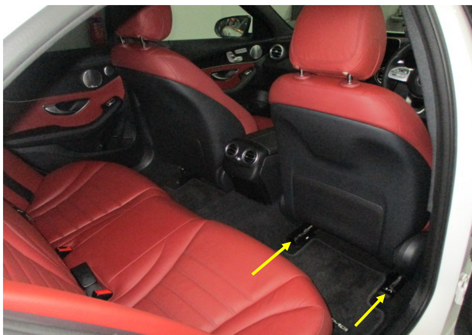
Photo 10 shows the interior compartment of the Motor Car. The seats of the Motor Car were secured via seat rails (arrowed) to the floorboard. All the seats of the Motor Car were fitted with a retractable seat belt reel and a pre-tensioner. The seat belts were tested and were able to be fastened into the respective pre-tensions that were fitted on the side of each individual seat.
