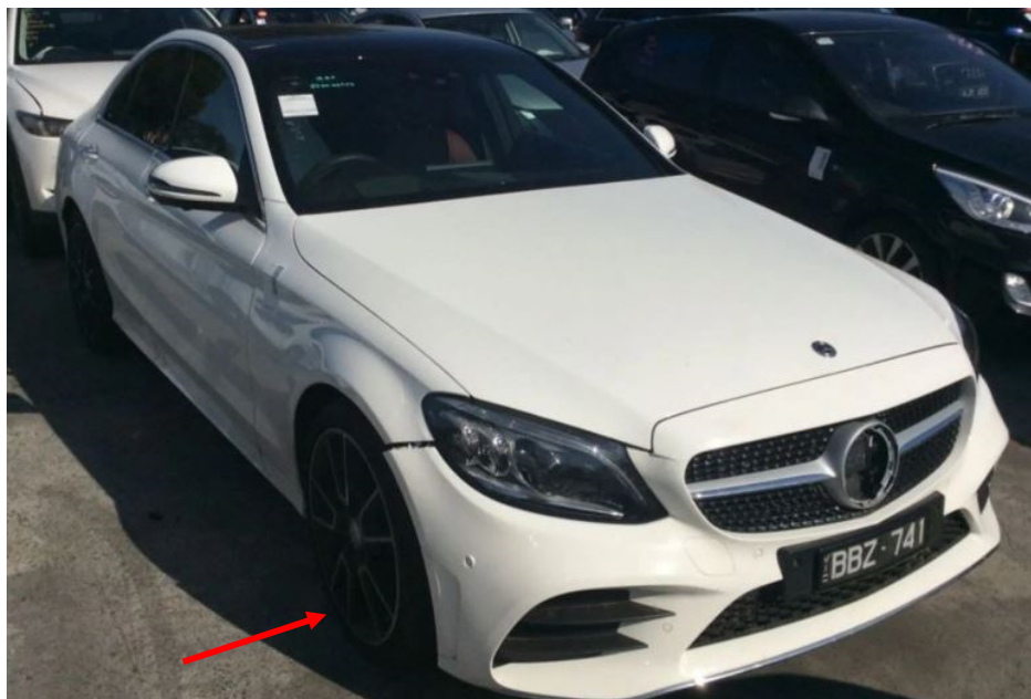
Photo 1 shows the front right body of the Motor Car prior to any repairs being carried out (photograph provided to me). The Motor Car was observed to have sustained damages at its frontal portion. The body parts damaged had included its front bumper, front radiator grille and front radiator grille logo amongst others. Note that the front right wheel (arrowed) was orientated in a straight direction.
