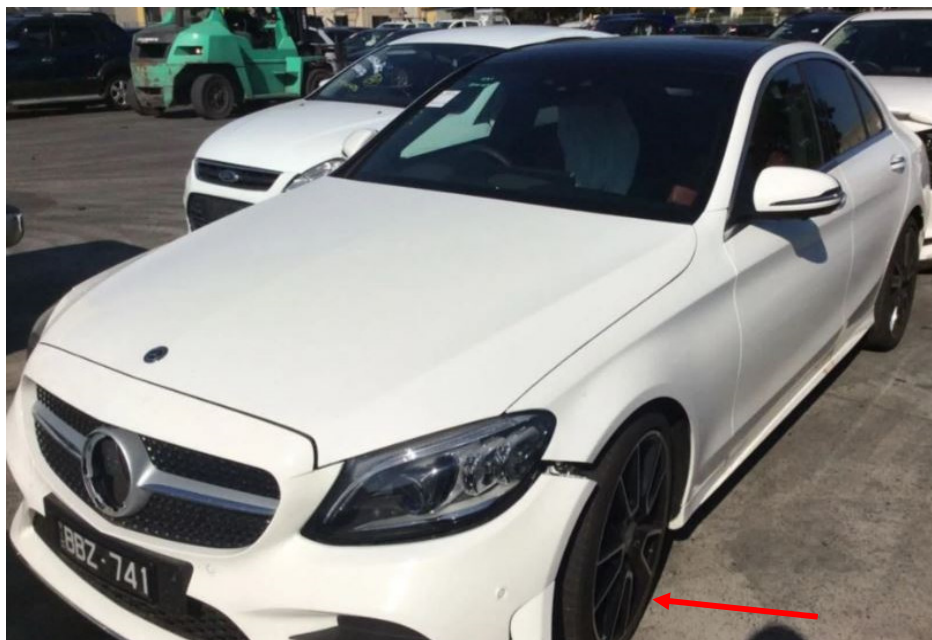
Photo 2 shows the front left body of the Motor Car prior to any repairs being carried out (photograph provided to me). Apart for the front bumper, front radiator grille and front radiator grille logo amongst others, the front left undercarriage parts of the Motor Car appear to be also affected as I had observed that the orientation of the front left wheel (arrowed) was slightly to the left direction as compared to the front right wheel which was in a straight direction (refer to photograph 1 above).
