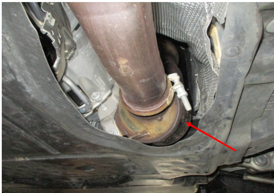
Photo 17 shows the Motor Car's catalytic convertor (arrowed). My examination of the Motor Car's exhaust system revealed no sign(s) or indication(s) of any cut or weld marks along its exhaust pipes and on its rear muffler.
