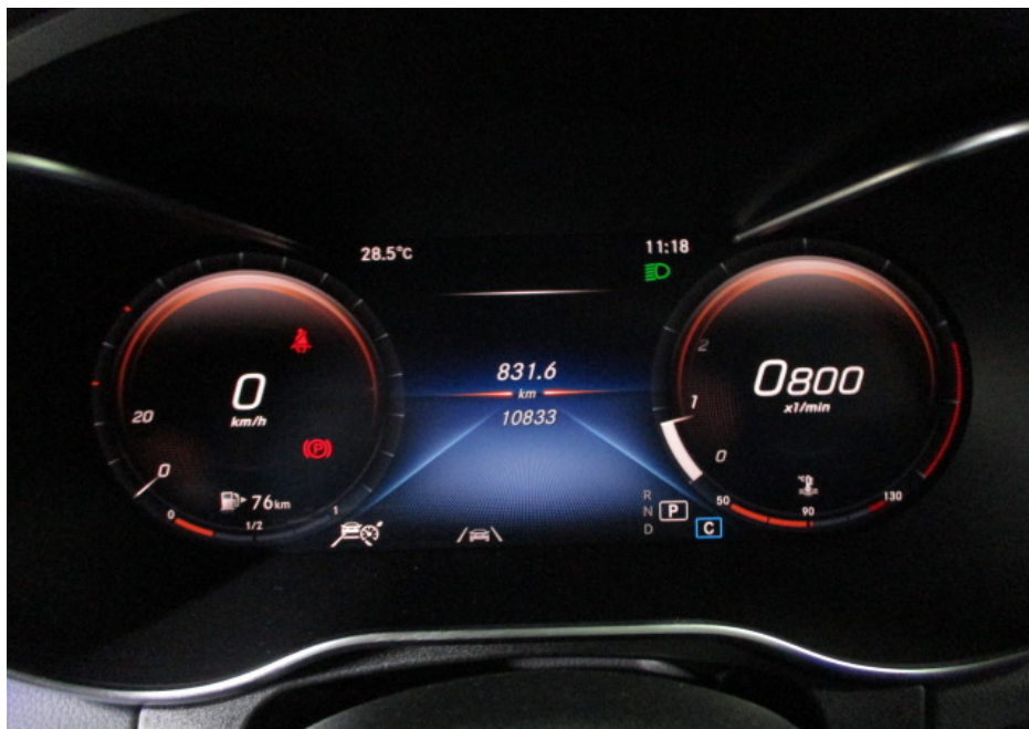
Photo 12 shows the respective warning lights no longer illuminated, indicating that there is no fault detected to the ABS, SRS, EPS, TPM and ESP systems of the Motor Car during the self-test. These electronic systems were hence in working condition at the time of my inspection.
