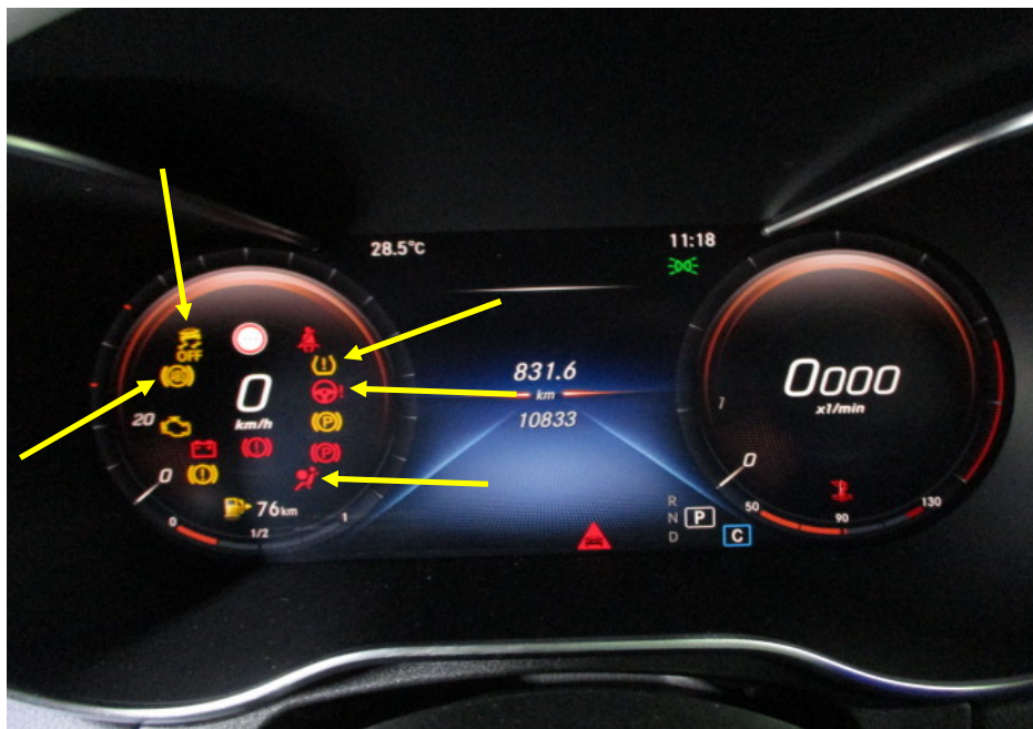
Photo 11 shows the warning lights for the various electronic safety features appearing on the instrument panel of the Motor Car during its self-test when the engine is cranked, in particular the ABS, SRS, EPS, TPM and ESP lights (arrowed).
