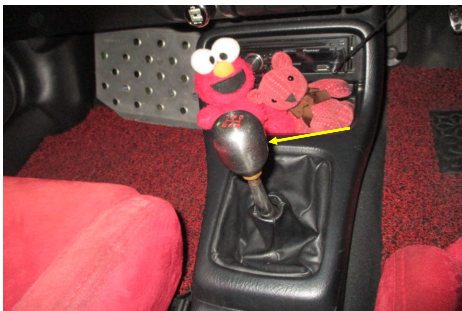
Photo 9 shows the gear shifter (arrowed) that was fitted on the Motor Car, for manually selecting the transmission gear to be engaged. The gear selector fork from the underside of the Motor Car (refer to photograph 7 above) connects to this gear shifter through the floorboard.
