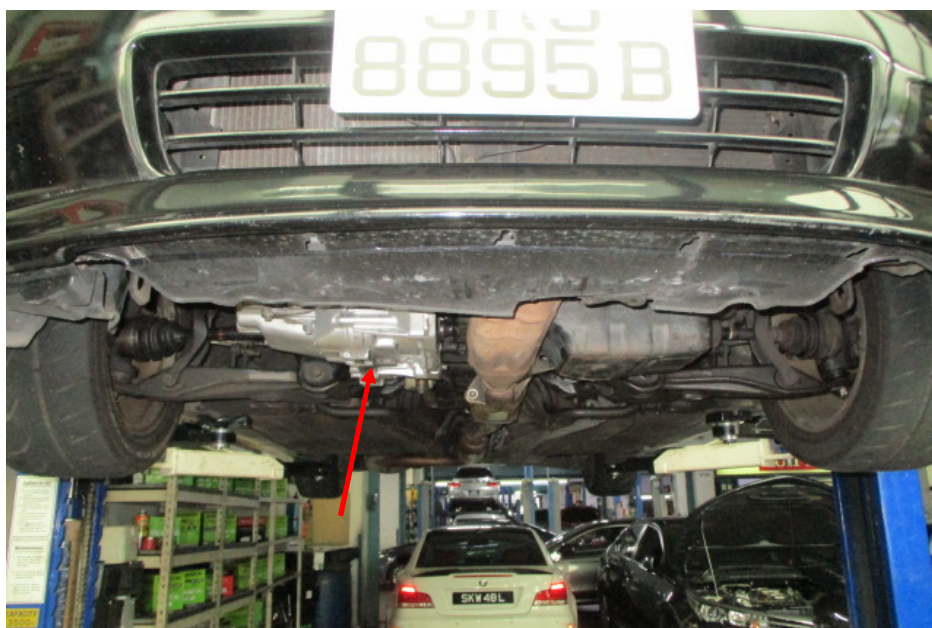
Photo 2 shows a general view of the transmission assembly (arrowed) that was fitted on the Motor Car. The input side of the transmission is bolted to the crankshaft side of the engine block. The left and right drive shafts were observed to be securely fitted from the main shaft, located inside the transmission, to the front left wheel and front right wheel respectively. There was also no crack and/or hole observed on the transmission housing.
