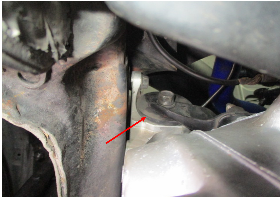
Photo 6 shows the bracket supporting the right side of the Motor Car's transmission (taken from the underside of the Motor Car). This bracket was mounted onto the right side front chassis, adjacent to the right side front wheel house. The bracket was with rubber bushings (arrowed) that absorbs any vibrations arising from the rotation of the transmission gears, minimising any stress to the bracket and correspondingly also minimise any stress to the right side front chassis member.
