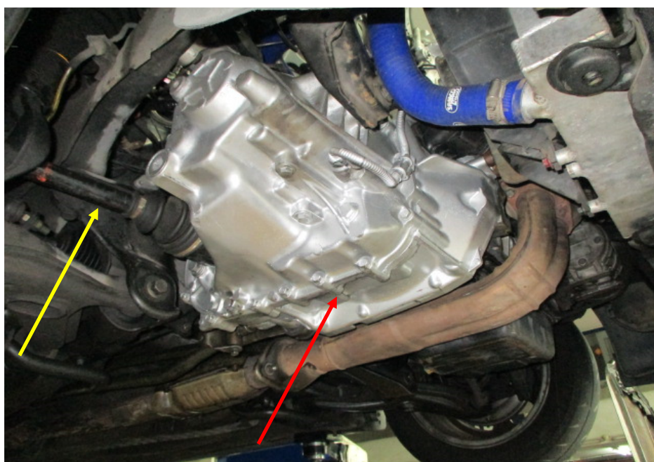
Photo 3 shows a general view of the transmission assembly (red arrow) that was fitted on the Motor Car. There was also no crack and/or hole observed on the transmission housing. The left and right drive shafts were observed to be securely fitted from the main shaft, located inside the transmission, to the front left wheel and front right wheel respectively. The right drive shaft is highlighted by the yellow arrow.
