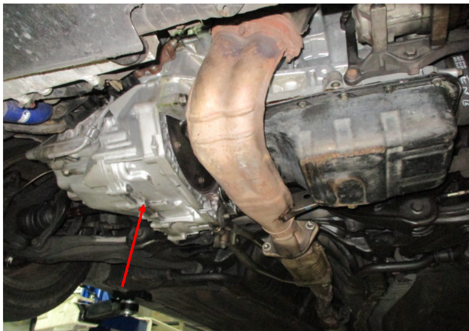
Photo 4 shows another view of the transmission assembly (arrowed) that was fitted on the Motor Car. This was at the input side where the transmission is bolted onto the crankshaft side of the engine block.
