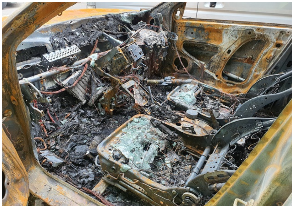
Photo 3 shows the interior compartment of the Insured Vehicle. All the parts inside the interior compartment were found to be extensively burnt. Its front seats, rear seats, roof upholstery, carpet and various trims were all burnt and/or melted, leaving charred skeletal remains.
