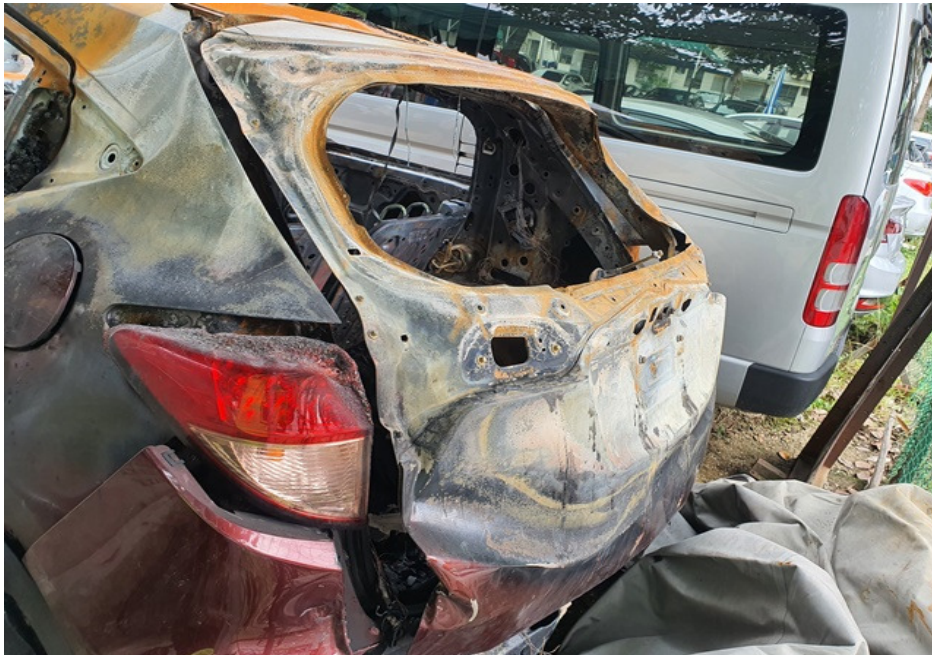
Photo 5 shows the rear body of the Insured Vehicle. Comparing the overall extent of fire damage like the rear tyres vs the front tyres, condition of rear body panels vs front body panels etc, it would appear that the front body of the Insured Vehicle was more severely affected than its rear portion.
