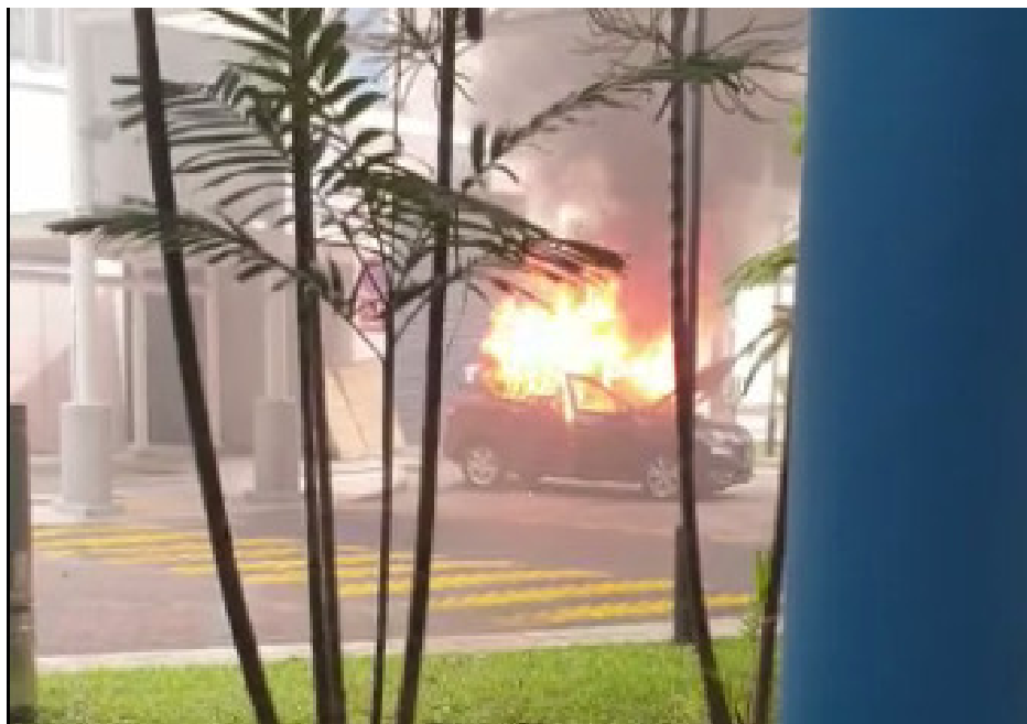
Photo 7 shows a screenshot of the right body of the Insured Vehicle on fire taken from the video recording that was provided by Mr Wong. Comparing the overall extent of fire damage like the rear tyres vs the front tyres, condition of rear body panels vs front body panels etc, it would appear that the left of the Insured Vehicle was most affected by the fire.
