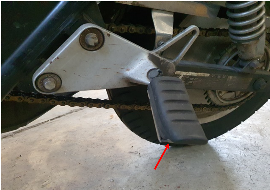
Photo 13 shows a closer view of the left pillion foot peg (arrowed) which was amongst the body parts of the Motorcycle that had sustained damage as a result of the accident.
