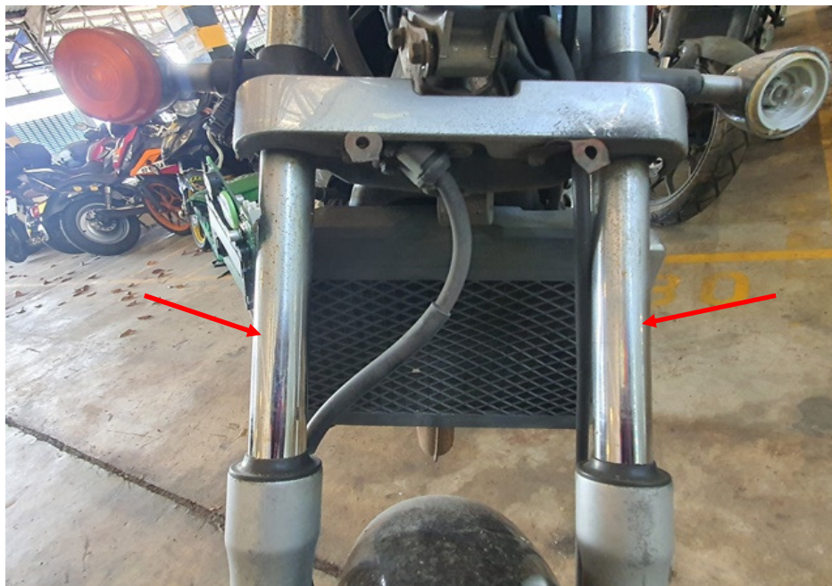
Photo 21 shows the front fork (arrowed) of the Motorcycle. The front fork and fork bracket of the Motorcycle were both found to be intact and undamaged. Turning the Motorcycle's handle bar towards the left and right did not produce any abnormal free play and/or resistance. The steering system of the Motorcycle was in serviceable condition at the time of our inspection.
