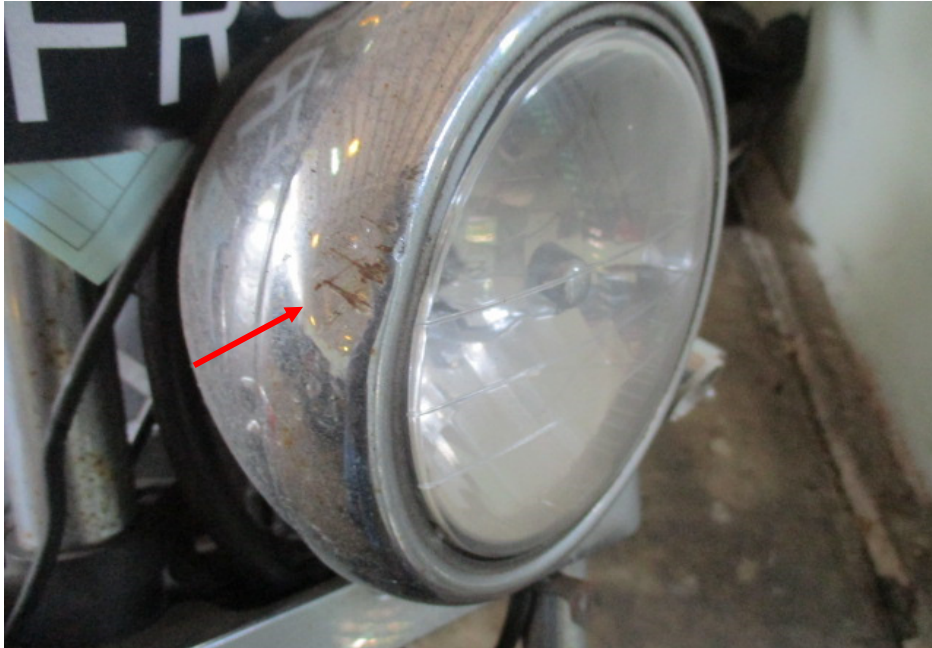
Photo 5 shows a closer view of the headlight assembly which was amongst the body parts of the Motorcycle that had sustained damages as a result of the accident (arrowed).
