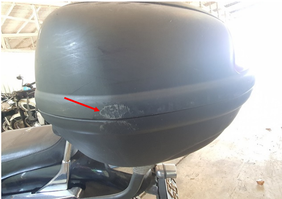
Photo 14 shows a closer view of the top box (arrowed) which was amongst the body parts of the Motorcycle that had sustained damage as a result of the accident.
