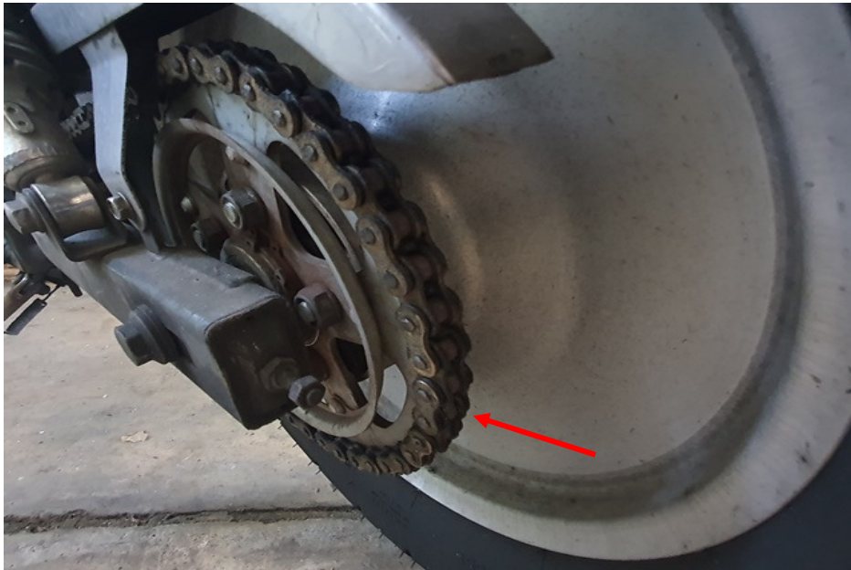
Photo 20 shows a closer view of the gear train (arrowed) of the Motorcycle, which was observed to be intact with no misalignment. It was also adequately lubricated for operating purposes.
