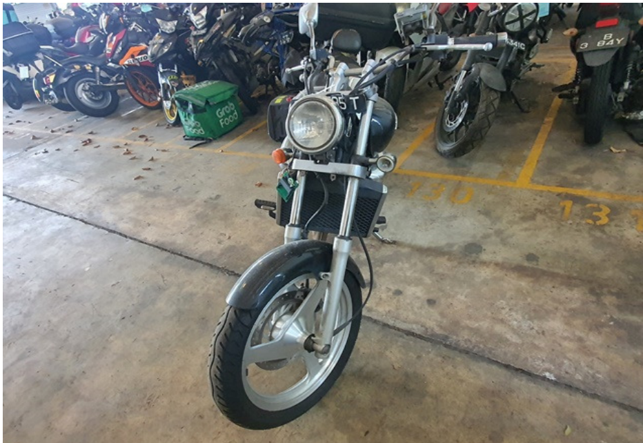
Photo 23 shows the front wheel of the Motorcycle turned towards its full right. Turning the Motorcycle's handle bar towards the left and right did not produce any abnormal free play and/or resistance. This would indicate that the steering system of the Motorcycle was in serviceable condition at the time of our inspection.
