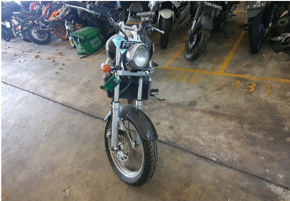
Photo 22 shows the front wheel of the Motorcycle turned towards its full left. Turning the Motorcycle's handle bar towards the left and right did not produce any abnormal free play and/or resistance. This would indicate that the steering system of the Motorcycle was in serviceable condition at the time of our inspection.
