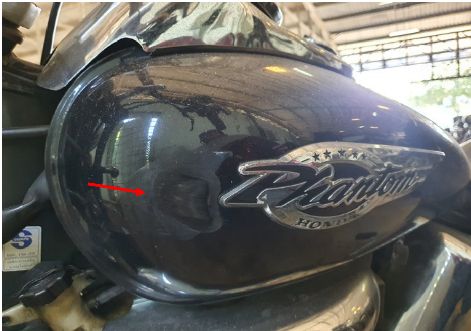
Photo 8 shows a closer view of the fuel tank of the Motorcycle that had sustained damages as a result of the accident (arrowed).
