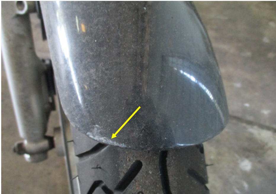
Photo 7 shows a closer view of the front mudguard which was amongst the body parts at the front body of the Motorcycle that had sustained damage as a result of the accident (arrowed).
