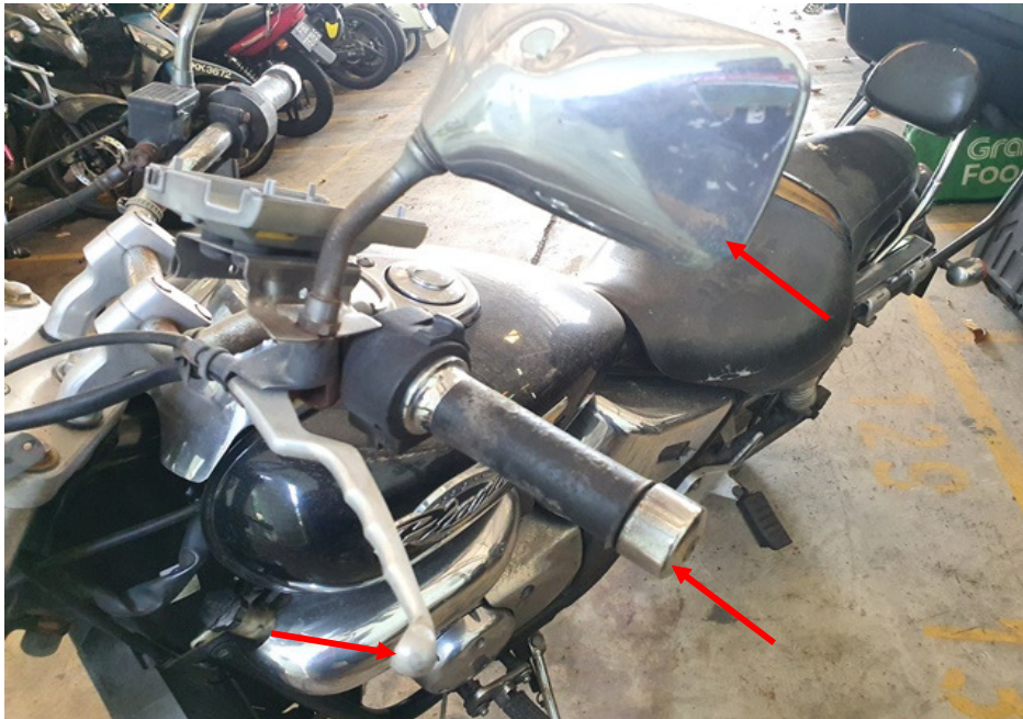
Photo 9 shows a closer view of the left handlebar end, clutch lever and left side mirror (arrowed) which were amongst the body parts of the Motorcycle that had sustained damage as a result of the accident.
