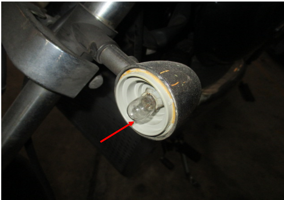
Photo 6 shows a closer view of the broken left front signal lamp of the Motorcycle as a result of the accident (arrowed).
