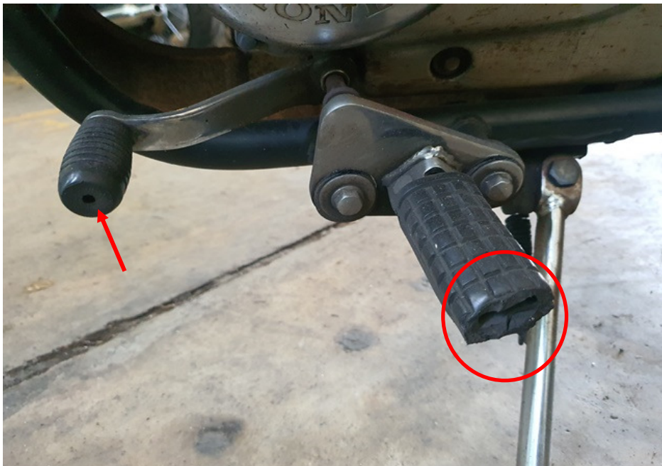
Photo 10 shows a closer view of the gear shift pedal (arrowed) and left front footrest (circled) which were amongst the body parts of the Motorcycle that had sustained damage as a result of the accident.
