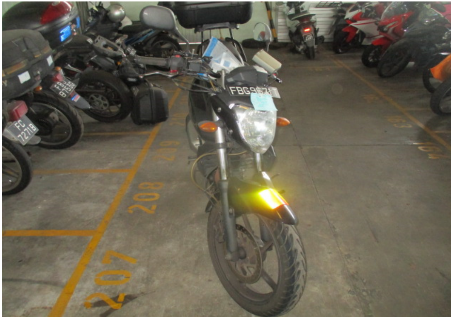
Photo 21 shows the front wheel of the Motorcycle turned towards its full left. Turning the Motorcycle's handle bar towards the left did not produce any abnormal free play and/or resistance. This would indicate that the steering system of the Motorcycle was in serviceable condition at the time of our inspection.
