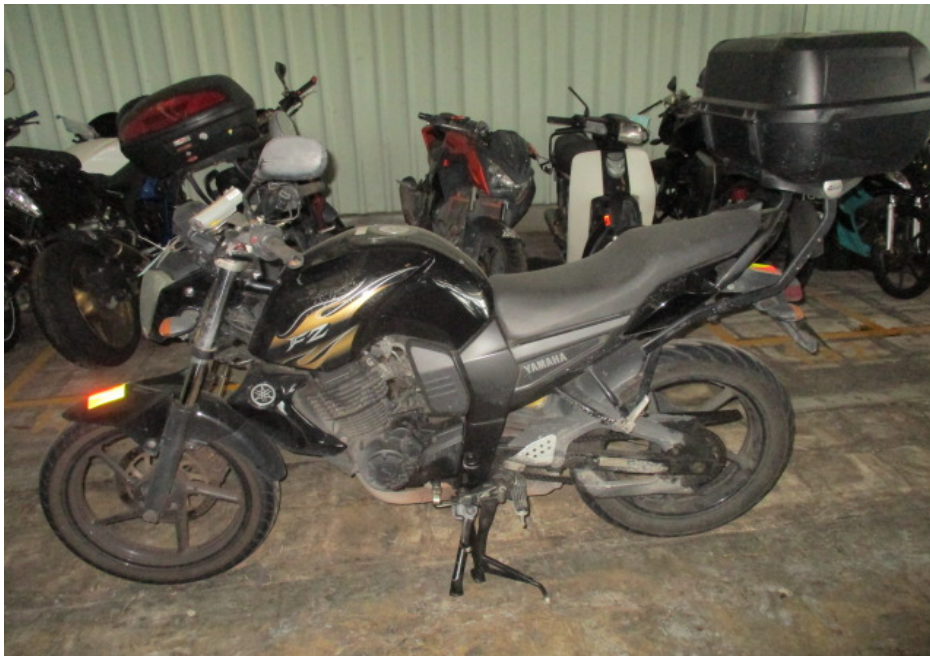
Photo 3 shows a general view of the left body of the Motorcycle at the time of our inspection. The Motorcycle was observed to have sustained damages at its frontal portion and left body. The body parts that were found to have been damaged include its IU unit, front mudguard, left front signal lamp, left side mirror, left handlebar end, clutch lever, gear shift pedal, left pillion foot peg, left radiator cover, side stand, left rear side cover and top box, amongst others.
