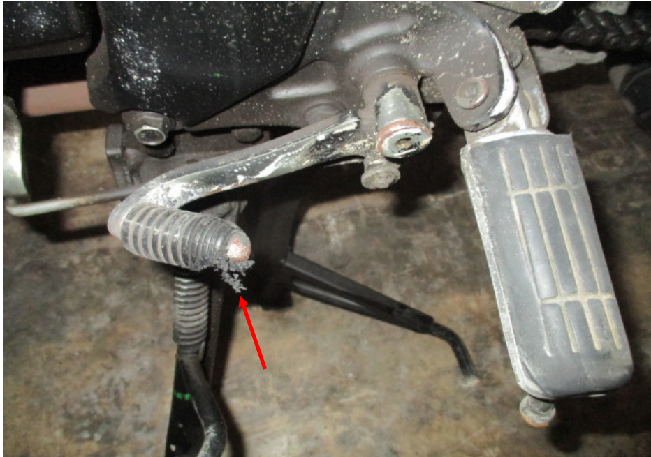
Photo 12 shows the bent gear shift pedal of the Motorcycle as a result of the accident (arrowed).
