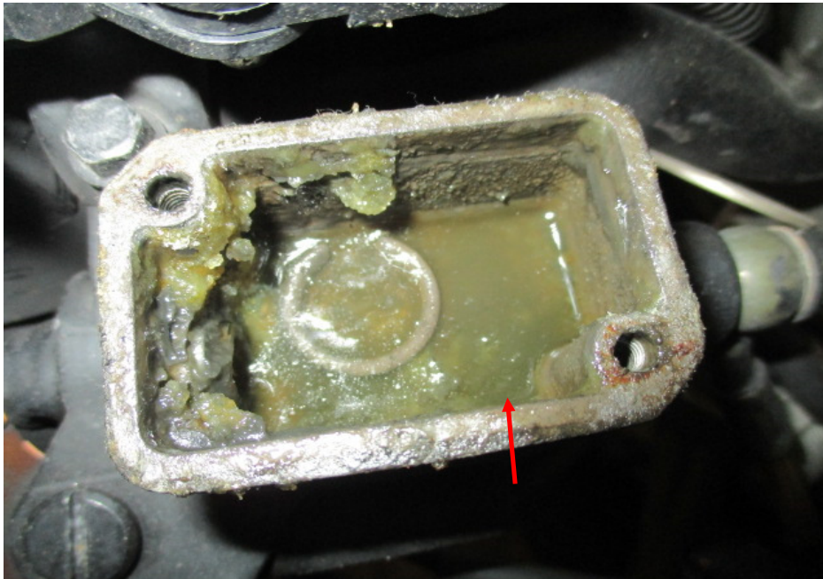
Photo 24 shows the brake fluid reservoir for the front brake of the Motorcycle. The brake fluid reservoir was found to be contaminated and of insufficient level for operating purposes (arrowed).
