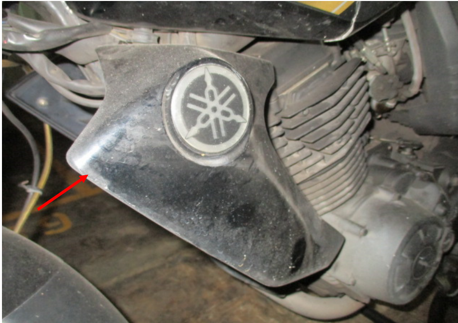
Photo 8 shows the left radiator cover (arrowed), which were amongst the body parts of the Motorcycle that had sustained damage as a result of the accident.
