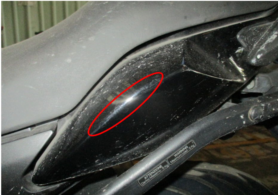
Photo 13 shows the left rear side cover of the Motorcycle that had sustained damage as a result of the accident (circled).
