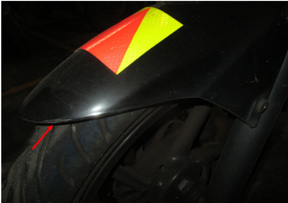
Photo 6 shows a closer view of the front mudguard (arrowed) which was amongst the body parts of the Motorcycle that had sustained damage as a result of the accident.
