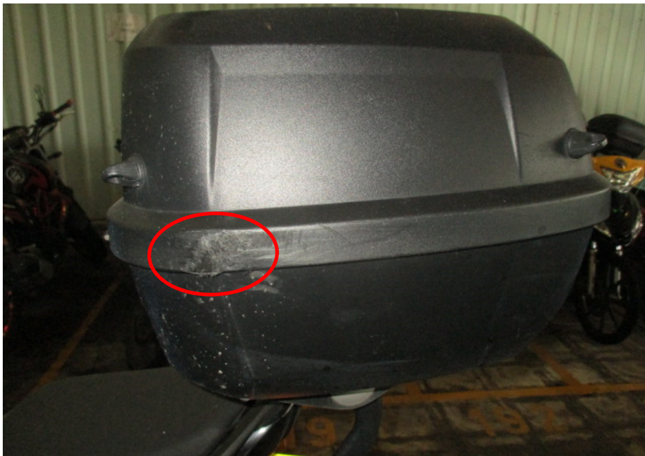
Photo 9 shows the top box which was amongst the body parts of the Motorcycle that had sustained damage as a result of the accident (circled).
