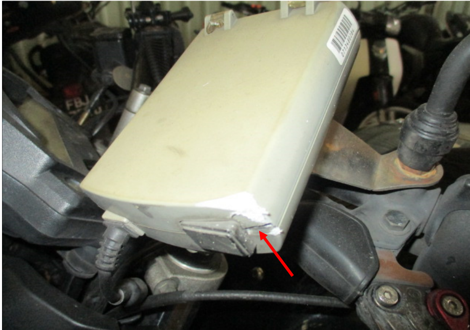
Photo 4 shows a close up view of the cracked IU unit (arrowed) of the Motorcycle as a result of the accident.
