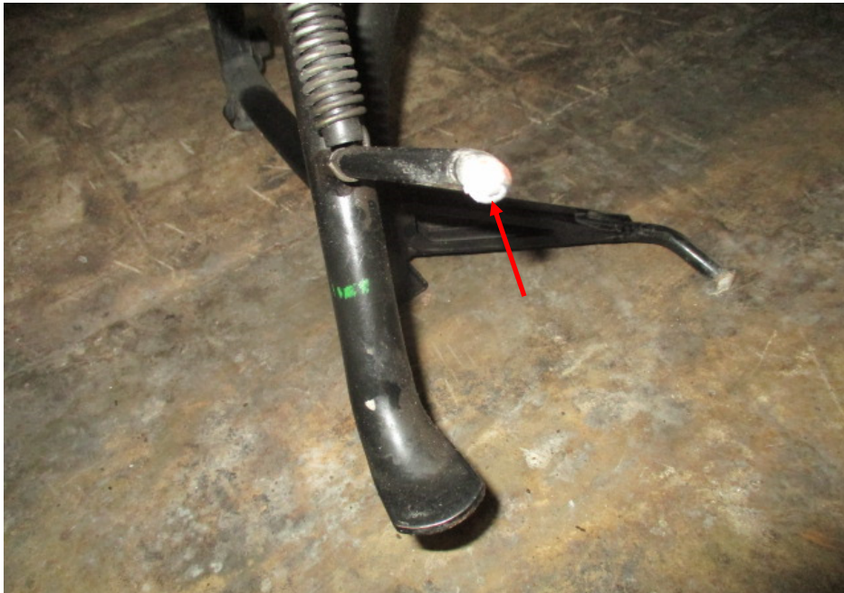
Photo 10 shows a closer view of the side stand which was amongst the body parts of the Motorcycle that had sustained damages as a result of the accident (arrowed).
