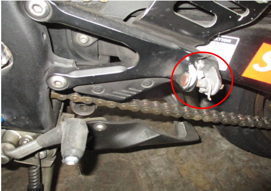
Photo 11 shows a closer view of the broken left front footrest (circled) which was amongst the body parts of the Motorcycle that had sustained damage as a result of the accident.
