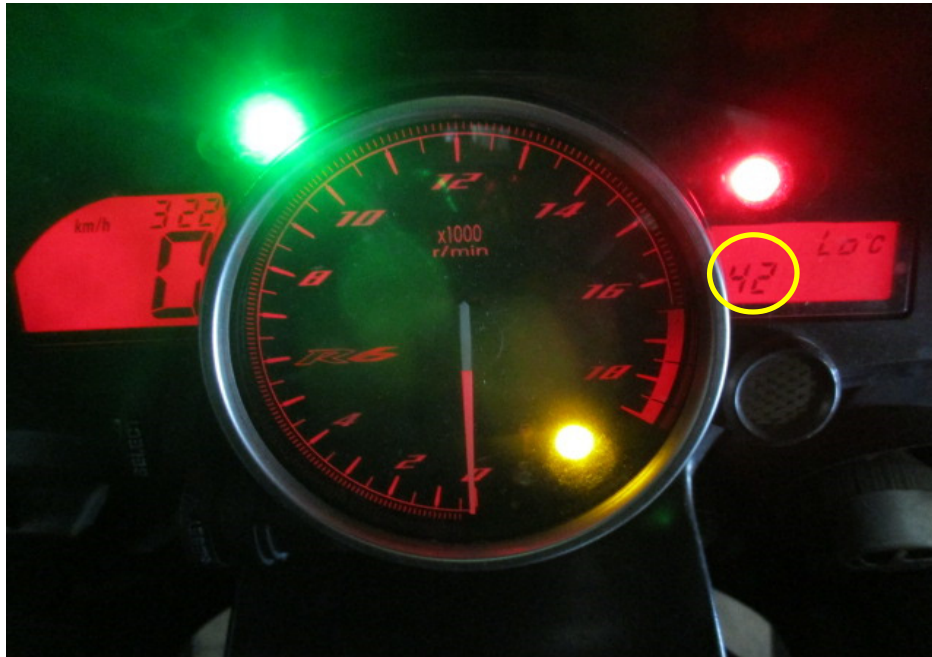
Photo 1 shows a closer view of the speedometer gauge of the Motorcycle. The mileage of the Motorcycle could not be recorded at the time of our inspection due to an error code displayed on the speedometer gauge as a result of the accident (circled).
