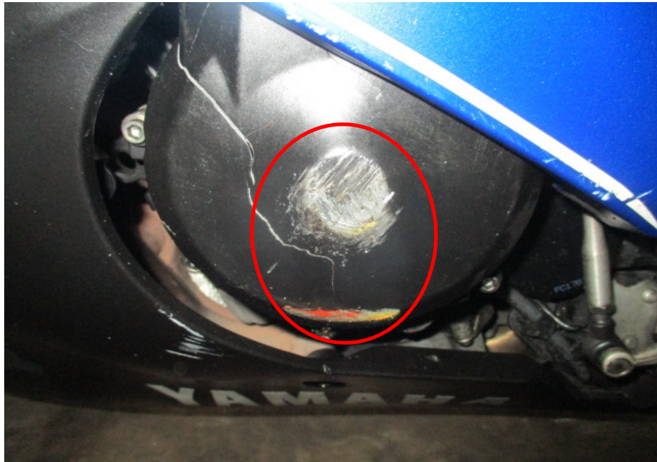
Photo 18 shows the left side of the engine of the Motorcycle at the time of our inspection. The various left engine components had sustained damage of grazing nature as a result of the accident (circled) however the engine components were still intact. There was also no fluid leak and/or fluid stain found around the left engine area of the Motorcycle.
