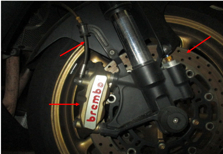
Photo 22 shows a close up view of the front brake caliper, front brake disc and front brake hose (arrowed) at the right side of the Motorcycle's front wheel, which are all part of the components in the hydraulic front brake system of the Motorcycle. Our visual checks of these various components had revealed all to be intact with no visible damage. No leakage of brake fluid was also observed.
