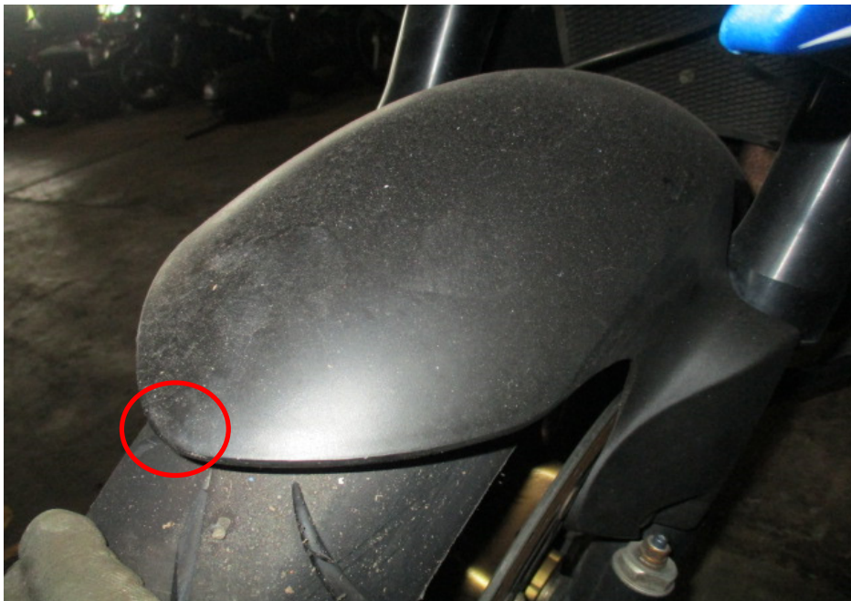
Photo 6 shows a closer view of the front mudguard, which was amongst the body parts of the Motorcycle that had sustained damage as a result of the accident (circled).
