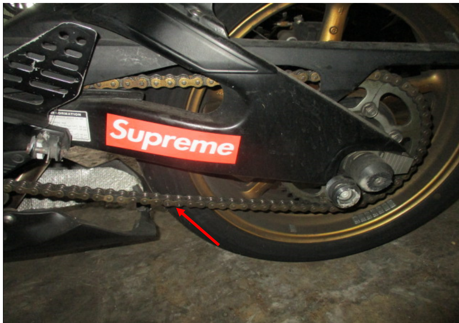
Photo 19 shows the gear chain (arrowed) of the Motorcycle, which was observed to be intact with no misalignment. It was also adequately lubricated for operating purposes. The gear chain rotates the rear wheel of the Motorcycle.
