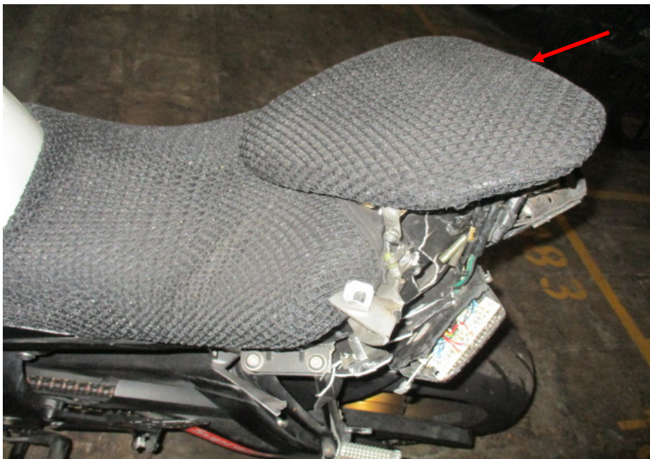
Photo 14 shows the dislodged rear seat of the Motorcycle of the Motorcycle as a result of the accident (arrowed).
