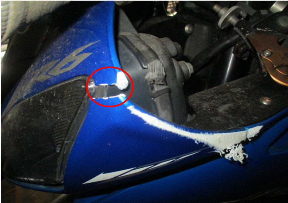
Photo 5 shows a closer view of the cracked head cowl of the Motorcycle as a result of the accident (circled).
