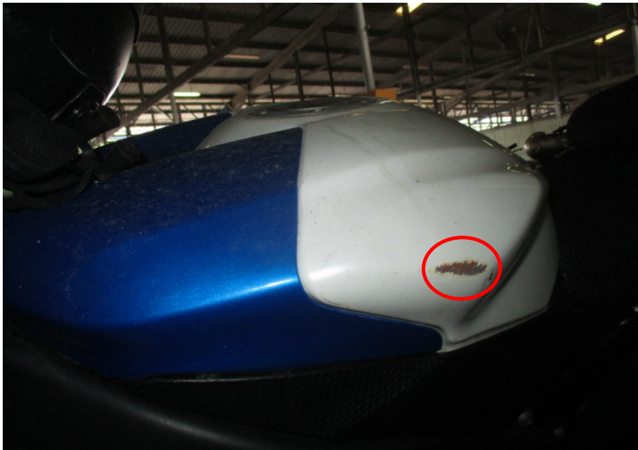
Photo 9 shows a closer view of the petrol tank, which was amongst the body parts of the Motorcycle that had sustained damage as a result of the accident (circled).
