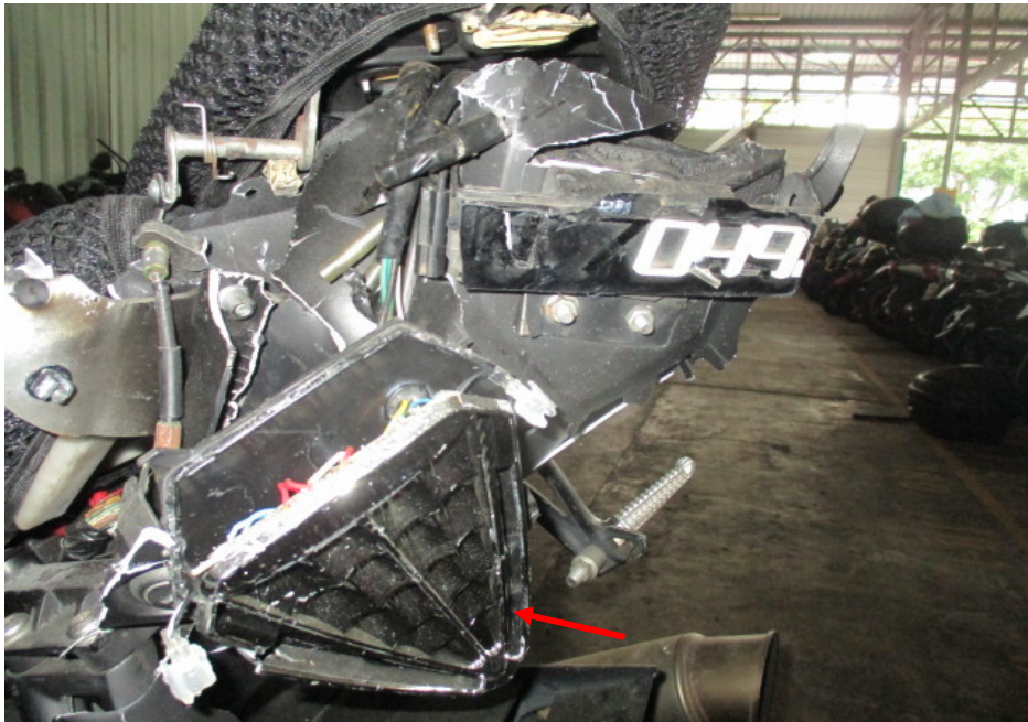
Photo 13 shows the broken tail light assembly of the Motorcycle as a result of the accident (arrowed).
