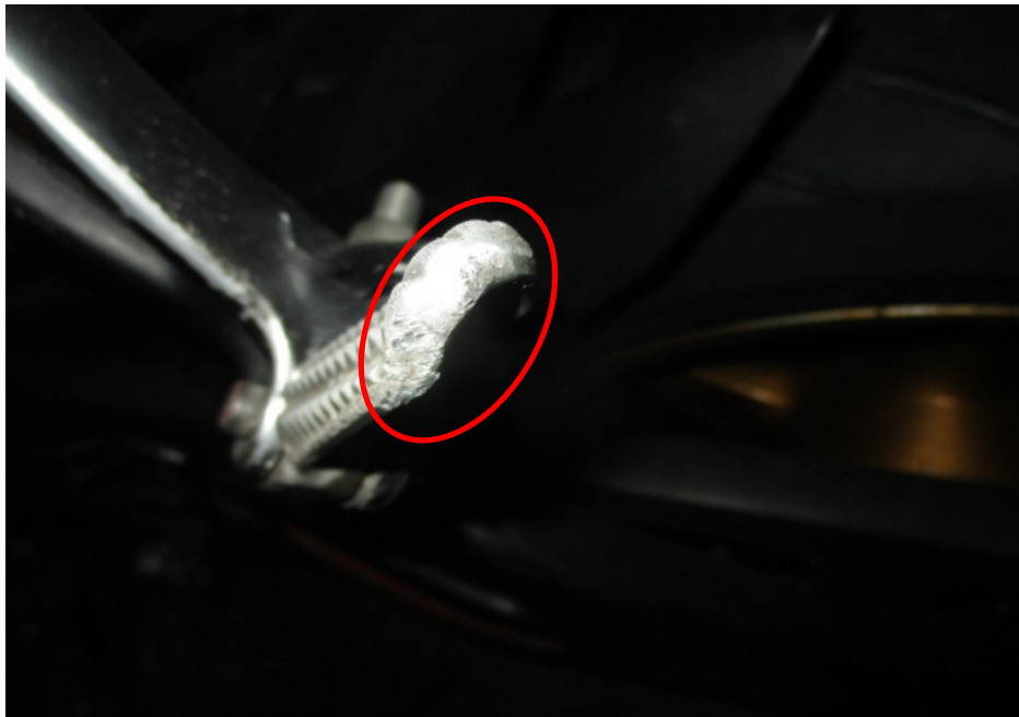
Photo 12 shows a closer view of the left pillion foot peg (circled) which was amongst the body parts of the Motorcycle that had sustained damages of grazing nature as a result of the accident.
