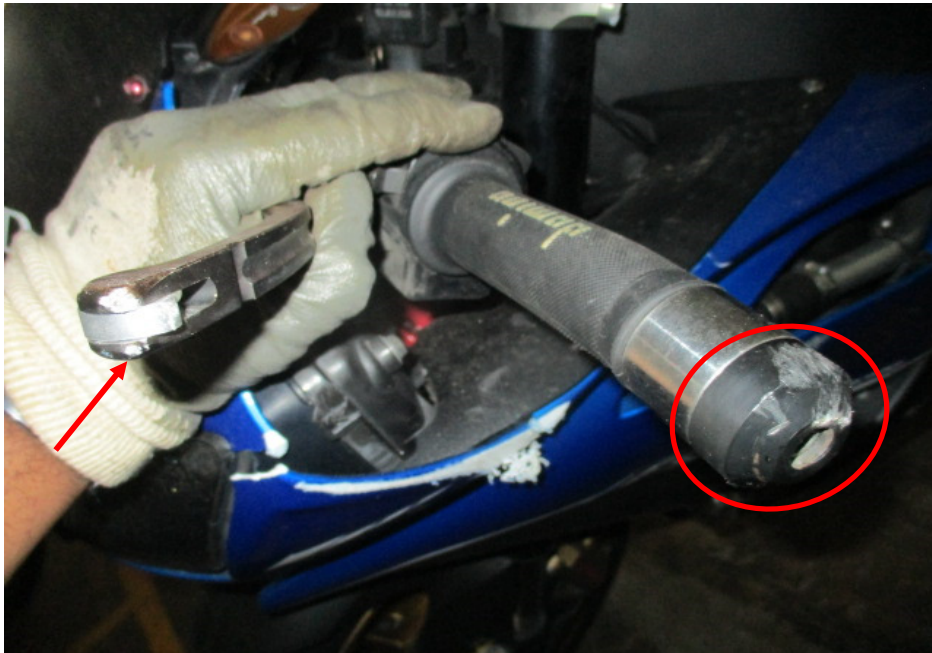
Photo 7 shows a closer view of the clutch lever (arrowed) and left handlebar end (circled) which were amongst the body parts at the front body of the Motorcycle that had sustained damage as a result of the accident.
