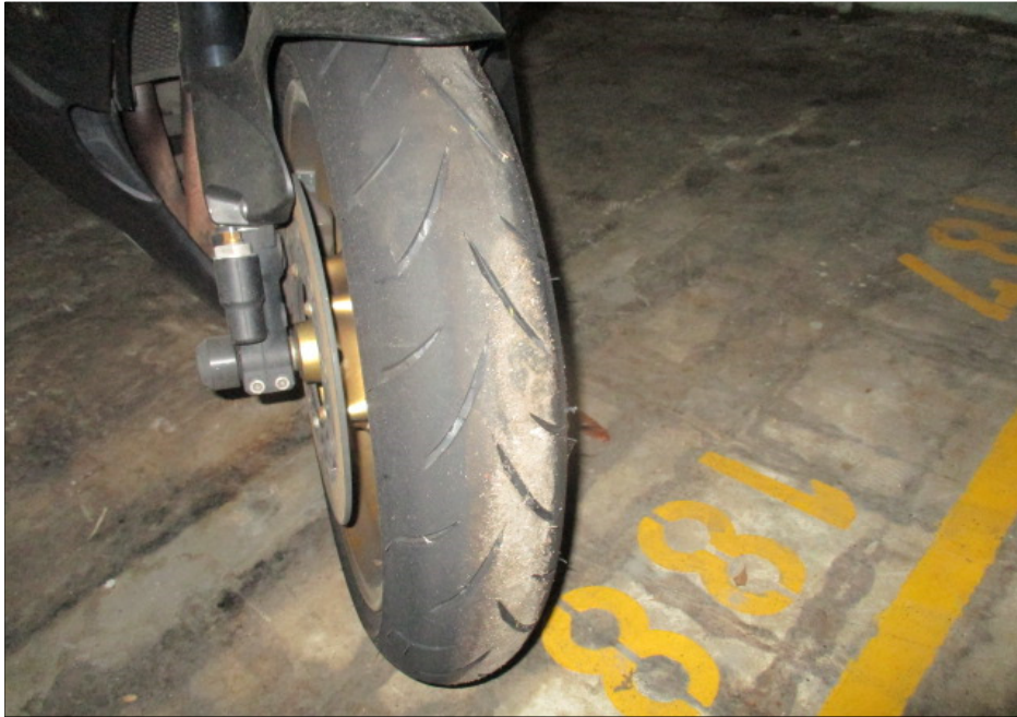
Photo 15 shows the condition of the Motorcycle's front tyre. The front tyre was observed to be in serviceable condition with remaining tread depth of approximately 3mm. The tyre was also observed to be sufficiently inflated for vehicular operation. We did not observe any tear, burst mark(s) and/or punctured hole(s) on the sidewalls as well as across the tread of the front tyre.
