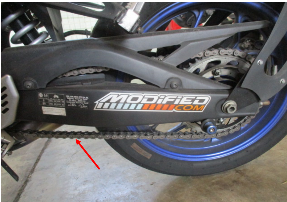
Photo 21 shows the general view of the gear train (arrowed) of the Motorcycle, which was observed to be intact with no misalignment. It was also adequately lubricated for operating purposes.
