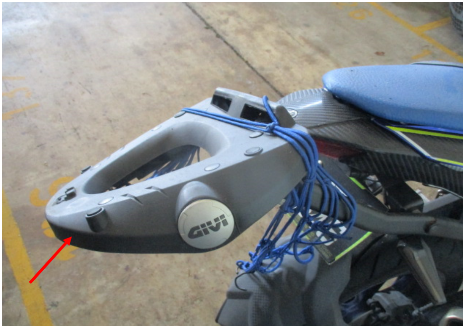
Photo 12 shows the damaged top box rack of the Motorcycle as a result of the accident (arrowed).
