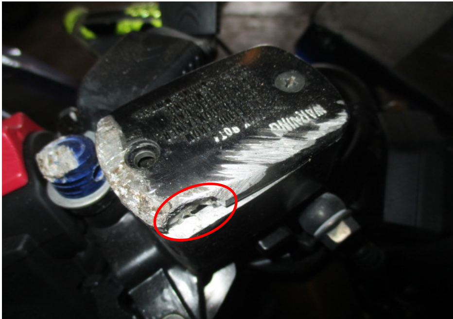
Photo 27 shows upon closer examination of the front brake reservoir, we observed a crack in the front brake reservoir as a result of the accident (circled).
