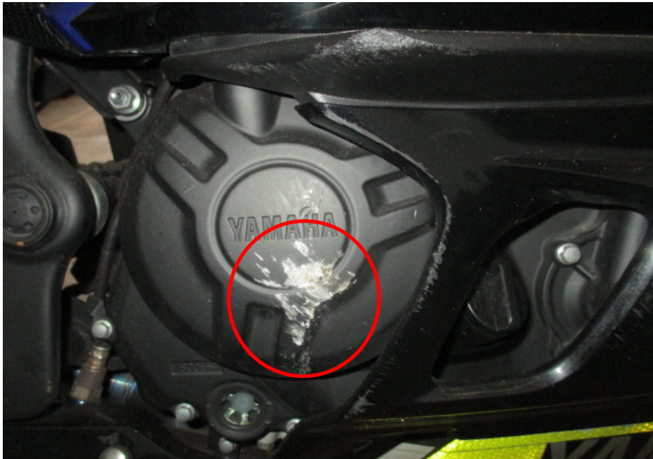
Photo 20 shows the right side of the engine of the Motorcycle at the time of our inspection. The various right engine components had sustained damage of grazing nature as a result of the accident (circled) however the engine components were still intact. There was also no fluid leak and/or fluid stain found around the right engine area of the Motorcycle.
