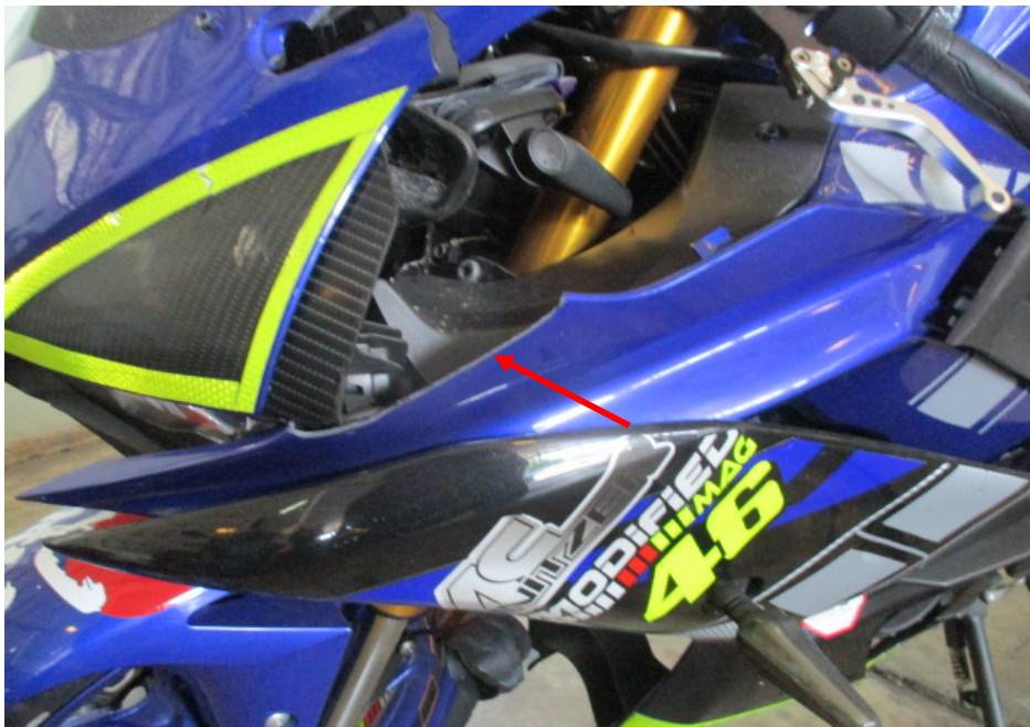
Photo 14 shows a closer view of the cracked left cowling of the Motorcycle as a result of the accident (arrowed).
