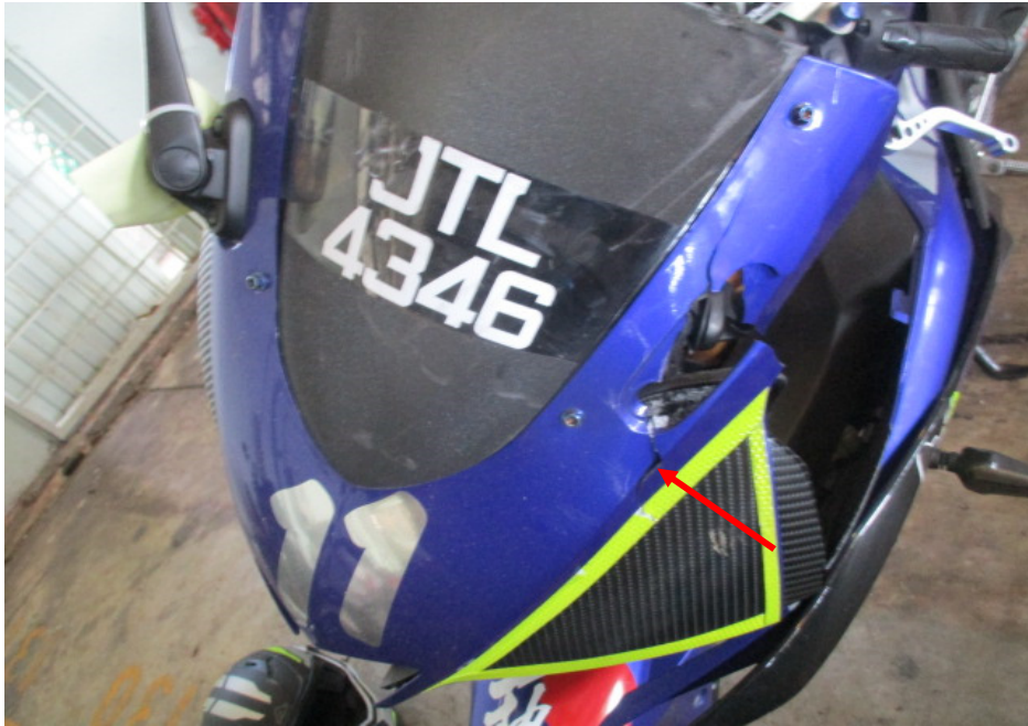
Photo 5 shows a closer view of the cracked front cowling (arrowed) of the Motorcycle as a result of the accident.
