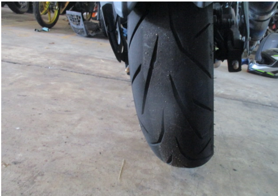
Photo 18 shows the condition of the Motorcycle's rear tyre. The rear tyre was observed to be in serviceable condition with remaining tread depth of approximately 4mm. The tyre was also observed to be sufficiently inflated for vehicular operation. We did not observe any tear, burst mark(s) and/or punctured hole(s) on the sidewalls as well as across the tread of the rear tyre.
