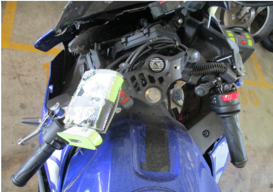
Photo 8 shows a closer view of the deformed handlebars which were amongst the body parts of the Motorcycle that had sustained damage as a result of the accident.
