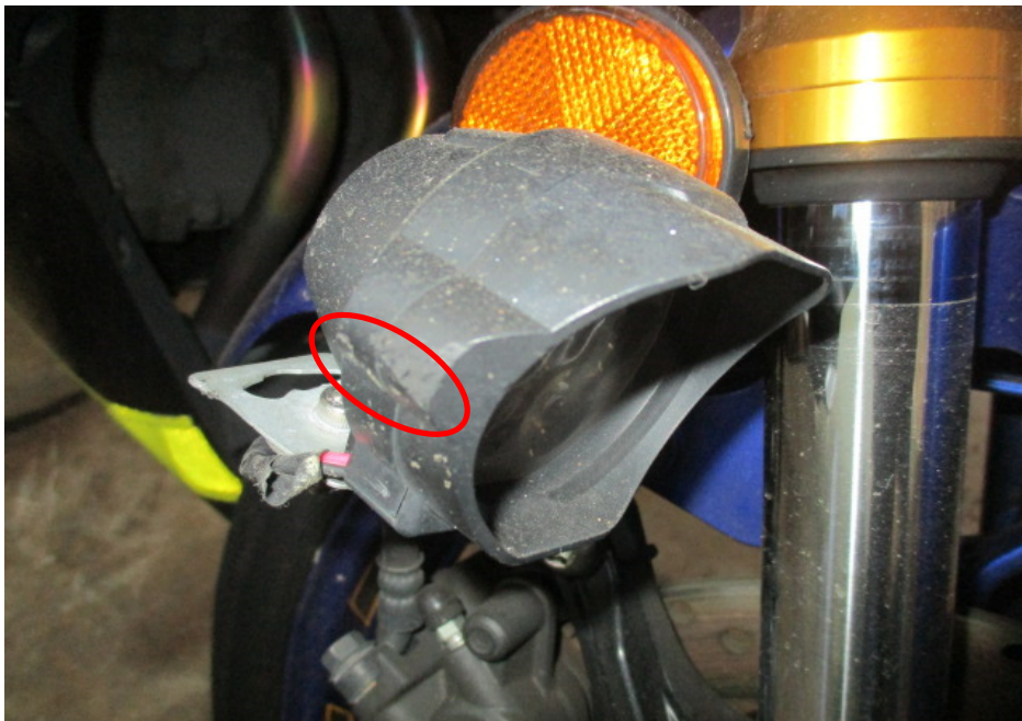
Photo 6 shows a close up view of the damaged right fog light of the Motorcycle as a result of the accident (circled).
