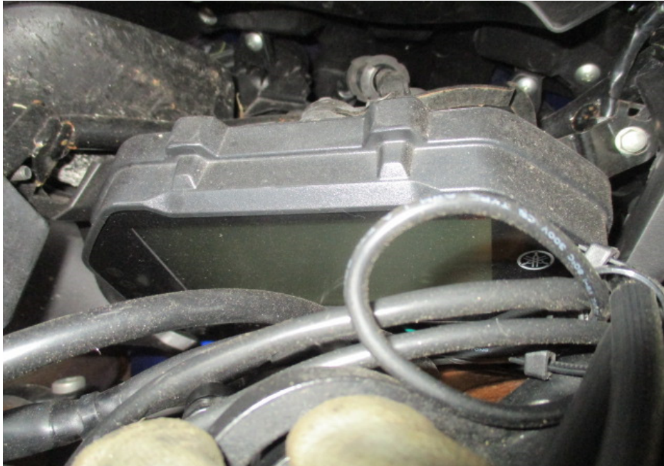
Photo 1 shows the speedometer gauge of the Motorcycle. The mileage of the Motorcycle could not be recorded at the time of our inspection due to damages sustained to the speedometer gauge.
