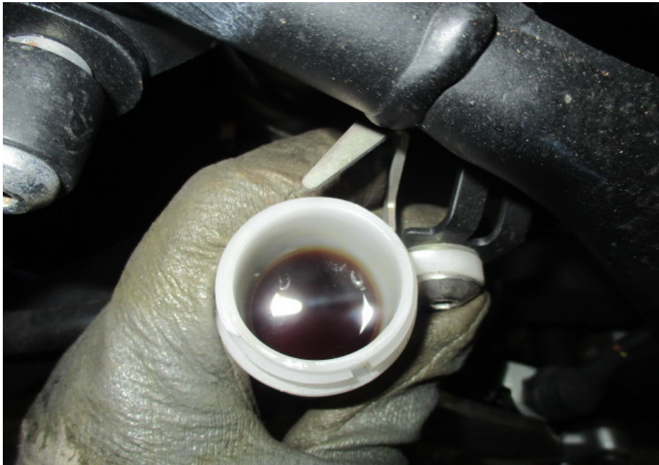
Photo 30 shows the brake fluid reservoir for the rear brake of the Motorcycle. The brake fluid was observed to be of sufficient level and without contamination for operational purposes.
