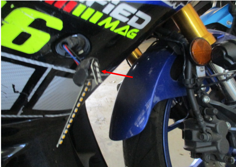
Photo 9 shows a closer view of the broken right front signal lamp of the Motorcycle as a result of the accident (arrowed).
