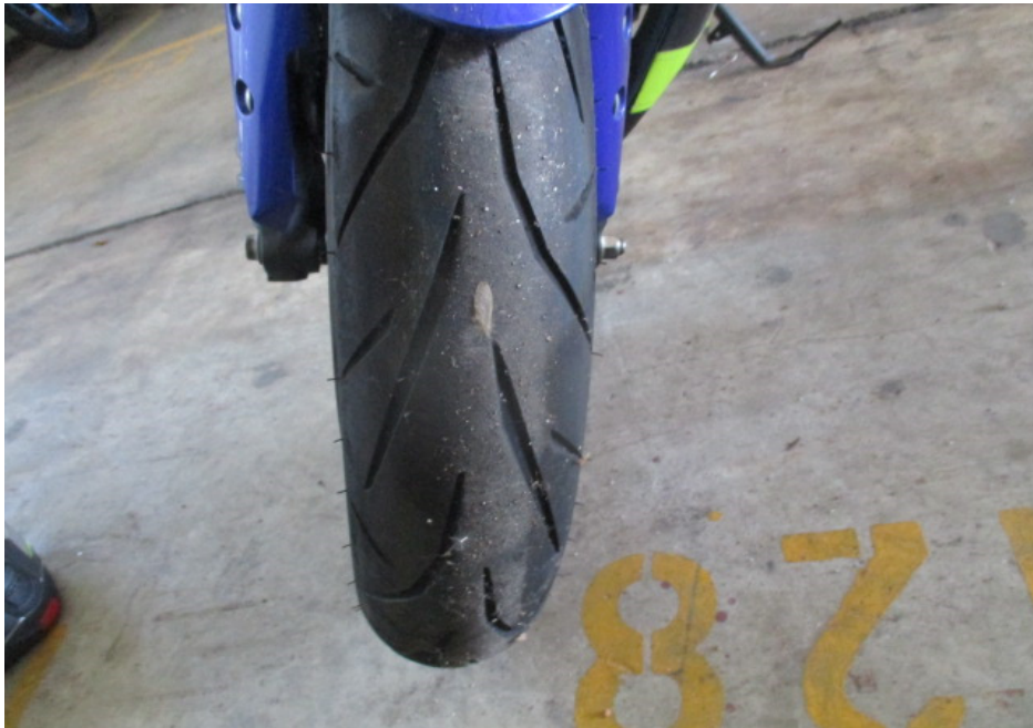
Photo 17 shows the condition of the Motorcycle's front tyre. The front tyre was observed to be in serviceable condition with remaining tread depth of approximately 4mm. There was no tear, burst mark(s) and/or punctured hole(s) on the sidewalls as well as across the tread of the front tyre.
