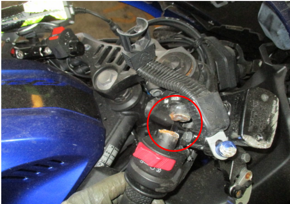
Photo 23 shows the right handlebar of the Motorcycle which was observed to be broken as a result of the accident (circled). We were hence not able to conduct any tests on the steering system of the Motorcycle.
