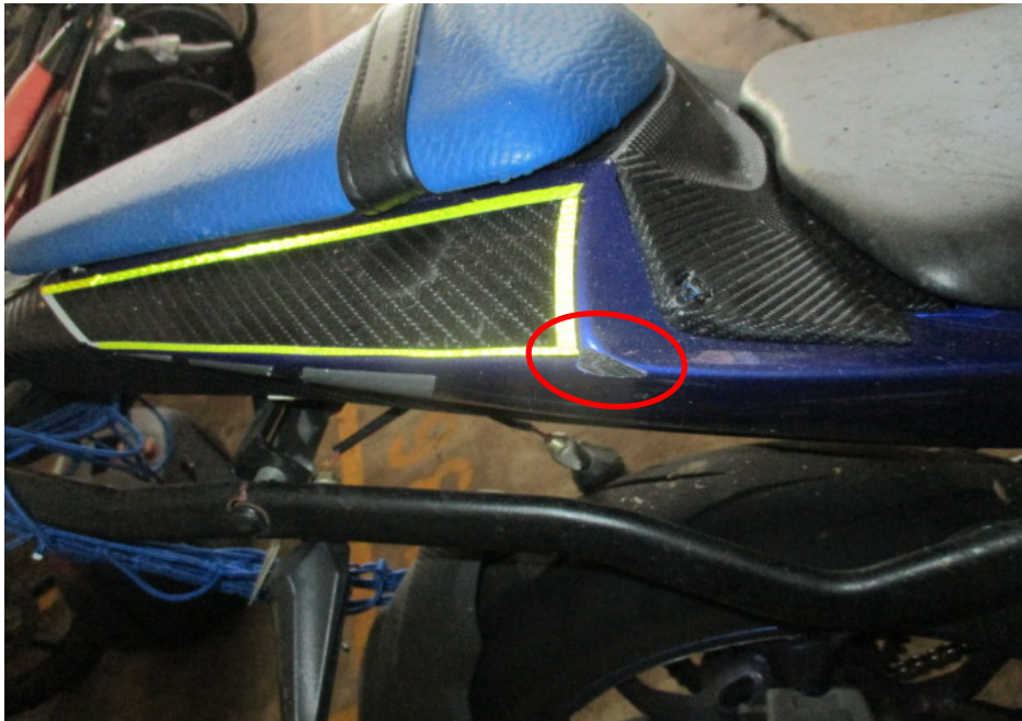
Photo 13 shows a closer view of the right rear side cover of the Motorcycle that had sustained damages of grazing nature as a result of the accident (circled).
