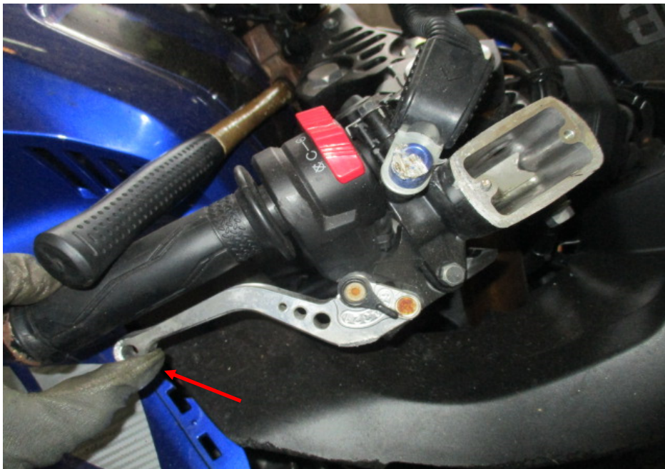
Photo 26 shows the front brake lever being depressed. There was no resistance felt (spongy like feel) upon pressing the front brake lever (arrowed). This would indicate that there may be a leakage of pressure/vacuum in the front brake system.
