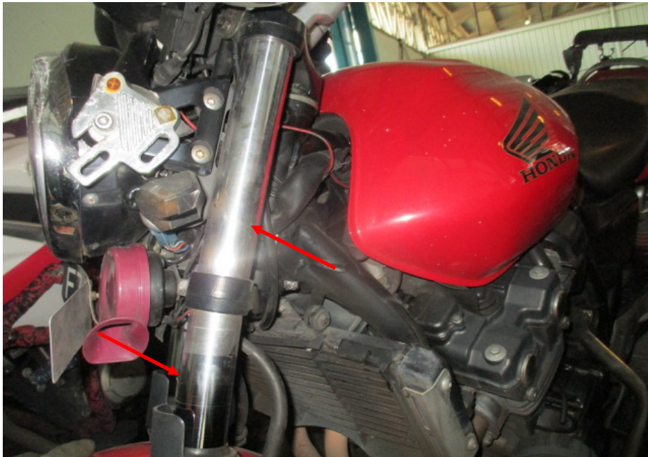
Photo 20 shows the left front fork of the Motorcycle. The left front fork (arrowed) was observed to be bent inwards as a result of the accident. We were hence not able to conduct any tests on the steering system of the Motorcycle.
