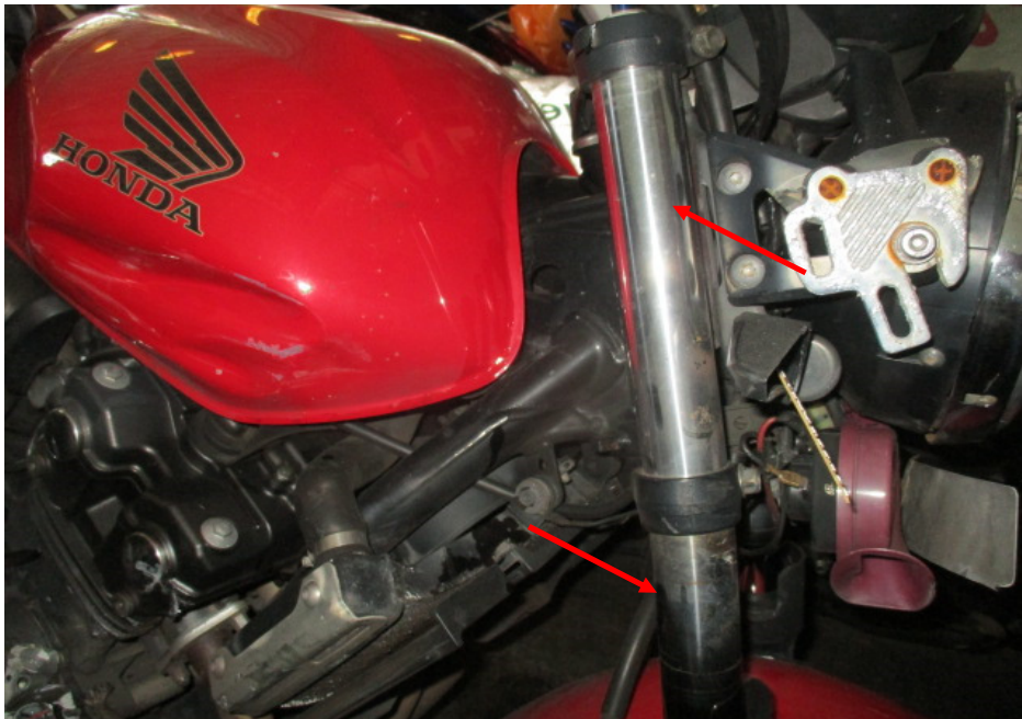
Photo 21 shows the right front fork of the Motorcycle. The right front fork (arrowed) was observed to be bent inwards as a result of the accident. We were hence not able to conduct any tests on the steering system of the Motorcycle.
