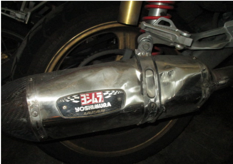
Photo 11 shows the dented exhaust muffler of the Motorcycle as a result of the accident.
