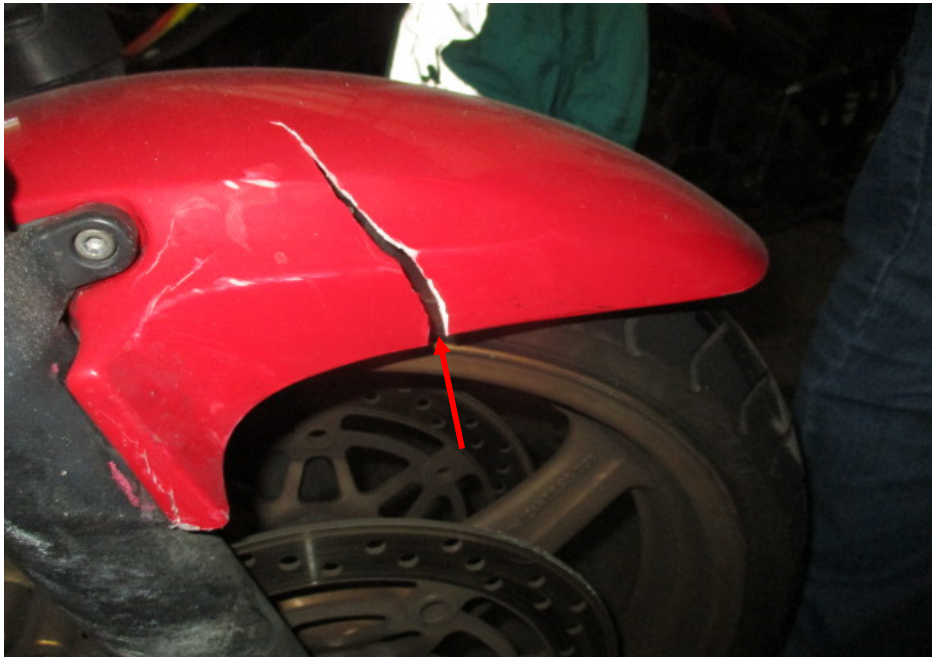
Photo 5 shows a closer view of the front mudguard which were amongst the body parts at the front body of the Motorcycle that had sustained damage as a result of the accident (arrowed).
