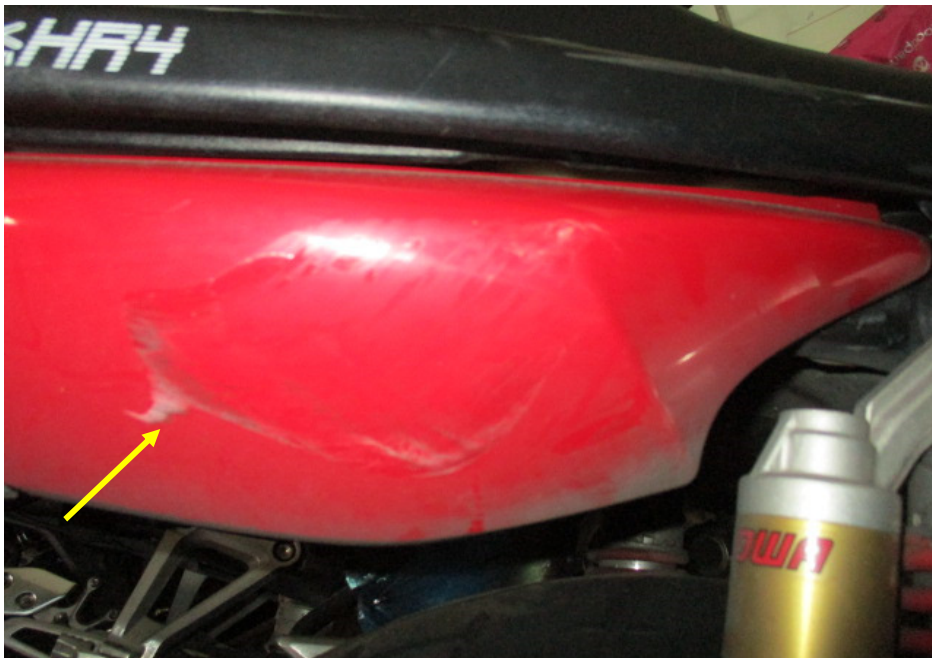
Photo 12 shows a closer view of the grazed right rear side cover (arrowed) of the Motorcycle as a result of the accident.
