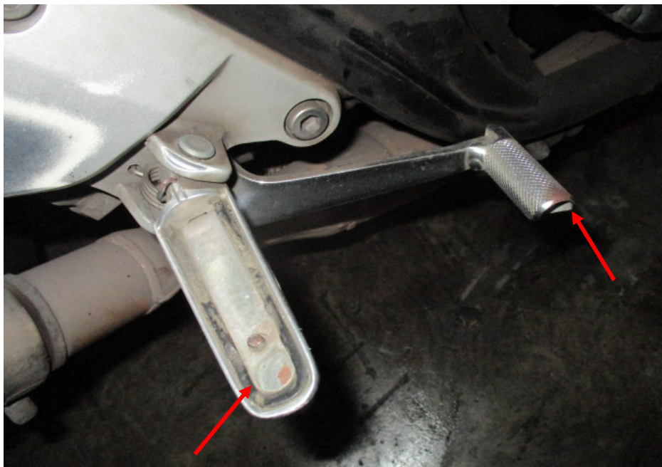
Photo 10 shows a closer view of the right front footrest and rear brake pedal (arrowed) which was amongst the body parts of the Motorcycle that had sustained damage as a result of the accident.
