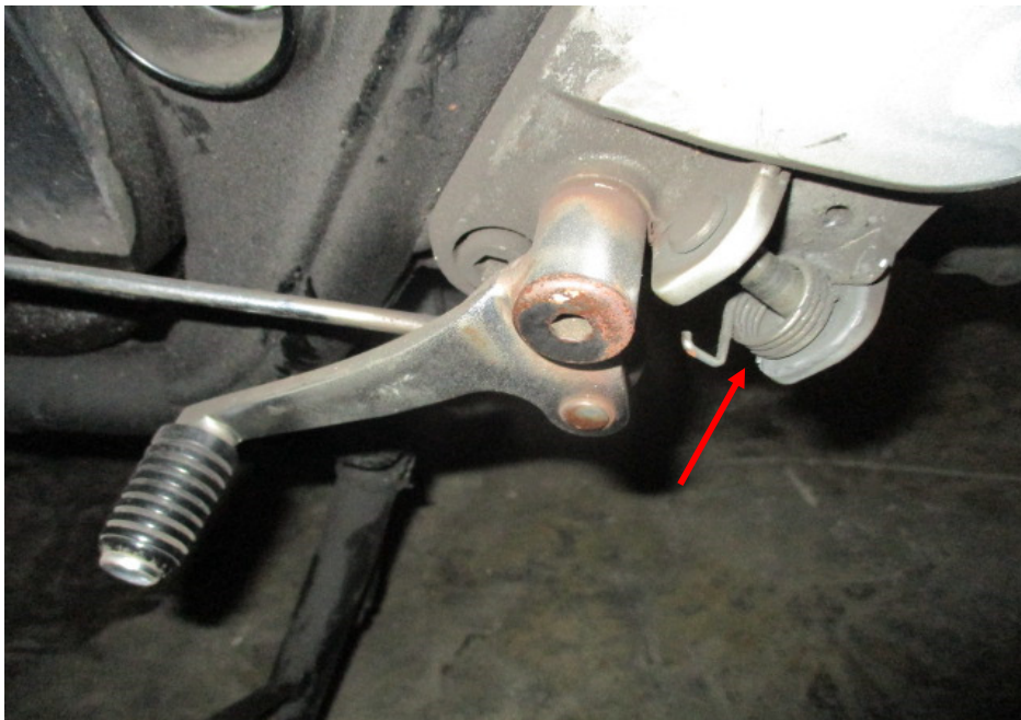
Photo 8 shows the broken left front footrest of the Motorcycle as a result of the accident (arrowed).
