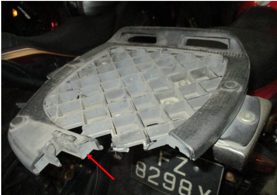
Photo 13 shows the cracked top box rack (arrowed) of the Motorcycle as a result of the accident.
