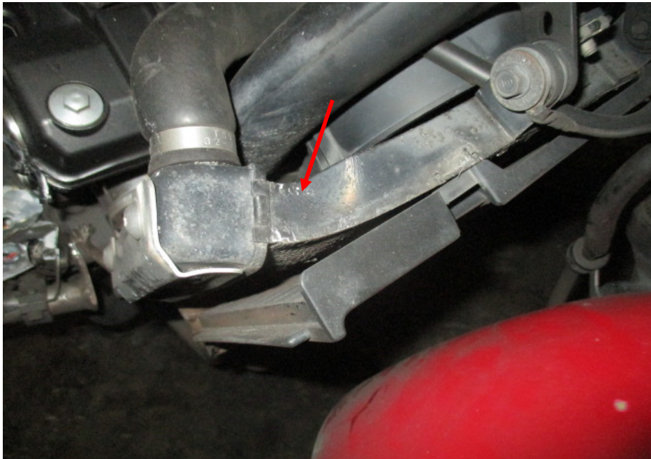
Photo 7 shows the deformed radiator of the Motorcycle as a result of the accident (arrowed).
