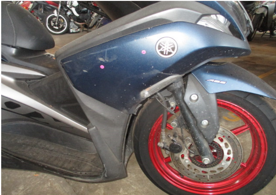
Photo 7 shows a closer view of the right cowling which was amongst the body parts at the front body of the Motorcycle that had sustained damage as a result of the accident.
