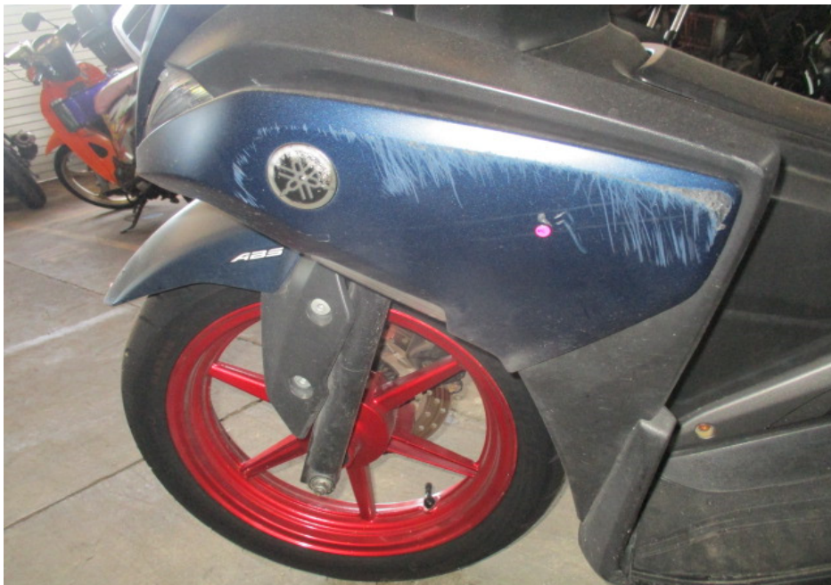
Photo 10 shows a closer view of the left cowling which was amongst the body parts at the front body of the Motorcycle that had sustained damage as a result of the accident.
