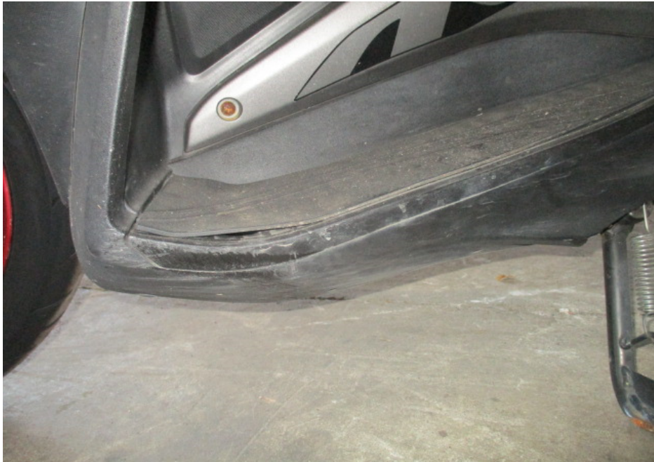
Photo 13 show a closer view of the left bottom cowling of the Motorcycle which was observed to be damaged due to the accident.
