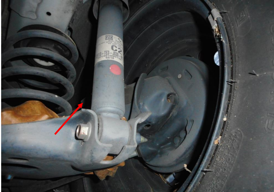
Photo 18 shows the brake pipe (arrowed) at the rear right wheel of the Motor Car. I did not observe any leakage of brake fluid at the time of my inspection of the Motor Car. My static tests of the Motor Car's braking system, along with my visual examination of the various mechanical components in the braking system, had indicated that there was no internal leakage of pressure/vacuum. Hence the braking system of the Motor Car was likely to be in serviceable condition at the material time of accident.
