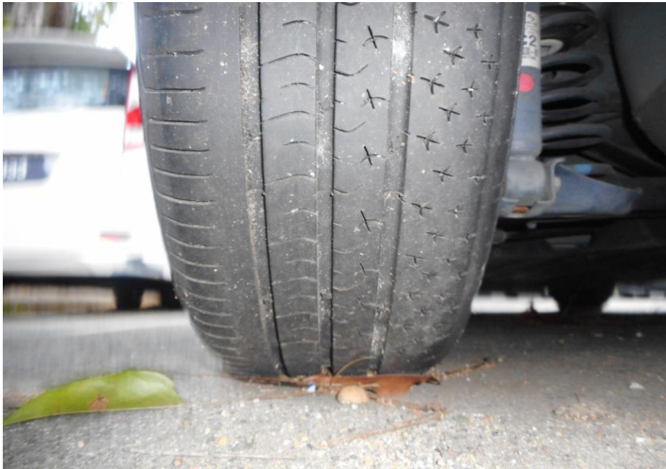
Photo 8 shows the condition of the rear left tyres of the Motor Car, which was observed to be in serviceable condition with remaining tread depth of approximately 6mm. The tyres, which were wrapped around standard alloy wheel rim, were also observed to be sufficiently inflated for vehicular operation. There was also no damage found on all 4 alloy wheel rims of the Motor Car.
