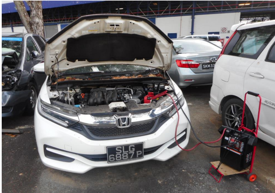
Photo 15 shows the jumpstarting of the Motor Car's engine, it was not able to be started up despite multiple attempts in jump starting the engine.
