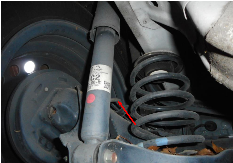
Photo 19 shows the brake pipe (arrowed) at the rear left wheel of the Motor Car. I did not observe any leakage of brake fluid at the time of my inspection of the Motor Car. My static tests of the Motor Car's braking system, along with my visual examination of the various mechanical components in the braking system had indicated that there was no internal leakage of pressure/vacuum. Hence the braking system of the Motor Car was likely to be in serviceable condition at the material time of accident.
