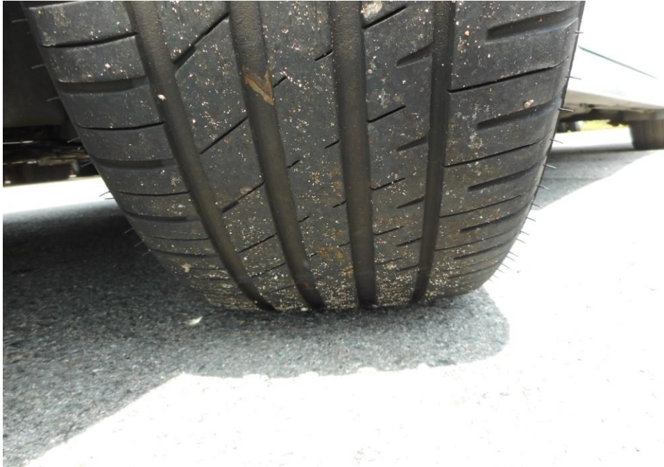
Photo 10 shows the condition of the front left tyre of the Motor Car, which was observed to be in serviceable condition with remaining tread depth of approximately 4.5mm. There was also no tear, cut or burst mark(s) on the outer and the inner sidewalls as well as across the tread of the Motor Car's 4 tyres.
