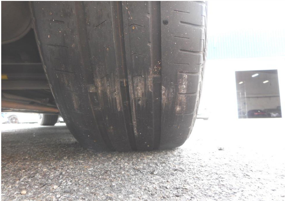
Photo 8 shows the condition of the rear right tyre of the Motor Car, which was observed to be in serviceable condition with remaining tread depth of approximately 3mm. The tyre was also observed to be sufficiently inflated for vehicular operation with no tear, cut or burst mark(s).
