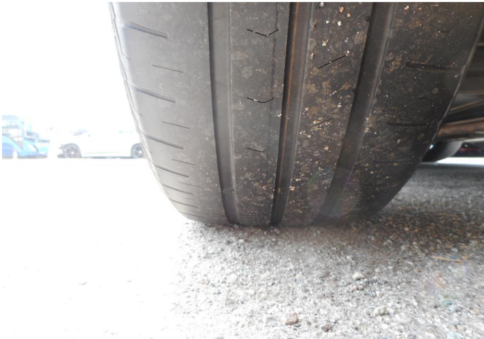
Photo 9 shows the condition of the rear left tyre of the Motor Car, which was observed to be in serviceable condition with remaining tread depth of approximately 2.8mm. The tyre, which was wrapped around steel wheel rim, was also observed to be sufficiently inflated for vehicular operation. The 4 tyres of the Motor Car were wrapped around standard steel wheel rims.
