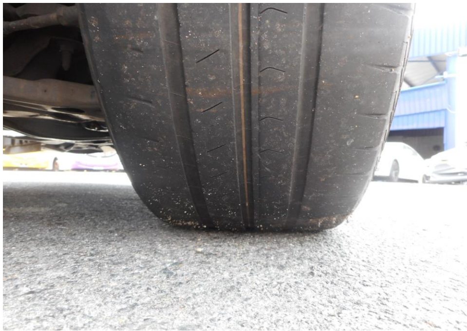
Photo 7 shows the condition of the front right tyre of the Motor Car, which was observed to be in serviceable condition with remaining tread depth of approximately 2.5mm. The tyre was sufficiently inflated for vehicular operation with no tear, cut or burst mark(s) on the outer and the inner sidewalls as well as across the tread. The 4 tyres of the Motor Car were wrapped around standard steel wheel rims without any damage.
