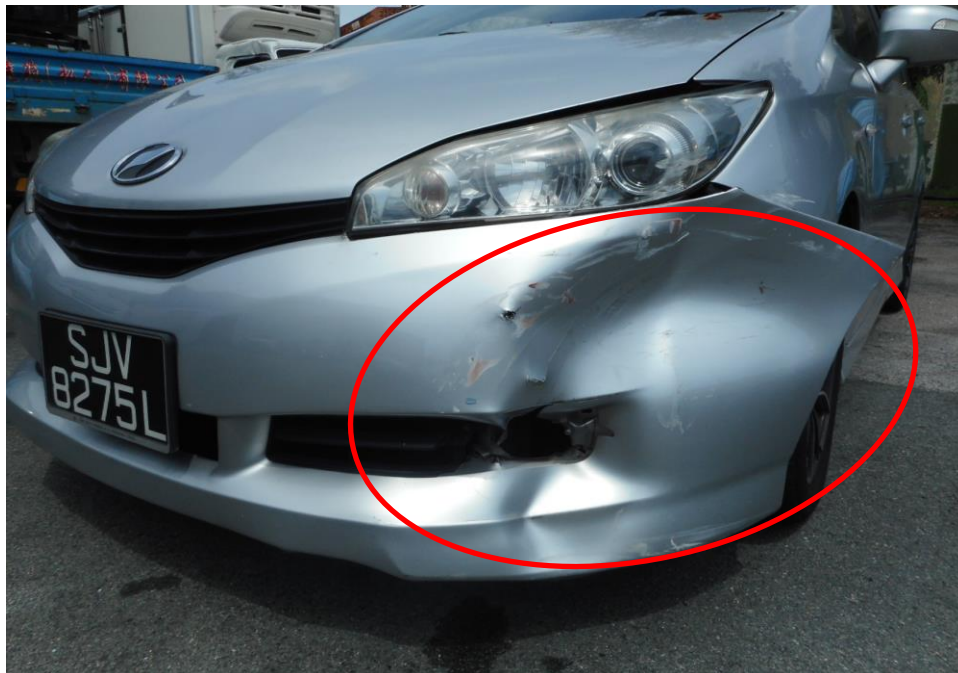
Photo 3 shows the close up view of the Motor Car's front body at the time of my inspection. The Motor Car was observed to have sustained damage at its front bumper (circled), as a result of the accident.
