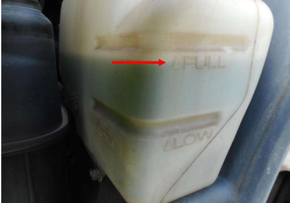
Photo 11 shows the engine coolant reservoir of the Motor Lorry at the time of my inspection. The engine coolant was observed to be of sufficient level (arrowed) and without any visible contamination.
