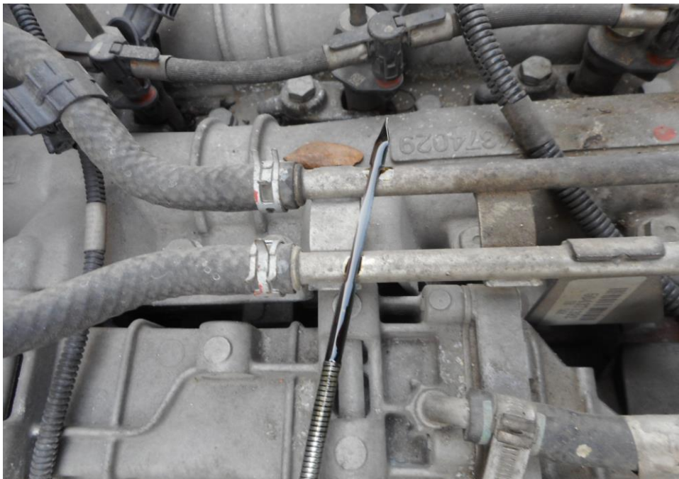
Photo 12 shows the engine oil dip stick of the Motor Lorry at the time of my inspection. The engine oil was observed to be of sufficient level and without any visible contamination.
