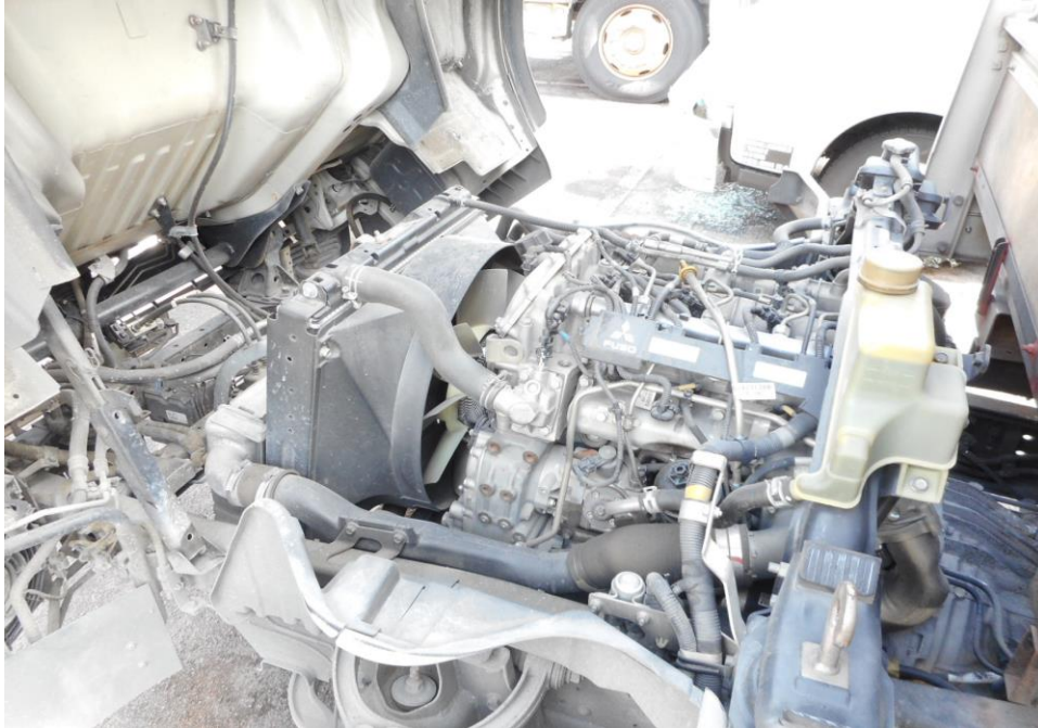
Photo 9 shows a general view of the Motor Lorry's engine compartment, which was accessed by lifting the front cabin of the Motor Lorry. The various parts and components inside the engine compartment were unaffected by the accident. There was also no sign(s) or indication(s) of fresh fluid leakage and/or fluid stain within the engine compartment
