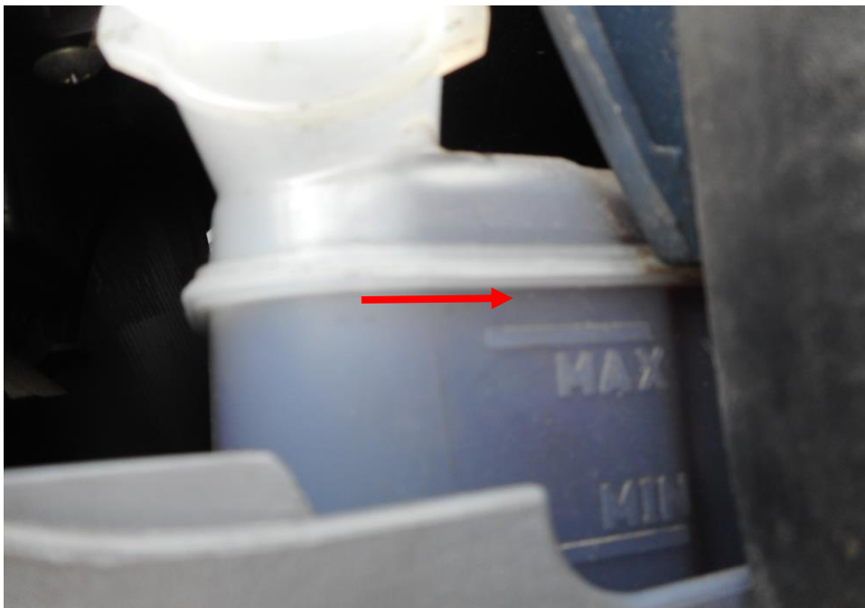
Photo 10 shows the brake fluid reservoir of the Motor Lorry at the time of my inspection. The brake fluid was observed to be of sufficient level (arrowed) and without any visible contamination.
