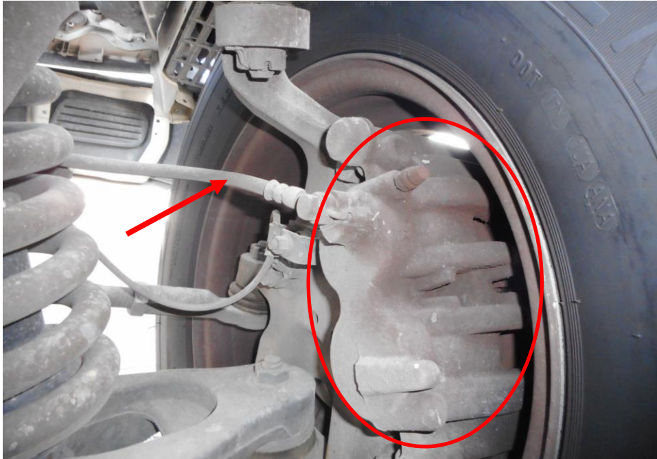
Photo 19 shows the brake hose/pipe (arrowed) at the front right wheel of the Motor Lorry. No leakage of brake fluid was observed. Visual examination of the various components of the braking system like the brake caliper (circled), brake booster, brake pedal etc had revealed all to be intact and without visible damage at the time of accident. There was also no sign of fluid stain(s) observed on the various undercarriage components.
