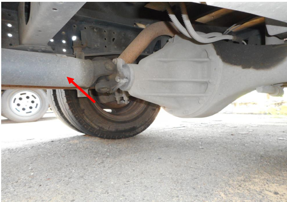
Photo 21 shows the various undercarriage components at the rear right wheel of the Motor Lorry, in particular the drive shaft (arrowed). The various steering components were all found to be intact, suggesting that the steering system of the Motor Lorry was likely to be in serviceable condition at the material time of accident. There was also no sign of fluid stain(s) observed on the various undercarriage components.
