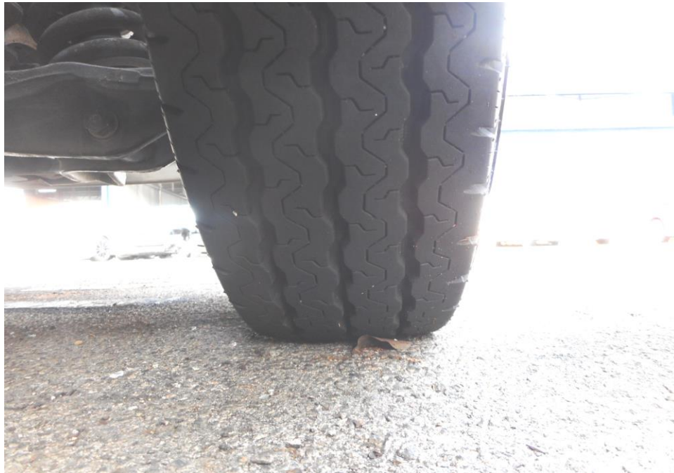
Photo 5 shows the condition of the front right tyre of the Motor Lorry, which was observed to be in serviceable condition with remaining tread depth of approximately 8.8mm. The tyre, which was wrapped around standard steel wheel rim, was also observed to be sufficiently inflated for vehicular operation. There was no tear, cut or burst mark(s) on the outer and the inner sidewalls as well as across the tread of the 6 tyres that were fitted on the Motor Lorry.
