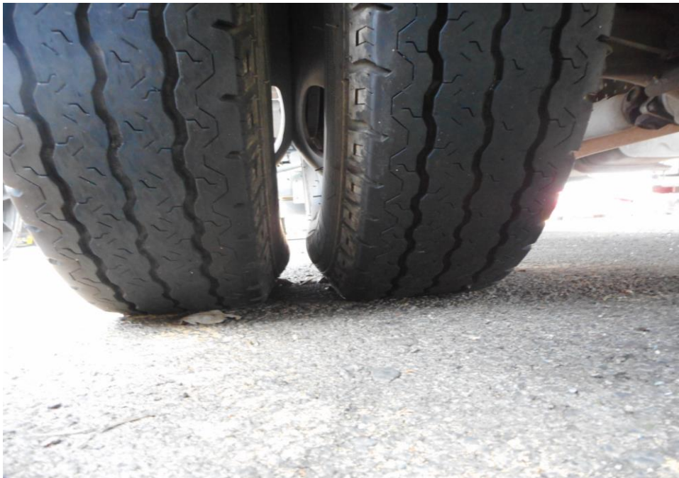
Photo 7 shows the condition of the rear left tyres of the Motor Lorry, which was observed to be in serviceable condition with remaining tread depth of approximately 3.5mm. The tyres, which were wrapped around standard steel wheel rim, were also observed to be sufficiently inflated for vehicular operation. There was also no damage found on all 6 steel wheel rims of the Motor Lorry.
