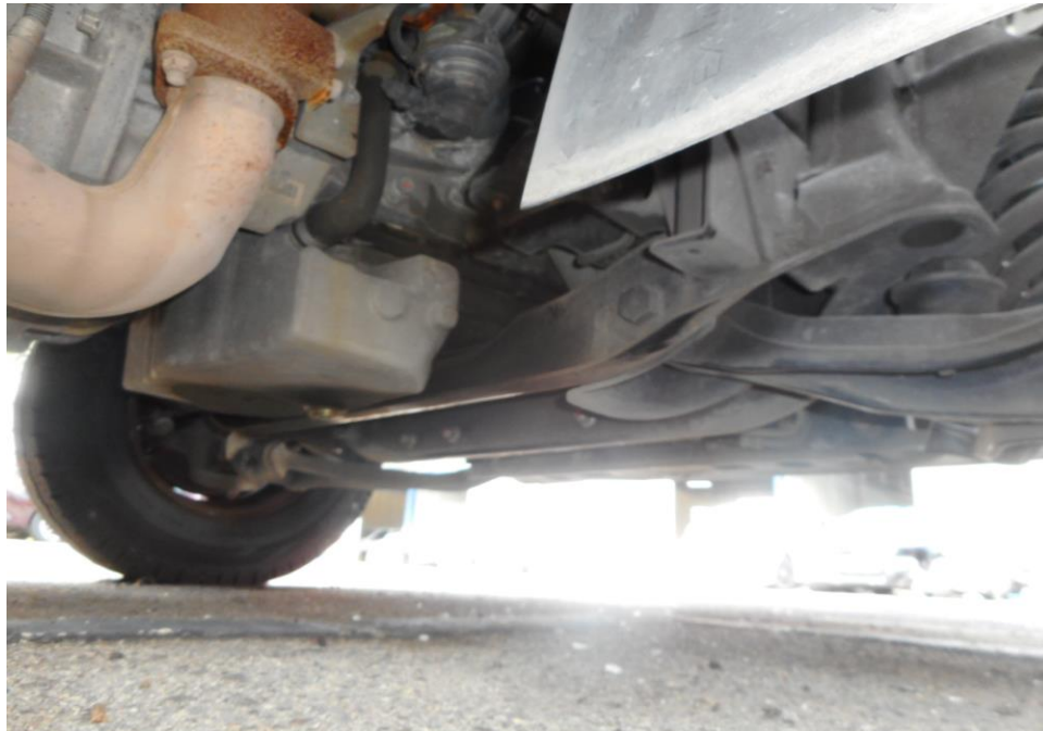
Photo 14 shows the undercarriage of the Motor Lorry, at the area where the engine housing and transmission housing are located. . I did not find any sign(s) or indication(s) of fluid leak and/or fluid stain(s) on the underside of the Motor Lorry.
