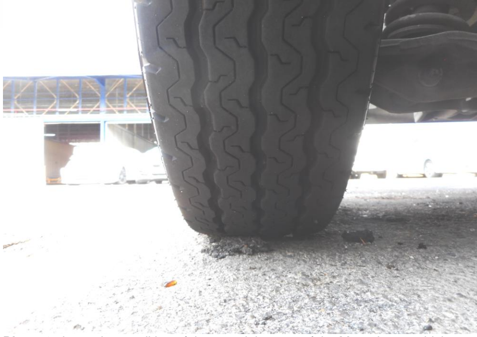
Photo 8 shows the condition of the rear right tyres of the Motor Lorry, which were observed to be in serviceable condition with remaining, tread depth of approximately 8.2mm. There was also no tear, cut or burst mark(s) on the outer and the inner sidewalls as well as across the tread of the 4 tyres that were fitted on the Motor Lorry.
