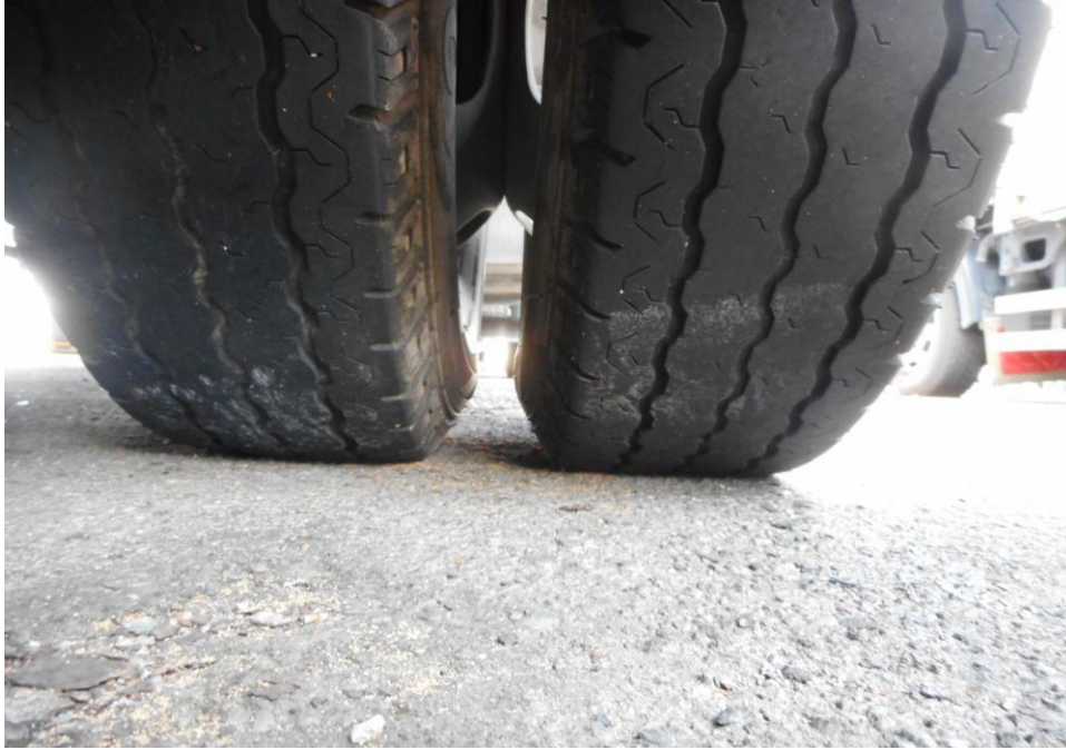
Photo 6 shows the condition of the rear right tyre of the Motor Lorry, which was observed to be in serviceable condition with remaining tread depth of approximately 7.8mm. The tyre, which was wrapped around standard steel wheel rim, was also observed to be sufficiently inflated for vehicular operation.
