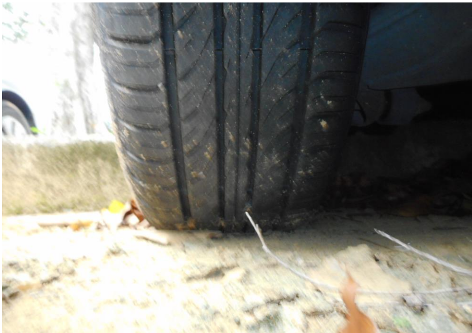
Photo 7 shows the condition of the rear right tyre of the Motor Car, which was observed to be in serviceable condition with remaining tread depth of approximately 6.2mm. The tyre was also observed to be sufficiently inflated for vehicular operation with no tear, cut or burst mark(s).
