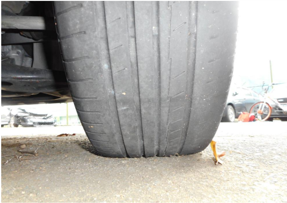
Photo 6 shows the condition of the front right tyre of the Motor Car, which was observed to be in serviceable condition with remaining tread depth of approximately 3.4mm. The tyre was sufficiently inflated for vehicular operation with no tear, cut or burst mark(s) on the outer and the inner sidewalls as well as across the tread. The 4 tyres of the Motor Car were wrapped around standard alloy wheel rims without any damage.
