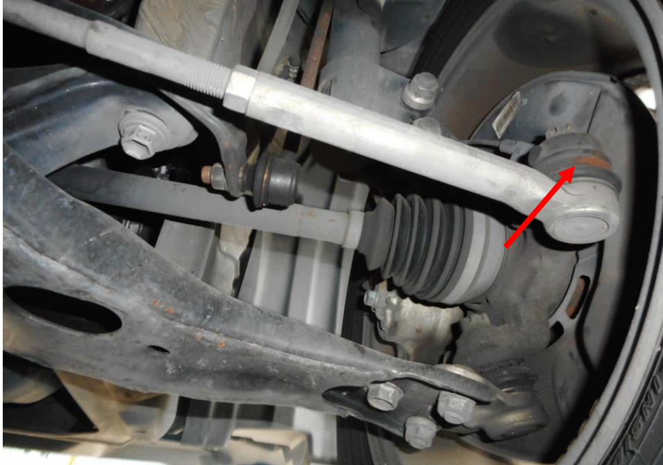
Photo 20 shows the various undercarriage components at the front right wheel of the Motor Car, in particular the steering tie rod (red arrow). The various steering components were all found to be intact, suggesting that the steering system of the Motor Car was likely to be in serviceable condition at the material time of accident. There was also no sign of fluid stain observed on the various undercarriage components at the front right wheel of the Motor Car.
