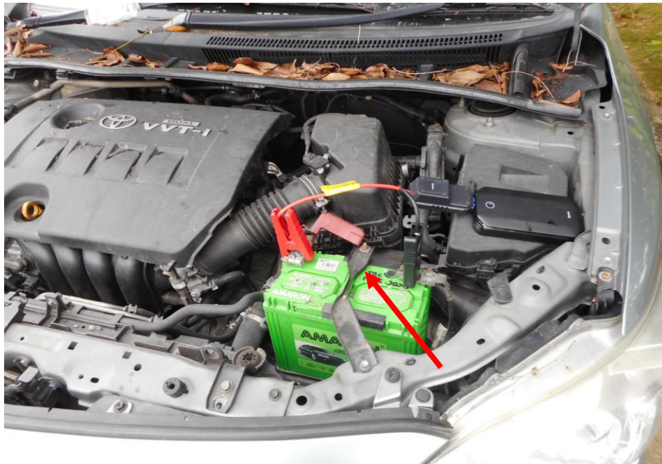
Photo 15 shows the jumpstarting process of the Motor Car's engine. The engine of the Motor Car was unable to be jumpstarted up despite multiple attempts in starting it.
