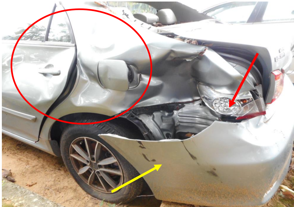
Photo 3 shows the close up view of the Motor Car's left body at the time of my inspection. The rear bumper (yellow arrow), rear left brake lamp (red arrow) and the left door and body panels (circled) of the Motor Car was observed to have been damaged by the accident.
