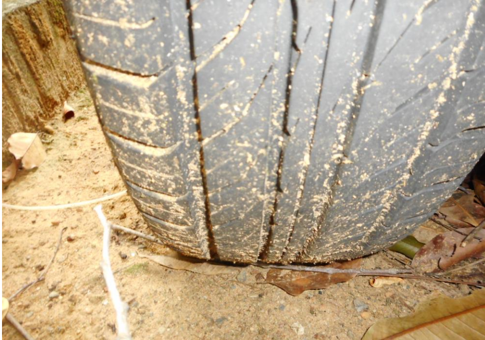
Photo 8 shows the condition of the rear left tyre of the Motor Car, which was observed to be in serviceable condition with remaining tread depth of approximately 6mm. The tyre was also observed to be sufficiently inflated for vehicular operation with no tear, cut or burst mark(s).
