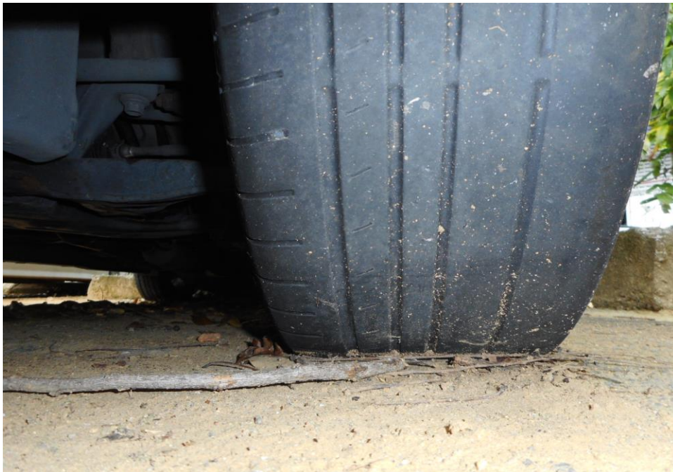
Photo 9 shows the condition of the front left tyre of the Motor Car, which was observed to be in serviceable condition with remaining tread depth of approximately 1.8 mm. There was also no tear, cut or burst mark(s) on the outer and the inner sidewalls as well as across the tread of the Motor Car's 4 tyres.
