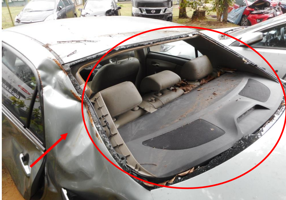
Photo 2 shows the close up view of the Motor Car's rear body at the time of my inspection. The rear windscreen (circled) and the rear body panel (arrowed) was observed to have been damaged by the accident.
