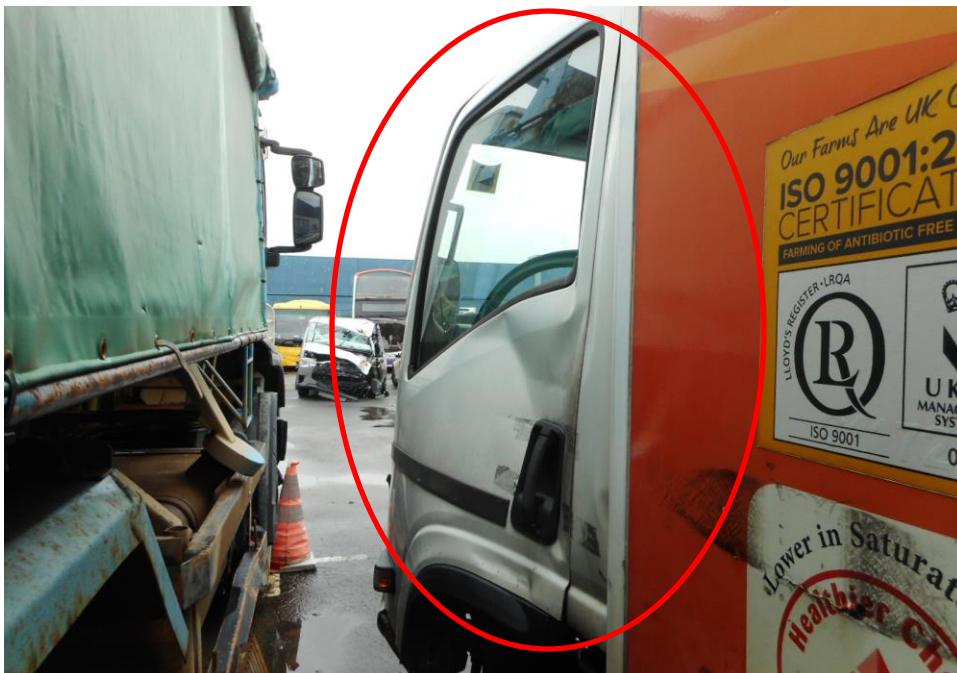
Photo 6 shows a close up view of the left body of the Motor Lorry at the time of our inspection. The Motor Lorry was observed to have sustained damages to its left door (circled) as a result of the accident.
