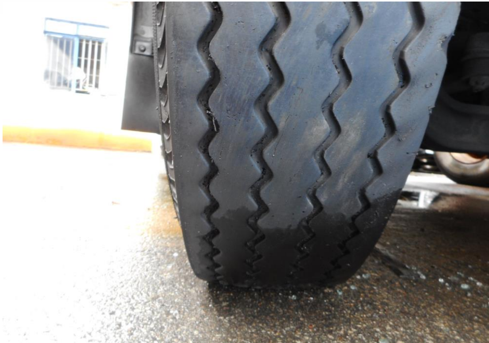
Photo 9 shows the condition of the front right tyre of the Motor Lorry, which was observed to be in serviceable condition with remaining tread depth of approximately 5.4mm. The tyre, which was wrapped around standard steel wheel rim, was also observed to be sufficiently inflated for vehicular operation.
