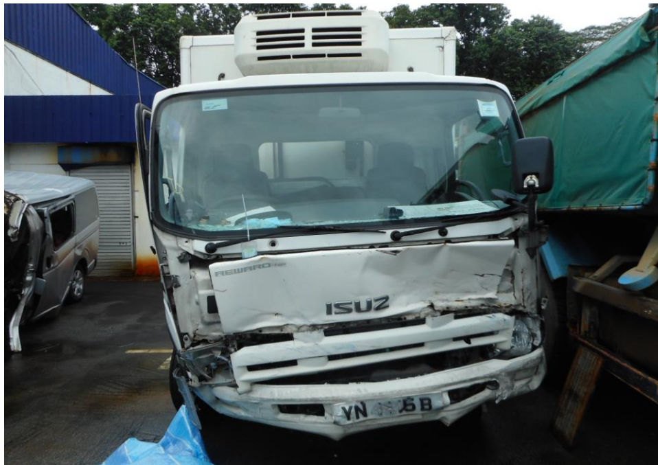
Photo 2 shows a general view of its front cabin structure portion. Its front windscreen, front body panel, front bumper, right and left doors as well as both front headlamps was damaged as a result of the accident.
