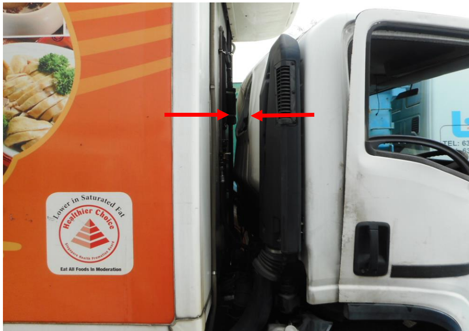
Photo 13 shows the induced damage to the cabin of the Motor Lorry's which immobilised the opening and viewing (arrowed) of the various parts and components inside the engine compartment, a result of the accident.
