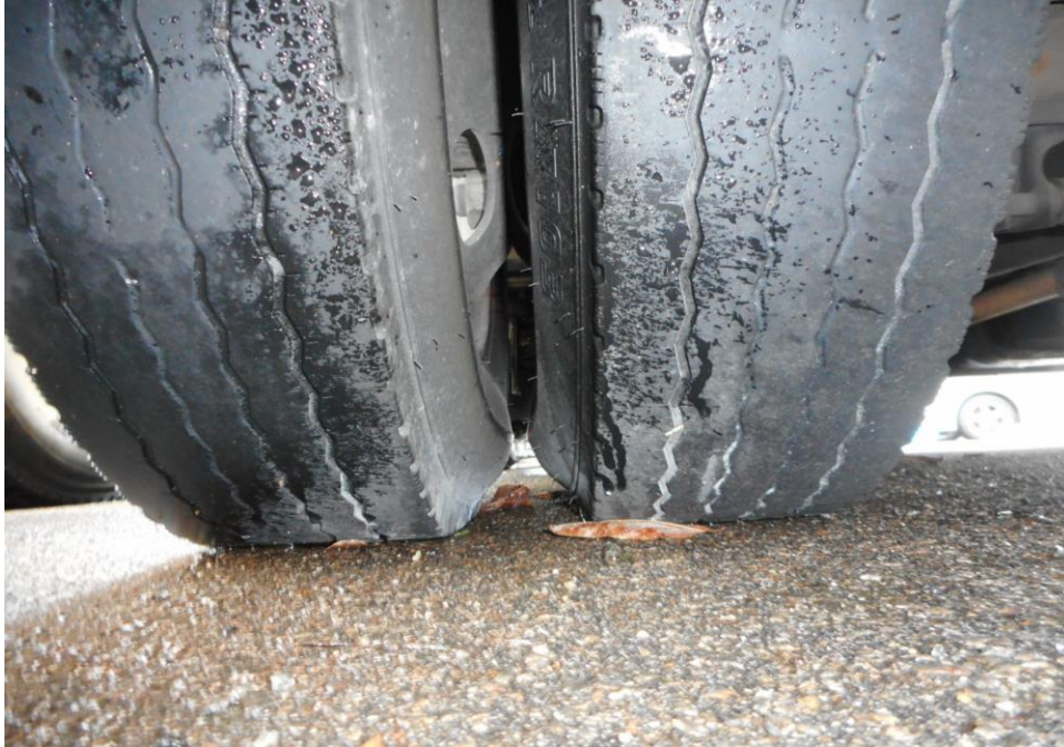
Photo 11 shows the condition of the rear left tyre of the Motor Lorry, which was observed to be in serviceable condition with remaining tread depth of approximately 1.8mm. The tyre, which was wrapped around standard steel wheel rim, was also observed to be sufficiently inflated for vehicular operation.
