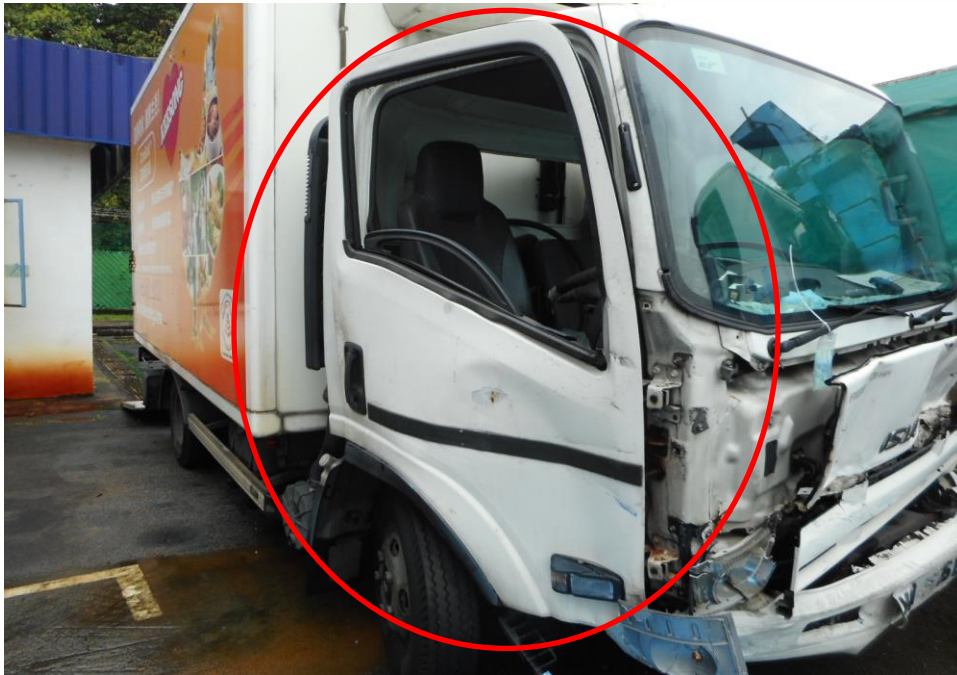
Photo 5 shows a close up view of the right body of the Motor Lorry at the time of our inspection. The Motor Lorry was observed to have sustained damages to its right door (circled) as a result of the accident.
