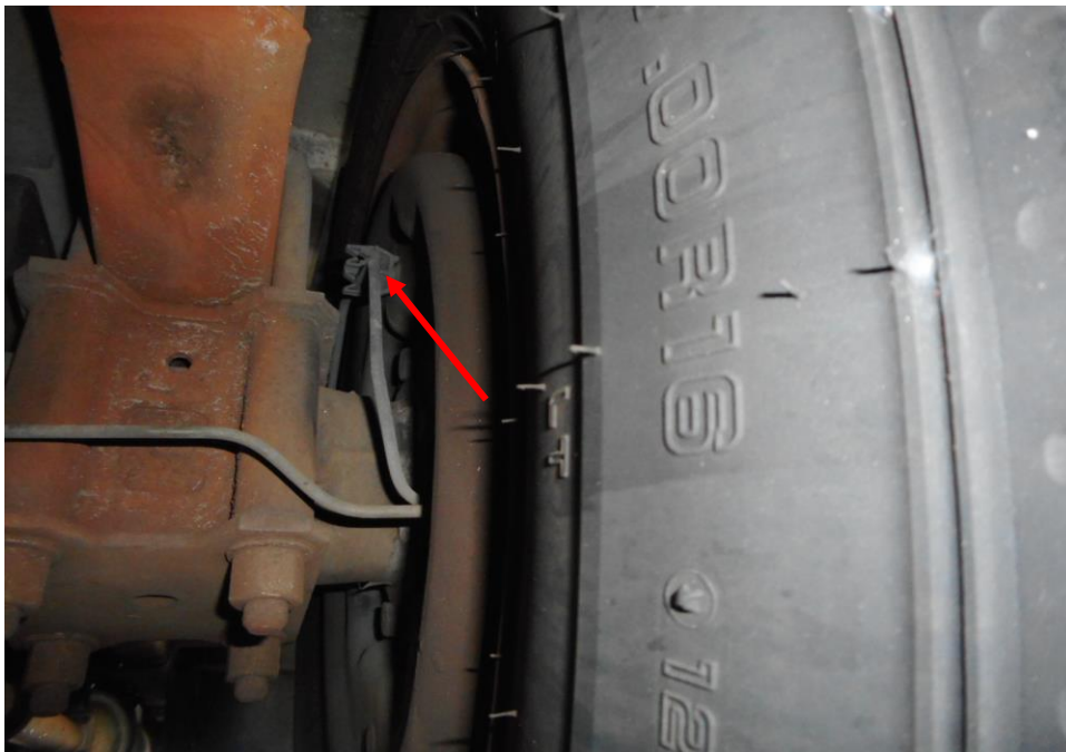
Photo 20 shows the brake pipe (arrowed) at the rear right wheel of the Motor Lorry. I did not observe any leakage of brake fluid at the time of my inspection of the Motor Lorry. My static tests of the Motor Lorry's braking system, along with my visual examination of the various mechanical components in the braking system, had indicated that there was no internal leakage of pressure/vacuum.
