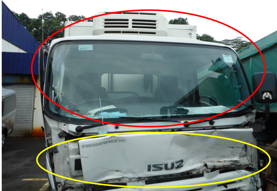
Photo 3 shows a close up view of the front body of the Motor Lorry at the time of our inspection. The Motor Lorry was observed to have sustained damages to its front cabin body structure, front windscreen (red circle) and front cabin body panel (yellow circle) as a result of the accident.
