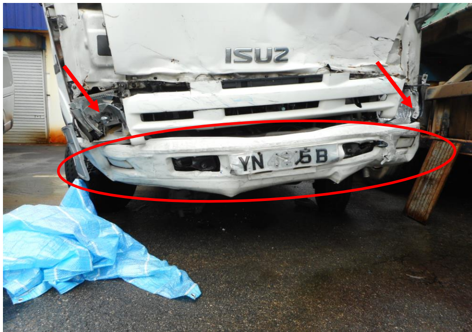
Photo 4 shows a close up view of the front body of the Motor Lorry at the time of our inspection. The Motor Lorry was observed to have sustained damages to its front bumper (circled) and both its front headlamps (arrowed) as a result of the accident.
