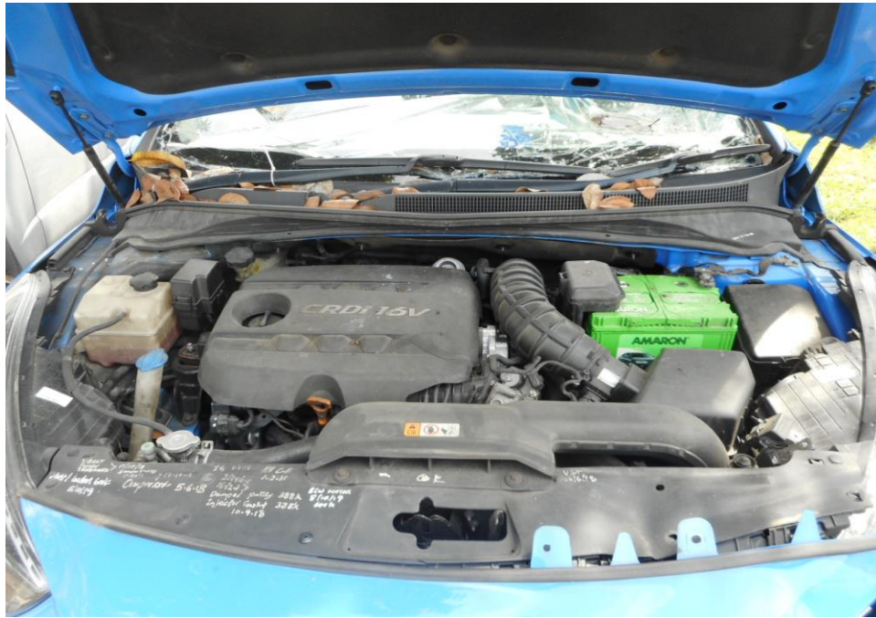
Photo 14 shows a general view of the Motor Taxi's engine compartment. The various parts and components inside the engine compartment were unaffected by the accident. There was also no sign(s) or indication(s) of fluid leakage and/or fluid stain within the engine compartment.
