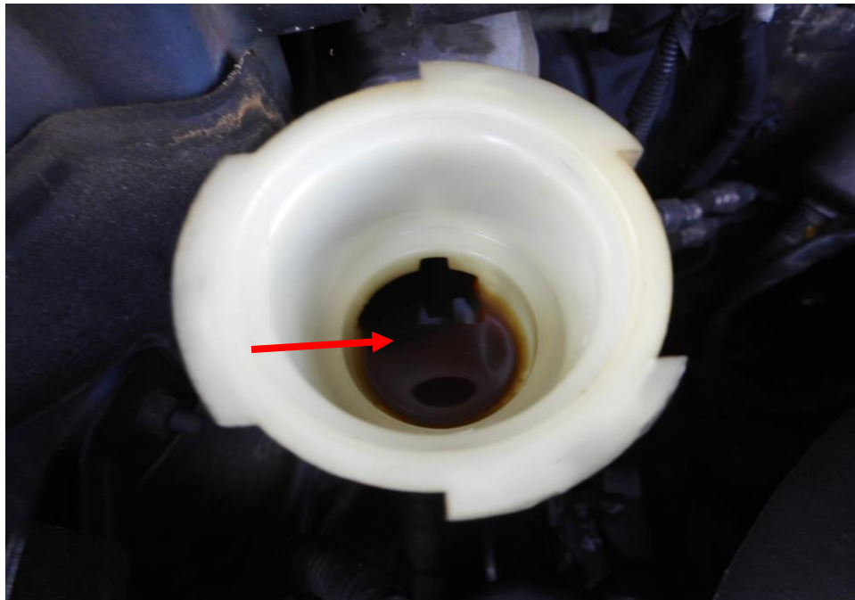
Photo 15 shows the brake fluid reservoir of the Motor Taxi at the time of my inspection. The brake fluid was observed to be of sufficient level (arrowed) and without any visible contamination.
