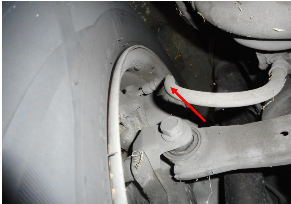
Photo 20 shows the brake hose/pipe (arrowed) at the rear left wheel of the Motor Taxi. I did not observe any leakage of brake fluid at the time of my inspection of the Motor Taxi. Static tests of the Motor Taxi's braking system had indicated that there was no internal leakage of pressure/vacuum. The undercarriage components of the Motor Taxi were also all found to be intact and without any visible damage.
