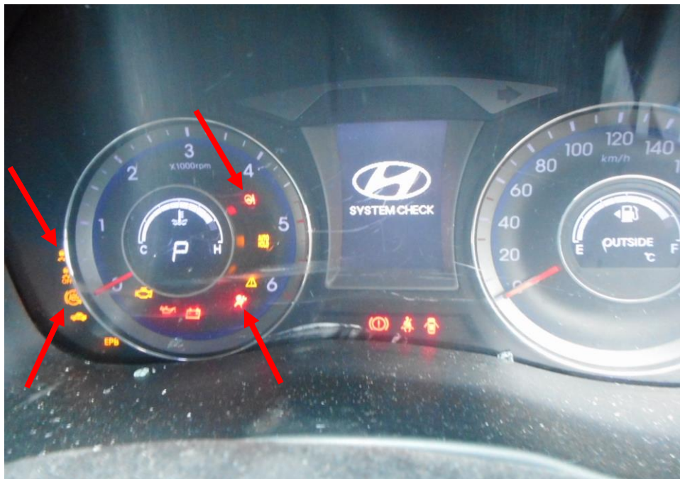
Photo 25 shows the warning light for Anti-Lock Brake System (ABS), Supplemental Restraint System (SRS), Electric Power Steering System (EPS) and Traction Control System (TC) appearing on the instrument panel of the Motor Taxi during the self-test of its various electronic operating systems when its engine was cranked.
