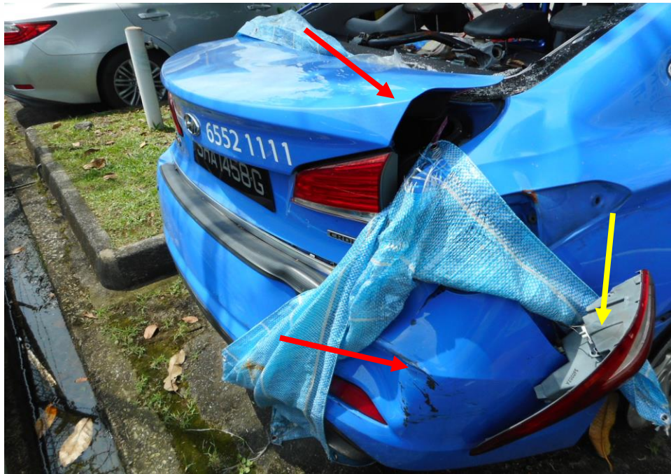
Photo 9 shows the close up view of the Motor Taxi's rear body at the time of my inspection. The Motor Taxi rear was observed to sustained damage at its rear portion. Its rear boot, rear bumper (red arrows) and rear right headlamp (yellow arrow) were amongst the body parts that were damaged as a result of the accident.
