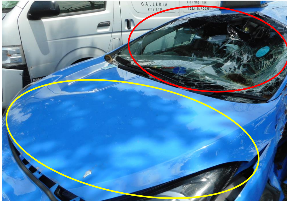
Photo 3 shows the close up view of the Motor Taxi's front body at the time of my inspection. The Motor Taxi was observed to have sustained damage at its front portion. Its front windscreen (red circle) and front bonnet (yellow circle) were amongst the body parts that were damaged as a result of the accident.
