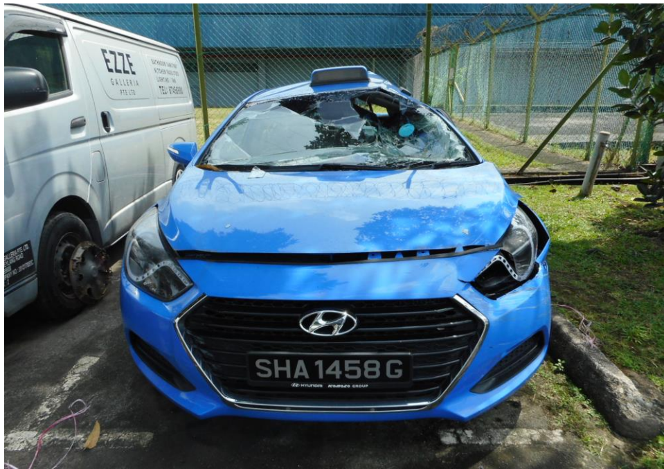
Photo 2 shows a general view of the Motor Taxi's front body at the time of my inspection. The Motor Taxi was observed to sustained damage at its front, left, rear and roof portion. Its front windscreen, bumper, bonnet, front left fender, front left headlamp, its left body panels, rear windscreen, rear boot and roof were amongst the body parts that were damaged as a result of the accident.
