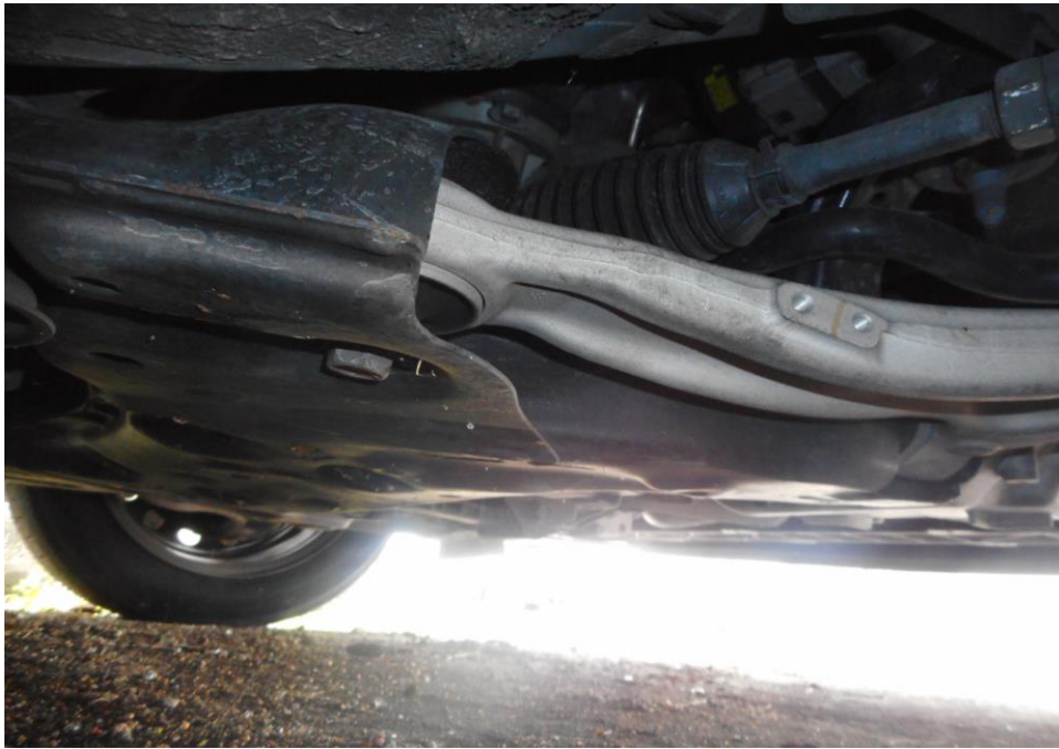
Photo 18 shows the undercarriage of the Motor Taxi, at the area where the engine housing and transmission housing are located. . I did not find any sign(s) or indication(s) of fluid leak and/or fluid stain(s) on the underside of the Motor Taxi.
