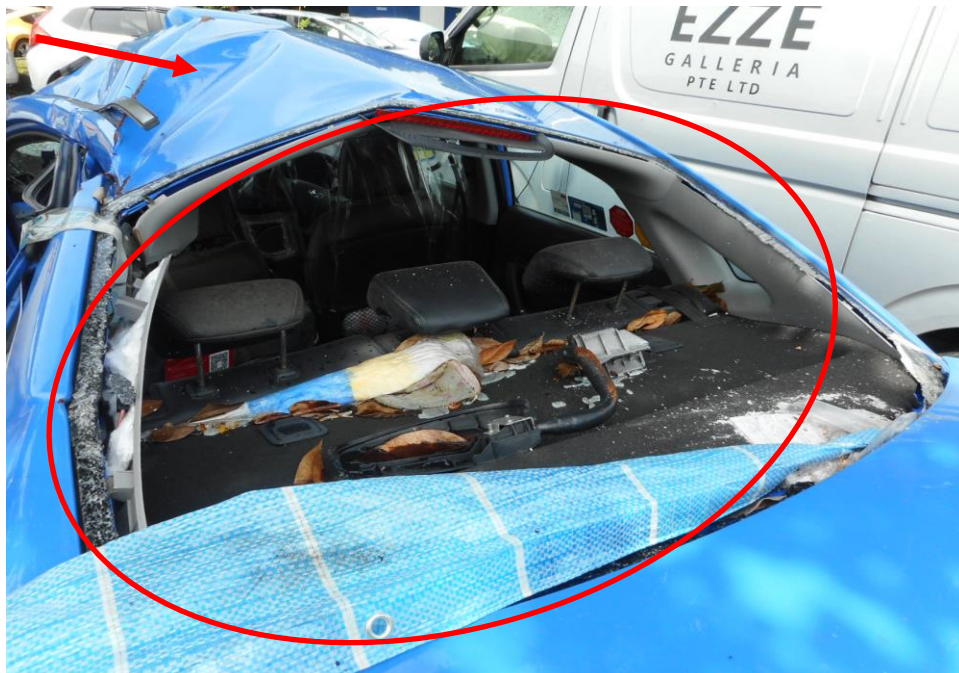
Photo 8 shows the close up view of the Motor Taxi's top and rear portion at the time of my inspection. The Motor Taxi was observed to sustained damage at its rear and roof portion. Its roof (arrowed) and rear windscreen (circled), were amongst the body parts that were damaged as a result of the accident.
