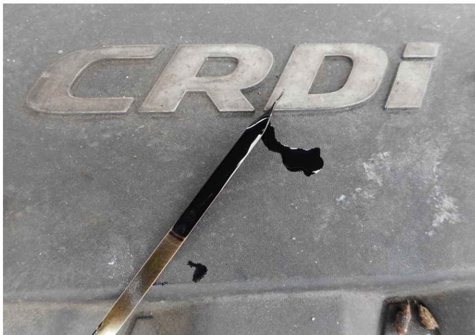
Photo 17 shows the engine oil dip stick of the Motor Taxi at the time of my inspection. The engine oil was observed to be of sufficient level and without any visible contamination.
