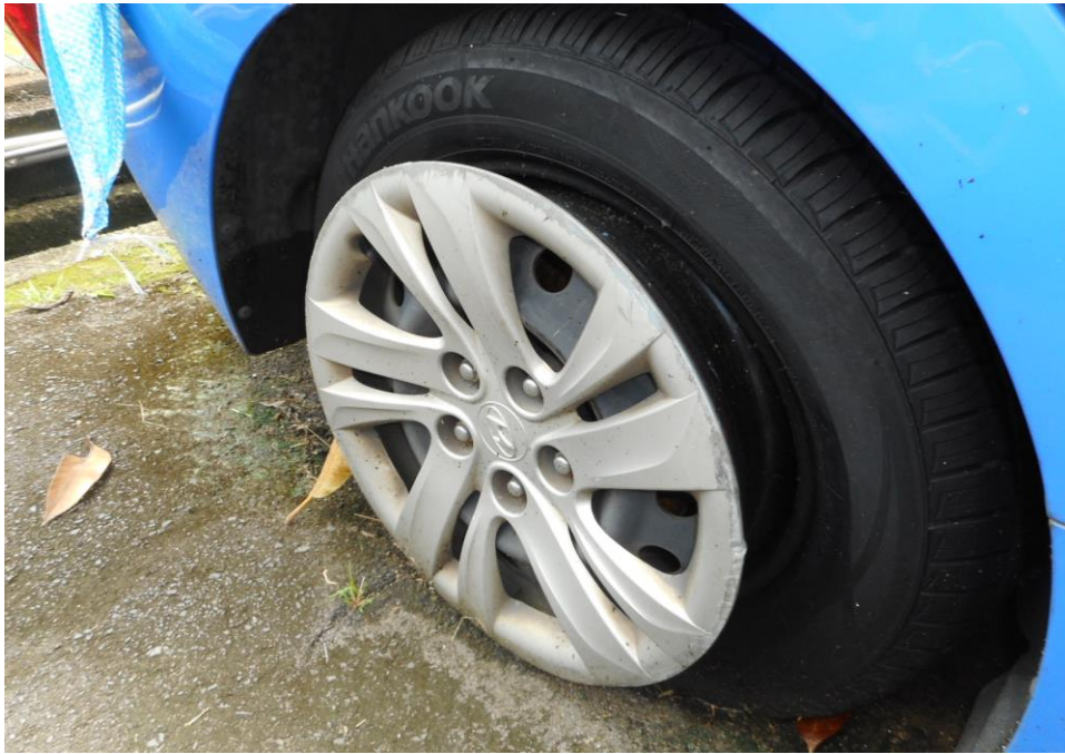
Photo 11 shows the condition of the rear right tyre of the Motor Taxi, which was observed to slip off the rim as a result of the accident. The remaining tread depth of approximately 6.7mm. The tyre was observed to be deflated with no tear, cut or burst mark(s).
