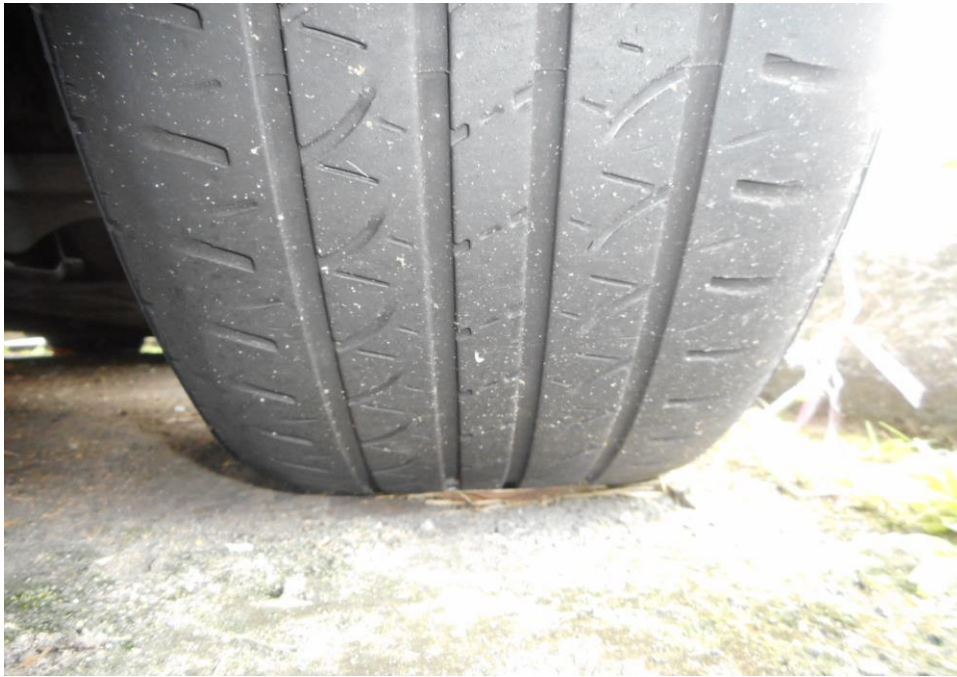
Photo 13 shows the condition of the front left tyre of the Motor Taxi, which was observed to be in serviceable condition with remaining tread depth of approximately 2.9mm. There was also no tear, cut or burst mark(s) on the outer and the inner sidewalls as well as across the tread of the Motor Taxi's 4 tyres.
