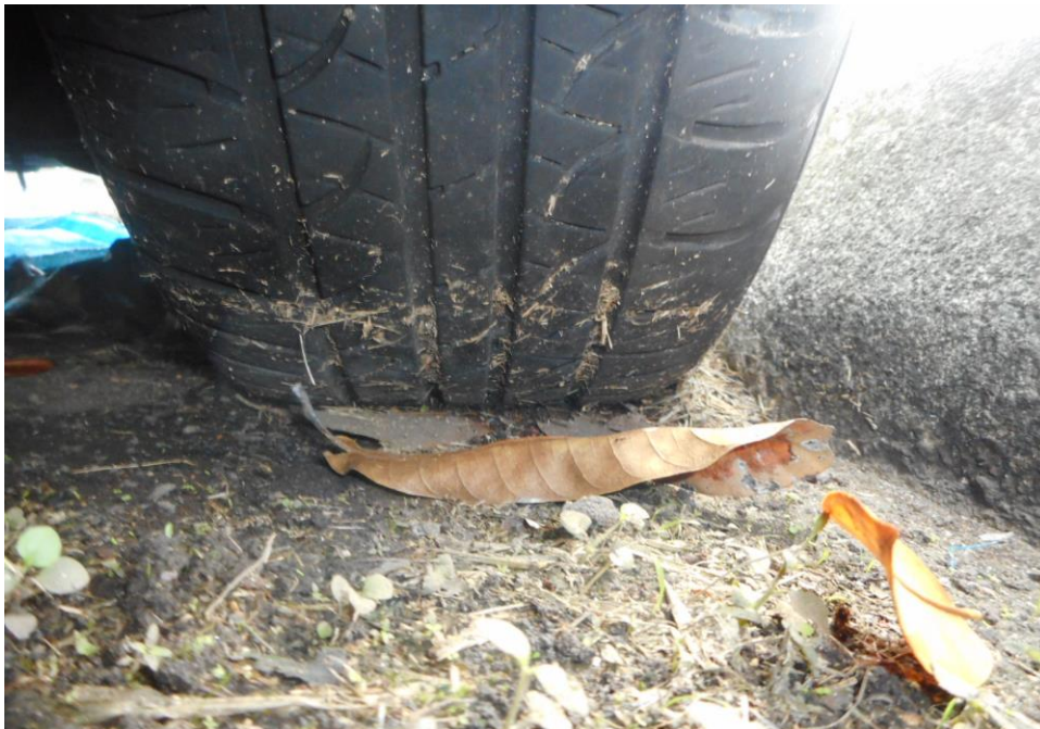
Photo 12 shows the condition of the rear left tyre of the Motor Taxi, which was observed to be in serviceable condition with remaining tread depth of approximately 4.6mm. The tyre, which was wrapped around steel wheel rim, was also observed to be sufficiently inflated for vehicular operation.
