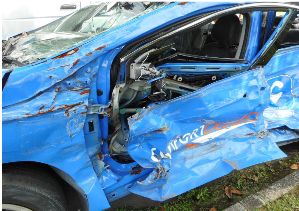
Photo 6 shows a close up view of the Motor Taxi's left body at the time of my inspection. The Motor Taxi was observed to sustained damage at its left portion. Its left front door body panel were amongst the body parts that were damaged as a result of the accident.
