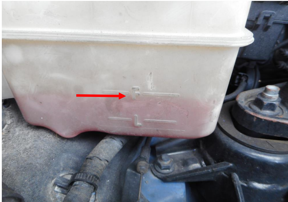
Photo 16 shows checks being carried out to the engine coolant of the Motor Taxi at the time of my inspection. The engine coolant was observed to be of sufficient level (arrowed) and without any visible contamination.
