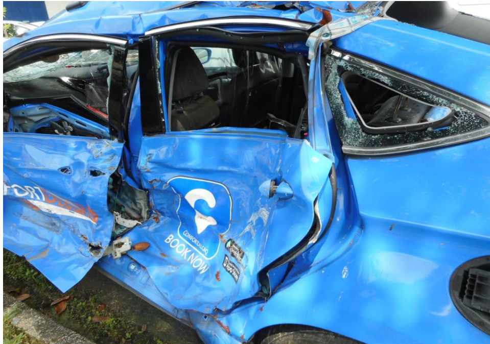
Photo 7 shows a close up view of the Motor Taxi's left body at the time of my inspection. The Motor Taxi was observed to sustained damage at its left portion. Its left rear door body panel were amongst the body parts that were damaged as a result of the accident.
