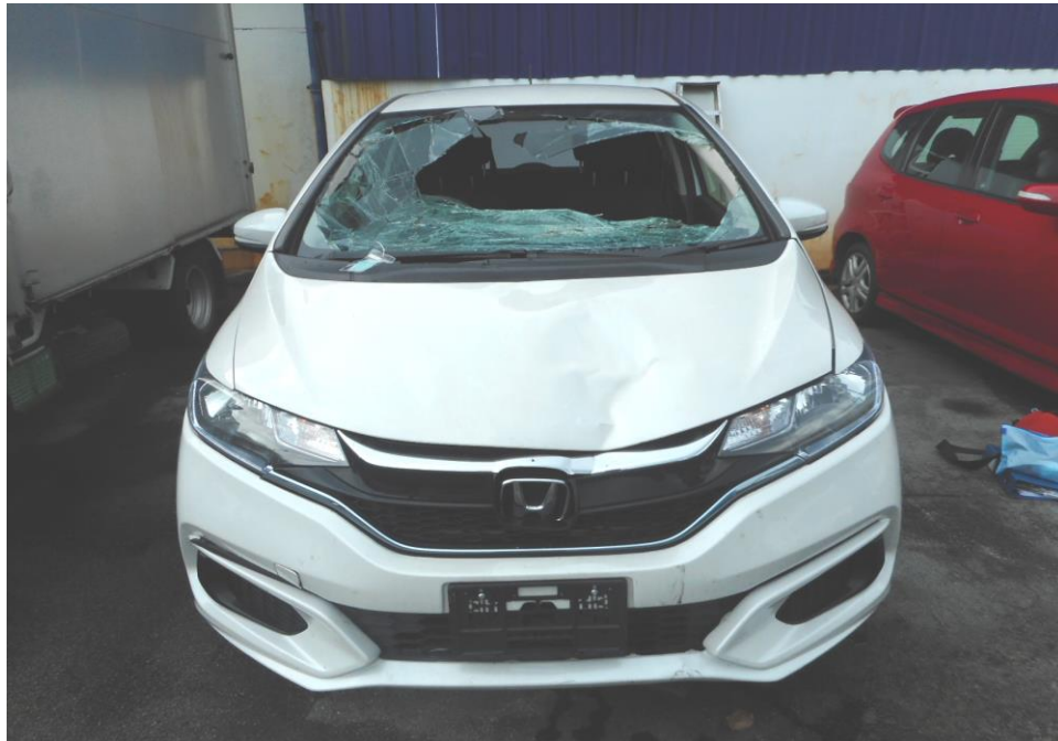
Photo 3 shows a general view of the Motor Car's front body at the time of my inspection. Its front windscreen, front bonnet, front grille, front number plate and front bumper was amongst the body parts that were damaged as a result of the accident.
