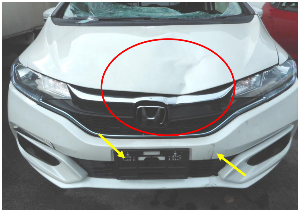
Photo 5 shows the close up view of the Motor Car's front body at the time of my inspection. The Motor Car was observed to have sustained damage at its front bonnet, front grille (circled), front number plate and front bumper (arrowed) was amongst the body parts that were damaged as a result of the accident.
