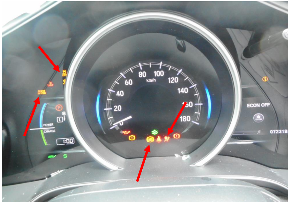
Photo 24 shows the warning light for Anti-Lock Brake System (ABS) and Power Steering System (EPS), Supplemental Restraint System (SRS) and Traction Control (TC) (arrowed) appearing on the instrument panel of the Motor Car during the self-test of its various electronic operating systems when its engine was cranked.
