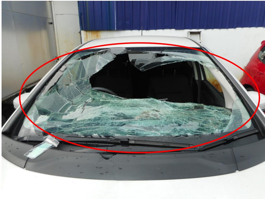
Photo 4 shows the close up view of the Motor Car's front body at the time of my inspection. The Motor Car was observed to have sustained damage at its front windscreen (circled), as a result of the accident.
