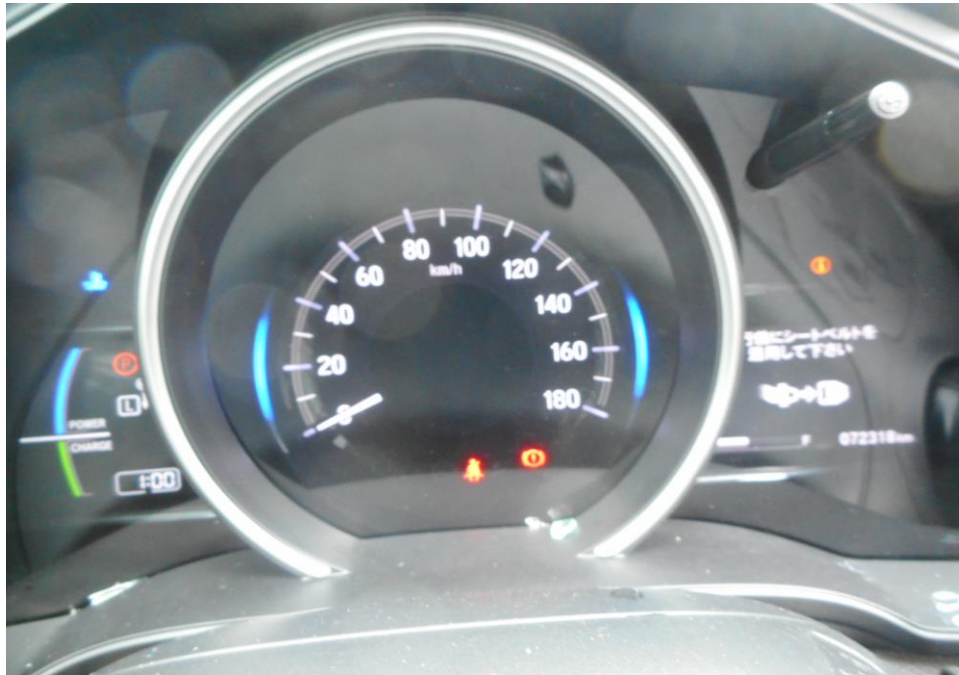
Photo 25 shows no warning lights illuminated on the instrument panel of the Motor Car after the engine was cranked. This would suggest that there was no abnormality to the electronic operating system of the Motor Car, like the ABS, EPS, SRS, and TC etc.
