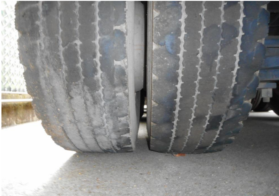
Photo 17 shows the condition of the right tyres of the rear trailer, which was observed to be in serviceable condition with remaining tread depth of approximately 5mm. The tyre, which was wrapped around standard steel wheel rim, was also observed to be sufficiently inflated for vehicular operation.
