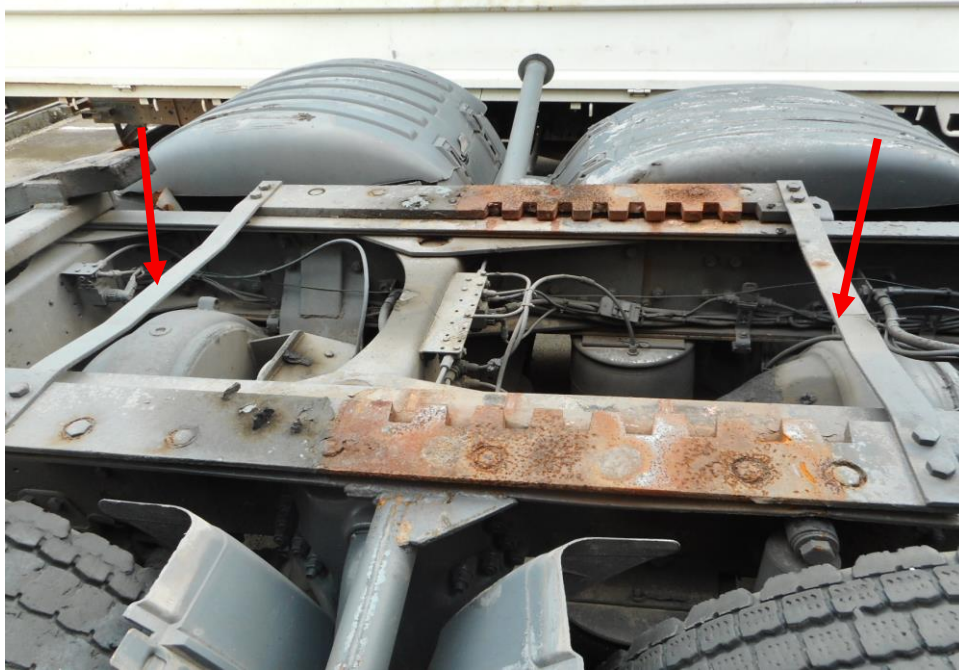
Photo 7 shows a close up view of the Motor Trailer's middle portion at the time of my inspection. The support bars for mounting plate for the middle fifth wheel unit was observed to be bent as a result of the accident.
