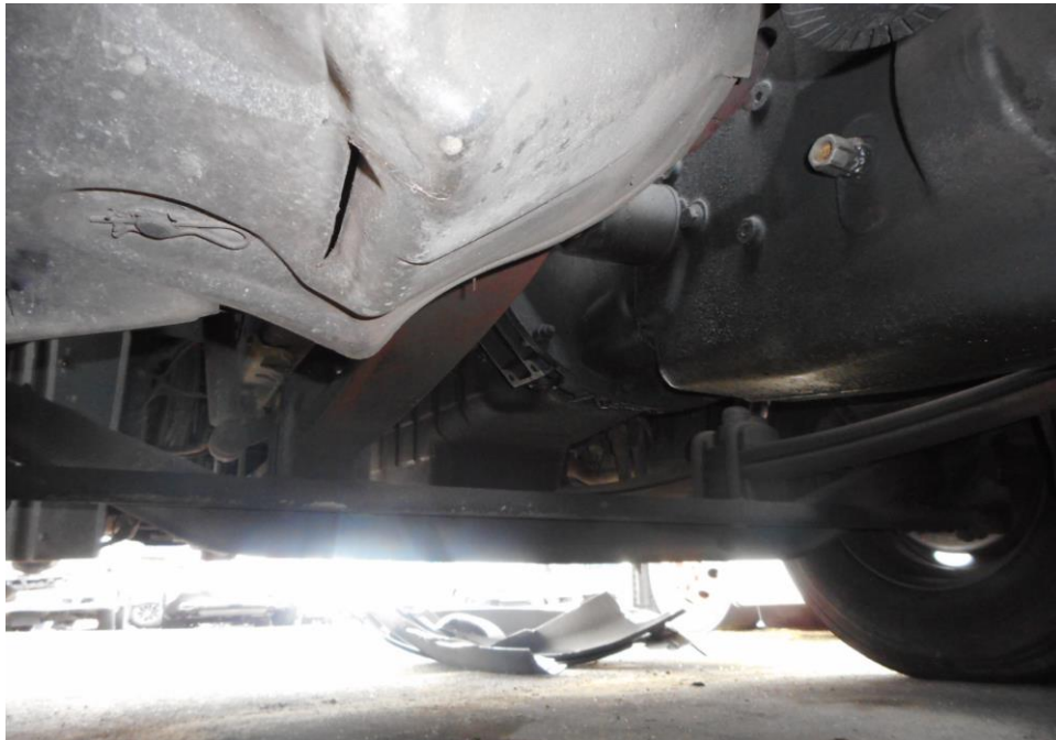
Photo 19 shows the undercarriage of the Motor Trailer, at the area where the engine housing located. I did not find any sign(s) or indication(s) of fluid leak or fluid stain(s) on the underside of the Motor Trailer.
