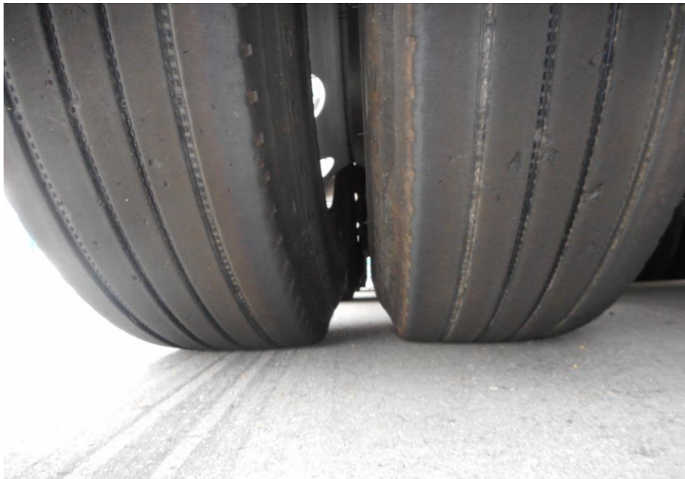
Photo 18 shows the condition of the left tyres of the rear trailer, which was observed to be in serviceable condition with remaining tread depth of approximately 4.2mm. The tyres, which were wrapped around standard steel wheel rim, were also observed to be sufficiently inflated for vehicular operation. There was also no damage found on all 12 steel wheel rims of the Rear Trailer.
