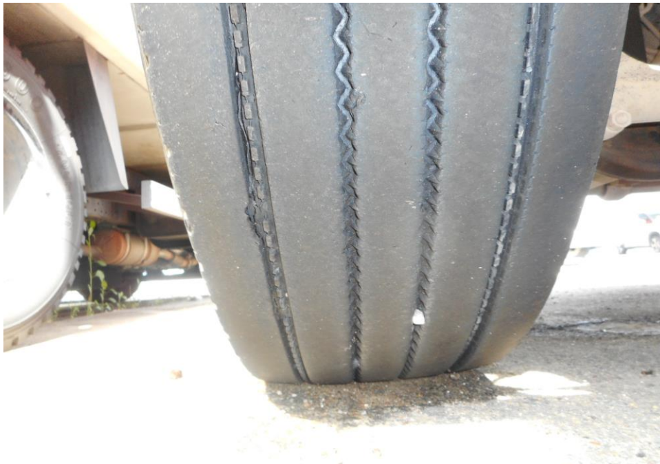
Photo 16 shows the condition of the front left tyres of the Motor Trailer, which were observed to be in serviceable condition with remaining tread depth of approximately 8.5mm. There was also no tear, cut or burst mark(s) on the outer and the inner sidewalls as well as across the tread of the 10 tyres that were fitted on the Motor Trailer.
