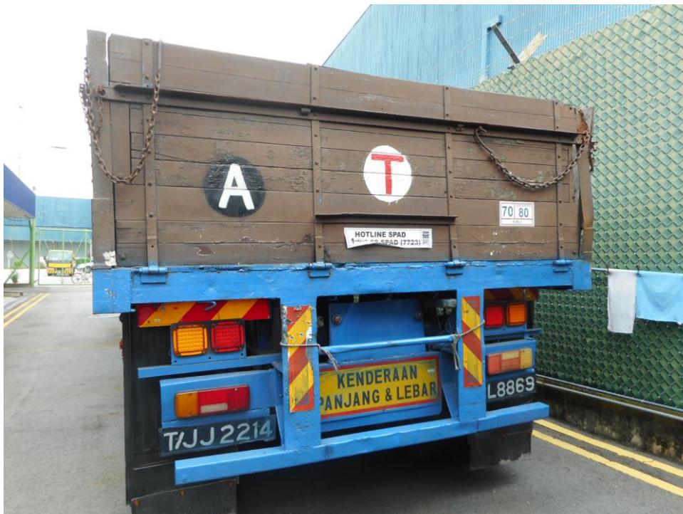
Photo 12 shows a general view of the rear body of the trailer at the time of my inspection. The Motor Trailer's rear body was observed to be intact and unaffected by the accident.
