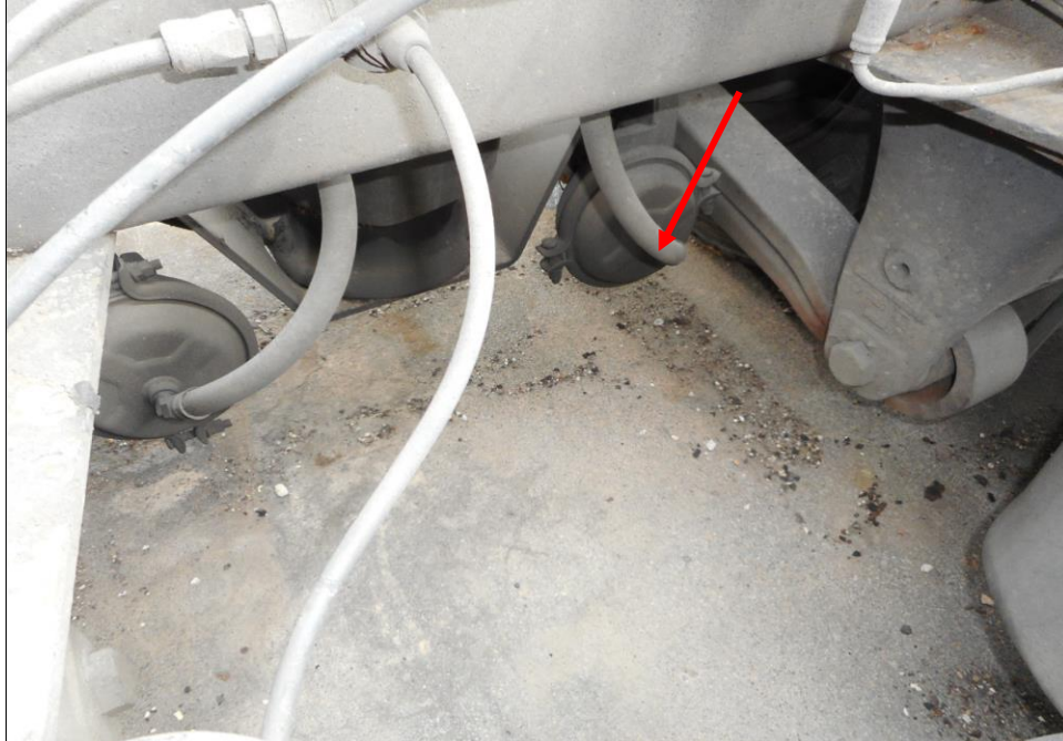
Photo 24 shows the brake pipe (arrowed) at the rear right wheel of the Motor Trailer. I did not observe any leakage of brake fluid at the time of my inspection of the Motor Trailer. My visual examination of the various mechanical components in the braking system, had indicated that there was no internal leakage of pressure/vacuum and were generally intact to suggest that its braking system was in serviceable condition at the material time of accident.
