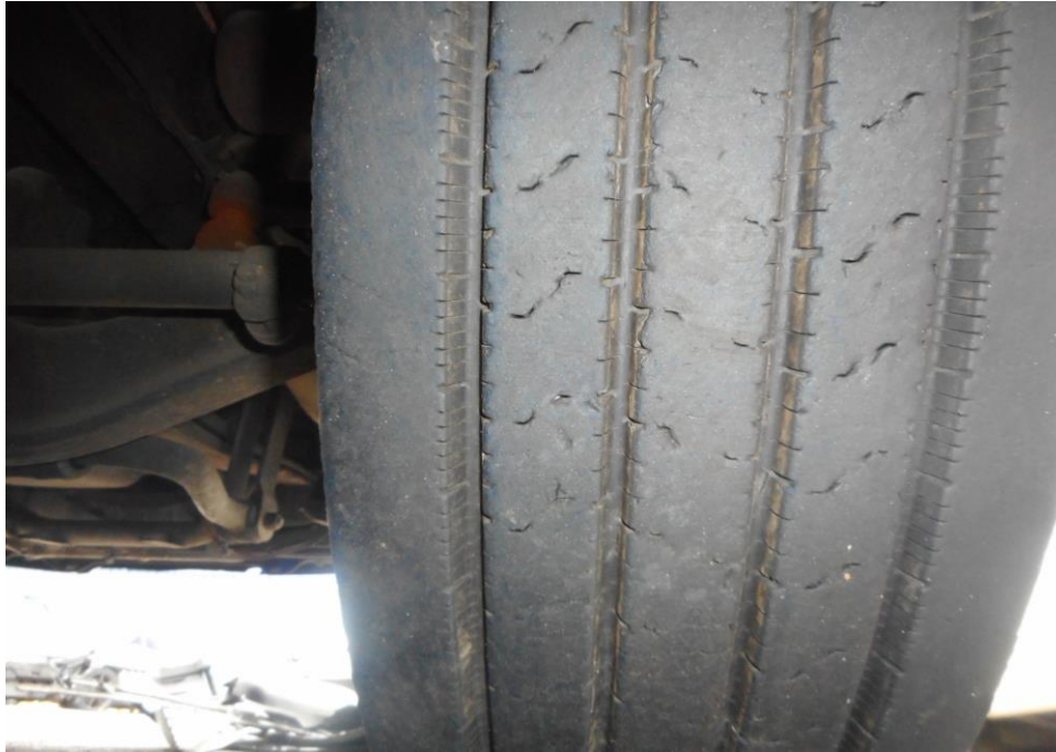
Photo 13 shows the condition of the front right tyre of the Motor Trailer, which was observed to be in serviceable condition with remaining tread depth of approximately 8.9 mm. The tyre, which was wrapped around standard steel wheel rim, was also observed to be sufficiently inflated for vehicular operation. There was no tear, cut or burst mark(s) on the outer and the inner sidewalls as well as across the tread of the 10 tyres that were fitted on the Motor Trailer.
