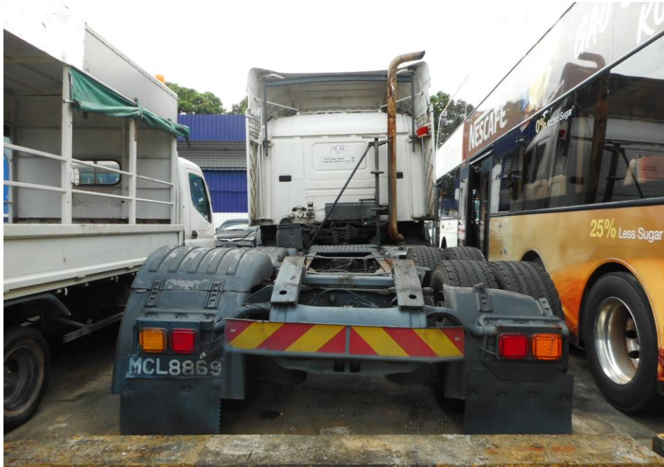
Photo 5 shows a general view of the Motor Trailer's middle chassis portion at the time of my inspection. The Motor Trailer middle chassis was bent and had slanted to the right side and its middle fifth wheel unit was observed to be missing from the middle chassis as a result of the accident.
