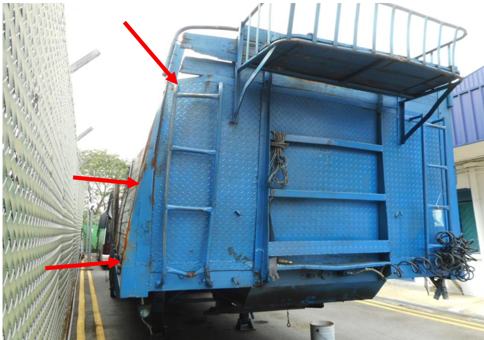
Photo 10 shows a general view of the rear trailer's right body at the time of my inspection. The Motor Trailer's right body panel was observed to sustained damage as a result of the accident.
