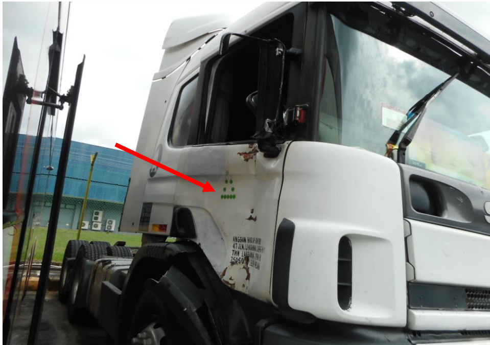
Photo 3 shows a close up view of the right body of the Motor Trailer at the time of my inspection. The Motor Trailer was observed to sustain damage at its right door (arrowed) as a result of the accident.
