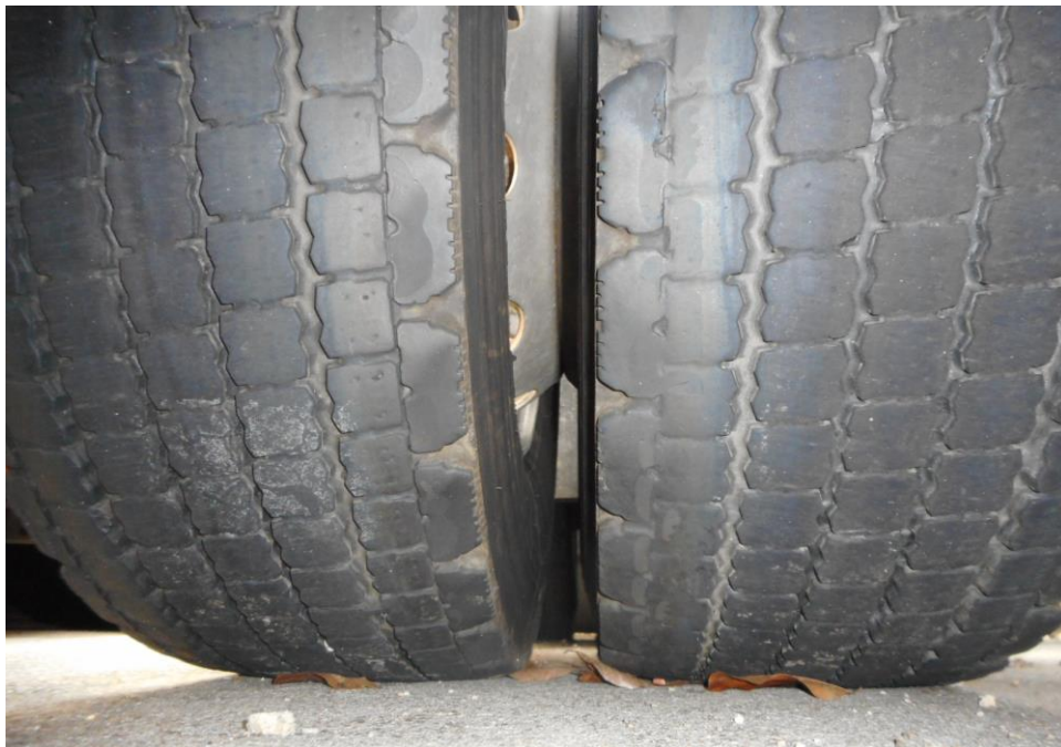
Photo 14 shows the condition of the rear right tyre of the Motor Trailer, which was observed to be in serviceable condition with remaining tread depth of approximately 7.4mm. The tyre, which was wrapped around standard steel wheel rim, was also observed to be sufficiently inflated for vehicular operation.
