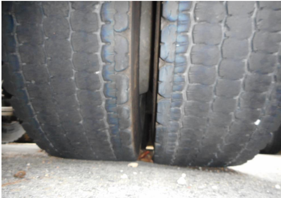
Photo 15 shows the condition of the rear left tyres of the Motor Trailer, which was observed to be in serviceable condition with remaining tread depth of approximately 4.8mm. The tyres, which were wrapped around standard steel wheel rim, were also observed to be sufficiently inflated for vehicular operation. There was also no damage found on all 10 steel wheel rims of the Motor Trailer.
