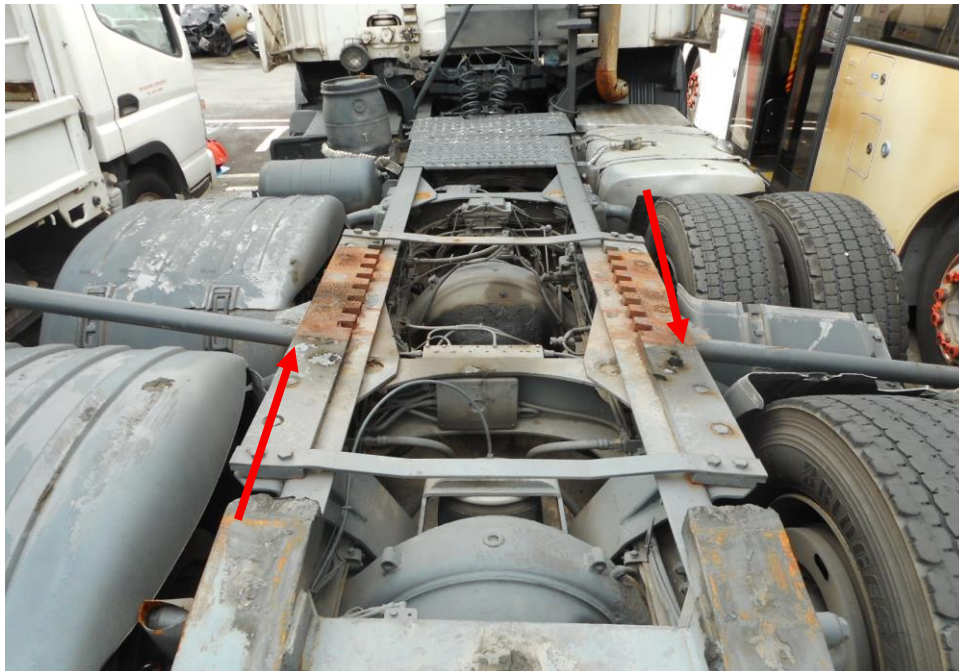
Photo 6 shows a close up view of the Motor Trailer's middle portion at the time of my inspection. The Motor Trailer middle chassis was bent and had slanted to the right side (arrowed); its fifth wheel unit was also observed to be missing as a result of the accident.
