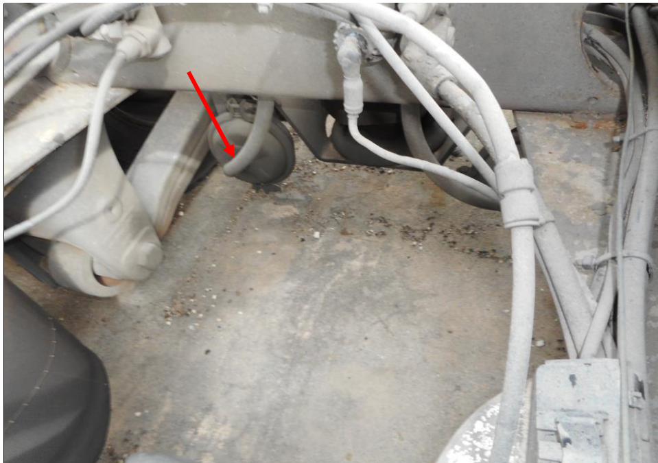
Photo 23 shows the brake pipe (arrowed) at the rear left wheel of the Motor Trailer. I did not observe any leakage of brake fluid at the time of my inspection of the Motor Trailer. My visual examination of the various mechanical components in the braking system, had indicated that there was no internal leakage of pressure/vacuum and were generally intact to suggest that its braking system was in serviceable condition at the material time of accident.
