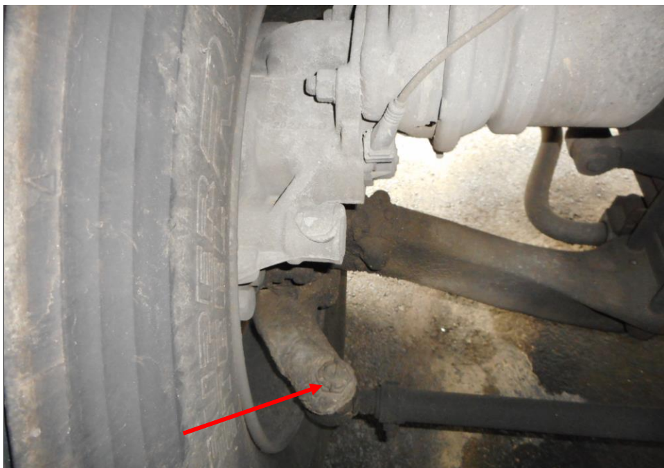
Photo 22 shows the various undercarriage components at the front left wheel of the Motor Trailer, in particular the steering tie rod end (arrowed). The various undercarriage components of the Motor Trailer were all found to be intact without any visible damage. There was also no sign of fluid stain(s) observed on the various undercarriage components to indicate that the Motor Trailer's steering system was in serviceable condition.
