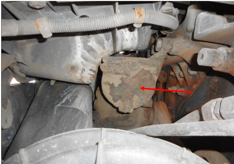
Photo 20 shows the front underside of the Motor Trailer. I was not able to conduct any test(s) on the steering system of the Motor Trailer as the engine of the Motor Trailer could not be started. However, my visual checks on the various mechanical components of the steering system like the steering box, steering shaft and steering linkages (arrowed) amongst others revealed all to be intact
