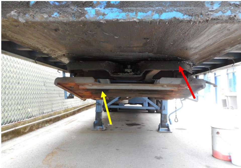
Photo 8 shows a general view of the rear Trailer undercarriage at the time of my inspection. We observed that the fifth wheel unit (red arrow) and the base plate (yellow arrow) that was supposedly mounted on the Motor Trailer had detached and stayed on the rear Trailer after the accident.
