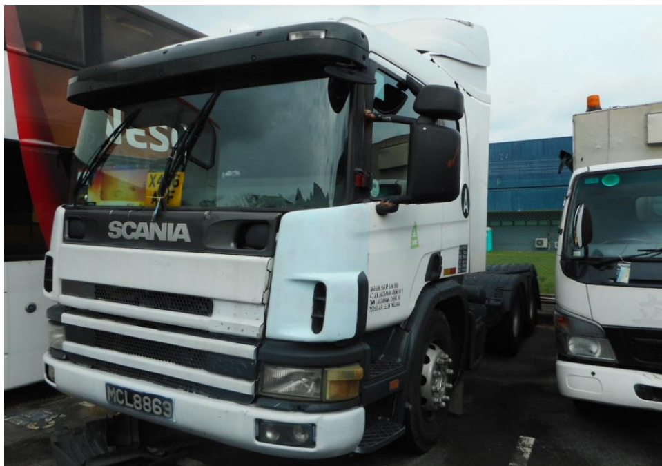
Photo 4 shows a general view of the left body of the Motor Trailer at the time of my inspection. The Motor Trailer left body was observed to be intact and unaffected by the accident.
