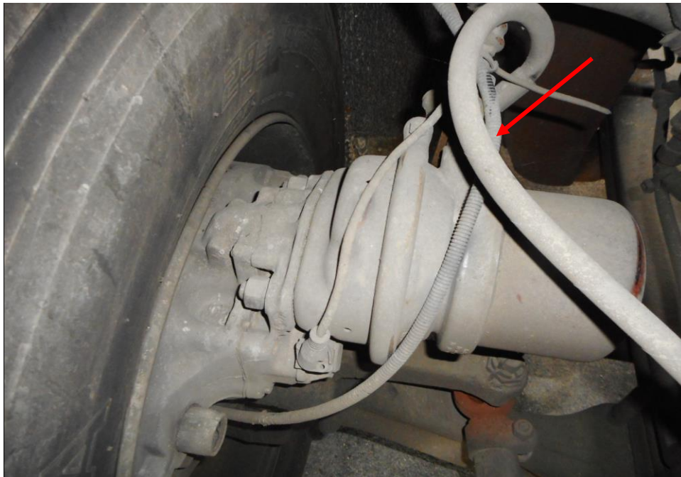
Photo 25 shows the brake pipe (arrowed) at the front right wheel of the Motor Trailer. I did not observe any leakage of brake fluid at the time of my inspection of the Motor Trailer. My visual examination of the various mechanical components in the braking system, had indicated that there was no internal leakage of pressure/vacuum and were generally intact to suggest that its braking system was in serviceable condition at the material time of accident.
