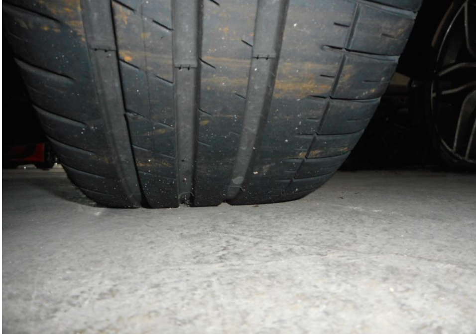
Photo 6 shows the condition of the front right tyre of the Motor Car, which was observed to be in serviceable condition with remaining tread depth of approximately 3.2mm. The tyre was sufficiently inflated for vehicular operation with no tear, cut or burst mark(s) on the outer and the inner sidewalls as well as across the tread. The 4 tyres of the Motor Car were wrapped around standard steel wheel rims without any damage.
