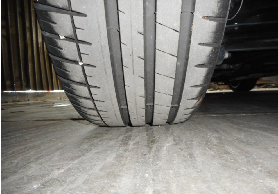
Photo 8 shows the condition of the rear left tyre of the Motor Car, which was observed to be in serviceable condition with remaining tread depth of approximately 5.2mm. The tyre, which was wrapped around alloy wheel rim, was also observed to be sufficiently inflated for vehicular operation. The 4 tyres of the Motor Car were wrapped around standard steel wheel rims.
