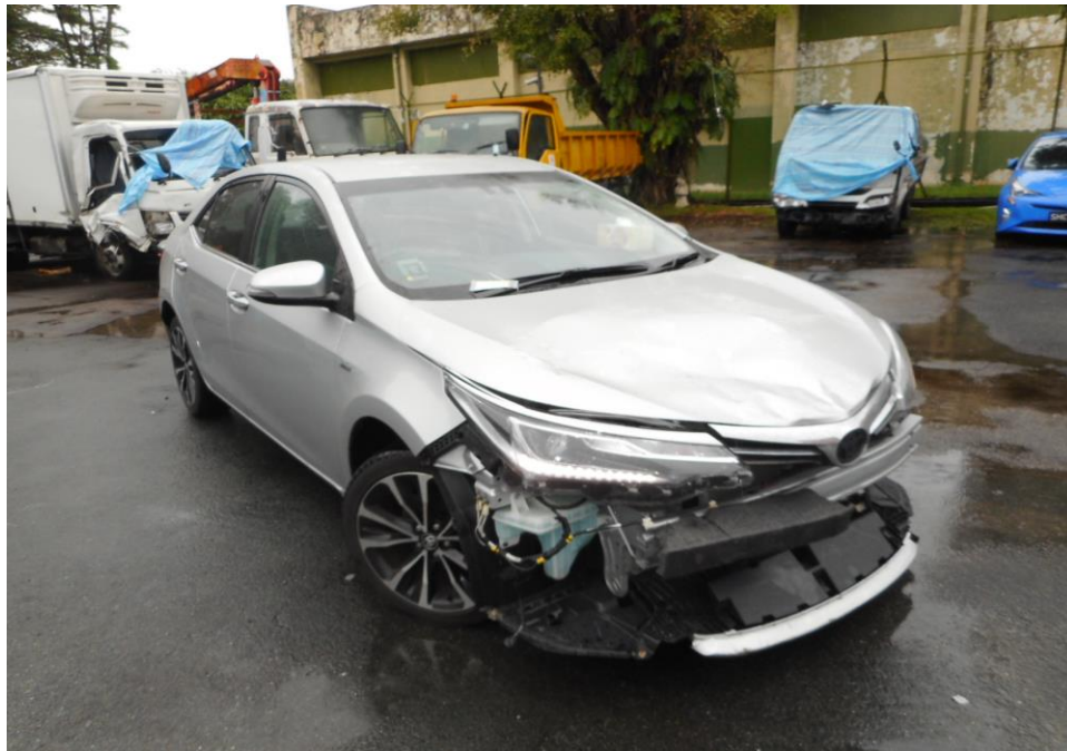
Photo 19 shows the front right wheel of the Motor Car turned to its full left. During my steering system test, I did not experience any abnormal free play and/or resistance when I had turned the steering wheel towards the left and right. This would suggest that the steering system of the Motor Car was likely to be in serviceable condition at the material time of accident.
