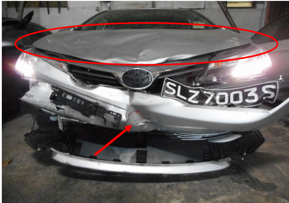
Photo 2 shows a general view of the Motor Car's front body at the time of my inspection. Its front bonnet (circled) and front bumper (arrowed) were the body parts that were damaged as a result of the accident.
