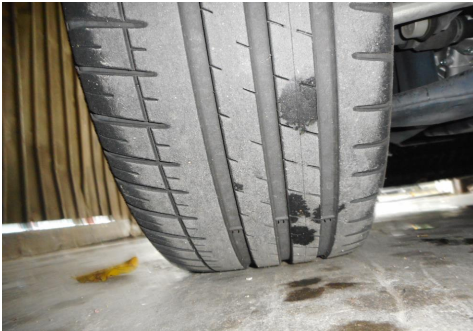
Photo 9 shows the condition of the front left tyre of the Motor Car, which was observed to be in serviceable condition with remaining tread depth of approximately 3.8mm. The tyre was sufficiently inflated for vehicular operation with no tear, cut or burst mark(s) on the outer and the inner sidewalls as well as across the tread. The 4 tyres of the Motor Car were wrapped around standard alloy wheel rims without any damage.
