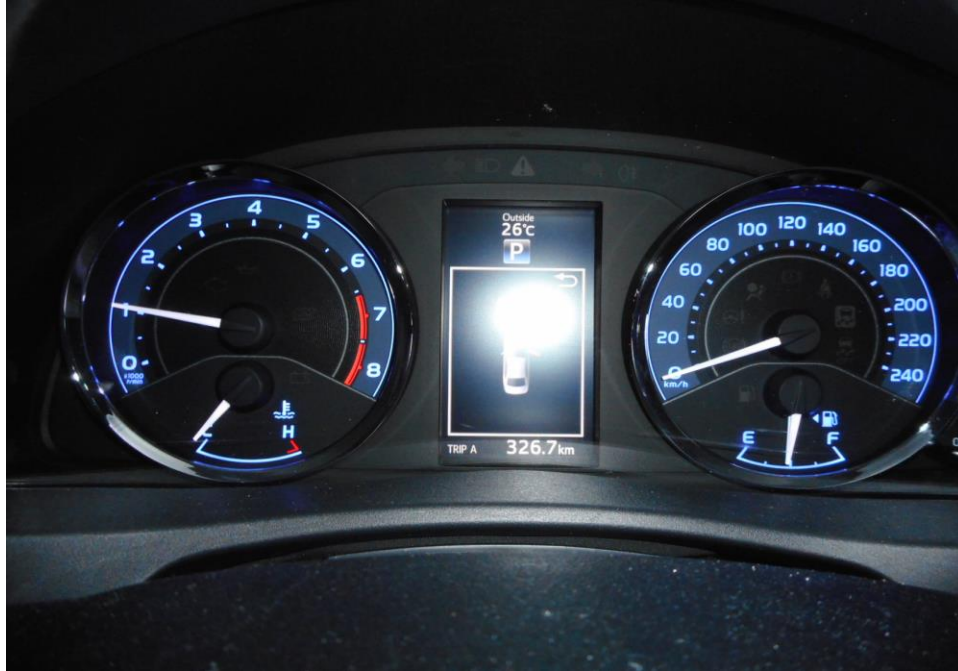
Photo 23 shows no warning lights illuminated on the instrument panel of the Motor Car after the engine was cranked. This would suggest that there was no abnormality to the various electronic operating systems of the Motor Car, like the ABS, SRS and TCS.
