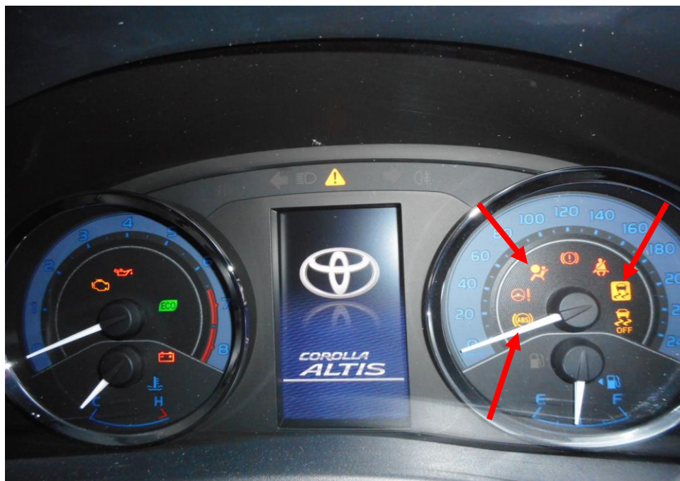
Photo 22 shows the warning light for Anti-Lock Brake System (ABS), Traction Control System (TCS) and Supplemental Restraint System (SRS) (arrowed) appearing on the instrument panel of the Motor Car during the self-test of its various electronic operating systems when its engine was cranked.
