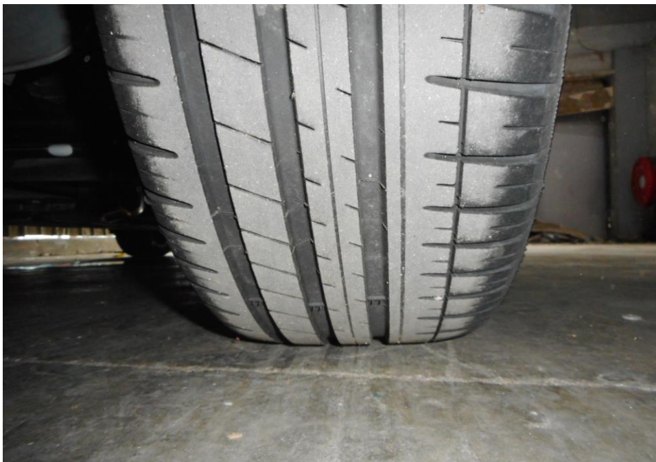
Photo 7 shows the condition of the rear right tyre of the Motor Car, which was observed to be in serviceable condition with remaining tread depth of approximately 5.5mm. The tyre was also observed to be sufficiently inflated for vehicular operation with no tear, cut or burst mark(s).
