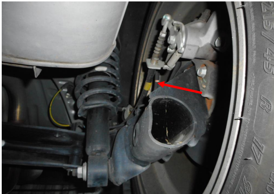
Photo 15 shows the brake hose/pipe (arrowed) at the rear right wheel of the Motor Car. No leakage of brake fluid was observed. Visual examination of the various components of the braking system like the brake caplier, brake booster, brake pedal etc. had revealed all to be intact and without visible damage.
