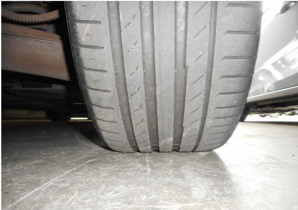
Photo 8 shows the condition of the rear right tyre of the Motor Car, which was observed to be in serviceable condition with remaining tread depth of approximately 2.5mm. The tyre was also observed to be sufficiently inflated for vehicular operation with no tear, cut or burst mark(s).
