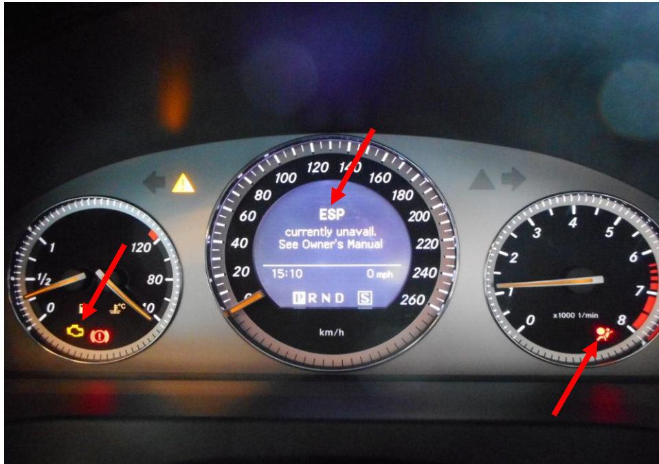
Photo 25 shows the Supplemental Restraint System (SRS), Electronic Stability System (ESP) and Engine warning light remained illuminated up on the instrument panel of the Motor Car after the engine was cranked. This is likely due to the result of the accident.
