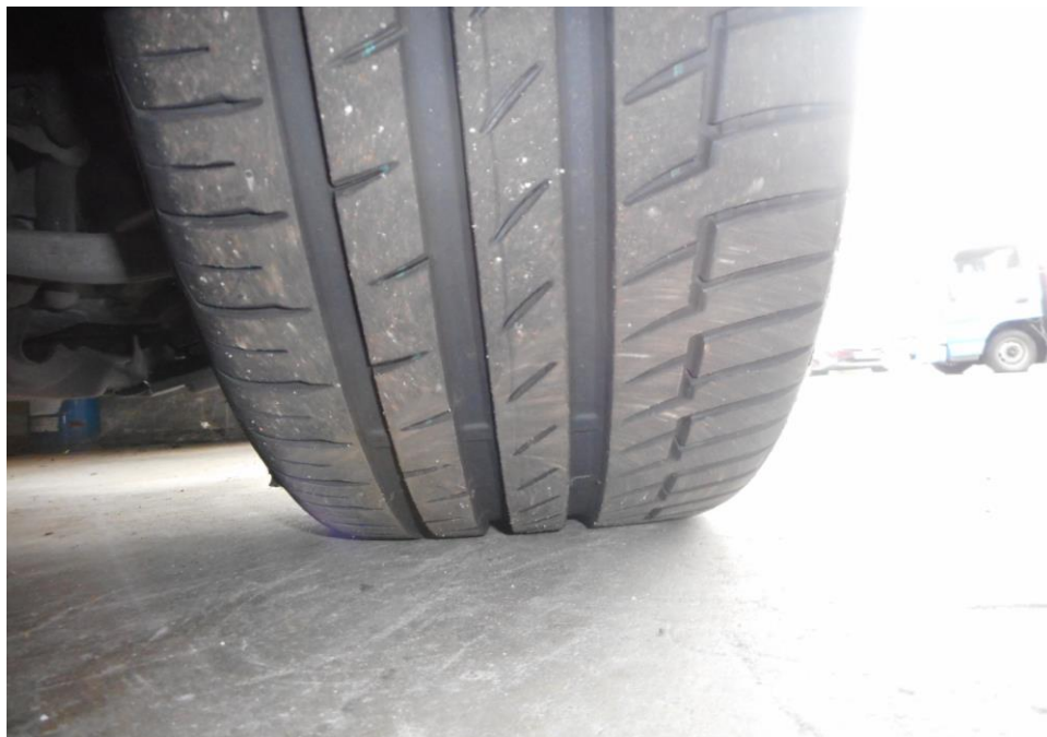
Photo 7 shows the condition of the front right tyre of the Motor Car, which was observed to be in serviceable condition with remaining tread depth of approximately 6.7mm. The tyre was sufficiently inflated for vehicular operation with no tear, cut or burst mark(s) on the outer and the inner sidewalls as well as across the tread. The 4 tyres of the Motor Car were wrapped around standard steel wheel rims without any damage.
