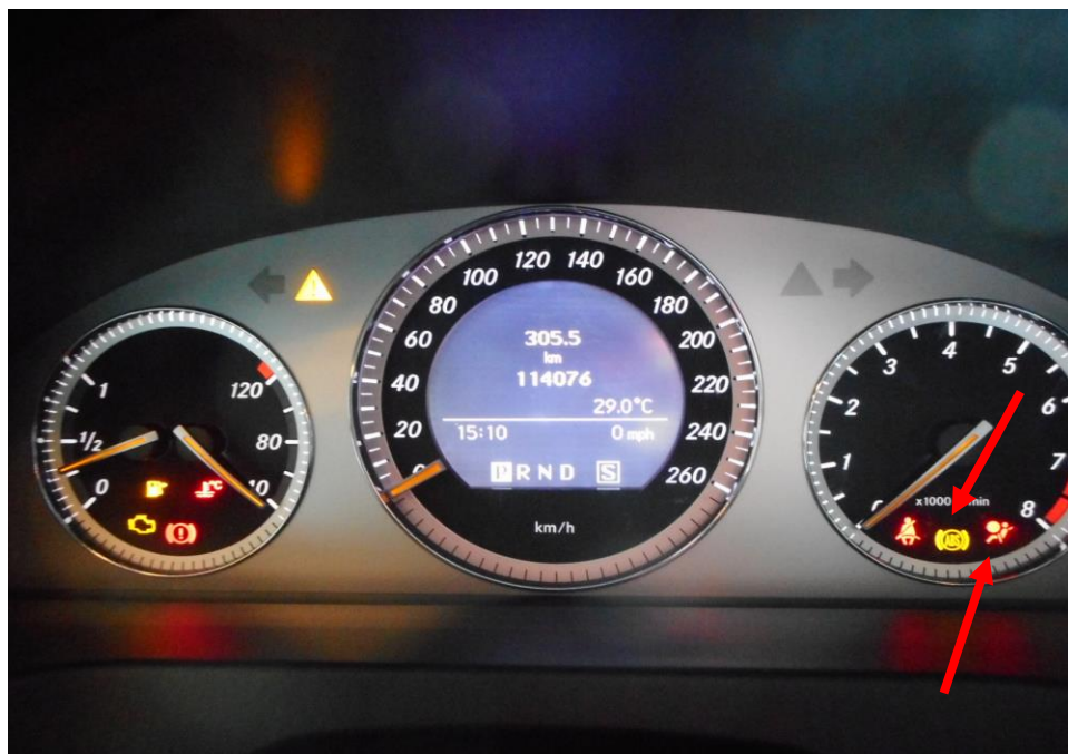
Photo 24 shows the warning light for Anti-Lock Brake System (ABS) Supplemental Restraint System (SRS) (arrowed) appearing on the instrument panel of the Motor Car during the self-test of its various electronic operating systems when its engine was cranked.
