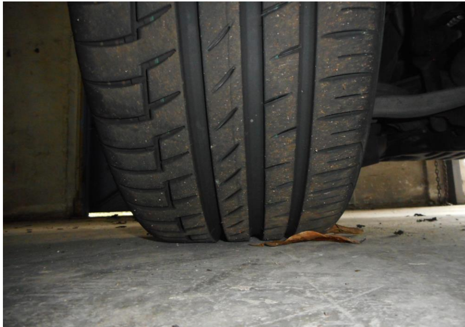
Photo 10 shows the condition of the front left tyre of the Motor Car, which was observed to be in serviceable condition with remaining tread depth of approximately 6.1mm. There was also no tear, cut or burst mark(s) on the outer and the inner sidewalls as well as across the tread of the Motor Car's 4 tyres.
