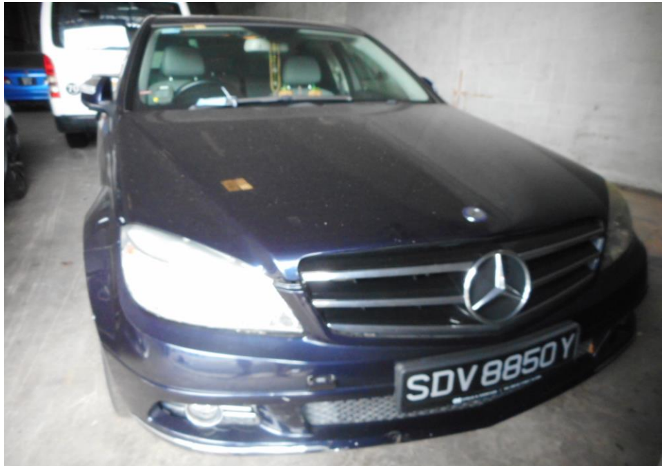
Photo 2 shows a general view of the Motor Car's front body at the time of my inspection. The front portion of the Motor Car was observed to have sustained damage. Its front bumper was the body part that were damaged as a result of the accident.
