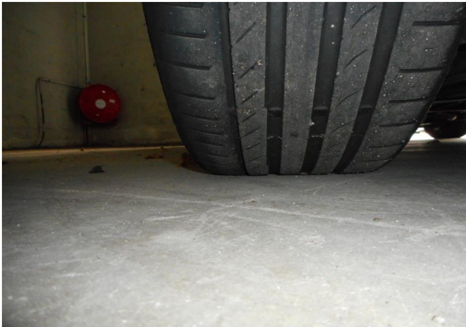
Photo 9 shows the condition of the rear left tyre of the Motor Car, which was observed to be in serviceable condition with remaining tread depth of approximately 2.5mm. The tyre, which was wrapped around steel wheel rim, was also observed to be sufficiently inflated for vehicular operation. The 4 tyres of the Motor Car were wrapped around standard steel wheel rims.
