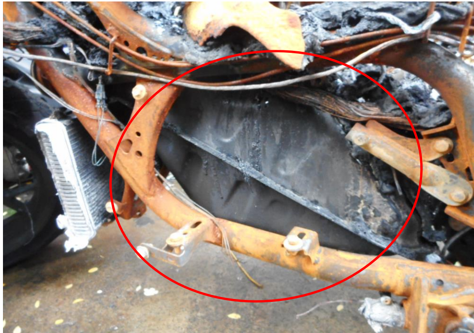
Photo 7 shows the general view of the fuel tank (circled) of the Insured Motorcycle partially burnt and/or melted as a result of the fire.
