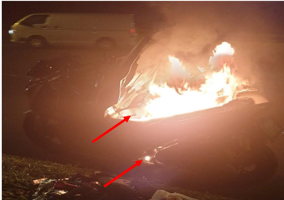
Photo 13 shows the flames started engulfing the centre part of the Insured Motorcycle at the incident scene. The fire could be seen burning from the seat and the engine below (arrowed) of the Insured Motorcycle
