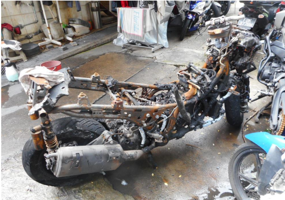
Photo 1 shows the general view of the right of the Insured Motorcycle at the time of inspection. The Insured Motorcycle was observed to have sustained severe fire damage all around. Its front and rear number plate, front fairings; handle bar assembly, instrument panel, fuel tank, engine and seats amongst others that were found to have been affected as a result of the fire.
