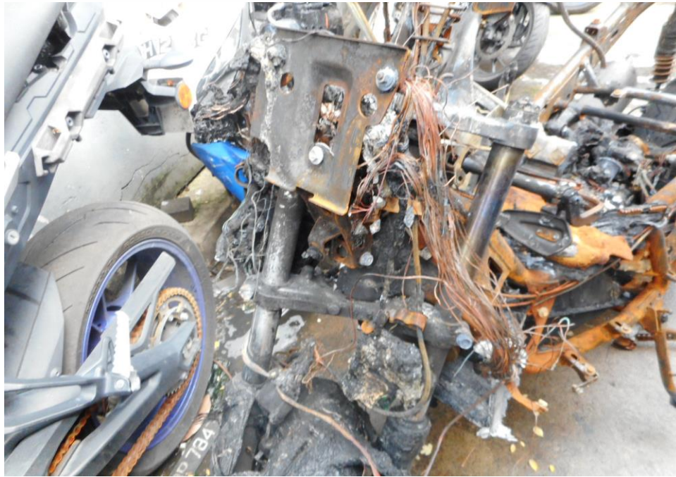
Photo 5 shows the front number plate and fairings of the Insured Motorcycle had been burnt and/or melted as a result of the fire.
