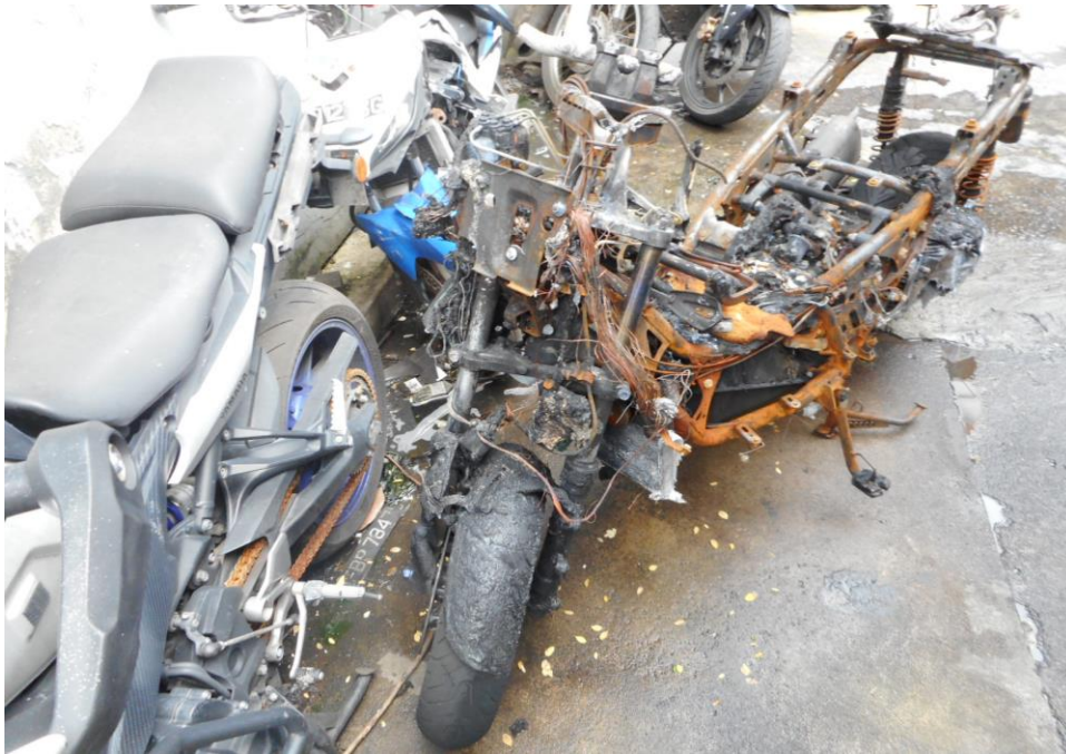
Photo 2 shows the general view of the front of the Insured Motorcycle at the time of inspection. The Insured Motorcycle was observed to have sustained severe fire damage all around. Its front and rear number plate, front fairings; handle bar assembly, instrument panel, fuel tank, engine and seats amongst others that were found to have been affected as a result of the fire.
