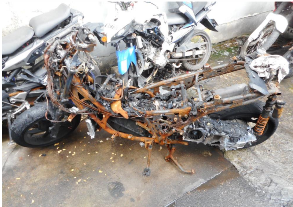
Photo 3 shows the general view of the left side of the Insured Motorcycle at the time of inspection. The Insured Motorcycle was observed to have sustained severe fire damage all around. Its front and rear number plate, front fairings; handle bar assembly, instrument panel, fuel tank, engine and seats amongst others that were found to have been affected as a result of the fire.
