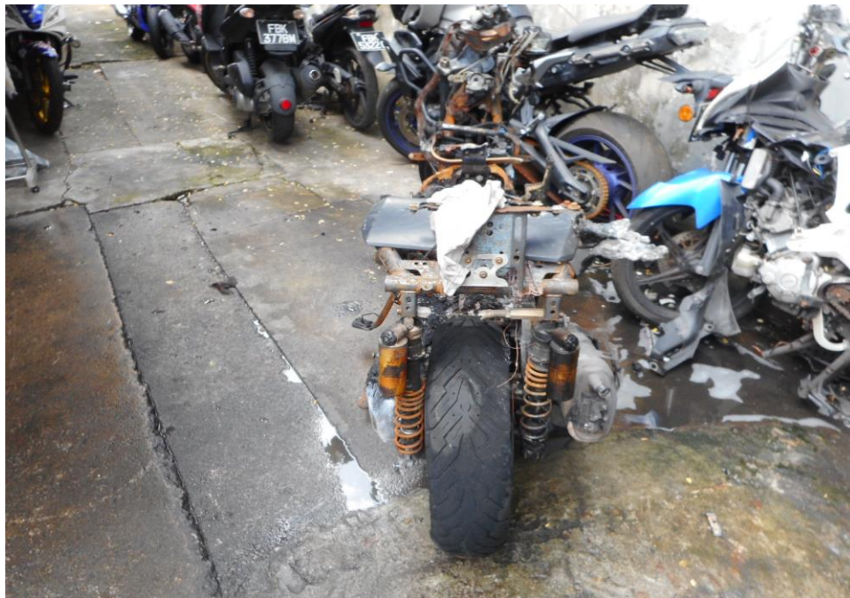
Photo 4 shows the general view of the rear of the Insured Motorcycle at the time of inspection. The Insured Motorcycle was observed to have sustained severe fire damage all around. Its front and rear number plate, front fairings; handle bar assembly, instrument panel, fuel tank, engine and seats amongst others that were found to have been affected as a result of the fire.
