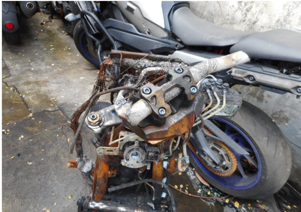
Photo 6 shows the general view of the handle bar assembly and instrument panel of the Insured Motorcycle had been partially burnt and/or melted as a result of the fire.
