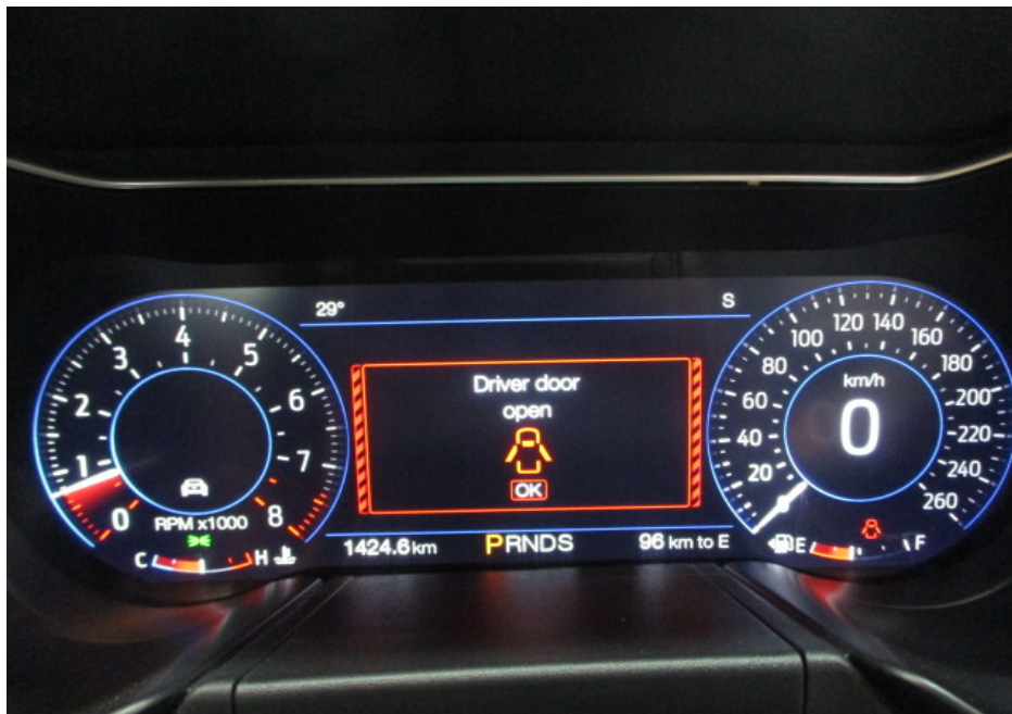
Photo 12 shows the respective warning lights no longer illuminated, indicating that there is no fault detected to the ABS, SRS, TPM and SCS systems of the Motor Car during the self-test. These electronic systems were hence in working condition at the time of my inspection.
