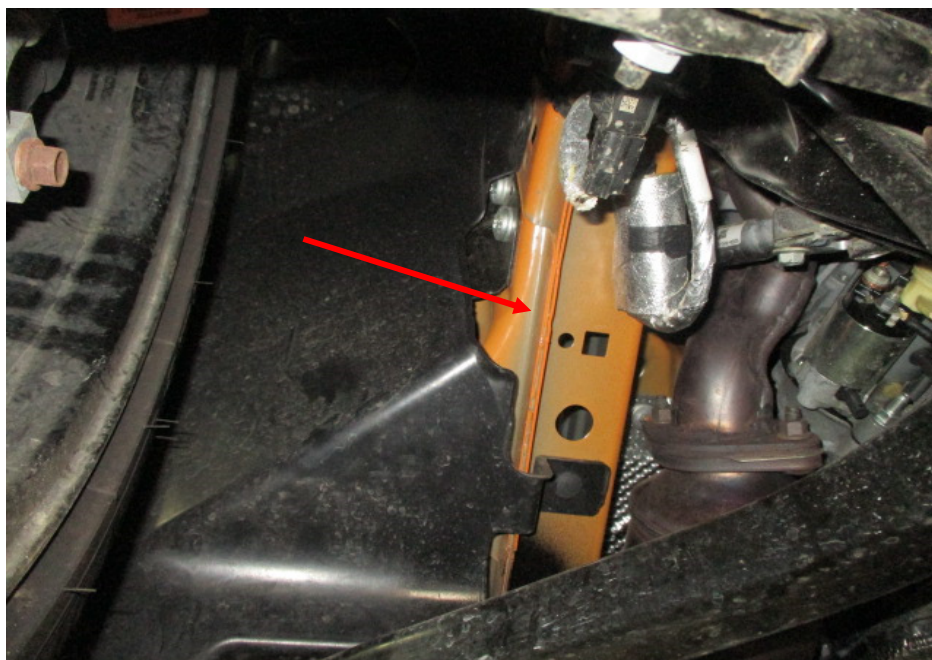
Photo 18 shows the chassis/structural body (arrowed) at the underside front right of the Motor Car. Visually, I did not find any weld marks other than original spot weld marks on the chassis/structural body of the Motor Car. The original factory sealant at the joints along the chassis/structural body was also untouched, indicating no work was done on the chassis/structural body of the Motor Car and that the chassis/structural body was originally fitted.
