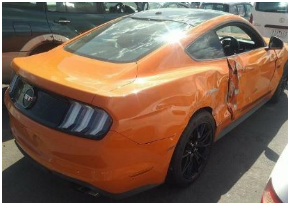
Photo 1 shows the rear right body of the Motor Car prior to any repairs being carried out (photograph provided to me). The Motor Car was observed to have sustained damages at its right centre portion. The body parts observed to be damaged had included its driver's door and right rear body panel.
