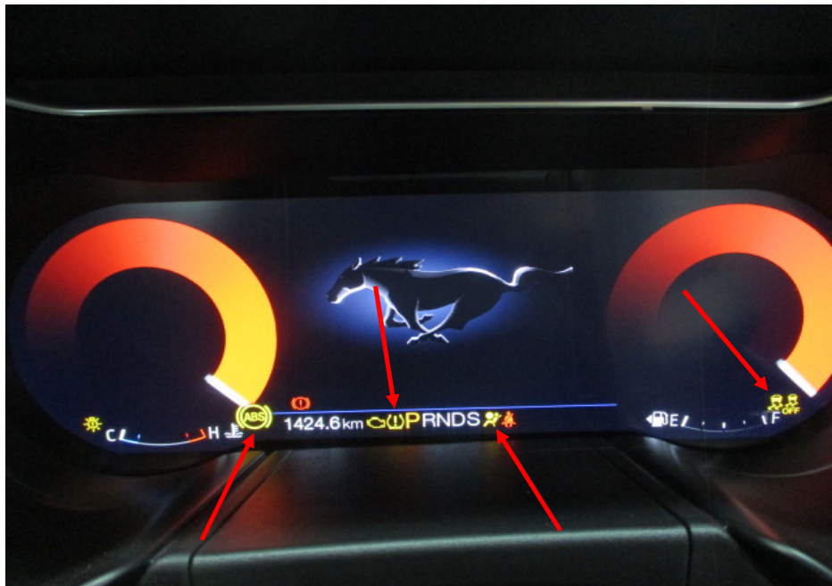
Photo 11 shows the warning lights for the various electronic safety features appearing on the instrument panel of the Motor Car during its self-test when the engine is cranked, in particular the ABS, SRS, TPM and SCS lights (arrowed).
