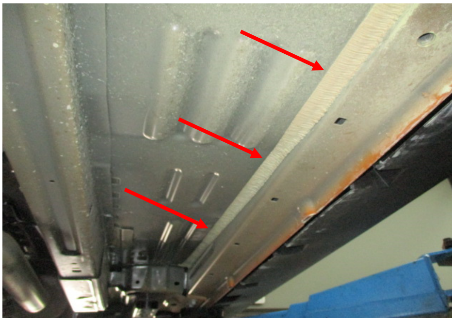
Photo 19 shows the floorboard at the right centre underside of the Motor Car. The original factory sealant (arrowed) at the joints along the floorboard were untouched, indicating that the floorboard of the Motor Car was originally fitted. In general, except for the right rear body panel, I had found all the non-detachable body panels of the Motor Car to be originally fitted at the time of my inspection.
