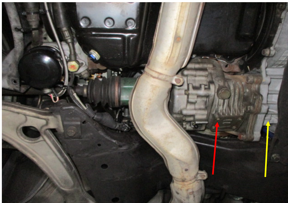
Photo 4 shows the transfer case (red arrow) of the Motor Car. The transfer case is also the output side of the Motor Car's transmission. The gear set in the input side of the transmission (yellow arrow) connects to the transfer case, which is the second of the 2 main housings of the Motor Car's transmission assembly. Drive to the front wheels of the Motor Car is provided via drive shafts that are extended from this transfer case. The transfer case also connects to the propeller shaft, which leads to the rear differential of the Motor Car.
