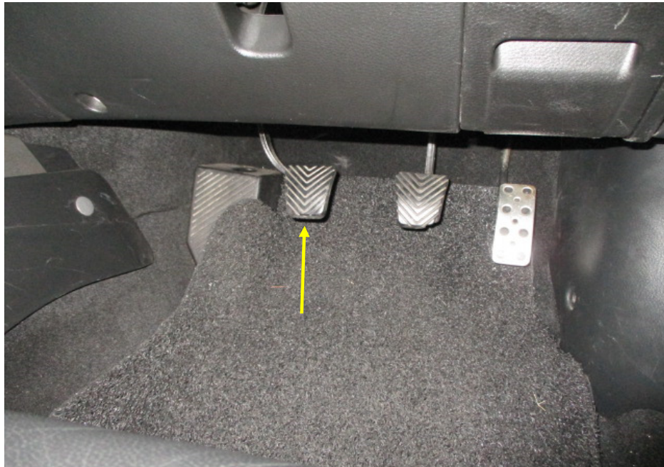
Photo 10 shows the clutch pedal (arrowed) of the Motor Car, for engaging and disengaging the transmission gears.
