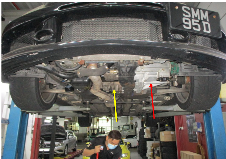
Photo 2 shows a general view of the transmission assembly (red arrow) that was fitted on the Motor Car. This was the input side of the transmission, which houses the main shaft and various gear sets. It is bolted to the crankshaft side of the engine block. The input side of the transmission connects to the transfer case (yellow arrow), which is the output side of the Motor Car's transmission.
