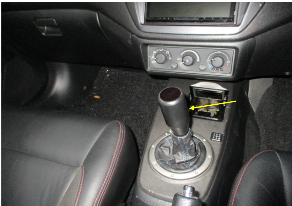
Photo 9 shows the manual gear shifter (arrowed) that was fitted on the Motor Car, for manually selecting the transmission gear to be engaged.
