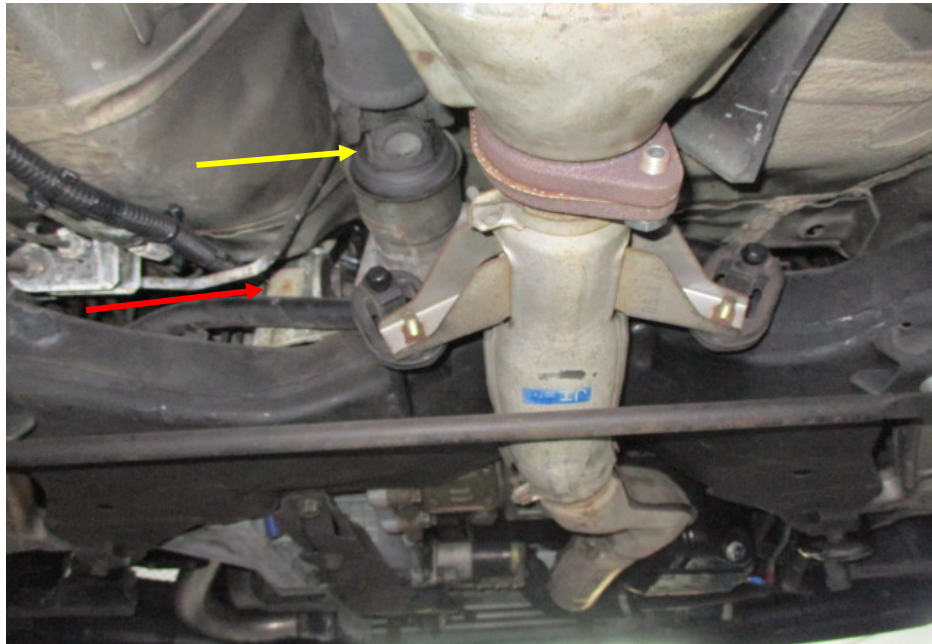
Photo 6 shows the propeller shaft (yellow arrow), which is connected to the transfer case of the Motor Car. This propeller shaft connects to the rear differential of the Motor Car, providing the drive to its rear wheels. The transmission assembly of the Motor Car is supported by 2 brackets. One at the front and one at the rear (red arrow) of the transmission assembly.
