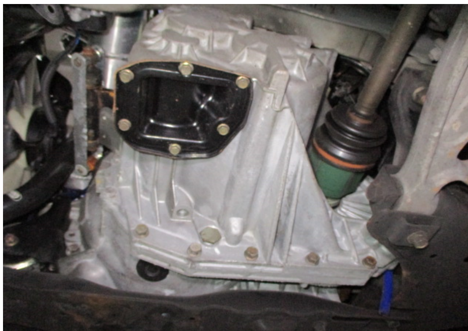
Photo 3 shows another view of the transmission assembly that was fitted on the Motor Car. This was the input side of the transmission, which houses the main shaft and various gear sets. There was no crack and/or hole observed on the transmission housing.
