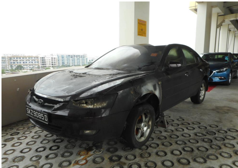
Photo 4 shows the general view of the left body of the Insured Vehicle at the time of our inspection. The Insured Vehicle was observed to have sustained extensive fire damage all around. Rust had accumulated all over the front and centre portion of the Insured Vehicle as a result of exposure to environmental condition for a period of time.
