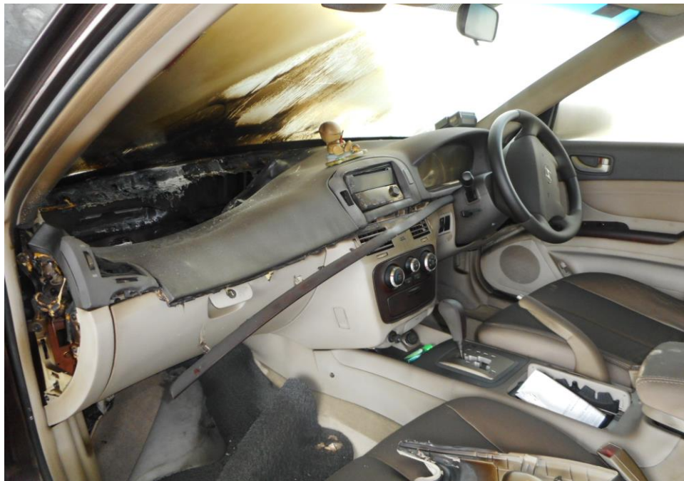
Photo 5 shows the general view of the interior compartment of the Insured Vehicle at the time of our inspection. Its interior compartment was had sustained heat and smoke damage as a result of the fire.
