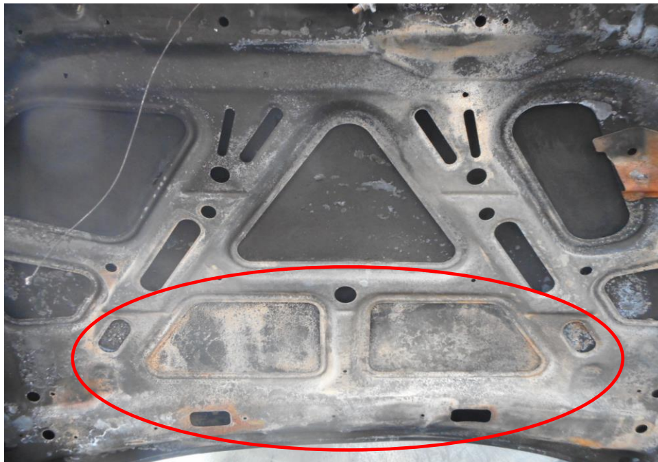
Photo 8 shows the underside of the front bonnet cover of the Insured Vehicle at the time of our inspection. The High heat intensity burn marks (whitish burn marks) and rust that had development found on the interior surface of the bonnet indicates that the fire had originated from the front portion of the Insured Vehicle.
