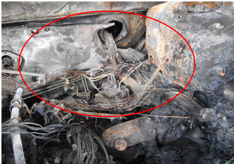
Photo 10 shows close up view of the engine compartment portion of the Insured Vehicle at the time of our inspection. The high heat intensity burn marks (whitish burn marks) and rust (circled) that had development found on the exterior surface indicates that the fire had originated from this area of the Insured Vehicle.
