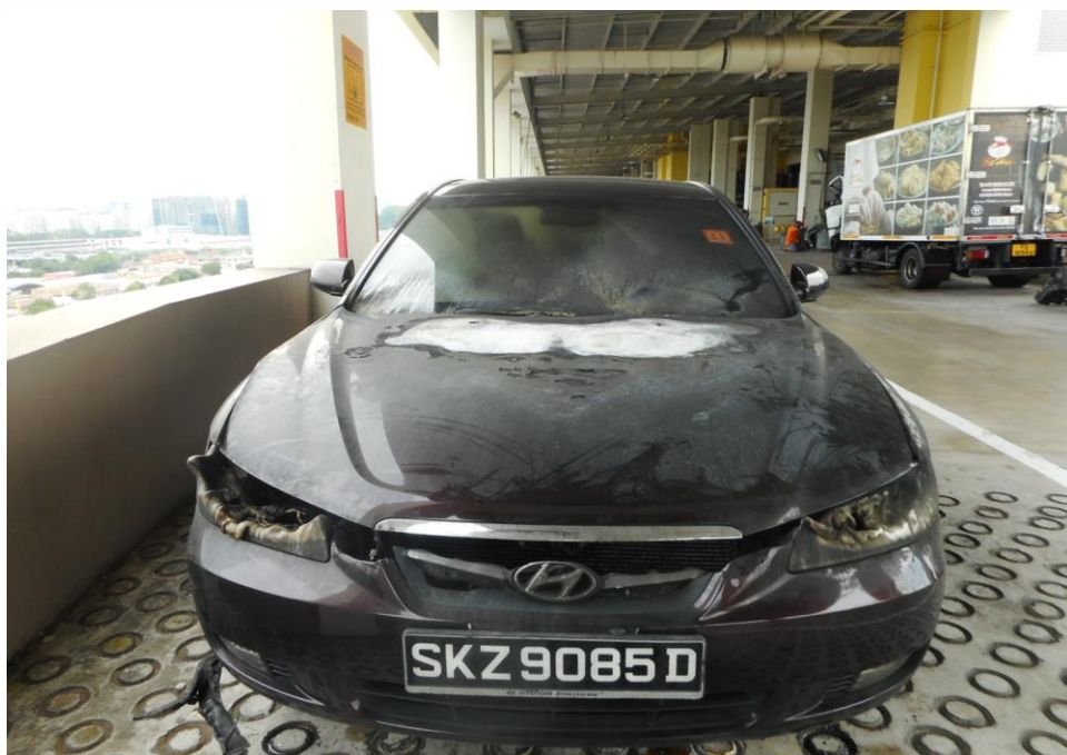
Photo 1 shows the general view of the front portion of the Insured Vehicle at the time of our inspection. The Insured Vehicle was observed to have sustained extensive fire damage all around. Its engine compartment completely burnt and interior compartment had sustained smoke and heat damage. Rust had accumulated all over the front engine portion of the Insured Vehicle as a result of exposure to environmental condition for a period of time.
