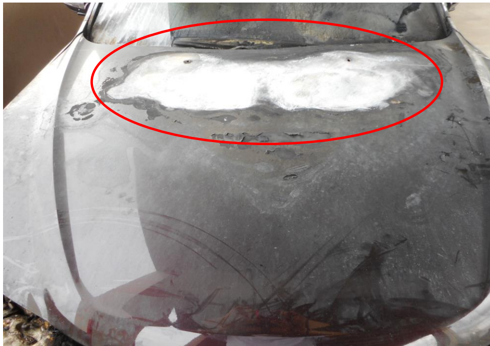
Photo 7 shows the exterior of the front bonnet of the Insured Vehicle at the time of our inspection. The high heat intensity burn marks (whitish burn marks) (circled) and rust that had development found on the exterior surface of the bonnet indicates that the fire had originated from the front portion of the Insured Vehicle.
