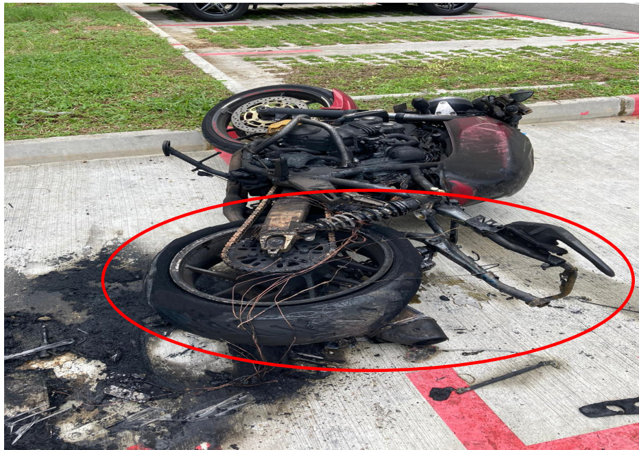
Photo 16 shows a closer view of the rear portion of the Insured Motorcycle at the incident scene after the fire was extinguished. The extent of fire damage observed indicates that the fire had started from the left rear portion (circled).
