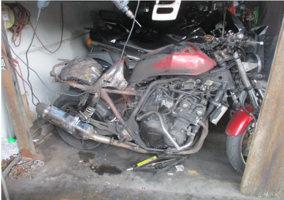
Photo 3 shows the general view of the right body of the Insured Motorcycle at the time of our inspection. The Insured Motorcycle was observed to have sustained extensive fire damage all around. Rust had accumulated all over the rear portion of the Insured Motorcycle as a result of exposure to environmental condition for a period of time.
