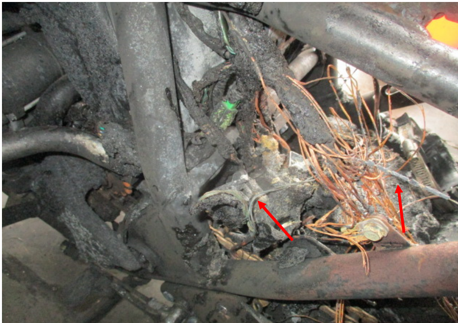
Photo 10 shows a closer view of the left rear portion of the Insured Motorcycle which was where the fire had likely started. We had found several stretches of wirings with greenish residue (arrowed). The presence of greenish residue indicates internal heating of copper wires, a sign of an electrical short circuit occurring.
