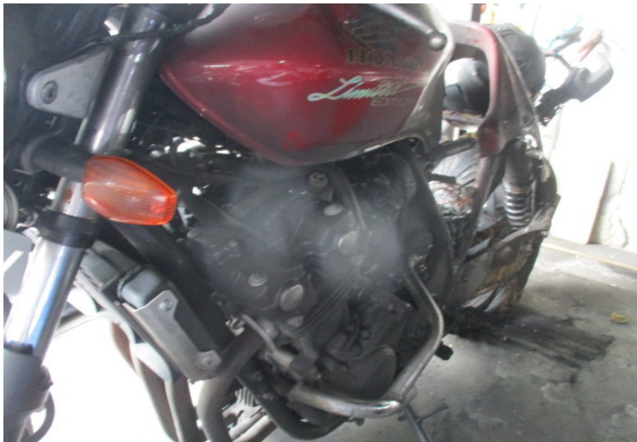
Photo 2 shows the general view of the left body of the Insured Motorcycle at the time of our inspection. The Insured Motorcycle was observed to have sustained extensive fire damage all around. Rust had accumulated all over the rear portion of the Insured Motorcycle as a result of exposure to environmental condition for a period of time.
