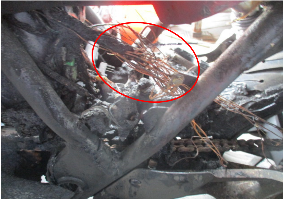
Photo 9 shows a closer view of the left rear portion of the Insured Motorcycle which was where the fire had likely started. We had found several stretches of wirings with greenish residue (circled). The presence of greenish residue indicates internal heating of copper wires, a sign of an electrical short circuit occurring.
