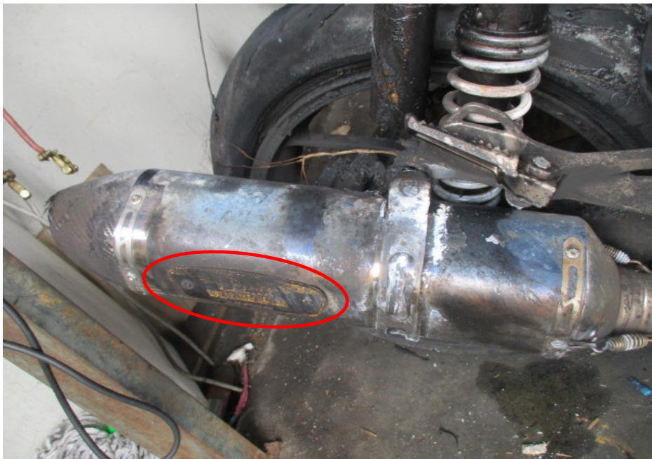
Photo 7 shows the right view of the non-standard rear exhaust muffler that was found to be fitted on the Insured Motorcycle at the time of our inspection. The brand of the rear exhaust muffler was 'YOSHIMURA' (circled).
