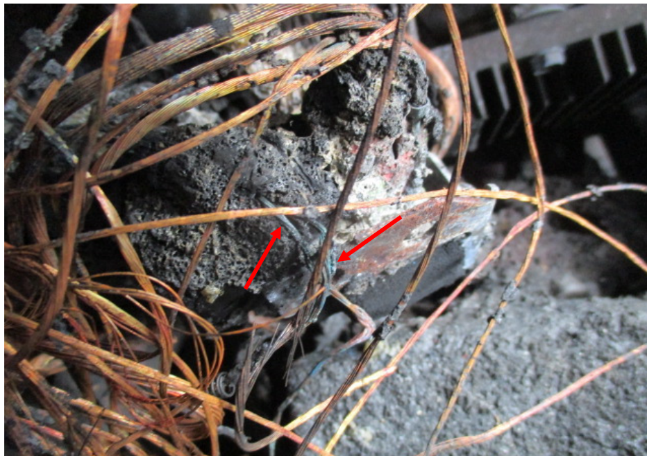
Photo 12 shows a close up view of the wirings with greenish residue (red arrows). The presence of greenish residue indicates internal heating of copper wires, a sign of an electrical short circuit occurring.
