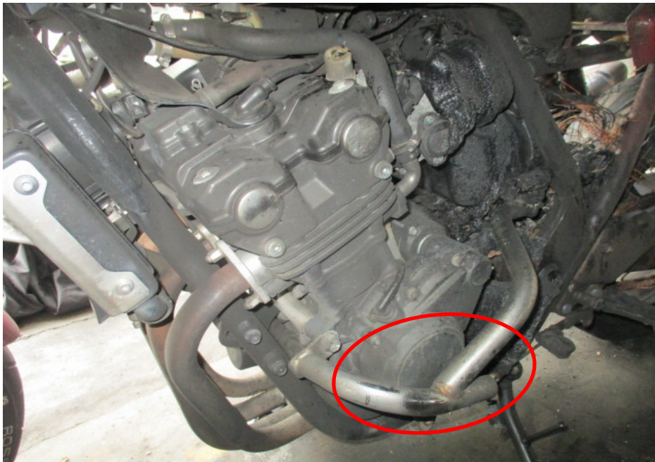
Photo 5 shows the left engine crash bar fitted on the Insured Motorcycle which had sustained visible fire damage (circled).
