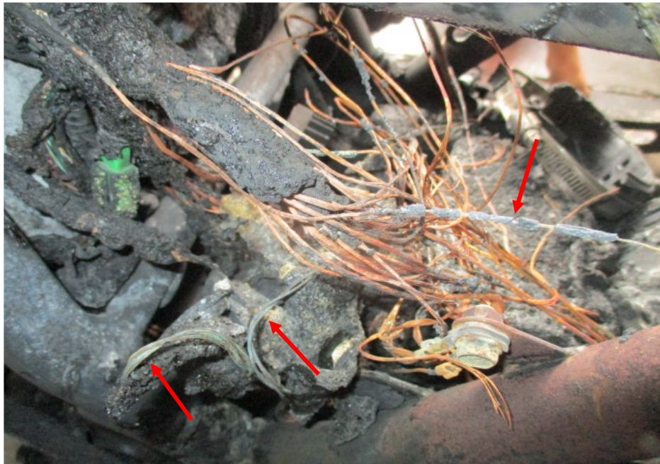
Photo 11 shows a closer view of the wirings with greenish residue (red arrows). The presence of greenish residue indicates internal heating of copper wires, a sign of an electrical short circuit occurring.
