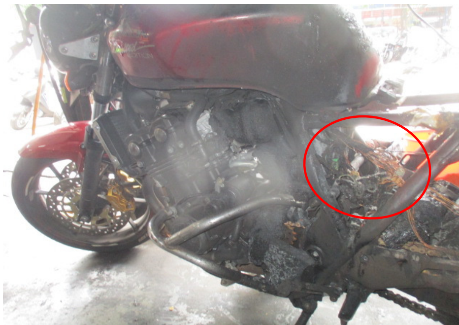
Photo 8 shows a view of the left body of the Insured Motorcycle. Upon closer examination of the left rear portion of the Insured Motorcycle which was where the fire had likely started, we had found several stretches of wirings with greenish residue (circled). These wirings were original factory fitted wirings. The presence of such greenish residue suggests occurrence of an electrical short circuit. The greenish residue is normally left behind from oxidation as a result of chemical reaction involving the copper wires.
