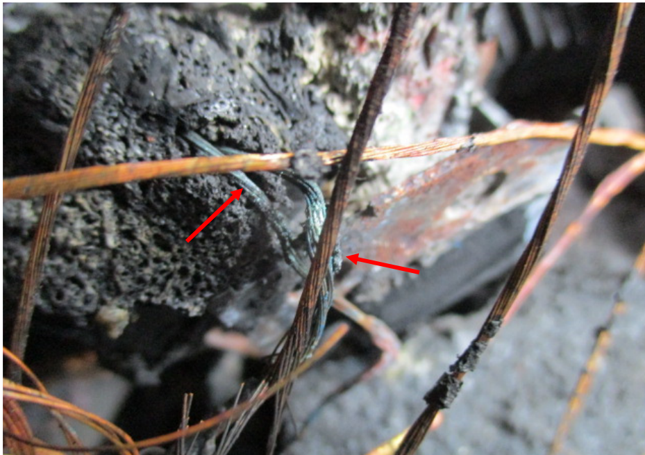
Photo 13 shows a close up view of the wirings with greenish residue (red arrows). The presence of greenish residue indicates internal heating of copper wires, a sign of an electrical short circuit occurring.
