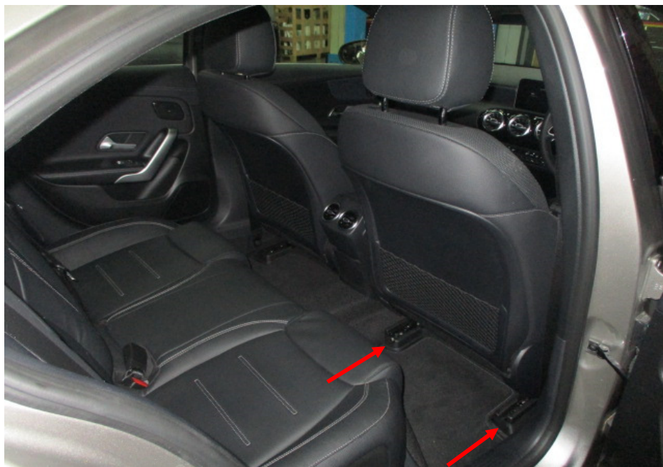
Photo 9 shows the interior compartment of the Motor Car. The seats of the Motor Car were secured via seat rails (arrowed) to the floorboard. All the seats of the Motor Car were fitted with a retractable seat belt reel and a pre-tensioner. The seat belts were tested and able to be fastened into the respective pre-tensions that were fitted on the side of each individual seat.
