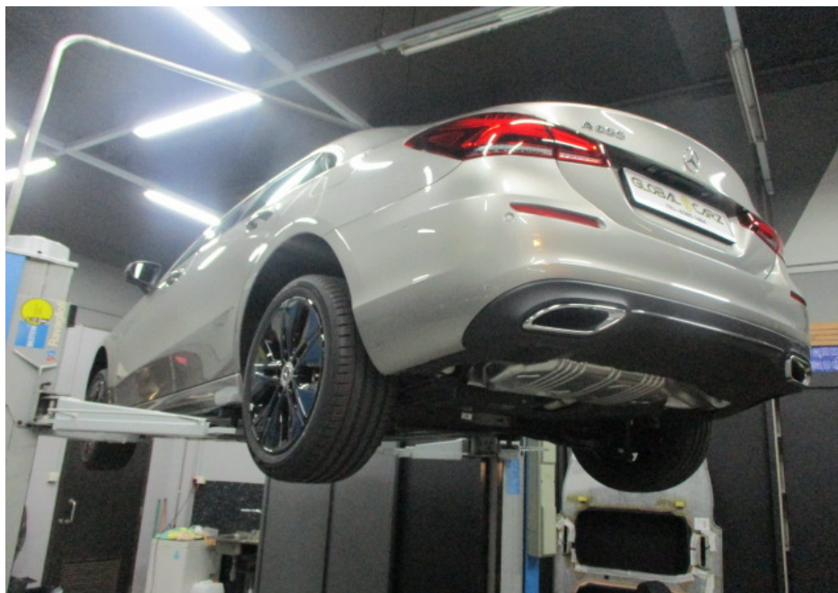
Photo 12 shows the Motor Car hoisted up for checks on its undercarriage. There was no sign(s) or indication(s) of fluid leakage and/or fluid stain(s) on the underside of the Motor Car. The undercarriage components of the Motor Car were also all observed to be intact and secured in an appropriate manner.
