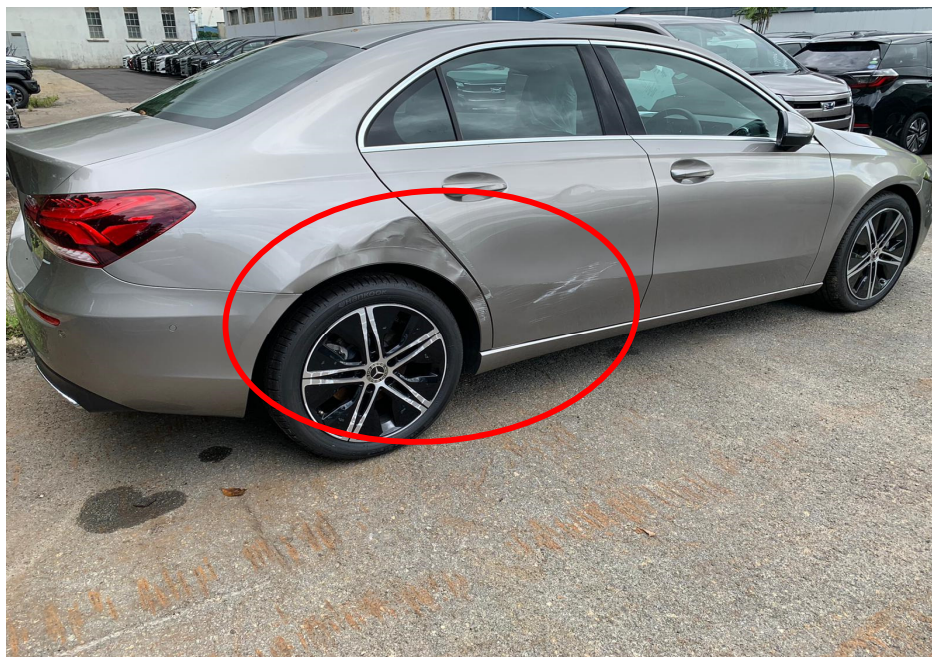
Photo 1 shows the right body of the Motor Car prior to any repairs being carried out (photograph provided to me). The Motor Car was observed to have sustained damages at its right side rear portion (circled). The body parts observed to be damaged had included its rear bumper, rear right fender, rear right door and rear right wheel rim amongst others.
