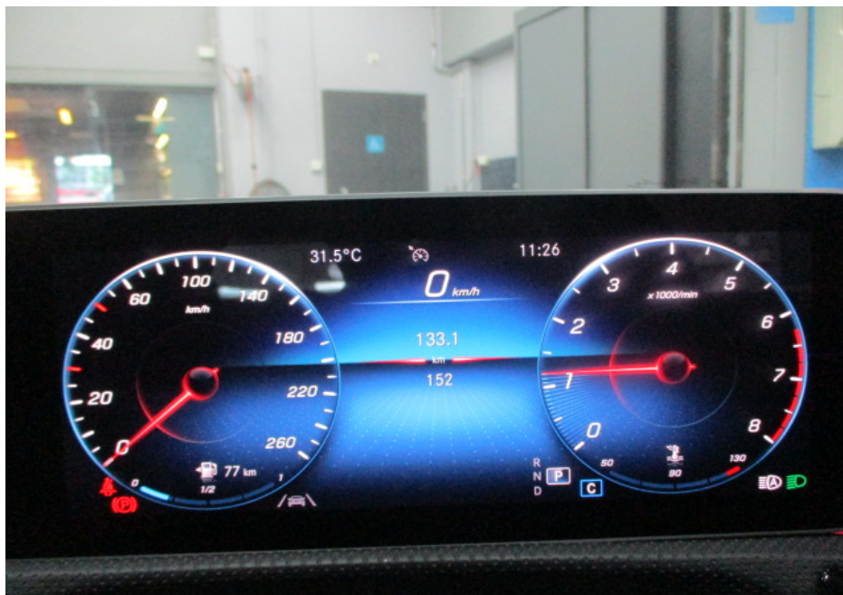
Photo 11 shows the respective warning lights no longer illuminated, indicating that there is no fault detected to the ABS, SRS, EPS and ESP systems of the Motor Car during the self-test. These electronic systems were hence in working condition at the time of my inspection.
