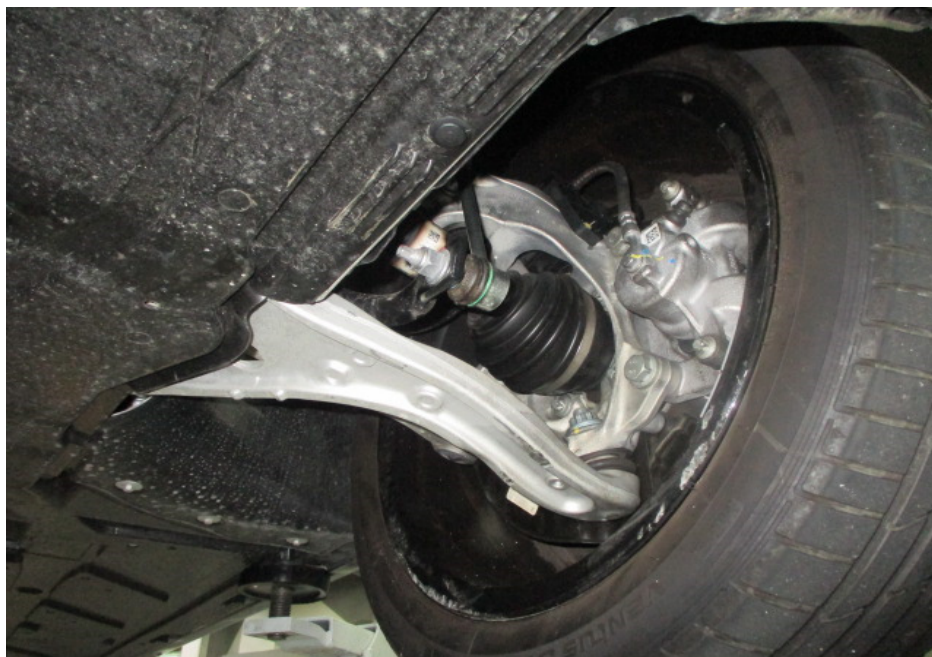
Photo 15 shows the various undercarriage components at the front left wheel of the Motor Car. The mechanical components, control arms and linkages were all found to be intact and secured in an appropriate manner. I also did not observe any fluid leak and/or fluid stain on the underside of the Motor Car.
