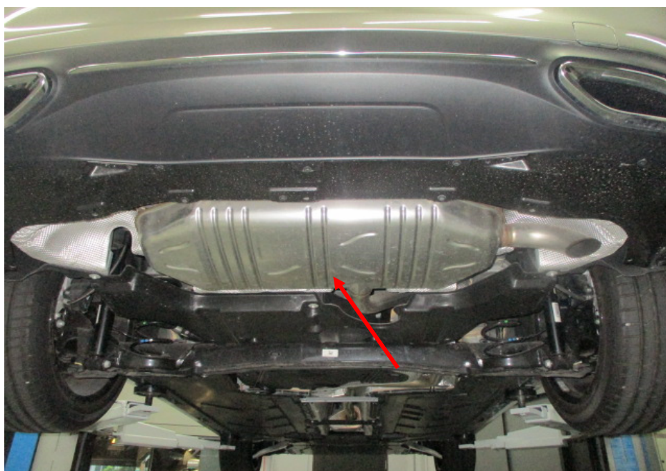
Photo 16 shows the Motor Car's rear muffler (arrowed). My examination of the Motor Car's exhaust system revealed no sign(s) or indication(s) of any cut or weld marks along its exhaust pipes and on its catalytic converter.
