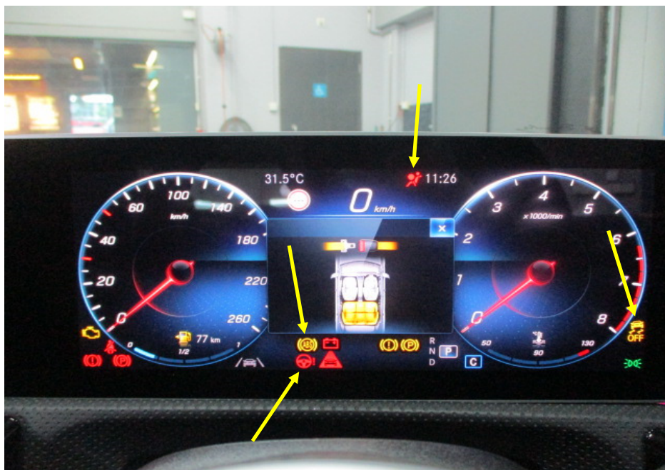
Photo 10 shows the warning lights for the various electronic safety features appearing on the instrument panel of the Motor Car during its self-test when the engine is cranked, in particular the ABS, SRS, EPS and ESP lights (arrowed).
