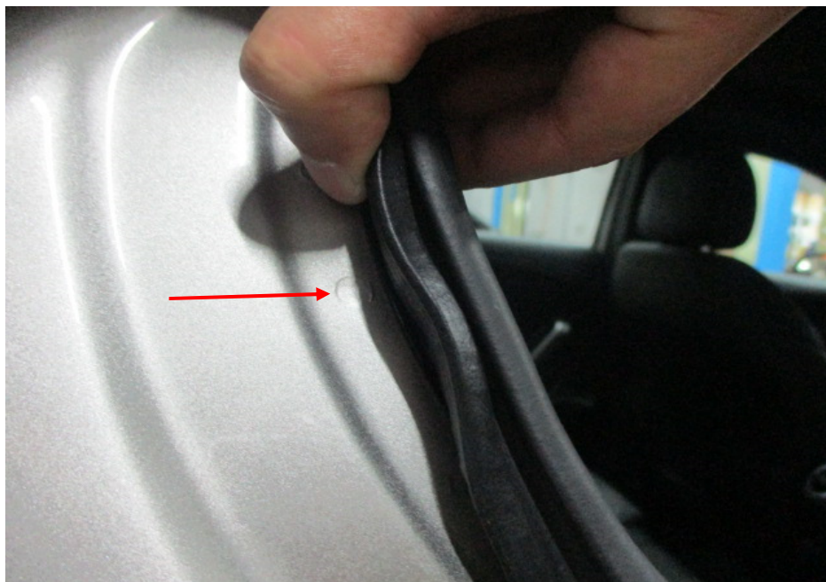
Photo 19 shows the right "C" pillar of the Motor Car. I did not find any weld marks other than original spot weld marks (arrowed) on the right "C" pillar of the Motor Car. In general, I had found all the non-detachable body panels of the Motor Car to be originally fitted at the time of my inspection.
