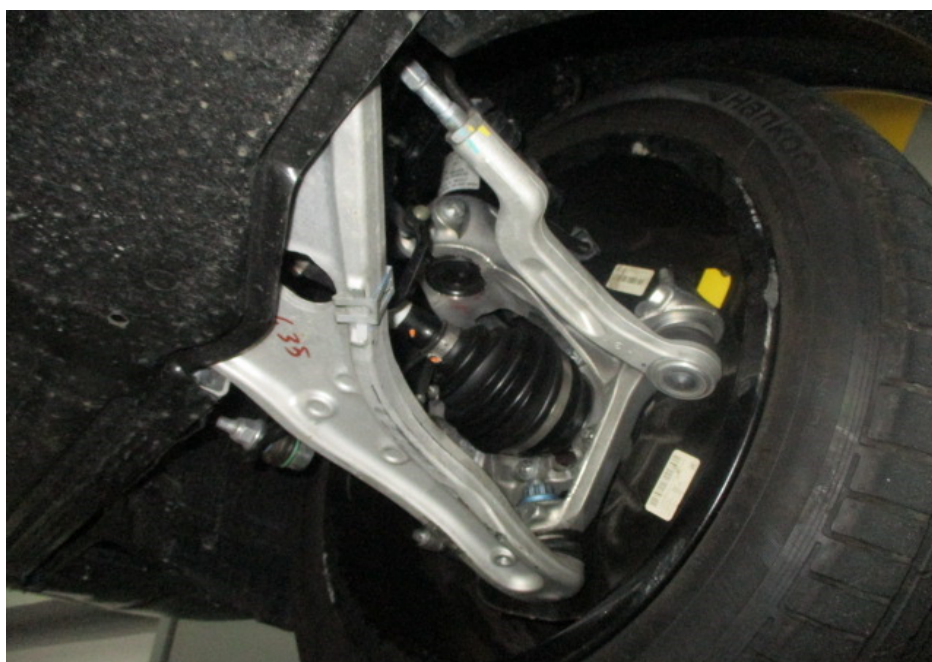
Photo 14 shows the various undercarriage components at the front right wheel of the Motor Car. The mechanical components, control arms and linkages were all found to be intact and secured in an appropriate manner.
