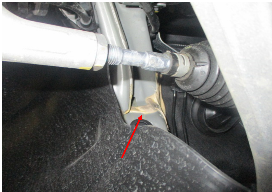
Photo 17 shows the chassis/structural body at the underside front right of the Motor Car. Visually, the original factory sealant (arrowed) at the joints along the chassis/structural body was untouched, indicating no work was done on the chassis/structural body of the Motor Car and that the chassis/structural body was originally fitted.
