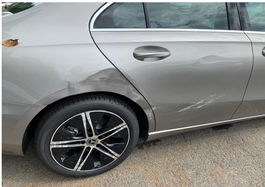
Photo 2 shows a closer view of the damaged right side rear portion of the Motor Car prior to any repairs being carried out (photograph provided to me). The rear bumper, rear right fender, rear right door and rear right wheel rim were observed to be damaged.
