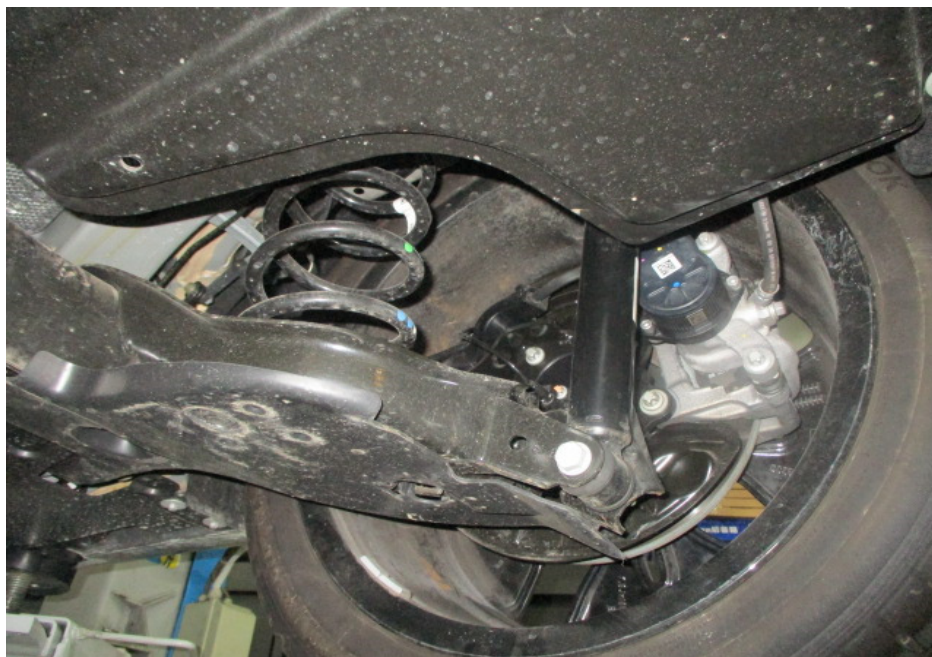
Photo 13 shows a general view of the control arms and linkages at the rear right wheel of the Motor Car. I did not observe any fluid leak and/or fluid stain on the underside of the Motor Car. All of the Motor Car's undercarriage components were observed to be intact and secured in an appropriate manner.
