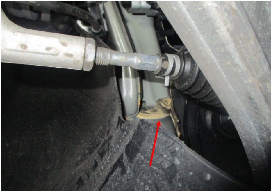
Photo 18 shows the chassis/structural body at the underside front right of the Motor Car. Visually, I did not find any weld marks other than original spot weld marks on the chassis/structural body of the Motor Car. The original factory sealant (arrowed) at the joints along the chassis/structural body was also untouched, indicating no work was done on the chassis/structural body of the Motor Car and that the chassis/structural body was originally fitted.
