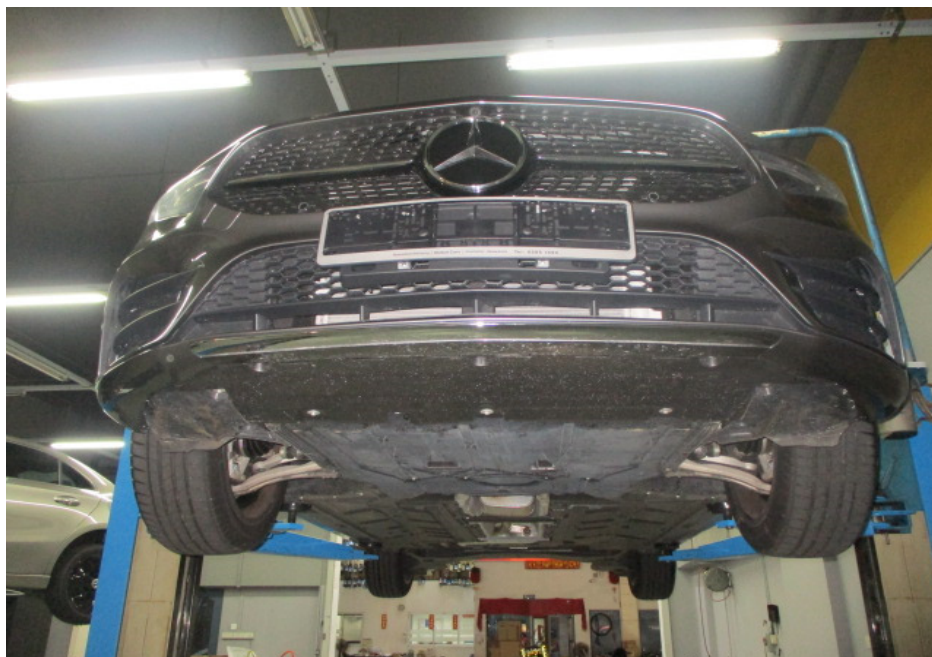
Photo 13 shows the Motor Car hoisted up for checks on its undercarriage. There was no sign(s) or indication(s) of fluid leakage and/or fluid stain(s) on the underside of the Motor Car. The undercarriage components of the Motor Car were also all observed to be intact and secured in an appropriate manner.
