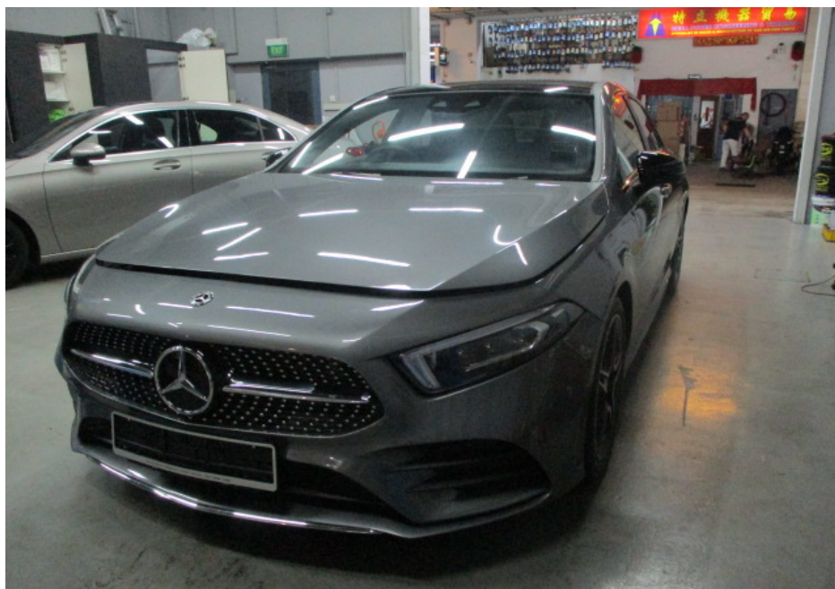
Photo 6 shows a general view of the front left body of the Motor Car at the time of my inspection. The Motor Car was observed to be in a relatively good general condition with no loose exterior fittings observed. The body parts at the frontal portion of the Motor Car were visually examined and it was observed that the repair/restoration works carried out to the damaged area of the Motor Car (refer photograph 1 & 2 above) were reasonably adequate and in order.
