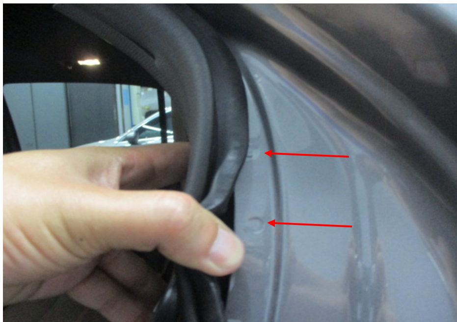
Photo 21 shows the left "C" pillar of the Motor Car. I did not find any weld marks other than original spot weld marks (arrowed) on the left "C" pillar of the Motor Car. In general, I had found all the non-detachable body panels of the Motor Car to be originally fitted at the time of my inspection.
