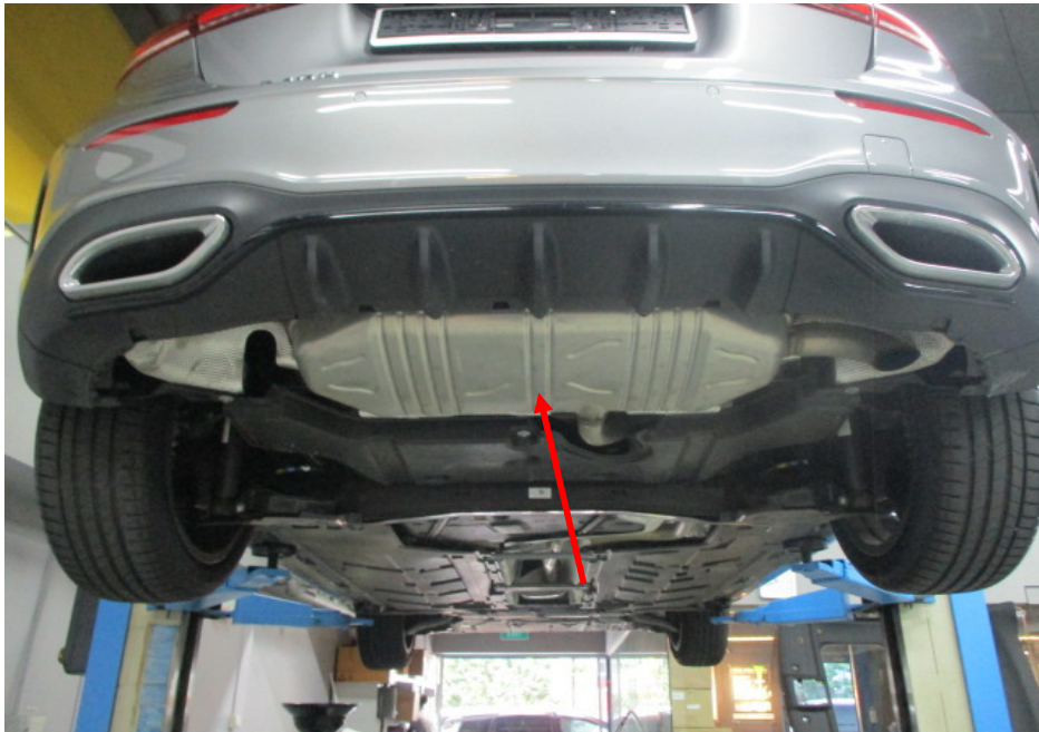
Photo 17 shows the Motor Car's rear muffler (arrowed). My examination of the Motor Car's exhaust system revealed no sign(s) or indication(s) of any cut or weld marks along its exhaust pipes and on its catalytic converter.
