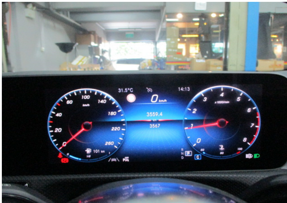
Photo 12 shows the respective warning lights no longer illuminated, indicating that there is no fault detected to the ABS, SRS, EPS and ESP systems of the Motor Car during the self-test. These electronic systems were hence in working condition at the time of my inspection.
