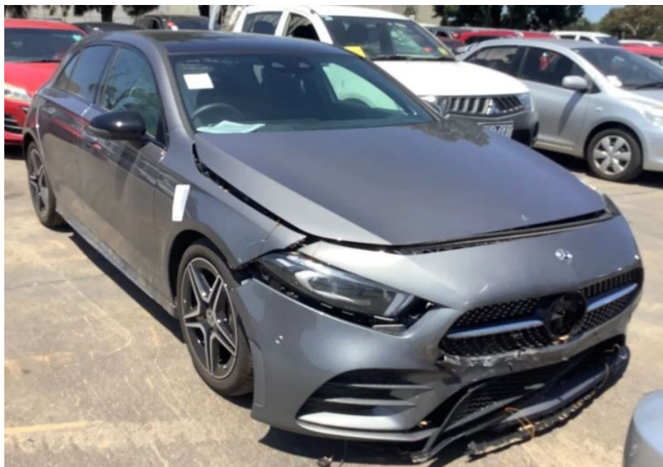
Photo 1 shows the front right body of the Motor Car prior to any repairs being carried out (photograph provided to me). The Motor Car was observed to have sustained damages at its frontal portion. The body parts observed to be damaged had included its front bumper, front bumper lower grille, front bumper lower skirt, radiator grille and front logo amongst others.
