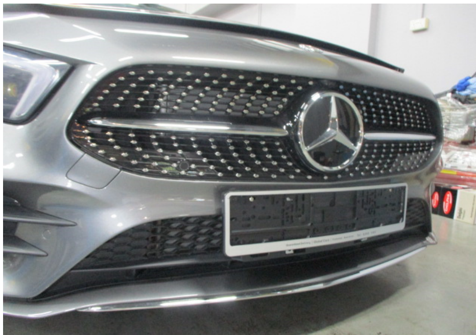
Photo 5 shows a closer view of the front bumper lower grille, front bumper lower skirt, radiator grille and logo of the Motor Car. The body parts at the frontal portion of the Motor Car were visually examined and it was observed that the repair/restoration works carried out to the damaged area of the Motor Car (refer photograph 1 & 2 above) were reasonably adequate and in order.
