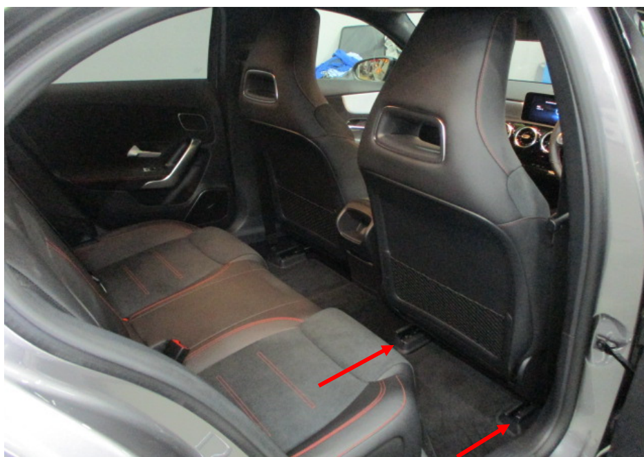
Photo 10 shows the interior compartment of the Motor Car. The seats of the Motor Car were secured via seat rails (arrowed) to the floorboard. All the seats of the Motor Car were fitted with a retractable seat belt reel and a pre-tensioner. The seat belts were tested and able to be fastened into the respective pre-tensions that were fitted on the side of each individual seat.
