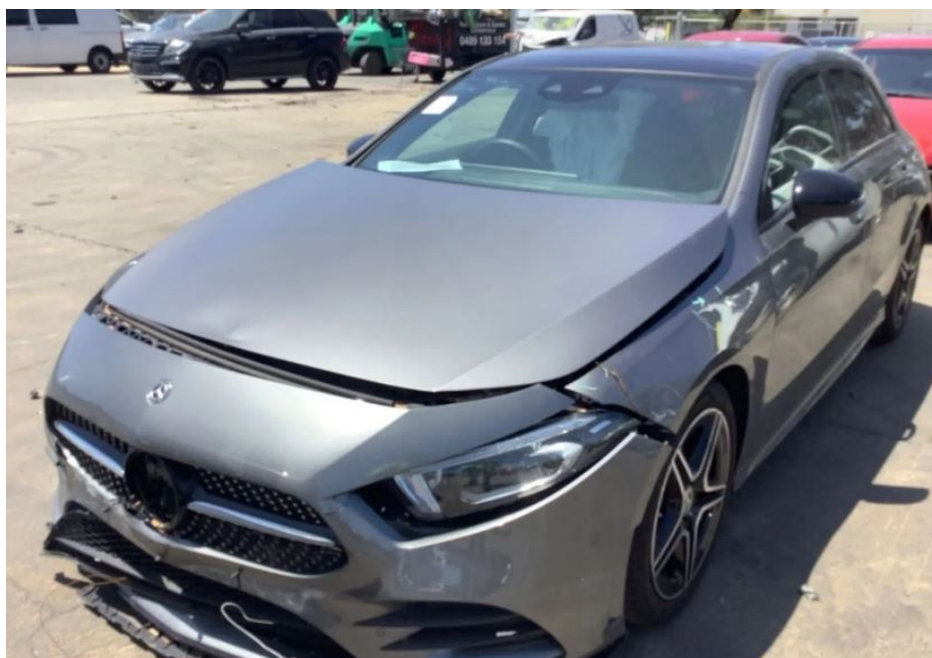
Photo 2 shows the front left body of the Motor Car prior to any repairs being carried out (photograph provided to me). The Motor Car was observed to have sustained damages at its frontal portion. The body parts observed to be damaged had included its front bumper, front bumper lower grille, front bonnet, front left fender, radiator grille and front logo amongst others.
